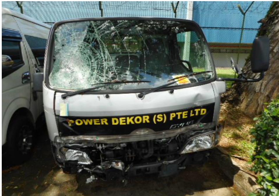
Photo 2 shows a general view of the Motor Lorry's frontal portion at the time of my inspection. It appeared to have sustained damage at its front portion. Its front windscreen, front body panel, front both headlamps and front bumper were damaged at the time of my inspection as a result of the accident.
