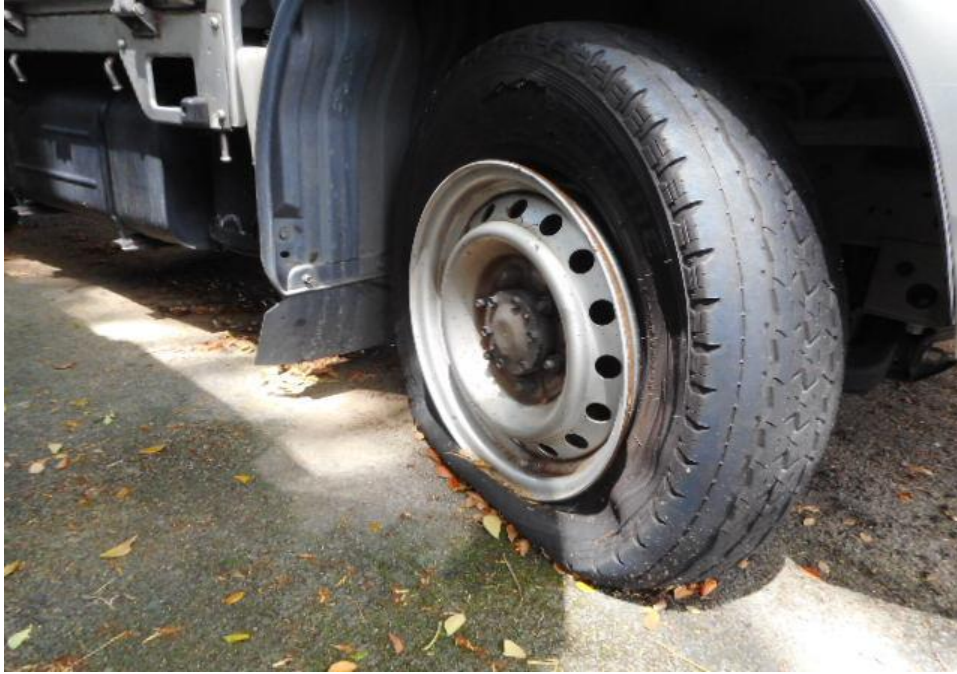
Photo 7 shows the condition of the front right tyre of the Motor Lorry, which was observed to of unserviceable condition with remaining tread depth of approximately 4.6mm. The tyre, was observed with cut marks on the outer and slip off the wheel rim as a result of the accident.
