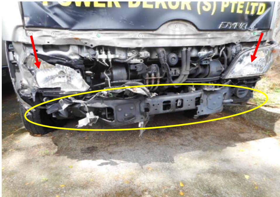
Photo 4 shows a close up view of the Motor Lorry's front portion at the time of my inspection. Its front both headlamps (arrowed) and front bumper (circled) was damage at the time of my inspection as a result of the accident.
