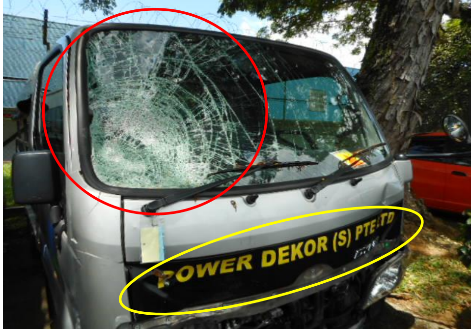
Photo 3 shows a close up view of the Motor Lorry's front portion at the time of my inspection. Its front windscreen (red circle) and front body panel (yellow circle) was damage at the time of my inspection as a result of the accident.
