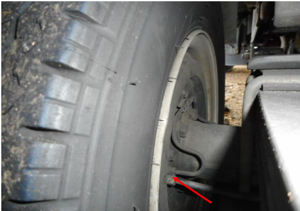
Photo 21 shows the brake pipe (arrowed) at the rear left wheel of the Motor Lorry. I did not observe any leakage of brake fluid at the time of my inspection of the Motor Lorry. My static tests of the Motor Lorry's braking system, along with my visual examination of the various mechanical components in the braking system had indicated that there was no internal leakage of pressure/vacuum. Hence the braking system of the Motor Lorry was likely to be in serviceable condition at the material time of accident.
