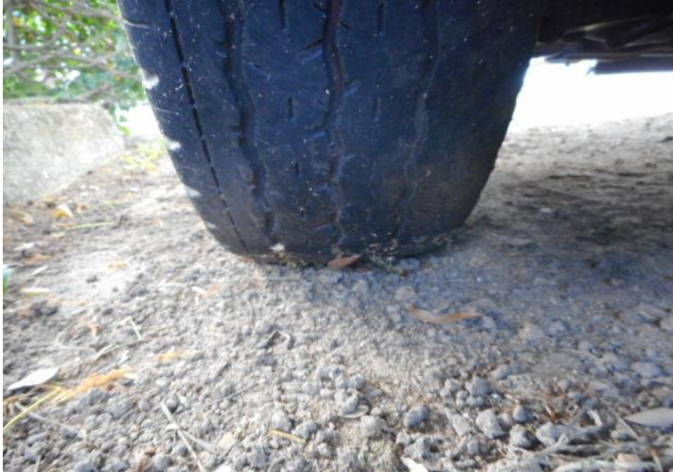
Photo 11 shows the condition of the rear right tyres of the Motor Lorry, which were observed to be in serviceable condition with remaining, tread depth of approximately 2.6mm. There was also no tear, cut or burst mark(s) on the outer and the inner sidewalls as well as across the tread of the 6 tyres that were fitted on the Motor Lorry.
