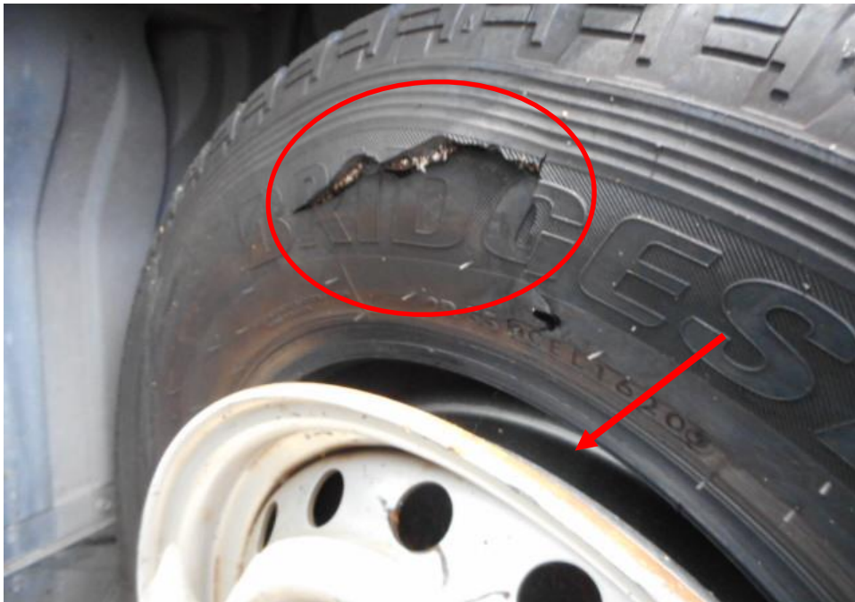
Photo 8 shows the close up condition of the front right tyre of the Motor Lorry, which was observed to of unserviceable condition with remaining tread depth of approximately 4.6mm. The tyre, was observed with cut marks (circled) on the outer and slip off the wheel rim (arrowed) as a result of the accident.
