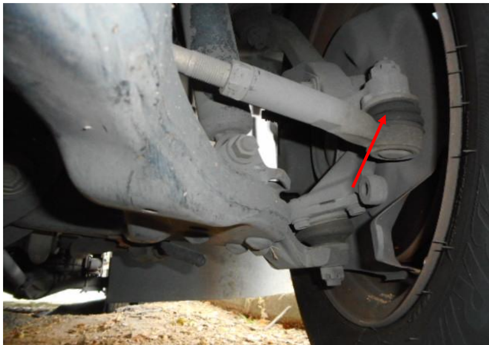
Photo 19 shows the various undercarriage components at the front left wheel of the Motor Lorry, in particular the steering tie rod end (arrowed). The various undercarriage components of the Motor Lorry were all found to be intact without any visible damage. There was also no sign of fluid stain(s) observed on the various undercarriage components.
