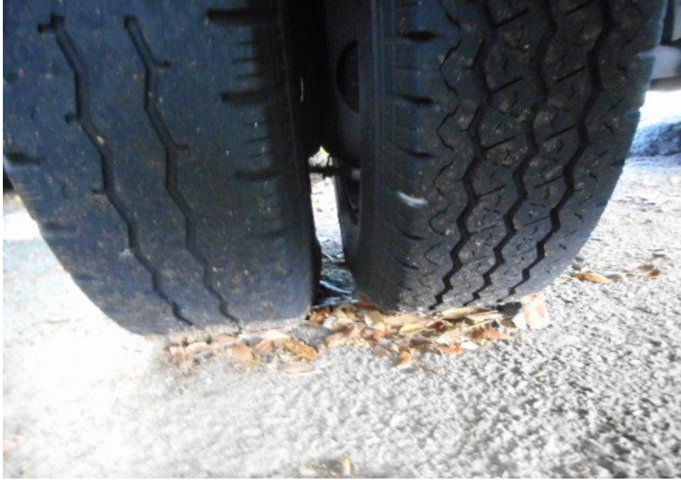
Photo 9 shows the condition of the rear right tyre of the Motor Lorry, which was observed to be in serviceable condition with remaining tread depth of approximately 2mm. The tyre, which was wrapped around standard steel wheel rim, it was observed to be sufficiently inflated for vehicular operation.
