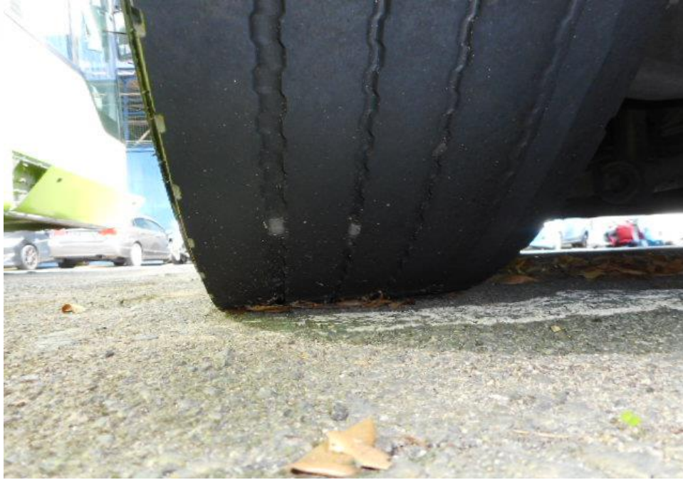
Photo 8 shows the condition of the front left tyres of the Motor Bus, which were observed to be in serviceable condition with remaining tread depth of approximately 5.6mm. There was also no tear, cut or burst mark(s) on the outer and the inner sidewalls as well as across the tread of the 6 tyres that were fitted on the Bus.
