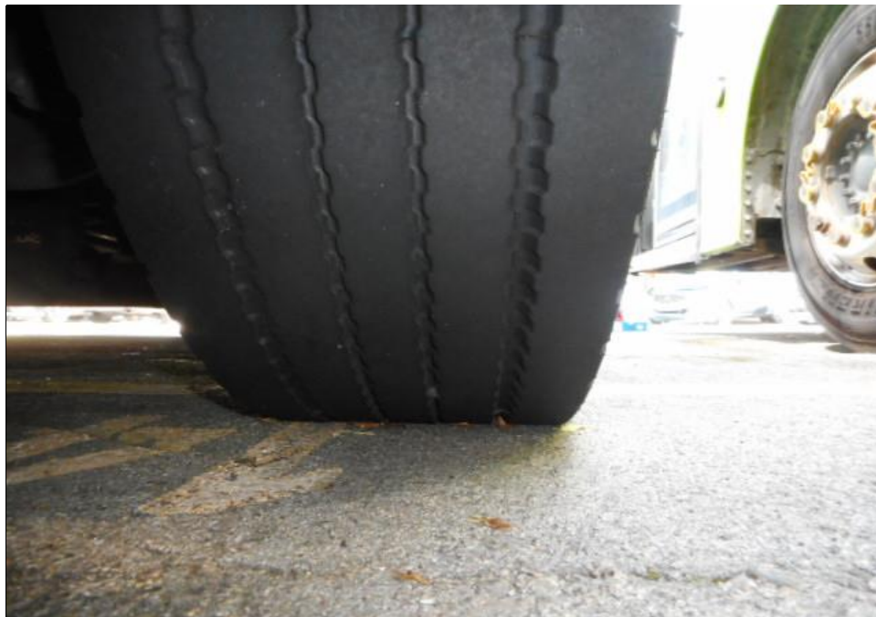
Photo 5 shows the condition of the front right tyre of the Motor Bus, which was observed to be in serviceable condition with remaining tread depth of approximately 6.8 mm. The tyre, which was wrapped around standard steel wheel rim, was also observed to be sufficiently inflated for vehicular operation. There was no tear, cut or burst mark(s) on the outer and the inner sidewalls as well as across the tread of the 6 tyres that were fitted on the Motor Bus.
