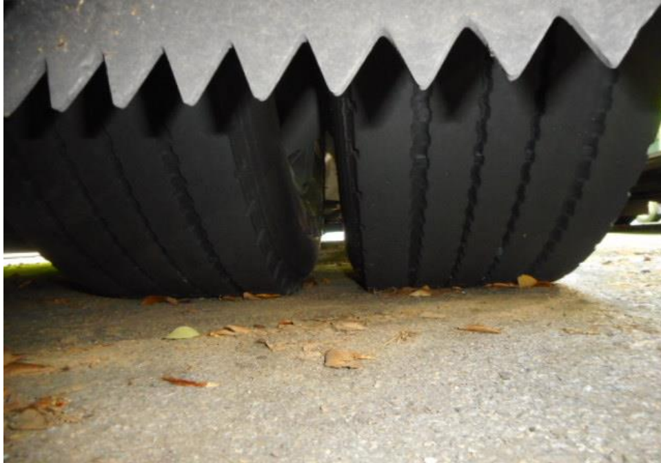
Photo 6 shows the condition of the rear right tyre of the Motor Bus, which was observed to be in serviceable condition with remaining tread depth of approximately 7.7mm. The tyre, which was wrapped around standard steel wheel rim, was also observed to be sufficiently inflated for vehicular operation.
