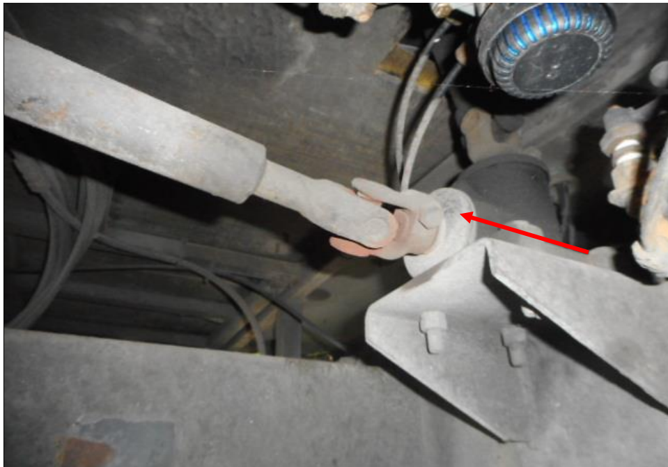
Photo 16 shows the steering box component (arrowed) at the undercarriage of the Motor Bus was found to be intact without any visible damage. There was also no sign of fluid stain(s) observed on the various undercarriage components.
