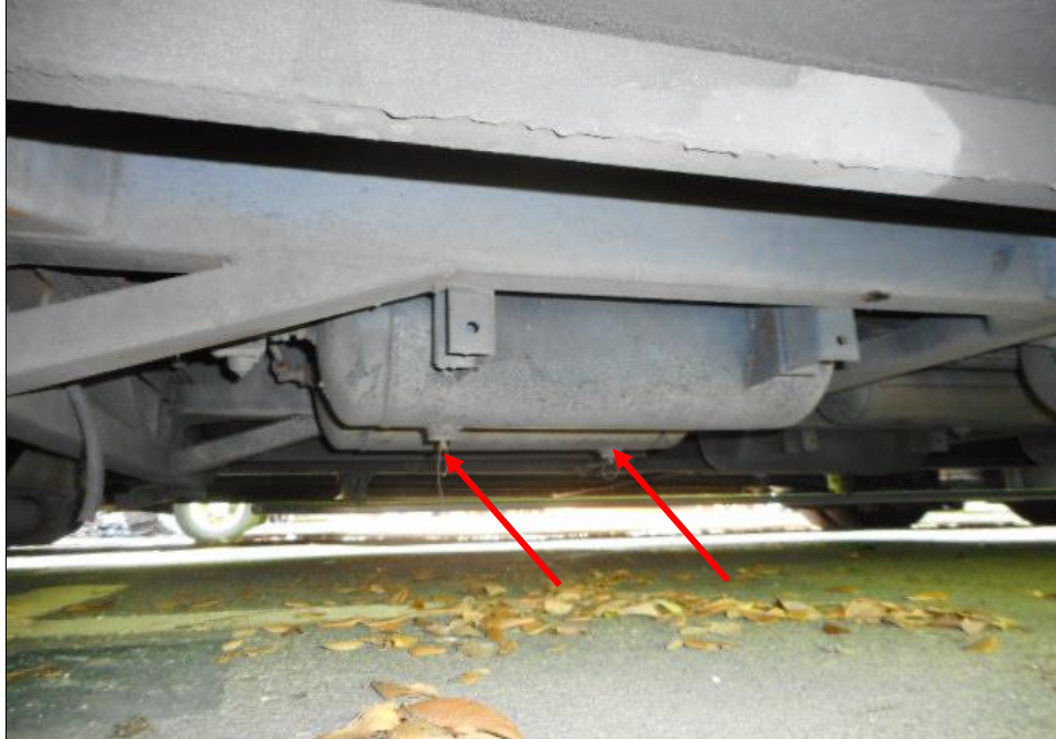
Photo 13 shows the air brake cylinders (arrowed) at the undercarriage of the Motor Bus. I did not observe any leakage of air brake fluid at the time of my inspection of the Motor Bus. My visual examination of the various mechanical components in the braking system had indicated that there was no internal leakage of pressure/vacuum and there components were generally in good condition.
