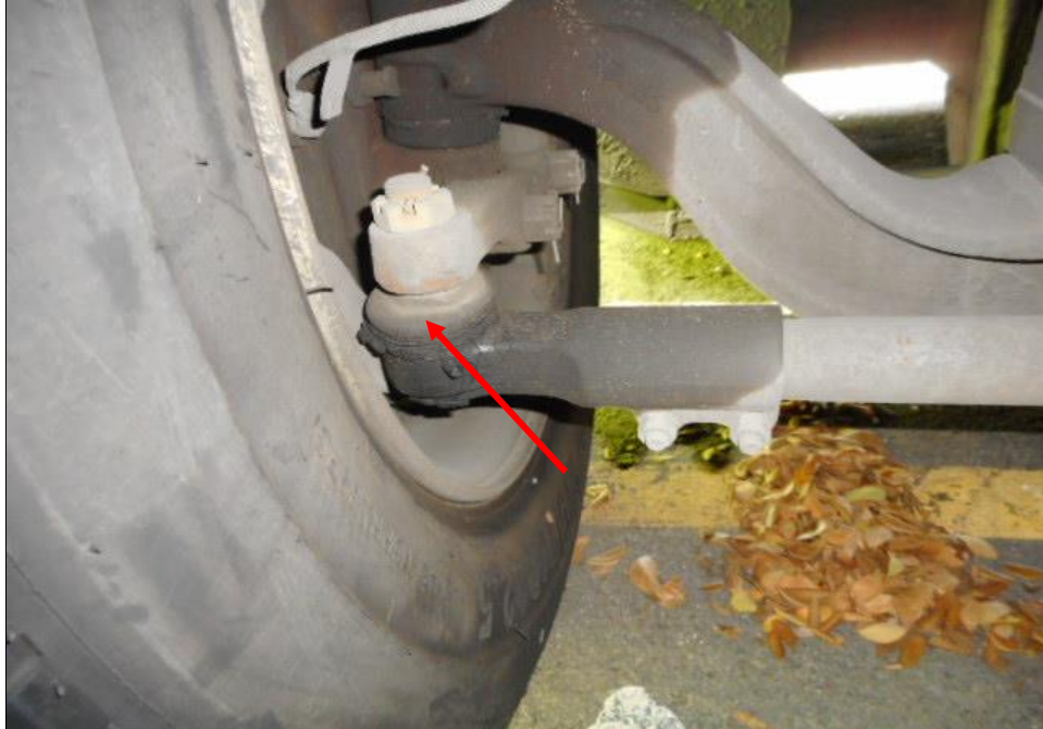
Photo 15 shows the various undercarriage components at the front left wheel of the Motor Bus, in particular the steering tie rod end (arrowed). The various undercarriage components of the Motor Bus were all found to be intact without any visible damage. There was also no sign of fluid stain(s) observed on the various undercarriage components.
