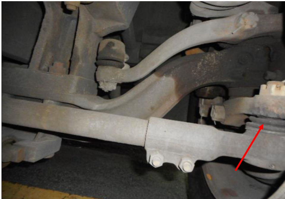
Photo 14 shows the various undercarriage components at the front right wheel of the Motor Bus, in particular the steering tie rod end (arrowed). The various steering components were all found to be intact, suggesting that the steering system of the Motor Bus was likely to be in serviceable condition at the material time of accident. There was also no sign of fluid stain(s) observed on the various undercarriage components.
