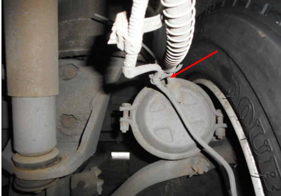
Photo 11 shows the brake pipe (arrowed) at the front right wheel of the Motor Bus. I did not observe any leakage of brake fluid at the time of my inspection of the Motor Bus. My static tests of the Motor Bus's braking system, along with my visual examination of the various mechanical components in the braking system, had indicated that there was no internal leakage of pressure/vacuum and there components were generally in good condition.
