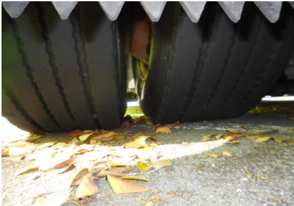
Photo 7 shows the condition of the rear left tyres of the Motor Bus, which was observed to be in serviceable condition with remaining tread depth of approximately 9.5mm. The tyres, which were wrapped around standard steel wheel rim, were also observed to be sufficiently inflated for vehicular operation. There was also no damage found on all 6 steel wheel rims of the Bus.
