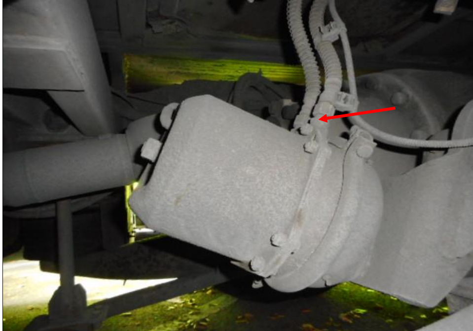
Photo 9 shows the brake pipe (arrowed) at the rear right wheel of the Motor Bus. I did not observe any leakage of brake fluid at the time of my inspection of the Motor Bus. My visual examination of the various mechanical components in the braking system, had indicated that there was no internal leakage of pressure/vacuum and there components were generally in good condition.
