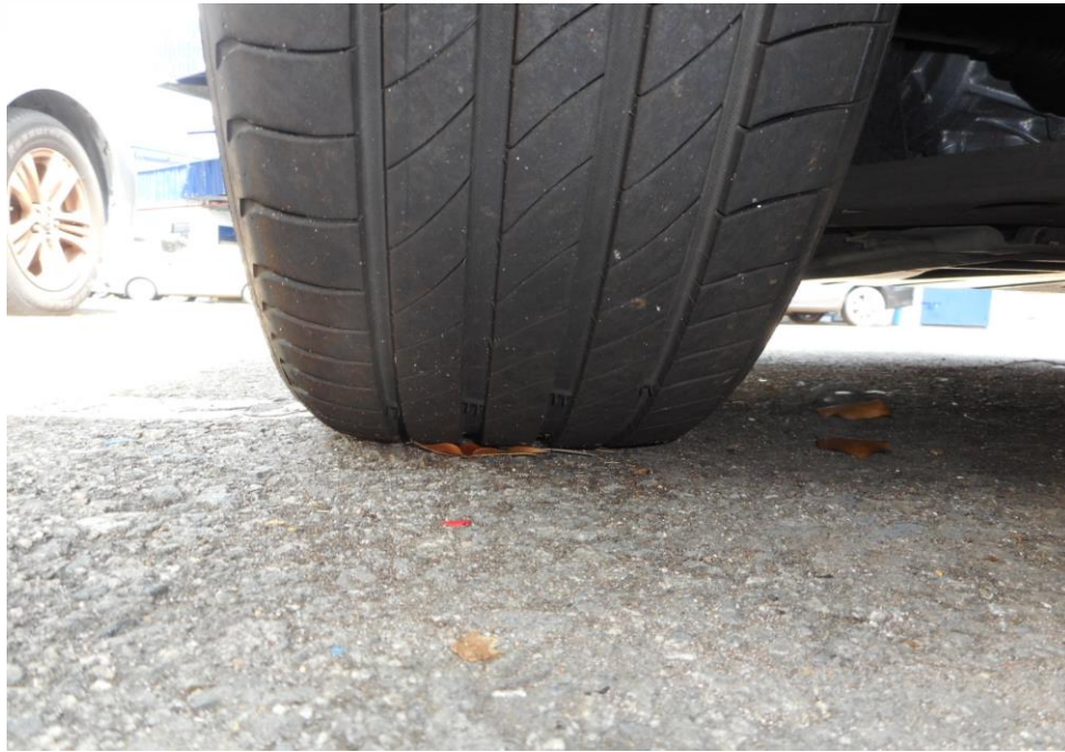
Photo 10 shows the condition of the front left tyre of the Motor Car, which was observed to be in serviceable condition with remaining tread depth of approximately 6mm. There was also no tear, cut or burst mark(s) on the outer and the inner sidewalls as well as across the tread of the Motor Car's 4 tyres.
