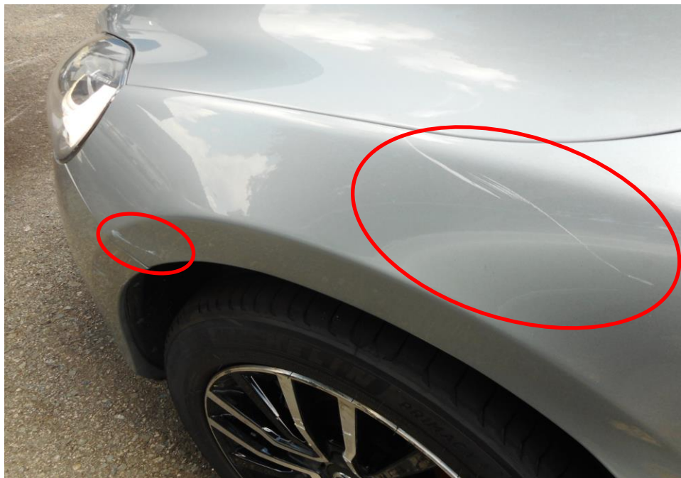
Photo 3 shows a close up view of the Motor Car's front body at the time of my inspection. The front portion of the Motor Car was observed to have sustained damage. Its front left fender (circled) was the body part that were damaged as a result of the accident.
