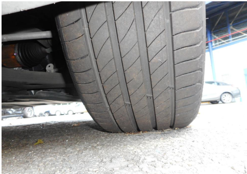
Photo 7 shows the condition of the front right tyre of the Motor Car, which was observed to be in serviceable condition with remaining tread depth of approximately 6.2mm. The tyre was sufficiently inflated for vehicular operation with no tear, cut or burst mark(s) on the outer and the inner sidewalls as well as across the tread. The 4 tyres of the Motor Car were wrapped around standard steel wheel rims without any damage.
