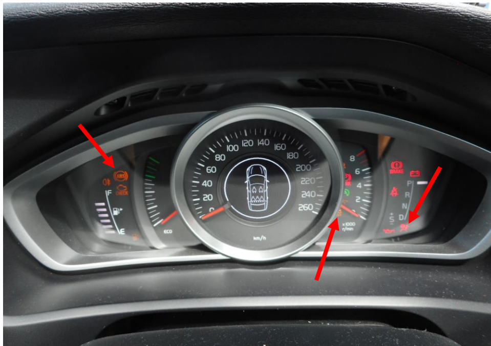
Photo 23 shows the warning light for Anti-Lock Brake System (ABS) and Traction Control System (TCS) and Supplemental Restraint System (SRS) (arrowed) appearing on the instrument panel of the Motor Car during the self-test of its various electronic operating systems when its engine was cranked.
