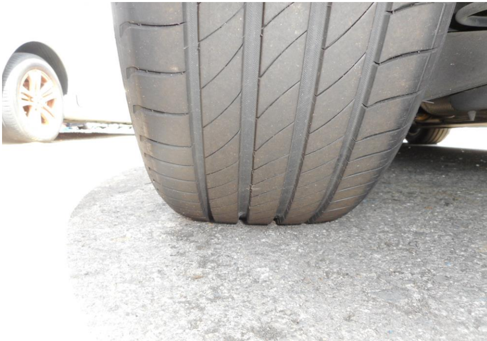
Photo 9 shows the condition of the rear left tyre of the Motor Car, which was observed to be in serviceable condition with remaining tread depth of approximately 6.4mm. The tyre, which was wrapped around steel wheel rim, was also observed to be sufficiently inflated for vehicular operation. The 4 tyres of the Motor Car were wrapped around standard steel wheel rims.
