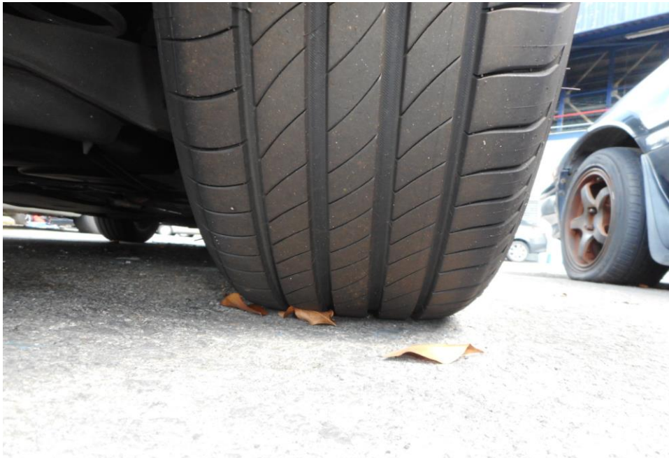
Photo 8 shows the condition of the rear right tyre of the Motor Car, which was observed to be in serviceable condition with remaining tread depth of approximately 6.4mm. The tyre was also observed to be sufficiently inflated for vehicular operation with no tear, cut or burst mark(s).
