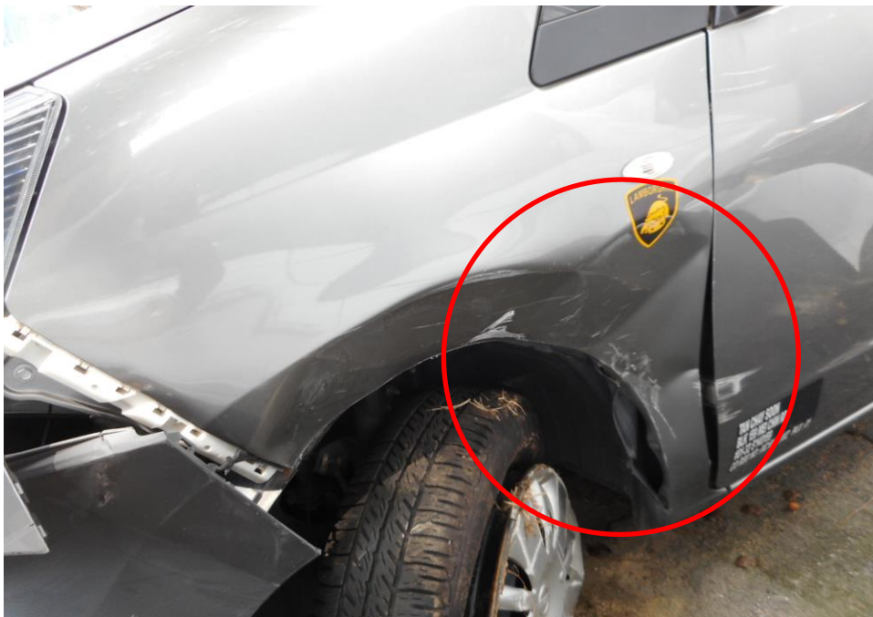
Photo 5 shows the close up view of the Motor Van's front body at the time of my inspection. The Motor Van was observed to have sustained damage at its front portion. Its front left fender (circled) were amongst the body parts that were damaged as a result of the accident.
