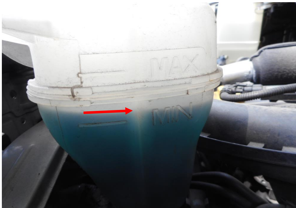
Photo 22 shows checks being carried out to the engine coolant of the Motor Van at the time of my inspection. The engine coolant was observed to be of sufficient level (arrowed) and without any visible contamination.
