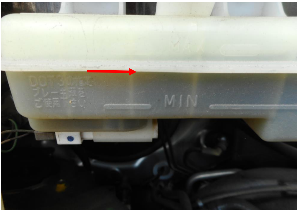
Photo 20 shows the brake fluid reservoir of the Motor Van at the time of my inspection. The brake fluid was observed to be of sufficient level (arrowed) and without any visible contamination.
