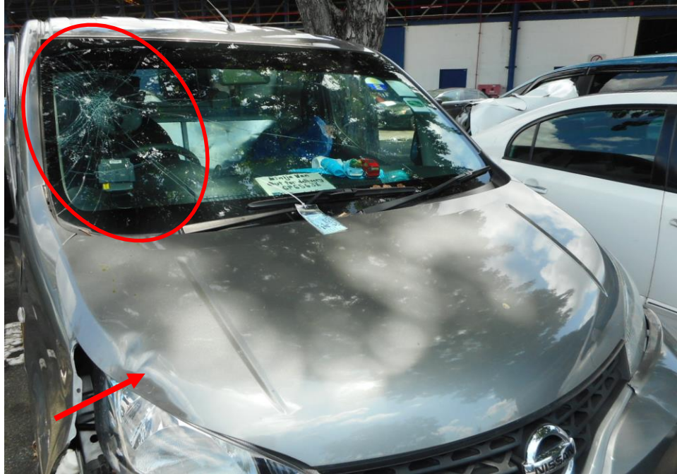
Photo 2 shows the close up view of the Motor Van's front body at the time of my inspection. The Motor Van was observed to have sustained damage at its front portion. Its front bonnet (arrowed) and front windscreen (circled) were amongst the body parts that were damaged as a result of the accident.
