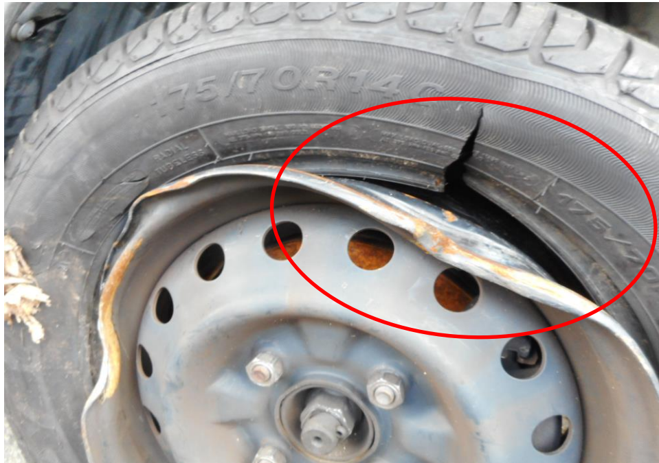
Photo 10 shows the close up view of the condition of the front right tyre of the Motor Van, which was observed to be unserviceable condition with remaining tread depth of approximately 4.7mm. The tyre was observed with cut mark(s) on the outer sidewalls and there was damage observed on the wheel rims (circled) as a result of the accident.
