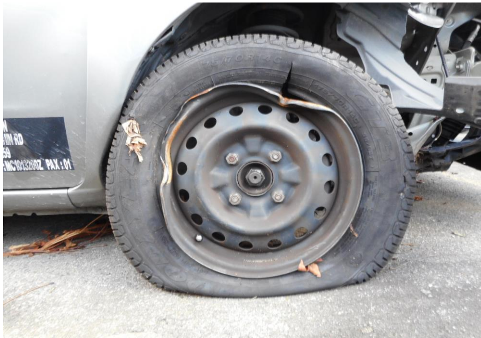
Photo 9 shows the condition of the front right tyre of the Motor Van, which was observed to be unserviceable condition with remaining tread depth of approximately 4.7mm. The tyre was observed with cut mark(s) on the outer sidewalls and there was damage observed on the wheel rims as a result of the accident.
