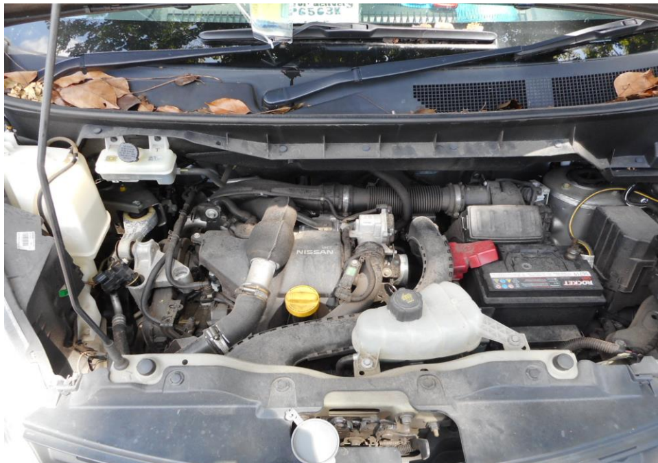
Photo 18 shows a general view of the Motor Van's engine compartment. The various parts and components inside the engine compartment were unaffected by the accident. There was also no sign(s) or indication(s) of fluid leakage and/or fluid stain within the engine compartment.
