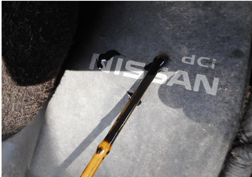
Photo 21 shows the engine oil dip stick of the Motor Van at the time of my inspection. The engine oil was observed to be of sufficient level and without any visible contamination.
