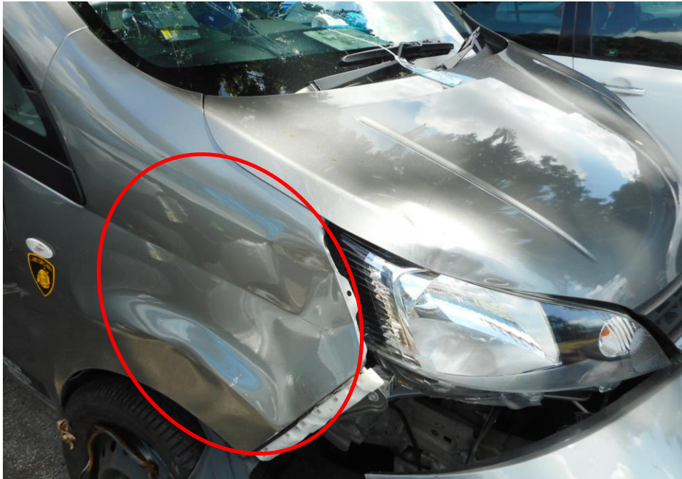
Photo 4 shows the close up view of the Motor Van's front body at the time of my inspection. The Motor Van was observed to have sustained damage at its front portion. Its front right fender (circled) were amongst the body parts that were damaged as a result of the accident.
