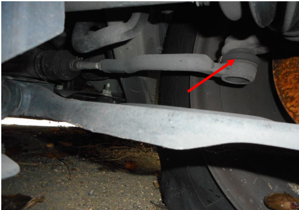
Photo 29 shows the various undercarriage components at the front left wheel of the Motor Van, in particular the steering tie rod (red arrow). The various steering components were all found to be intact, suggesting that the steering system of the Motor Van was likely to be in serviceable condition at the material time of accident. There was also no sign of fluid stain observed on the various undercarriage components at the front left wheel of the Motor Van.
