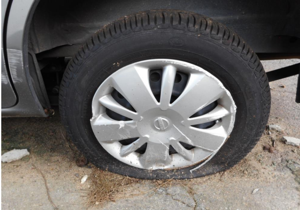
Photo 14 shows the condition of the rear left tyre of the Motor Van, which was observed to be unserviceable condition with remaining tread depth of approximately 5.7mm. The tyre was observed with cut mark(s) on the outer sidewalls and there was damage observed on the wheel rims as a result of the accident.
