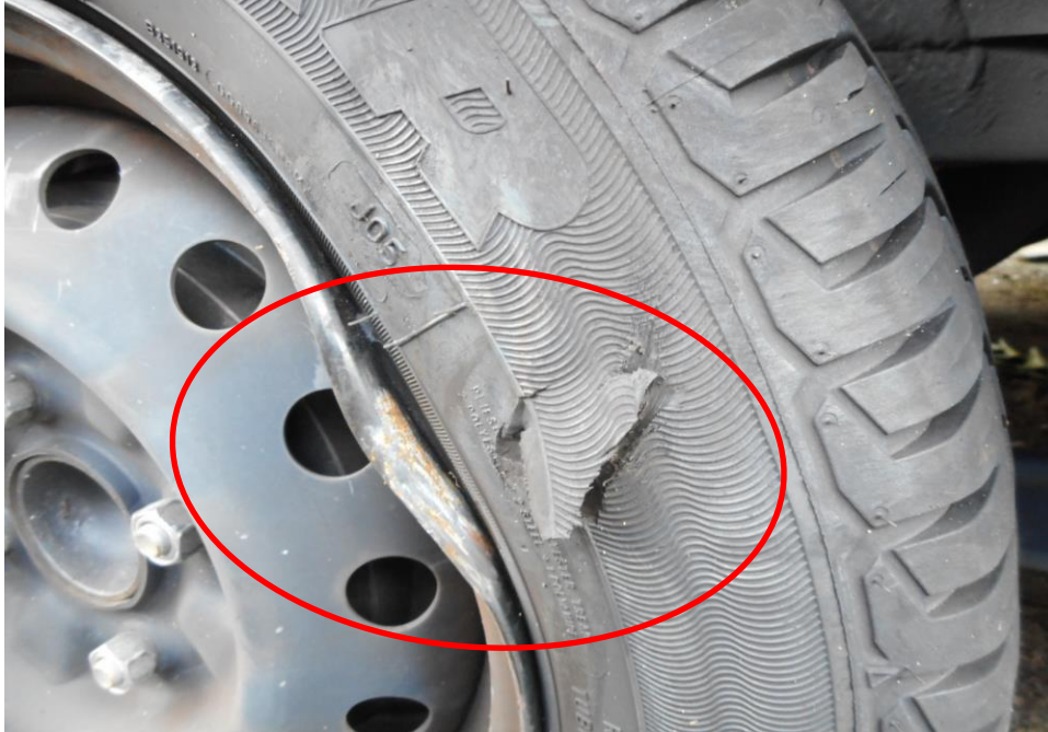
Photo 12 shows the close up view of the condition of the rear right tyre of the Motor Van, which was observed to be in serviceable condition with remaining tread depth of approximately 6.5mm. The tyre was observed with cut marks and wheel rim damage (circled) as a result of the accident, however it was observed to be sufficiently inflated for vehicular operation
