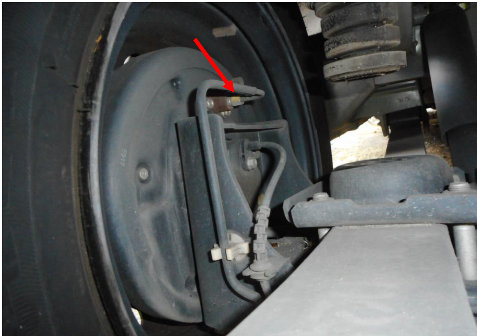
Photo 25 shows the brake hose/pipe (arrowed) at the rear left wheel of the Motor Van. I did not observe any leakage of brake fluid at the time of my inspection of the Motor Van. Static tests of the Motor Van's braking system had indicated that there was no internal leakage of pressure/vacuum. The undercarriage components of the Motor Van were also all found to be intact and without any visible damage.
