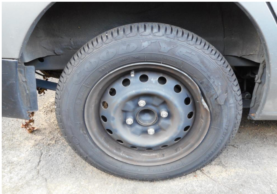
Photo 11 shows the condition of the rear right tyre of the Motor Van, which was observed to be in serviceable condition with remaining tread depth of approximately 6.5mm. The tyre was observed with cut marks and wheel rim damage as a result of the accident, however it was observed to be sufficiently inflated for vehicular operation
