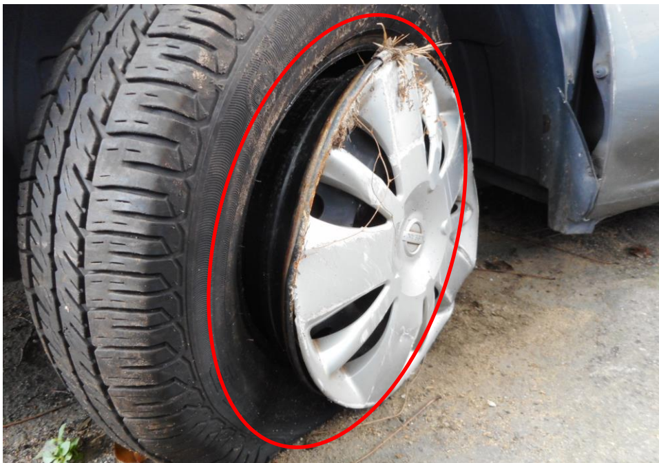
Photo 17 shows the close up view of the condition of the front left tyre of the Motor Van, which was observed to be unserviceable condition with remaining tread depth of approximately 3.9mm. The tyre was observed to slip out the wheel rim and there was damage observed on the wheel rims (circled) as a result of the accident.
