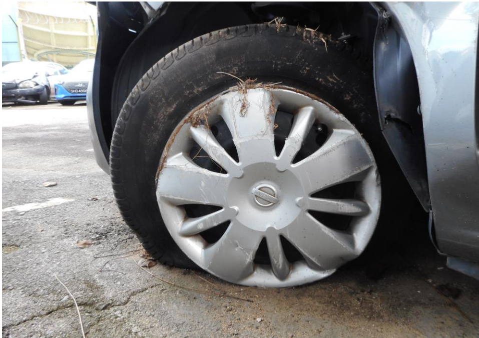
Photo 16 shows the condition of the front left tyre of the Motor Van, which was observed to be unserviceable condition with remaining tread depth of approximately 3.9mm. The tyre was observed to slip out the wheel rim and there was damage observed on the wheel rims as a result of the accident.
