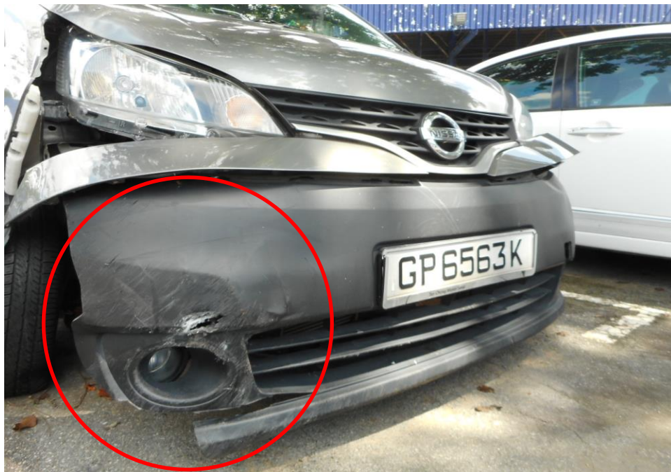
Photo 3 shows the close up view of the Motor Van's front body at the time of my inspection. The Motor Van was observed to have sustained damage at its front portion. Its front bumper (circled) were amongst the body parts that were damaged as a result of the accident.
