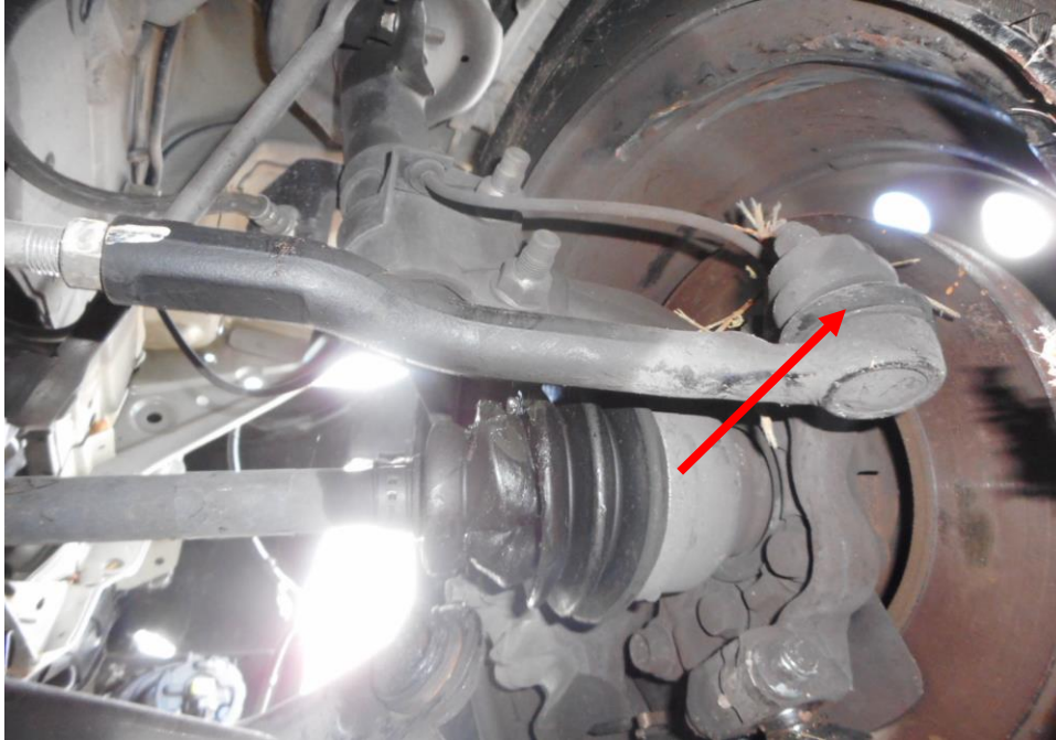
Photo 28 shows the various undercarriage components at the front right wheel of the Motor Van, in particular the steering tie rod (red arrow). The various steering components were all found to be intact, suggesting that the steering system of the Motor Van was likely to be in serviceable condition at the material time of accident. There was also no sign of fluid stain observed on the various undercarriage components at the front right wheel of the Motor Van.
