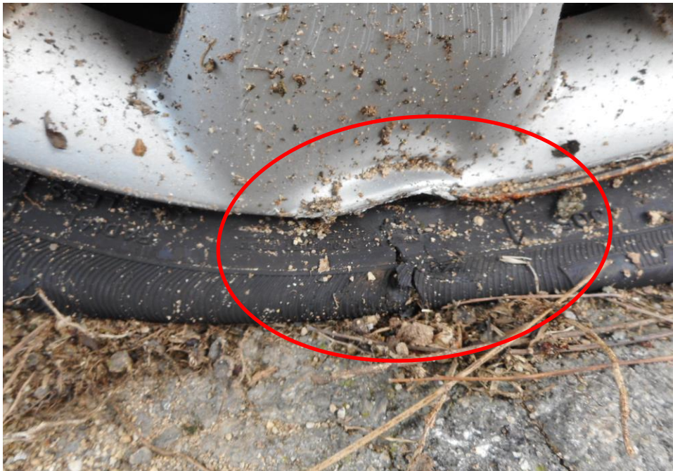
Photo 15 shows the close up view of the condition of the rear left tyre of the Motor Van, which was observed to be unserviceable condition with remaining tread depth of approximately 5.7mm. The tyre was observed with cut mark(s) on the outer sidewalls and there was damage observed on the wheel rims (circled) as a result of the accident.
