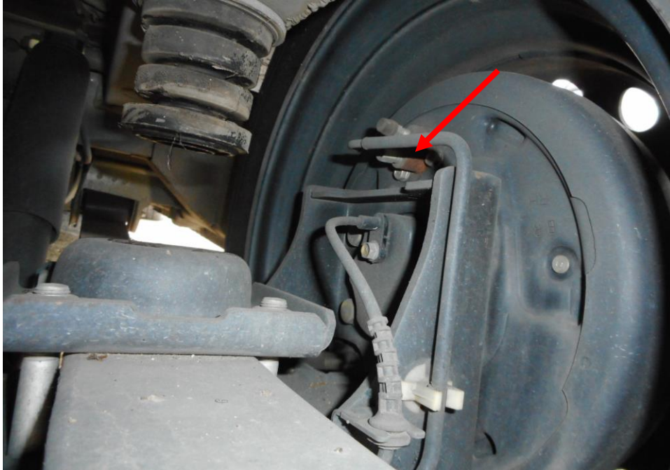
Photo 24 shows the brake hose/pipe (arrowed) at the rear right wheel of the Motor Van. No leakage of brake fluid was observed. Visual examination of the various components of the braking system like the drum brake, brake booster, brake pedal etc. had revealed all to be intact and without visible damage.
