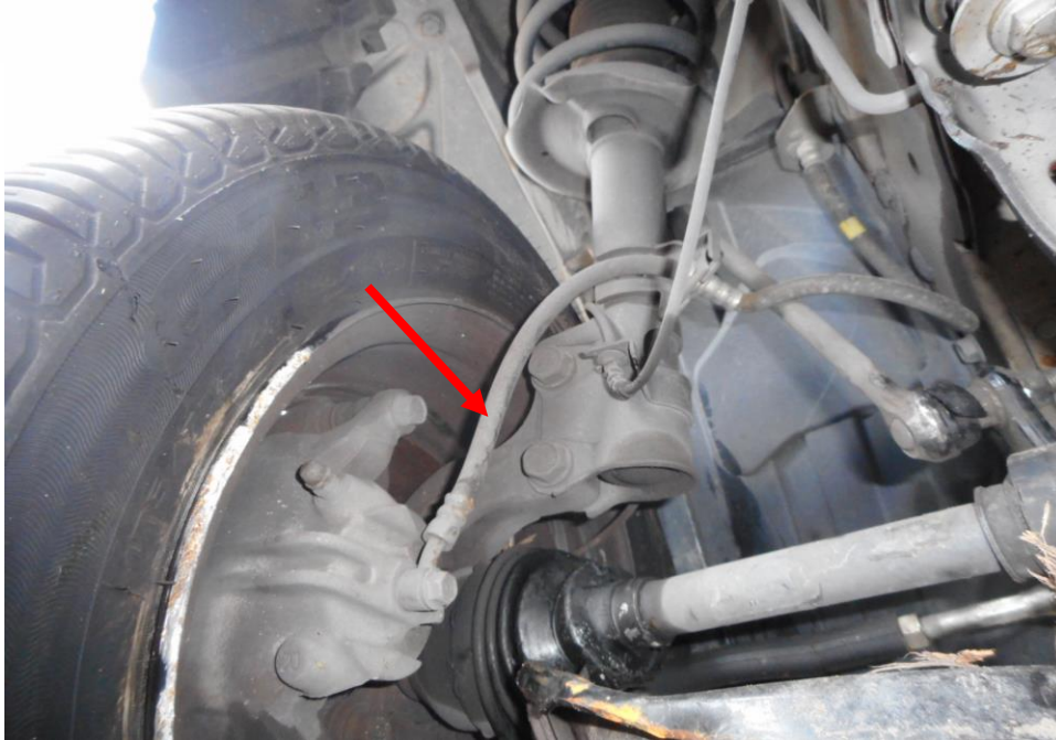
Photo 26 shows the brake hose/pipe (arrowed) at the front right wheel of the Motor Van. I did not observe any leakage of brake fluid at the time of my inspection of the Motor Van. Static tests of the Motor Van's braking system had indicated that there was no internal leakage of pressure/vacuum. The undercarriage components of the Motor Van were also all found to be intact and without any visible damage.
