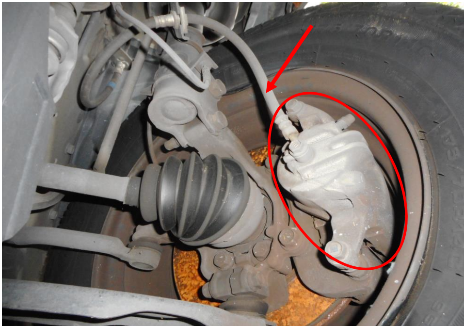
Photo 27 shows the brake hose/pipe (arrowed) at the front left wheel of the Motor Van. No leakage of brake fluid was observed. Visual examination of the various components of the braking system like the brake caliper (circled), brake booster, brake pedal etc had revealed all to be intact and without visible damage.
