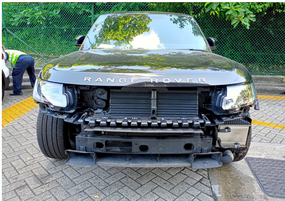
Photo 1 shows the frontal body of the Motor Car (photograph provided to me). The Motor Car's front bumper and all its related parts and attachments were observed to be damaged/dislodged/missing.
