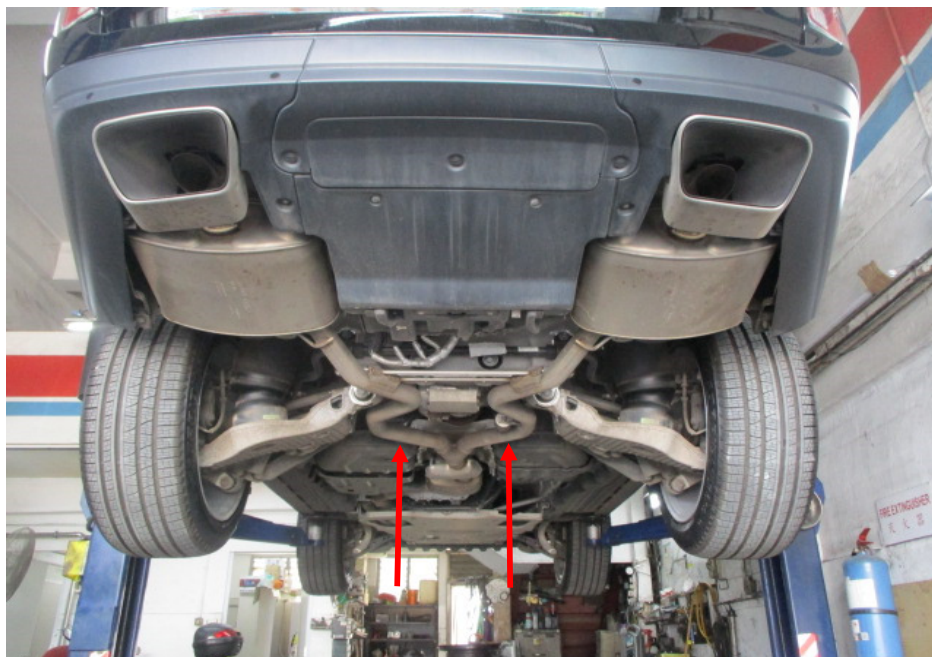
Photo 20 shows a general view of the rear section of the Motor Car's exhaust system. My examination of the Motor Car's exhaust system revealed no sign(s) or indication(s) of any cut or weld marks along its exhaust pipes (arrowed), on its catalytic converter, centre resonator boxes and on its rear mufflers.
