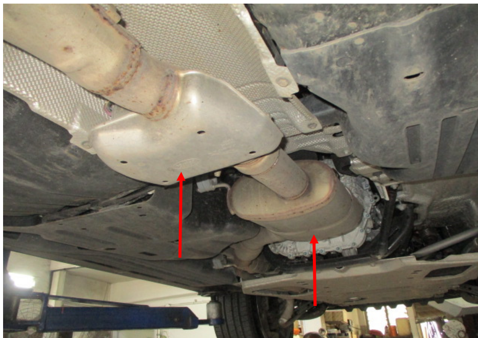
Photo 21 shows the front section of the Motor Car's exhaust system. My examination of the Motor Car's exhaust system revealed no sign(s) or indication(s) of any cut or weld marks along its exhaust pipes, on its catalytic converters, centre resonator boxes (arrowed) and on its rear mufflers.
