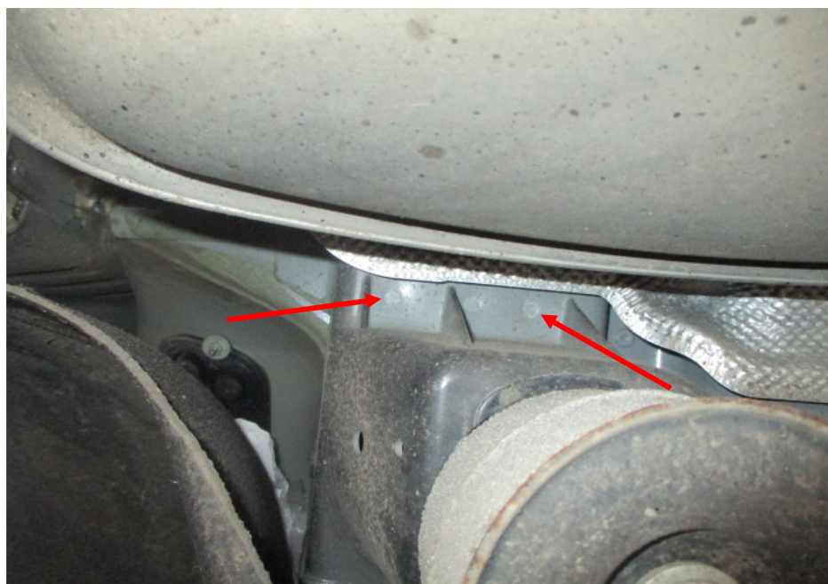
Photo 23 shows the chassis/structural body at the underside rear left of the Motor Car. I did not find any weld marks other than original spot weld marks (arrowed) on the chassis/structural body of the Motor Car. In general, I had found no work was carried out on the chassis/structural body of the Motor Car. The chassis/structural body of the Motor Car was originally fitted.
