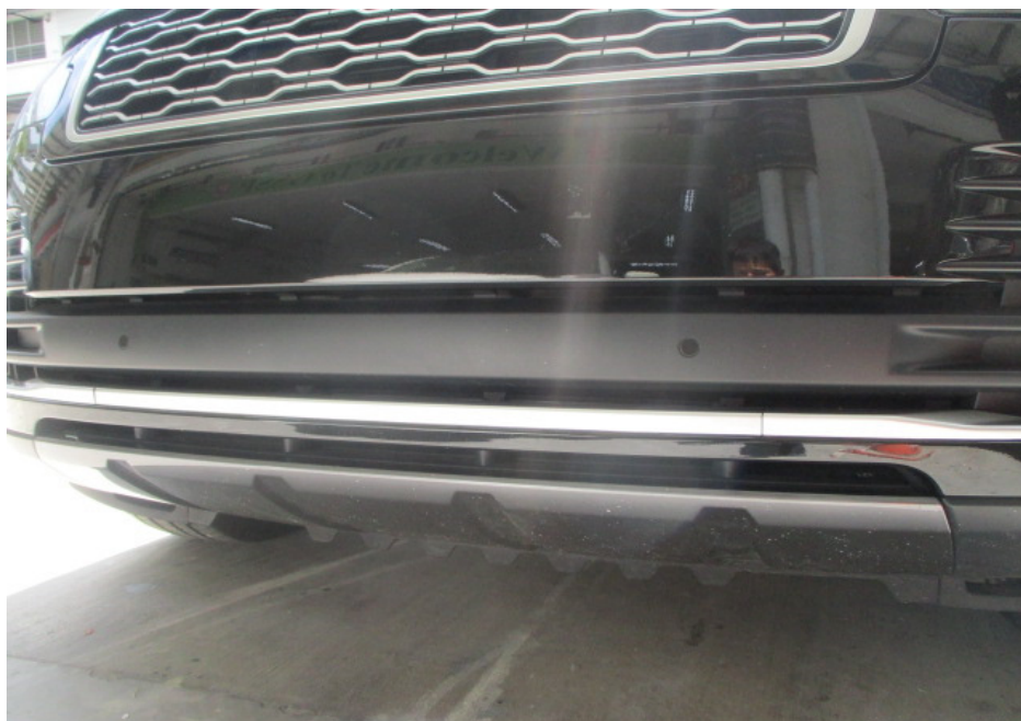
Photo 7 shows a closer view of the Motor Car's front bumper and front bumper lower garnishes at the time of my inspection. The frontal body of the Motor Car was visually examined, and it was observed that the repair/restoration works carried out to the damaged area of the Motor Car (refer to photograph 1 above) were reasonably adequate and in order.
