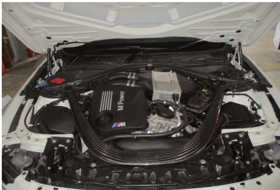
Photo 12 shows a general view of the engine compartment of the Motor Car at the time of my inspection. The various parts and components inside the engine compartment were all observed to be intact and properly fitted. There was also no sign(s) or indication(s) of fluid leak and/or fluid stain found inside the engine compartment. The repair/restoration works carried out to the various parts within the engine compartment like the front top panel garnish, front support panel and aircon condenser amongst others, were reasonably adequate and in order.
