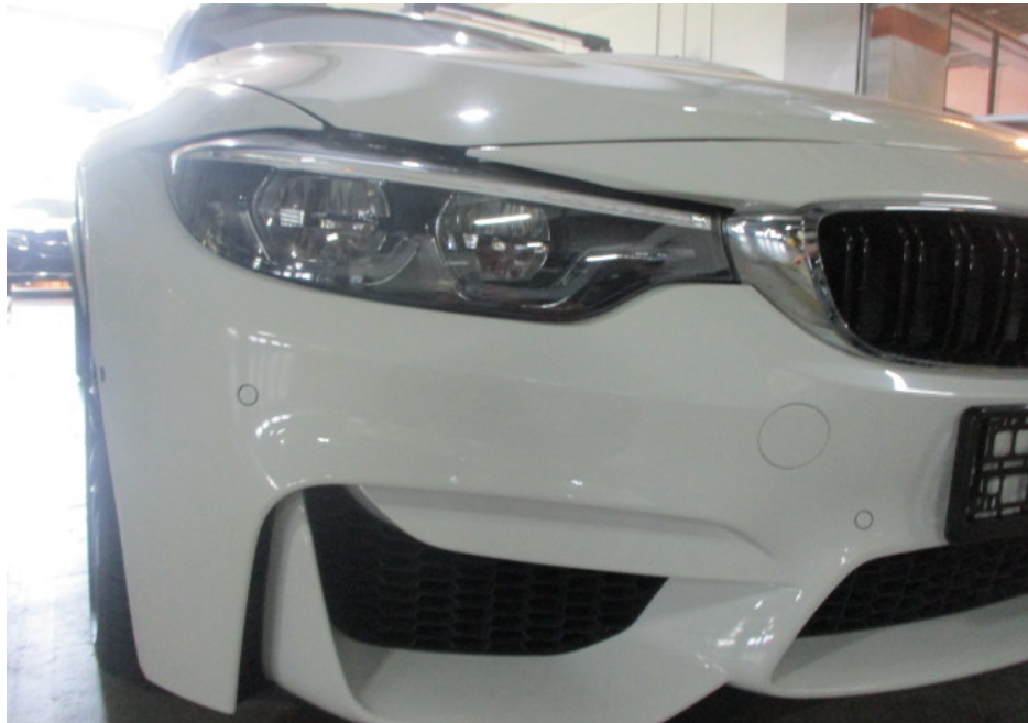
Photo 8 shows a closer view of the Motor Car's front bumper, front bumper right lower grille and front right headlamp. The body parts at the frontal portion of the Motor Car were visually examined and it was observed that the repair/restoration works carried out to the damaged area of the Motor Car (refer to photograph 1 & 2 above) were reasonably adequate and in order.
