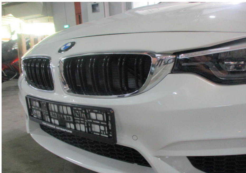
Photo 6 shows a closer view of the Motor Car's front bumper, front bumper centre lower grille, front radiator grilles and front left headlamp. The body parts at the frontal portion of the Motor Car were visually examined and it was observed that the repair/restoration works carried out to the damaged area of the Motor Car (refer to photograph 1 & 2 above) were reasonably adequate and in order.
