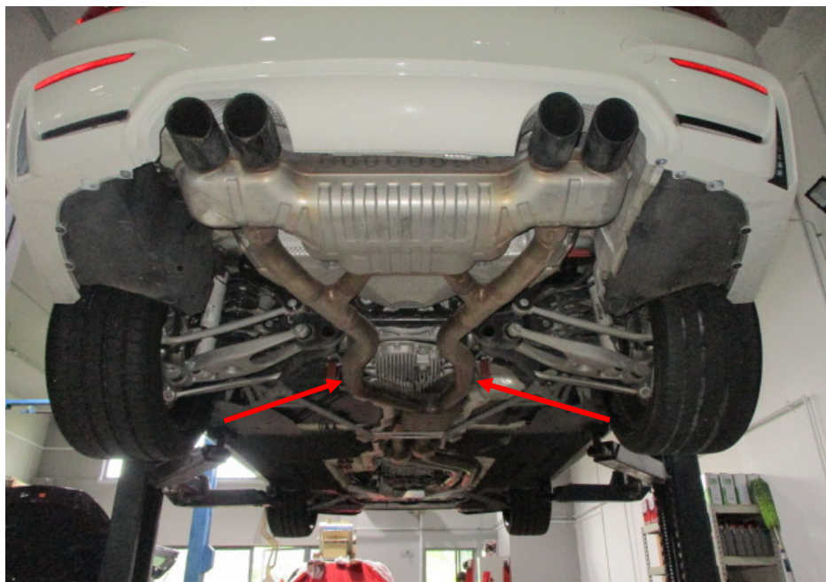
Photo 20 shows a general view of the rear section of the Motor Car's exhaust system. My examination of the Motor Car's exhaust system revealed no sign(s) or indication(s) of any cut or weld marks along its exhaust pipes (arrowed), on its catalytic converters and on its rear mufflers.
