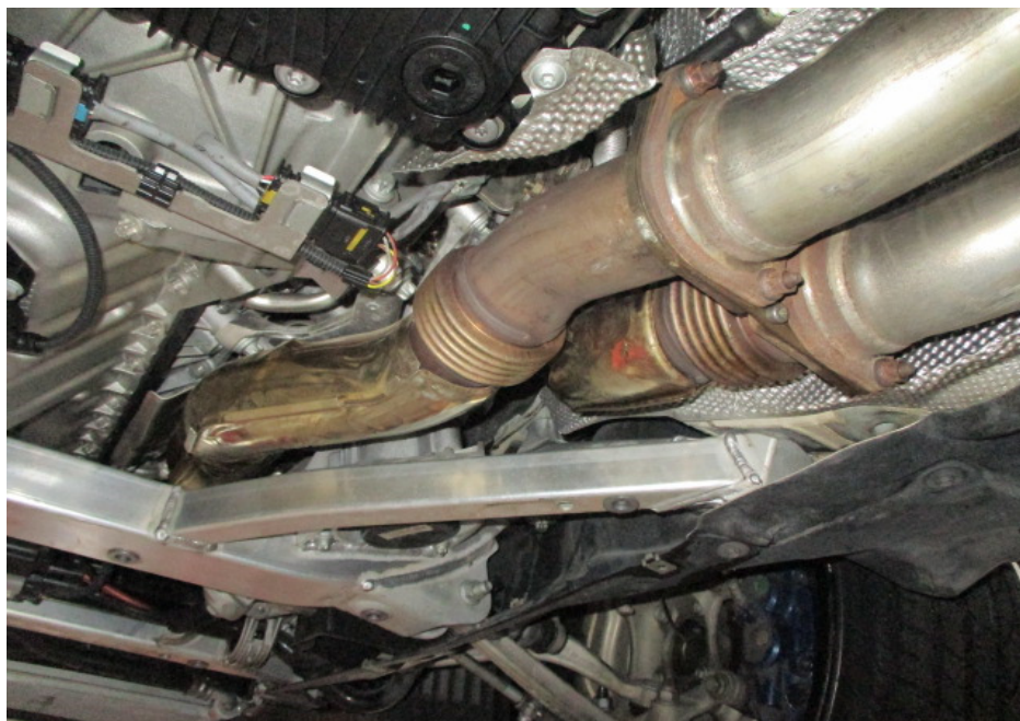
Photo 21 shows a general view of the Motor Car's catalytic converters. My examination of the Motor Car's exhaust system revealed no sign(s) or indication(s) of any cut or weld marks along its exhaust pipes, on its catalytic converters and on its rear mufflers.
