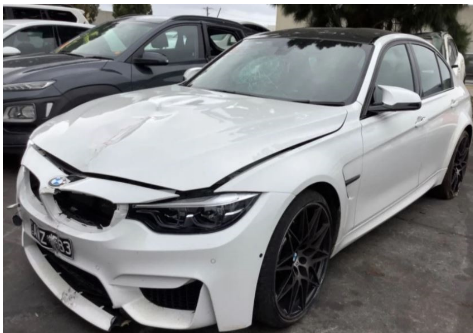
Photo 2 shows the front left body of the Motor Car prior to any repairs being carried out (photograph provided to me). The Motor Car was observed to have sustained damages at its frontal portion. Body parts observed to be damaged include the front bumper, front bumper centre lower grille, front radiator grilles, front left headlamp and front bonnet amongst others.
