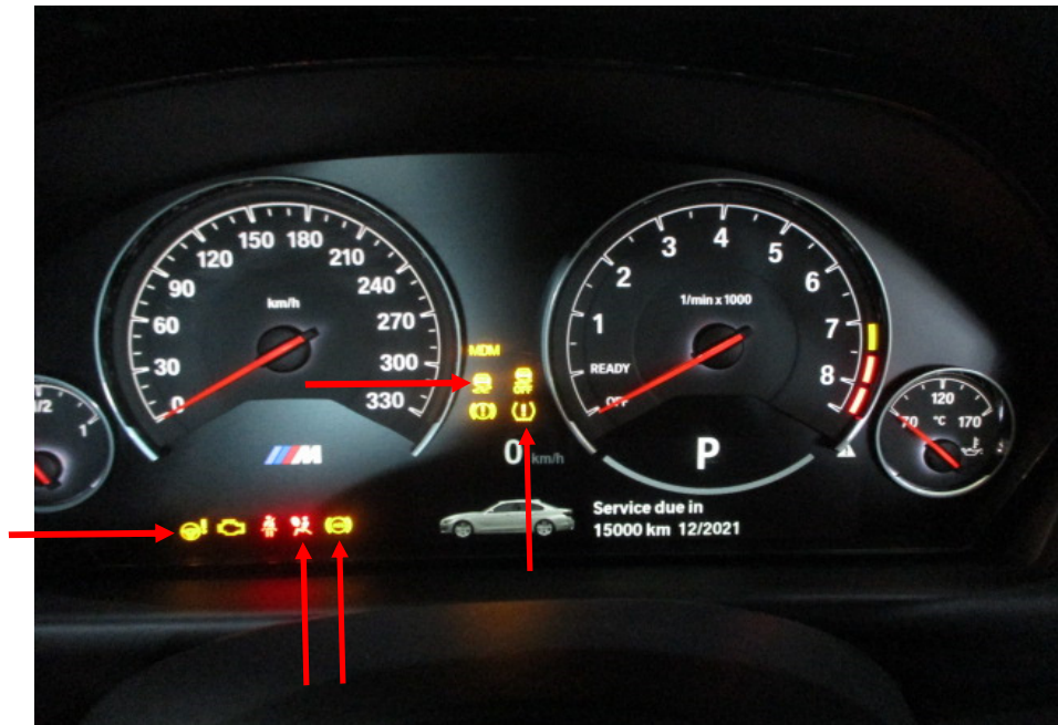
Photo 14 shows the warning lights for the various electronic safety features appearing on the instrument panel of the Motor Car during its self-test when the engine is cranked, in particular the ABS, SRS, IAS, TPM and DSC lights (arrowed).
