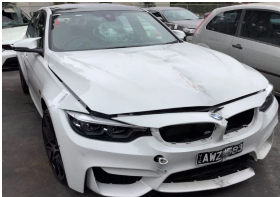
Photo 1 shows the front right body of the Motor Car prior to any repairs being carried out (photograph provided to me). The Motor Car was observed to have sustained damages at its frontal portion. Body parts observed to be damaged include the front bumper, front bumper centre lower grille, front radiator grilles, front right headlamp and front bonnet amongst others.
