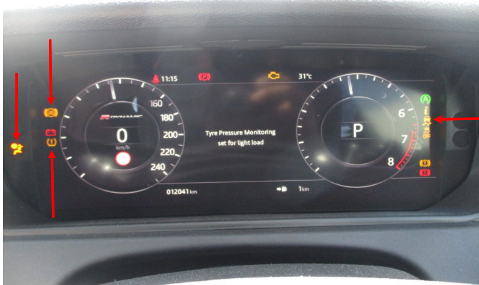
Photo 19 shows the warning lights for the various electronic safety features appearing on the instrument panel of the Motor Car during its self-test when the engine is cranked, in particular the ABS, SRS, TPM and TCS lights (arrowed).
