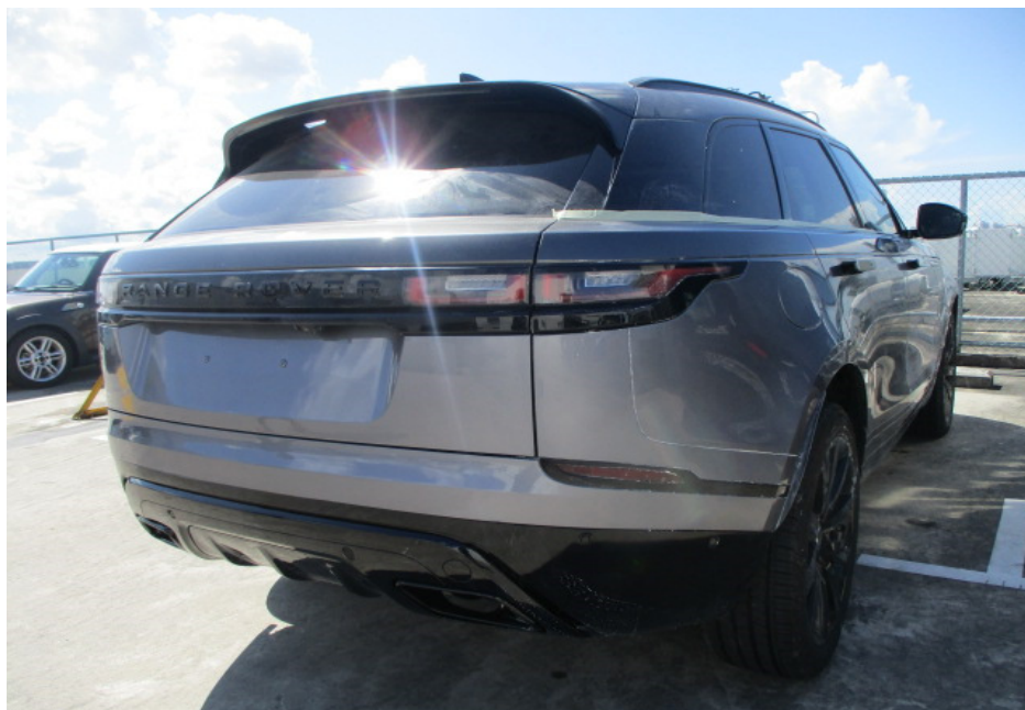
Photo 12 shows a general view of the rear right body of the Motor Car at the time of my inspection. The Motor Car was observed to be in a relatively good general condition with no loose exterior fittings observed. The body parts at the rear portion of the Motor Car were visually examined and it was observed that the repair/restoration works carried out to the damaged area of the Motor Car (refer to photograph 1 - 5 above) were reasonably adequate and in order.
