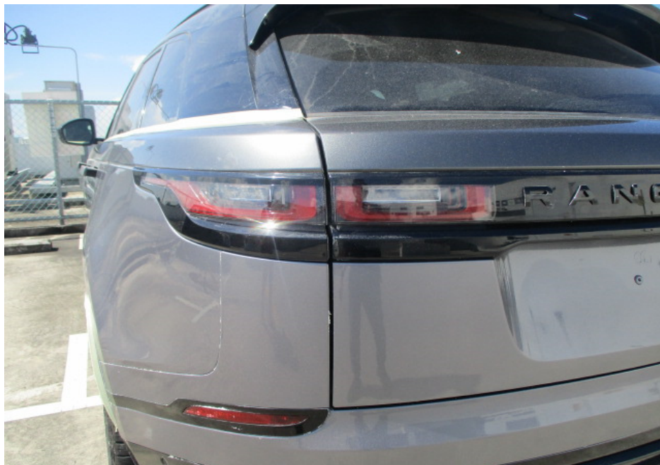
Photo 11 shows a closer view of the Motor Car's rear left taillamp. The body parts at the rear portion of the Motor Car were visually examined and it was observed that the repair/restoration works carried out to the damaged area of the Motor Car (refer to photograph 5 above) were reasonably adequate and in order.
