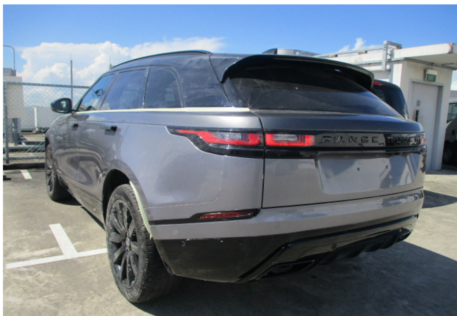
Photo 9 shows a general view of the rear left body of the Motor Car at the time of my inspection. The Motor Car was observed to be in a relatively good general condition with no loose exterior fittings observed. The body parts at the rear portion of the Motor Car were visually examined and it was observed that the repair/restoration works carried out to the damaged area of the Motor Car (refer to photograph 1 - 5 above) were reasonably adequate and in order.
