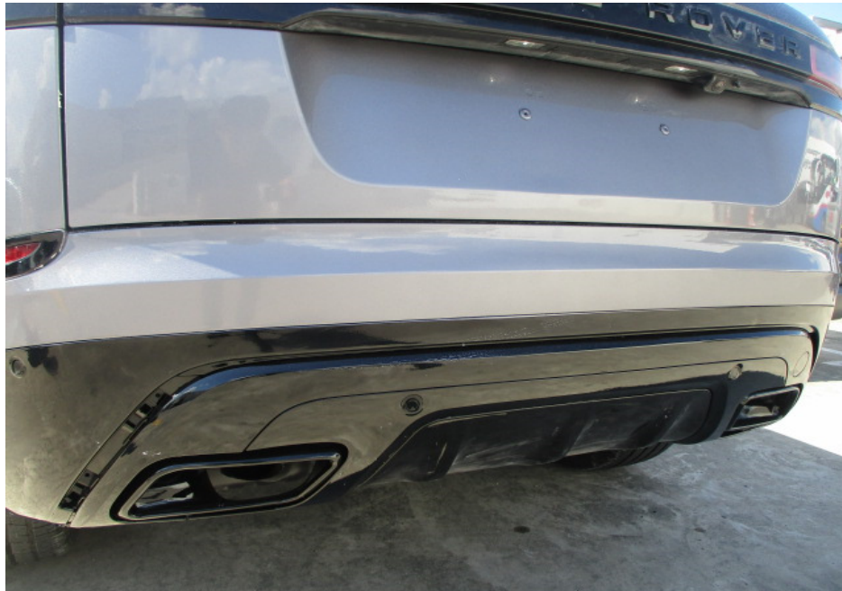
Photo 10 shows a closer view of the Motor Car's rear bumper, rear bumper lower cover, reverse sensors, rear left exhaust garnish and rear tailgate. The body parts at the rear portion of the Motor Car were visually examined and it was observed that the repair/restoration works carried out to the damaged area of the Motor Car (refer to photograph 1 - 4 above) were reasonably adequate and in order.
