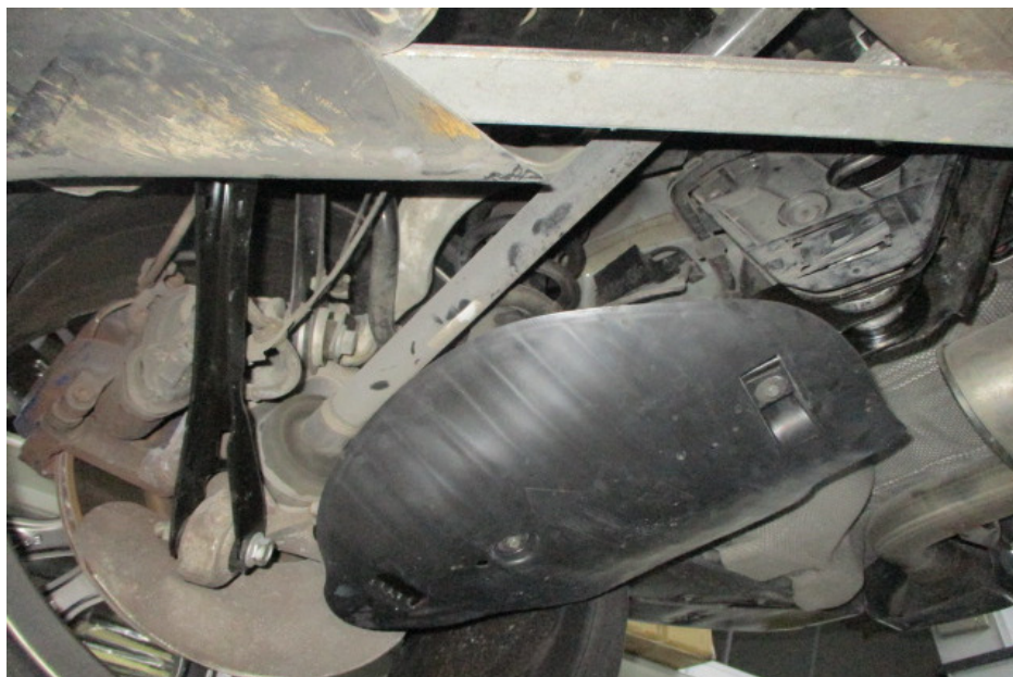
Photo 24 shows the various undercarriage components at the rear right wheel of the Motor Car. The mechanical components, control arms and linkages were all found to be intact and secured in an appropriate manner. I also did not observe any fluid leak and/or fluid stain on the underside of the Motor Car.
