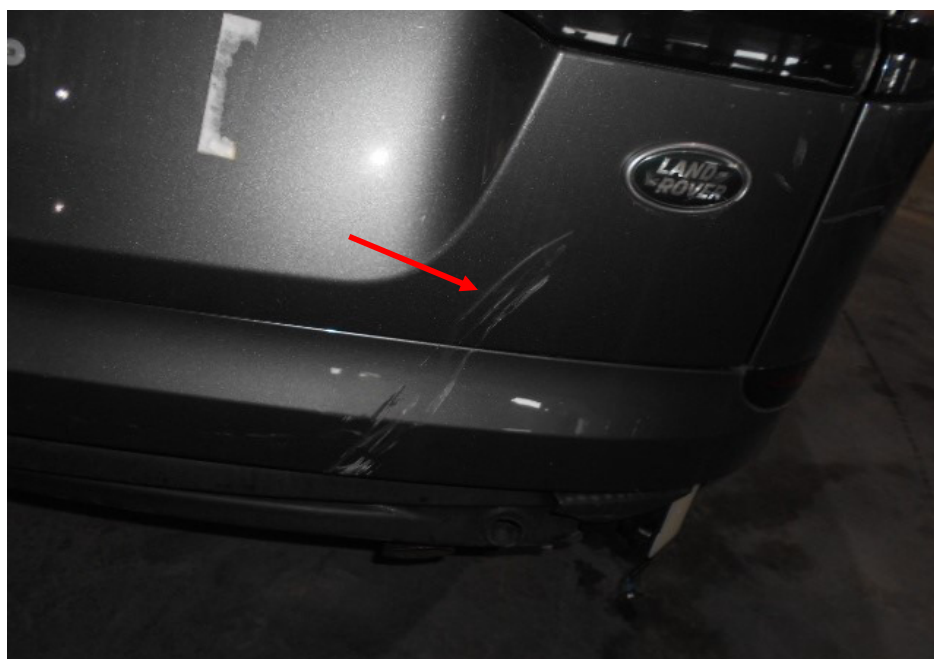
Photo 4 shows a closer view of the damage to the rear bumper and rear tailgate (arrowed) of the Motor Car (photograph provided to me).
