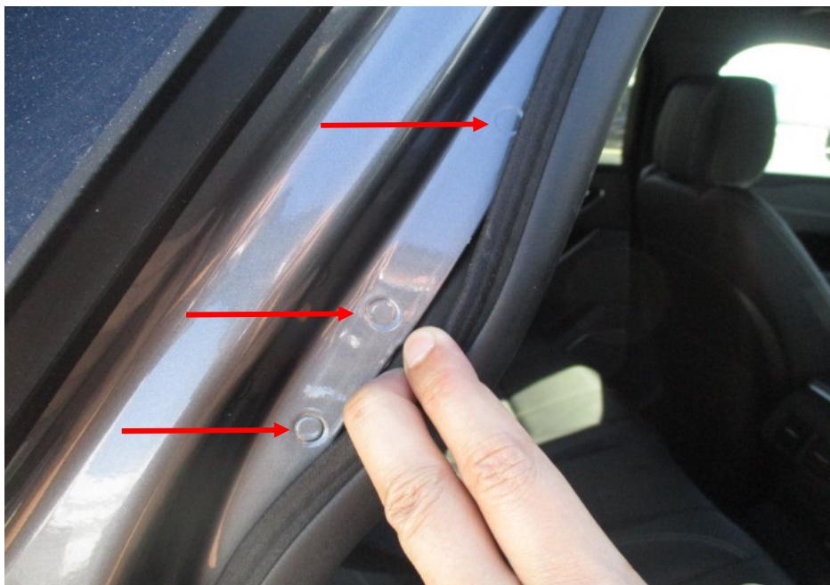
Photo 30 shows the right side "C" pillar of the Motor Car. I did not find any weld marks other than original spot weld marks (arrowed) on the right side "C" pillar of the Motor Car which, indicates that there was no re-welding works carried out. In general, I had found all the non-detachable body panels of the Motor Car to be originally fitted at the time of my inspection.
