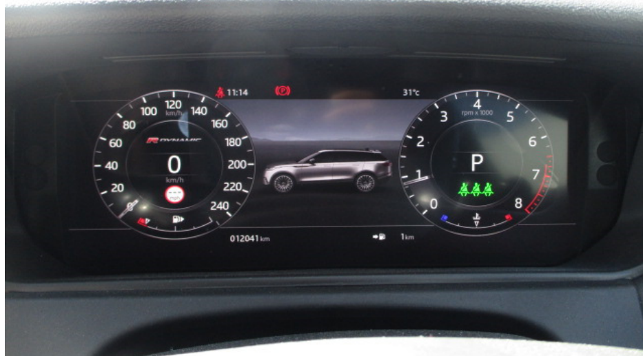
Photo 20 shows the respective warning lights no longer illuminated, indicating that there is no fault detected to the ABS, SRS, TPM and TCS systems of the Motor Car during the self-test. These electronic systems were hence in working condition at the time of my inspection.
