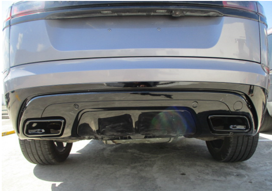
Photo 14 shows a closer view of the Motor Car's rear bumper, rear bumper lower cover, reverse sensors, rear exhaust garnishes and rear tailgate. The body parts at the rear portion of the Motor Car were visually examined and it was observed that the repair/restoration works carried out to the damaged area of the Motor Car (refer to photograph 1 - 4 above) were reasonably adequate and in order.
