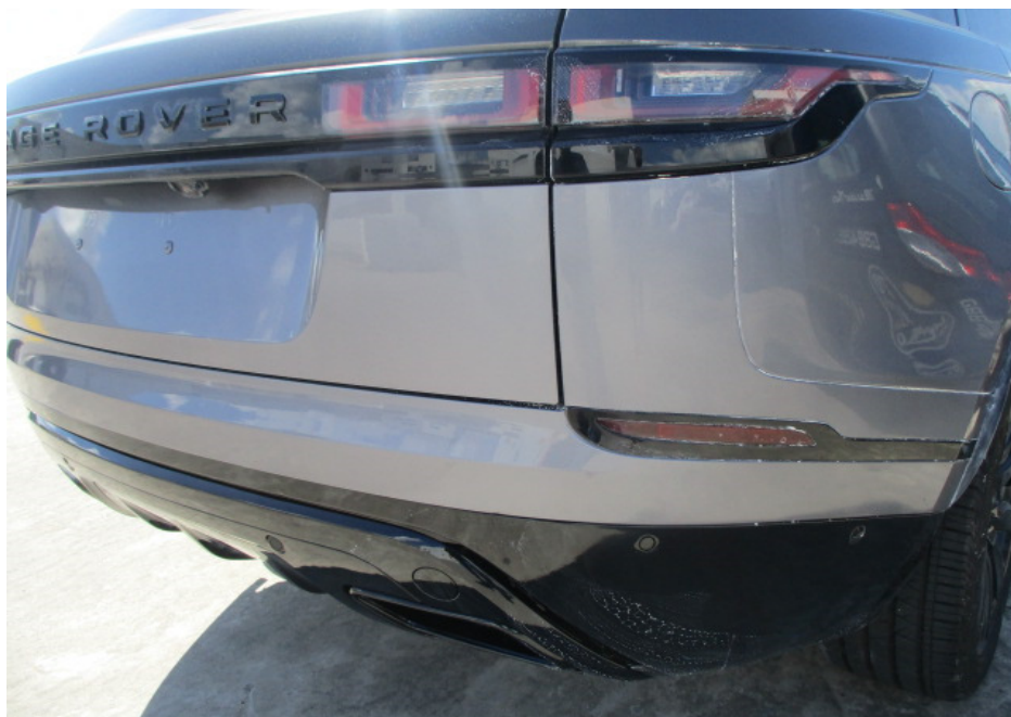
Photo 13 shows a closer view of the Motor Car's rear bumper, rear bumper lower cover, rear right exhaust garnish and rear tailgate. The body parts at the rear portion of the Motor Car were visually examined and it was observed that the repair/restoration works carried out to the damaged area of the Motor Car (refer to photograph 1 - 4 above) were reasonably adequate and in order.
