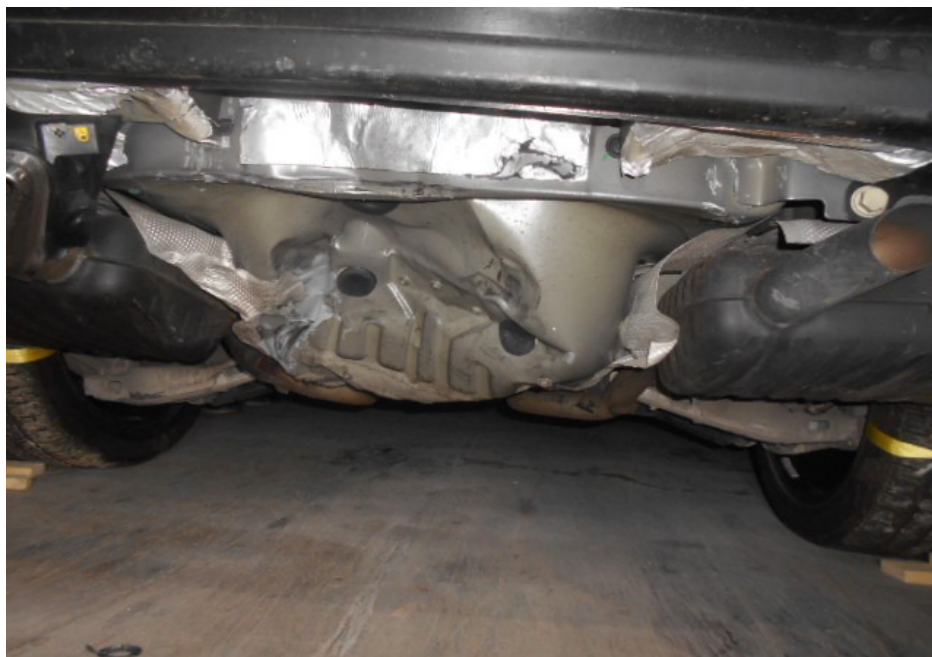
Photo 3 shows a closer view of the damage to the rear end panel, spare tyre panel and rear exhaust heat shields of the Motor Car (photograph provided to me).
