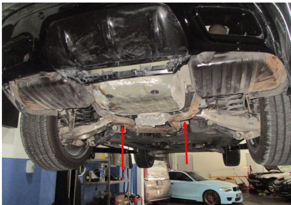
Photo 25 shows the rear section of the Motor Car's exhaust system. My examination of the Motor Car's exhaust system revealed no sign(s) or indication(s) of any cut or weld marks along its exhaust pipes (arrowed), on its centre resonator box, catalytic converter and on its rear mufflers.
