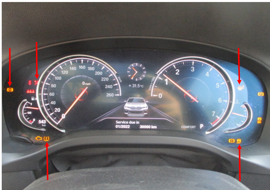
Photo 14 shows the warning lights for the various electronic safety features appearing on the instrument panel of the Motor Car during its self-test when the engine is cranked, in particular the ABS, SRS, IAS, TPM and DSC lights (arrowed).
