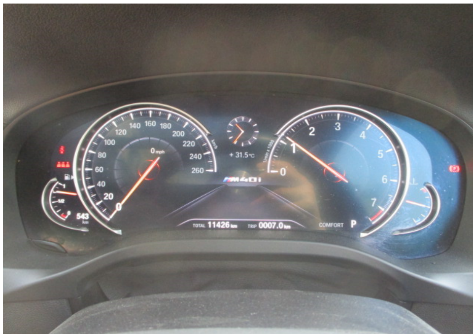
Photo 15 shows the respective warning lights no longer illuminated, indicating that there is no fault detected to the ABS, SRS, IAS, TPM and DSC systems of the Motor Car during the self-test. These electronic systems were hence in working condition at the time of my inspection.
