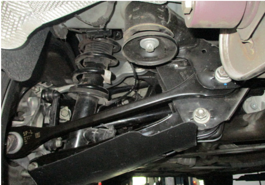
Photo 18 shows the various undercarriage components at the rear left wheel of the Motor Car. The mechanical components, control arms and linkages were all found to be intact and secured in an appropriate manner. The undercarriage parts at the rear left wheel of the Motor Car were visually examined and it was observed that the repair/restoration works carried out were reasonably adequate and in order.
