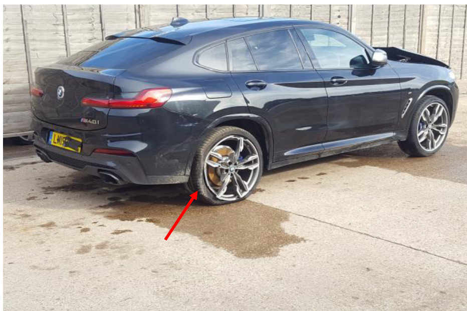
Photo 2 shows the rear right body of the Motor Car (photograph provided to me). The rear right wheel (arrowed) was oriented in an unnatural position, which would indicate likely damage to the various undercarriage parts at the rear right wheel of the Motor Car. Parts that may be damaged include the rear right shock absorber, rear right lower arm and rear right knuckle arm amongst others. The rear right tyre was observed to be punctured.
