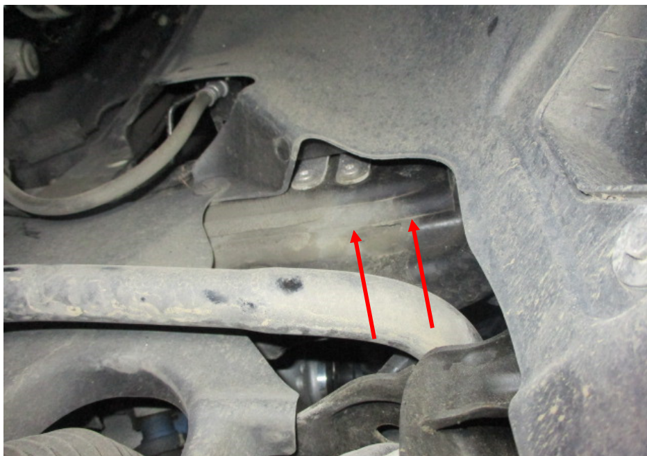
Photo 24 shows the chassis/structural body at the underside front right of the Motor Car. I did not find any weld marks other than original spot weld marks on the chassis/structural body of the Motor Car. The original factory sealant (arrowed) at the joints along the chassis/structural body was also untouched, indicating no work was done on the chassis/structural body of the Motor Car and that the chassis/structural body was originally fitted.
