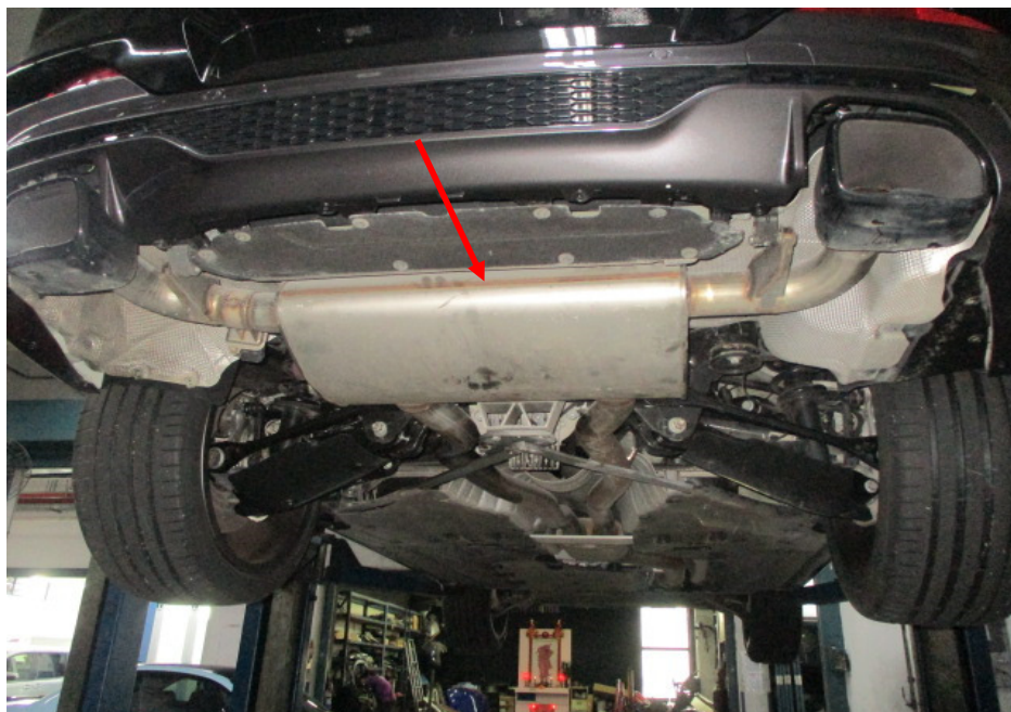
Photo 20 shows the rear section of the Motor Car's exhaust system. My examination of the Motor Car's exhaust system revealed no sign(s) or indication(s) of any cut or weld marks along its exhaust pipes and on its centre resonator box, catalytic converter and on its rear muffler (arrowed).
