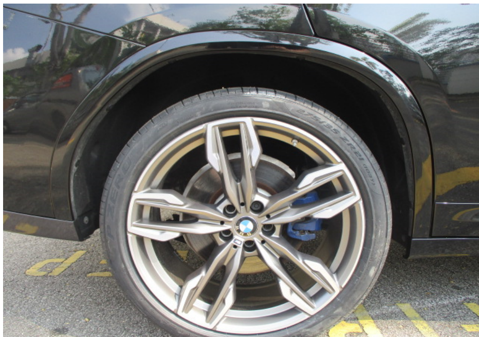
Photo 6 shows a closer view of the rear right wheel rim of the Motor Car. The body parts at the rear portion and undercarriage parts at the rear left wheel and rear right wheel of the Motor Car were visually examined and it was observed that the repair/restoration works carried out to the damaged area of the Motor Car (refer to photograph 1 & 2 above) were reasonably adequate and in order.
