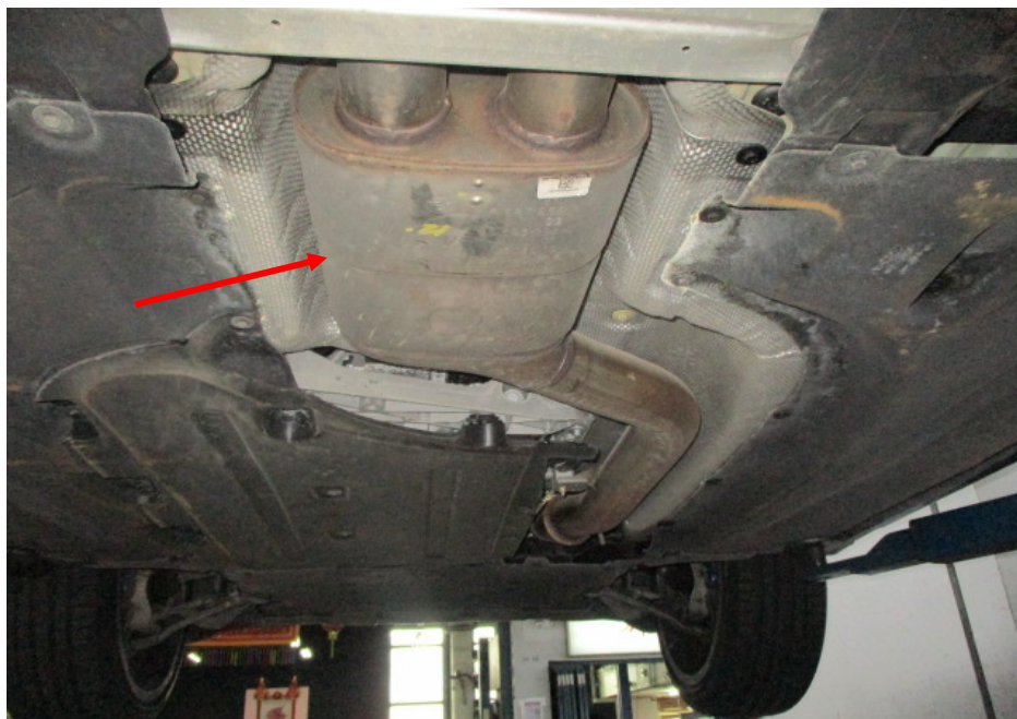
Photo 21 shows the front section of the Motor Car's exhaust system. My examination of the Motor Car's exhaust system revealed no sign(s) or indication(s) of any cut or weld marks along its exhaust pipes and on its centre resonator box (arrowed), catalytic converter and on its rear muffler.
