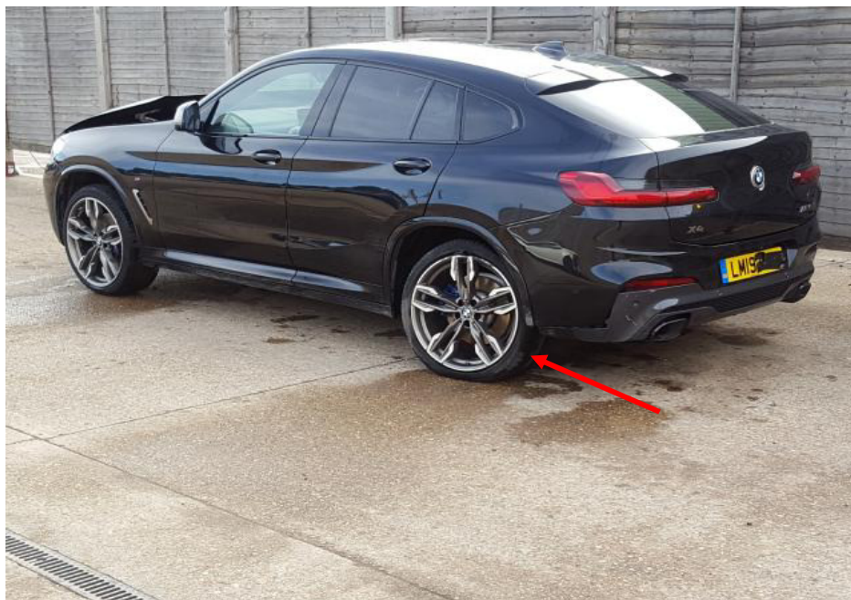
Photo 1 shows the rear left body of the Motor Car (photograph provided to me). The rear left wheel (arrowed) was oriented in an unnatural position, which would indicate likely damage to the various undercarriage parts at the rear left wheel of the Motor Car. Parts that may be damaged include the rear left shock absorber, rear left lower arm and rear left knuckle arm amongst others. The rear left tyre was observed to be punctured.
