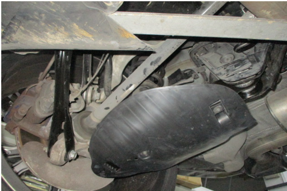
Photo 19 shows the various undercarriage components at the rear right wheel of the Motor Car. The mechanical components, control arms and linkages were all found to be intact and secured in an appropriate manner. The undercarriage parts at the rear right wheel of the Motor Car were visually examined and it was observed that the repair/restoration works carried out were reasonably adequate and in order.
