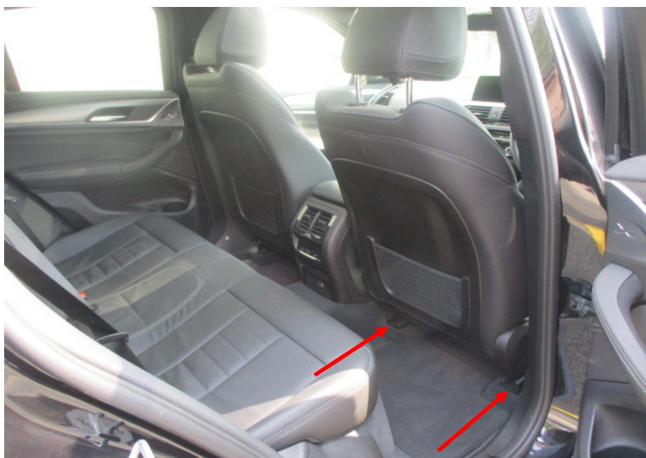
Photo 13 shows the seats of the Motor Car. All the seats of the Motor Car were secured via seat rails (arrowed) to the floorboard. They were also fitted with a retractable seat belt reels and pre-tensioners. The seat belts were tested and were able to be fastened into the respective pre-tensions that were fitted on the side of each individual seat.
