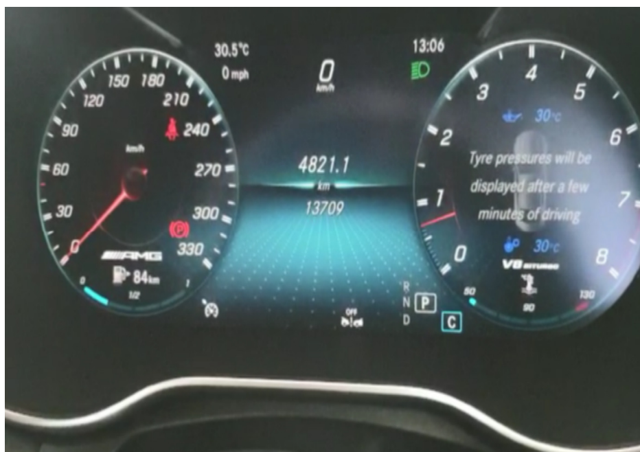
Photo 14 shows the respective warning lights no longer illuminated, indicating that there is no fault detected to the ABS, SRS, EPS, TPM and TCS systems of the Motor Car during the self-test. These electronic systems were hence in working condition at the time of my inspection.
