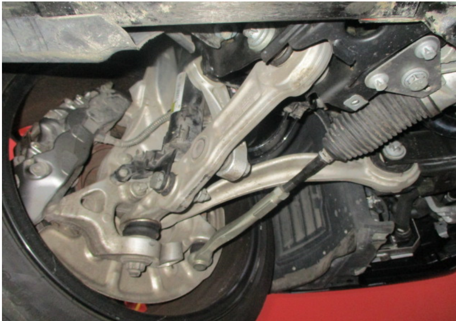
Photo 18 shows the various undercarriage components at the front left wheel of the Motor Car. The mechanical components, control arms and linkages were all found to be intact and secured in an appropriate manner. I also did not observe any fluid leak and/or fluid stain on the underside of the Motor Car.
