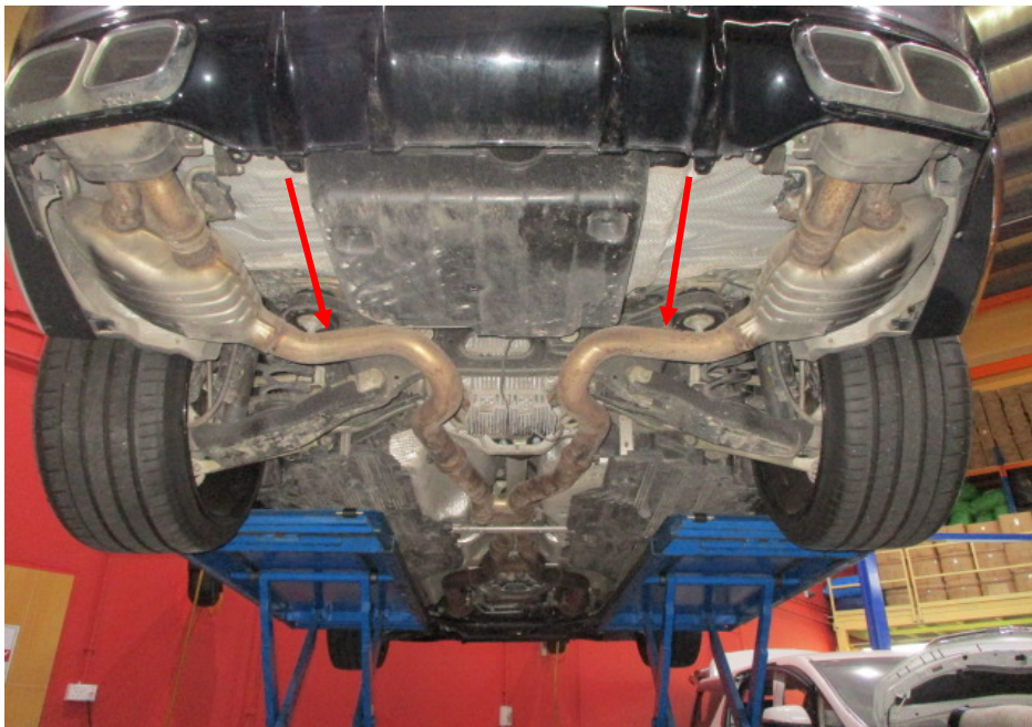
Photo 19 shows the Motor Car's exhaust system. My examination of the Motor Car's exhaust system revealed no sign(s) or indication(s) of any cut or weld marks along its exhaust pipes (arrowed), rear mufflers and on its catalytic converters.
