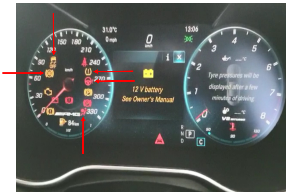
Photo 13 shows the warning lights for the various electronic safety features appearing on the instrument panel of the Motor Car during its self-test when the engine is cranked, in particular the ABS, SRS, EPS, TPM and TCS lights (arrowed).
