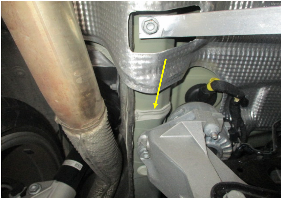
Photo 22 shows the chassis/structural body at the underside rear left of the Motor Car. I did not find any weld marks other than original spot weld marks on the chassis/structural body of the Motor Car. The original factory sealant (arrowed) at the joints along the chassis/structural body was untouched, indicating no work was done on the chassis/structural body of the Motor Car and that the chassis/structural body was originally fitted.
