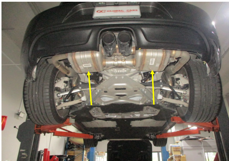
Photo 20 shows the Motor Car's rear mufflers (arrowed). My examination of the Motor Car's exhaust system revealed no sign(s) or indication(s) of any cut or weld marks along its exhaust pipes, on its catalytic converters and on its rear mufflers.
