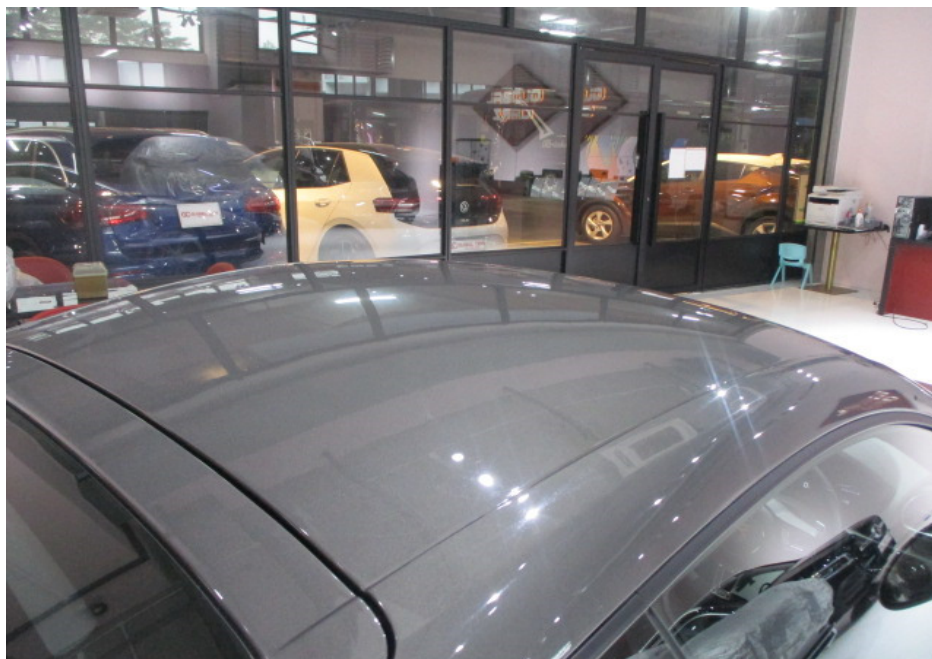
Photo 11 shows the roof panel of the Motor Car at the time of my inspection. In general, I had found that the repair/restoration works carried out to the damaged area of the Motor Car (refer to photograph 3 above) were reasonably adequate and in order.
