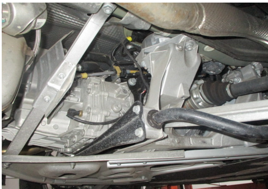
Photo 21 shows a general view of the engine compartment of the Motor Car at the time of my inspection. The engine compartment was at the rear underside of the Motor Car. The various parts and components inside the engine compartment were all observed to be intact and properly fitted. There was also no sign(s) or indication(s) of fluid leak and/or fluid stain found inside the engine compartment.
