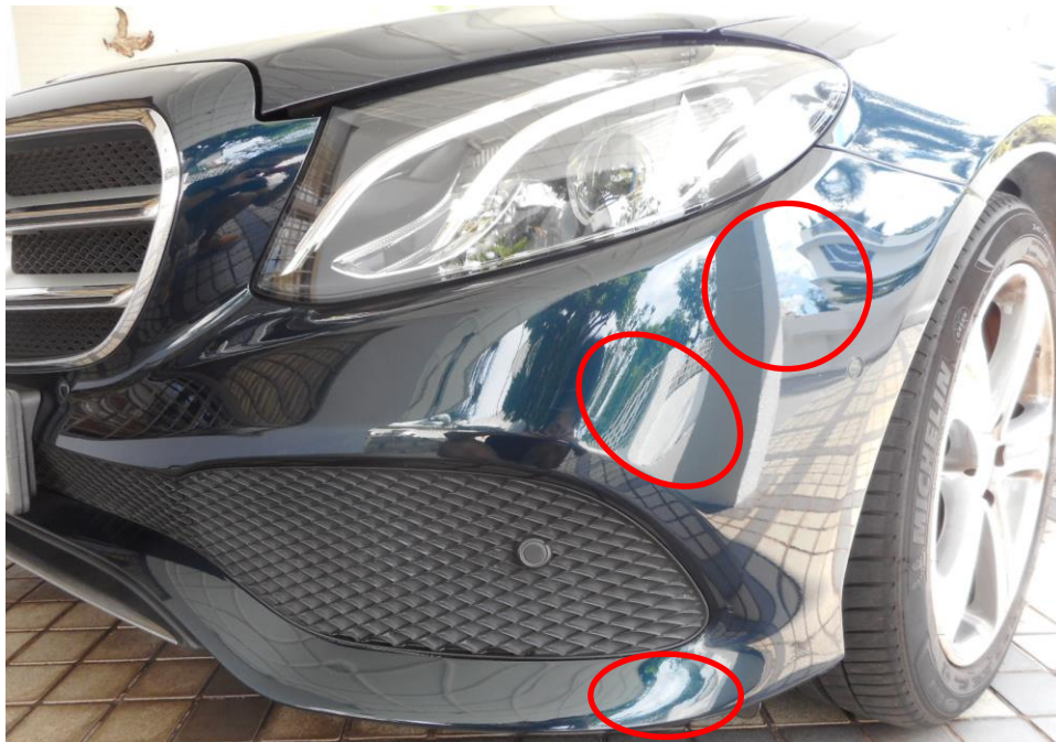
Photo 10 shows a general view of the Mercedes front portion. We observed multiple groups of scratch marks on the left corners of its front bumper (circled).
