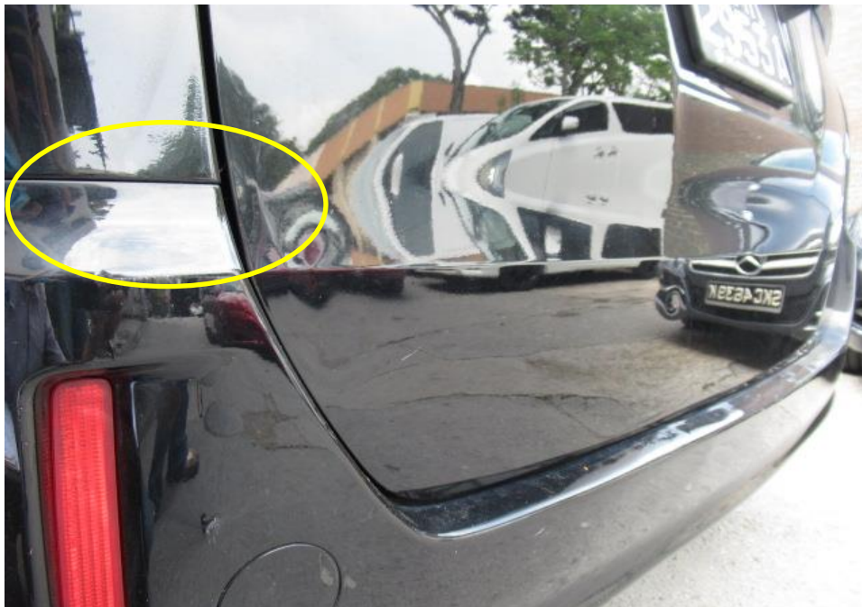
Photo 7 shows a close up view of the rear portion of the Toyota. We note that there was neither dislodgement nor misalignment of the rear bumper at the rear portion (circled) of Toyota.
