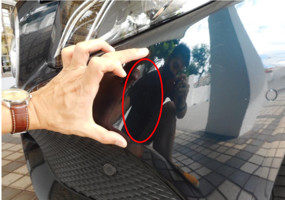
Photo 13 shows a close up view of the Mercedes front portion. We observed multiple groups of scratch marks on the left corners of its front bumper (circled).
