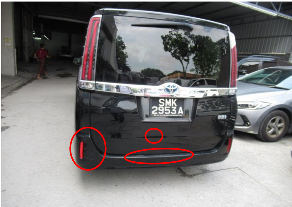
Photo 1 shows the general view of the rear portion of Toyota at the time of inspection. The rear bonnet and bumper had been damaged. It was also noted that there were paint crack marks and dents (circled) on the rear bumper of Toyota.
