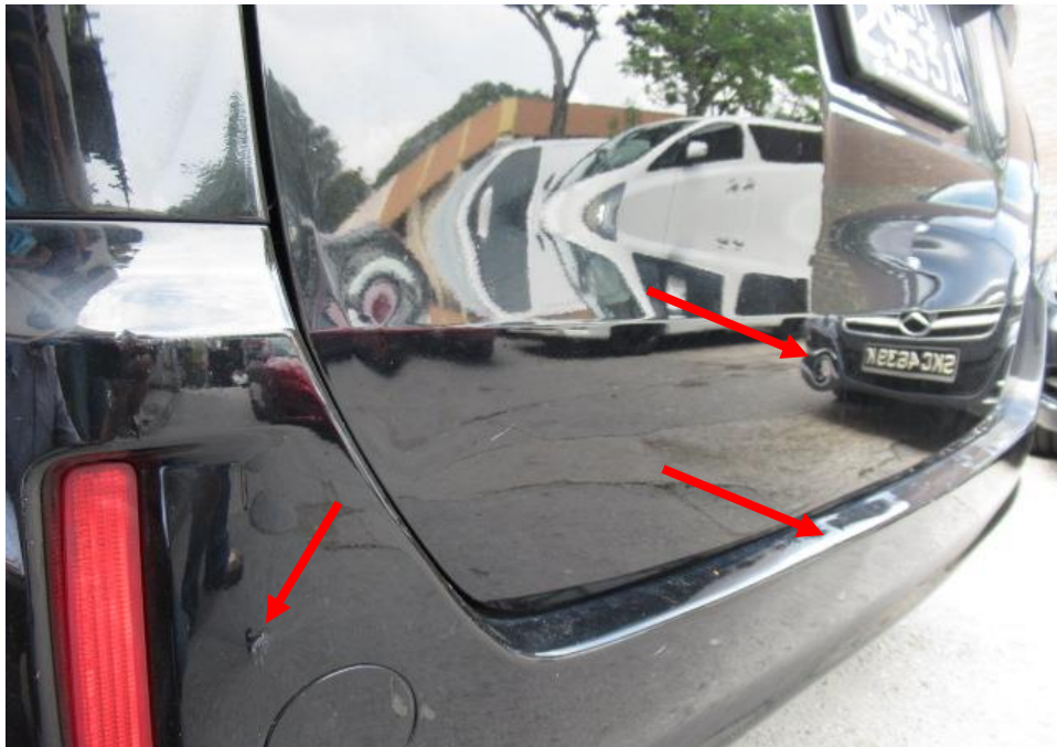
Photo 2 shows a close up view of the rear portion of the Toyota. We noted that there were dent marks on the rear bonnet and rear bumper (arrowed).
