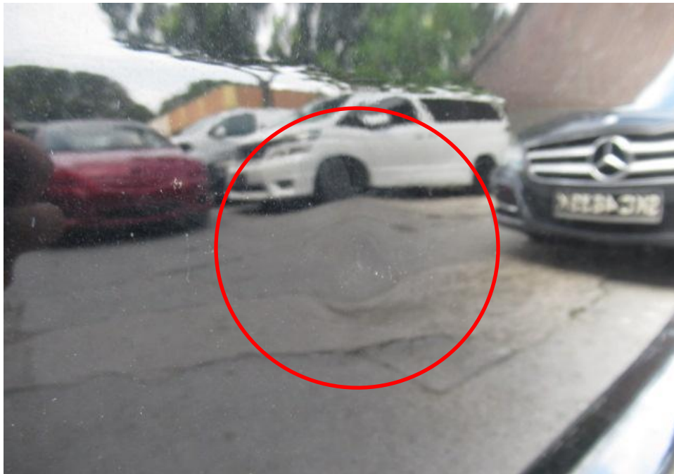
Photo 3 shows a close up view of the rear portion of the Toyota. We noted that there were dent marks on the rear bonnet (circled).
