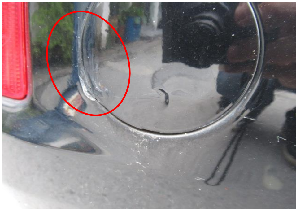
Photo 5 shows a close up view of the rear portion of the Toyota. We noted that there were paint dent and crack marks on the tow hook cap of the rear bumper (circled).
