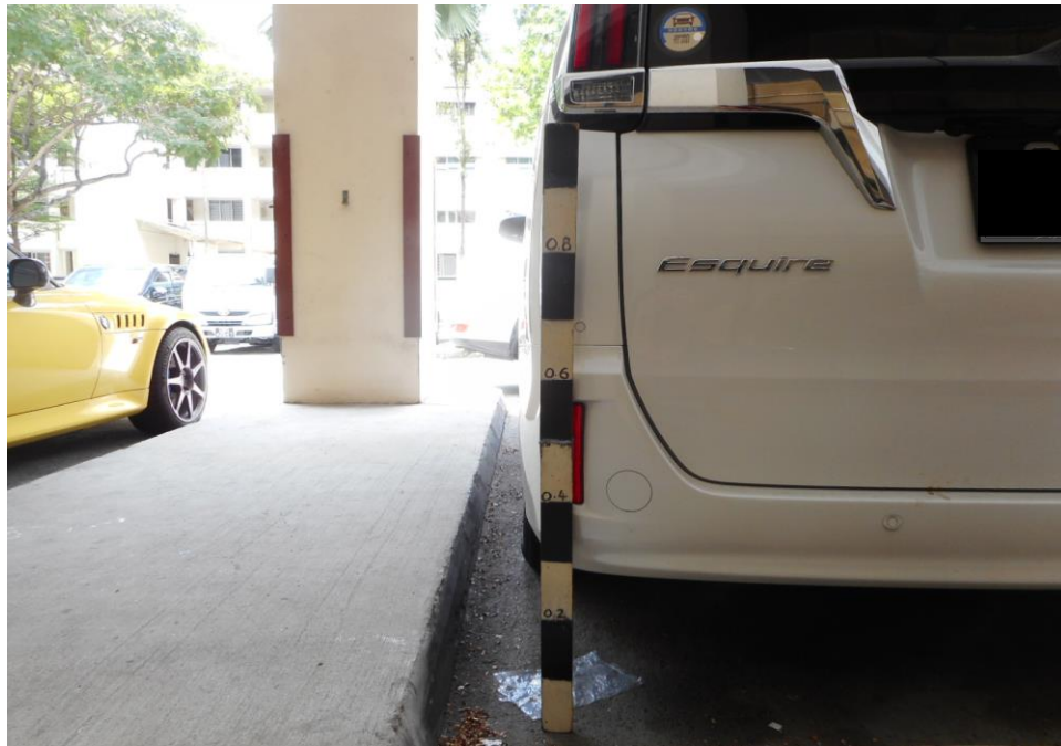
Photo 16 shows the general view of the height measurement being conducted on the rear portion of Toyota. The height above ground level of where the dent and crack marks were found to the rear bonnet and rear bumper of the Toyota was at 60cm; 47cm, 42cm and 40cm respectively.
