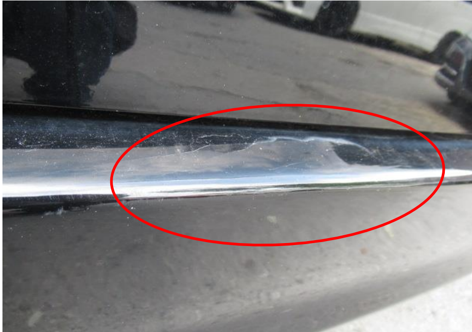
Photo 6 shows a close up view of the rear portion of the Toyota. We noted that there were paint crack marks on the rear bumper (circled).
