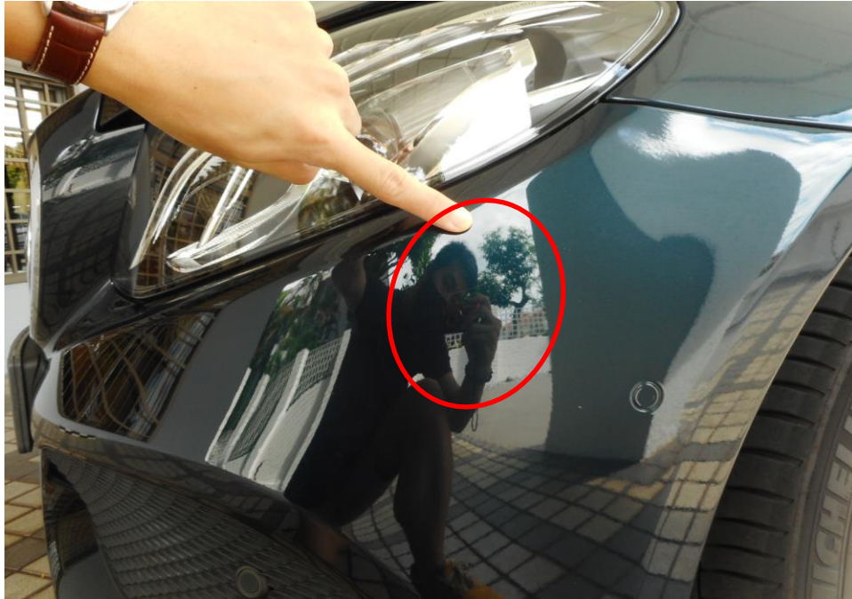
Photo 11 shows a close up view of the Mercedes front portion. We observed multiple groups of scratch marks on the left corners of its front bumper (circled).
