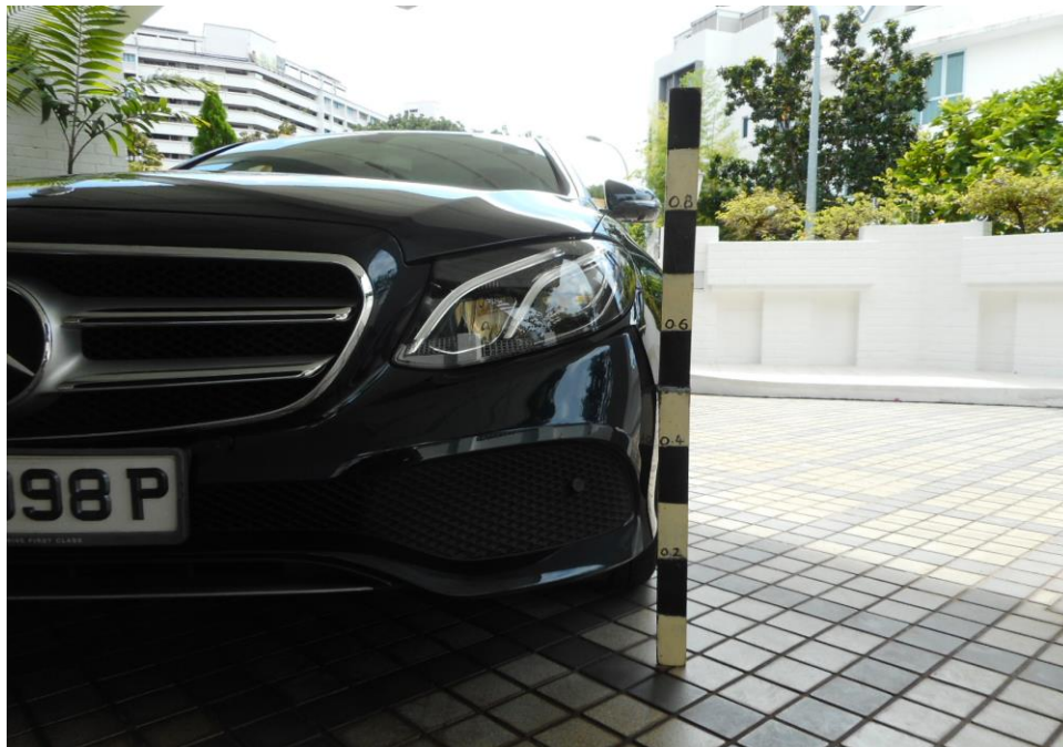
Photo 17 shows a general view of the height measurement being conducted on the front portion of Mercedes. The scratch marks found on the front bumper left corner was measured to be at 58cm to 60cm, 41cm to 56cm and 23cm to 28cm above ground level.
