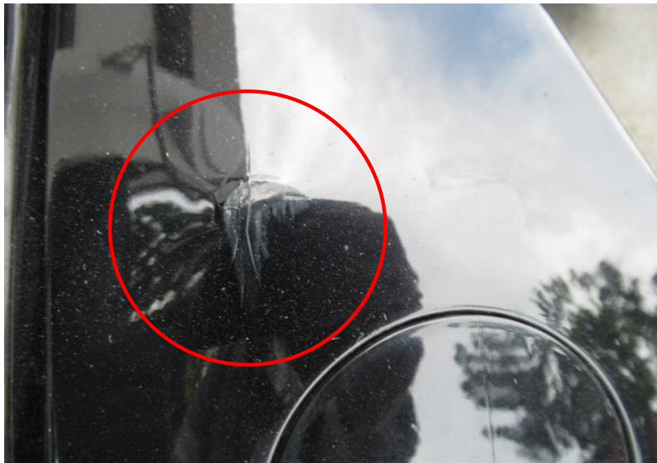
Photo 4 shows a close up view of the rear portion of the Toyota. We noted that there were dent and paint crack marks on the rear bumper (circled).
