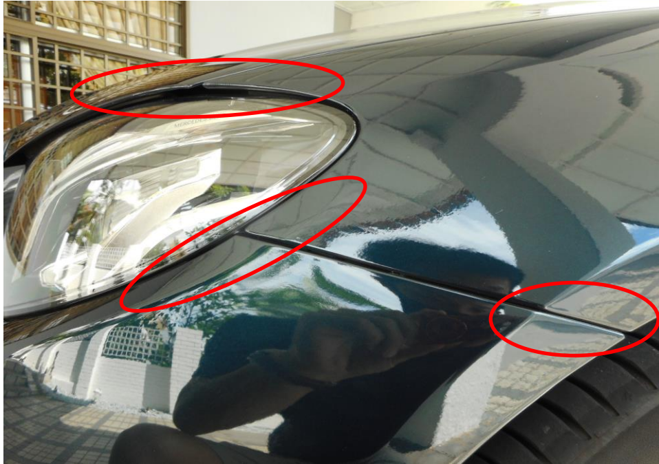
Photo 15 shows a close up view of the front portion of the Mercedes. We note that there was neither dislodgement nor misalignment of the front bumper at the front portion (circled) of Mercedes.
