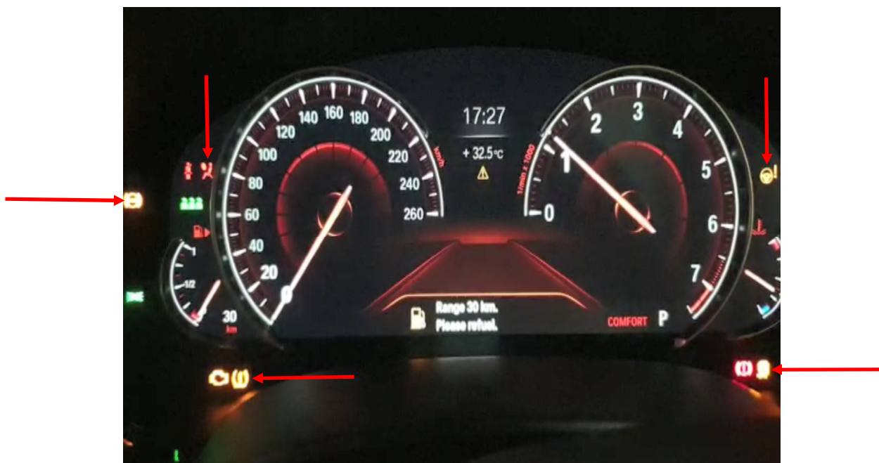
Photo 15 shows the warning lights for the various electronic safety features appearing on the instrument panel of the Motor Car during its self-test when the engine is cranked, in particular the ABS, SRS, IAS, TPM and DSC lights (arrowed).
