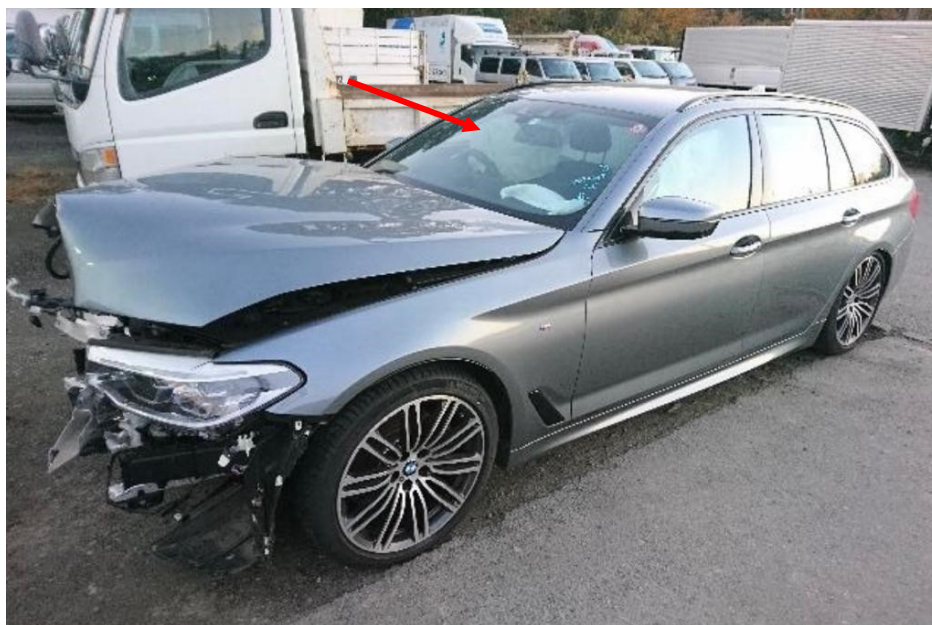
Photo 2 shows the front left body of the Motor Car (photograph provided to me). The Motor Car was observed to have sustained damage at its frontal portion. The front bumper and all its related parts and attachments, front left headlamp, front bonnet and front left fender inner shield were amongst the body parts that were observed to have been damaged. The right side curtain airbag (arrowed) was observed to be deployed.
