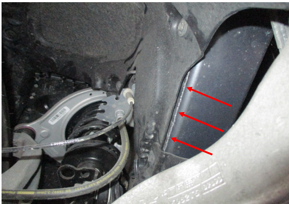
Photo 24 shows the chassis/structural body at the underside front right of the Motor Car. The original factory sealant (arrowed) at the joints along the chassis/structural body was observed to be untouched. In general, I had found no work was carried out on the chassis/structural body of the Motor Car. The chassis/structural body of the Motor Car was originally fitted.
