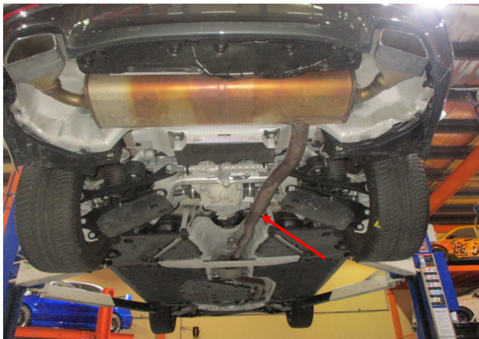
Photo 21 shows a general view of the Motor Car's exhaust system. My examination of the Motor Car's exhaust system revealed no sign(s) or indication(s) of any cut or weld marks along its catalytic converter, centre resonator box, exhaust pipe (arrowed) and on its rear muffler.
