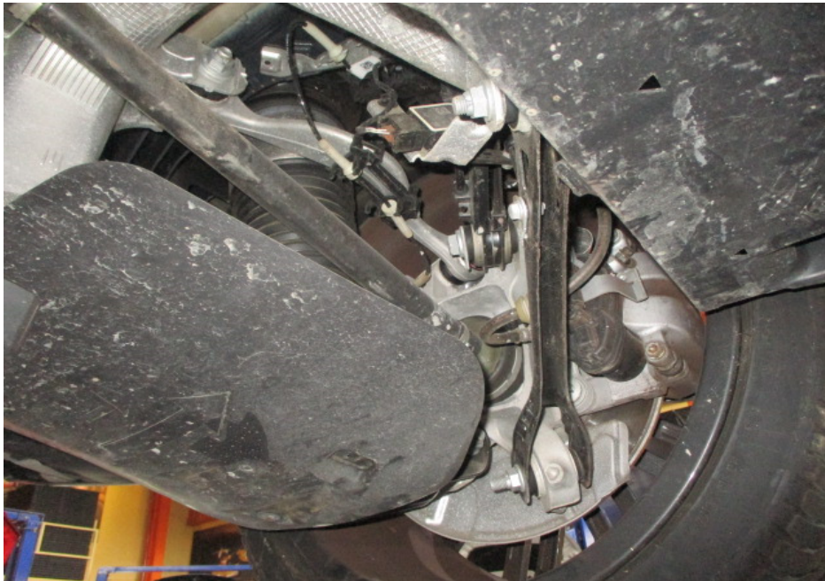
Photo 18 shows a general view of the control arms and linkages at the rear left wheel of the Motor Car. I did not observe any fluid leak and/or fluid stain on the underside of the Motor Car. All of the Motor Car's undercarriage components were observed to be intact and secured in an appropriate manner.
