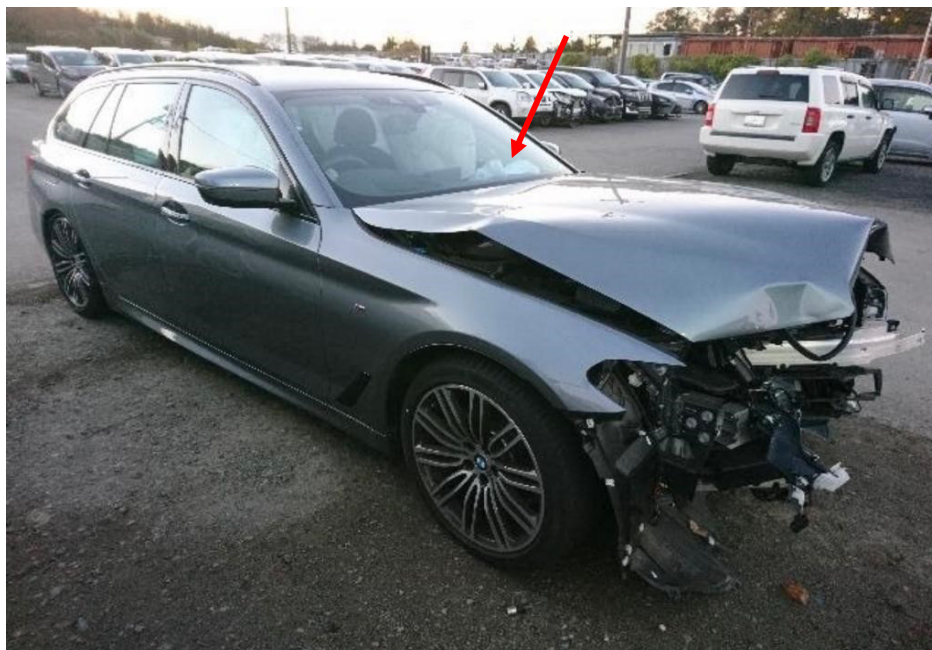
Photo 1 shows the front right body of the Motor Car (photograph provided to me). The Motor Car was observed to have sustained damage at its frontal portion. The front bumper and all its related parts and attachments, front bumper reinforcement, front radiator grilles, front right headlamp and front bonnet were amongst the body parts that were observed to have been damaged. The front left passenger airbag (arrowed) was observed to be deployed.
