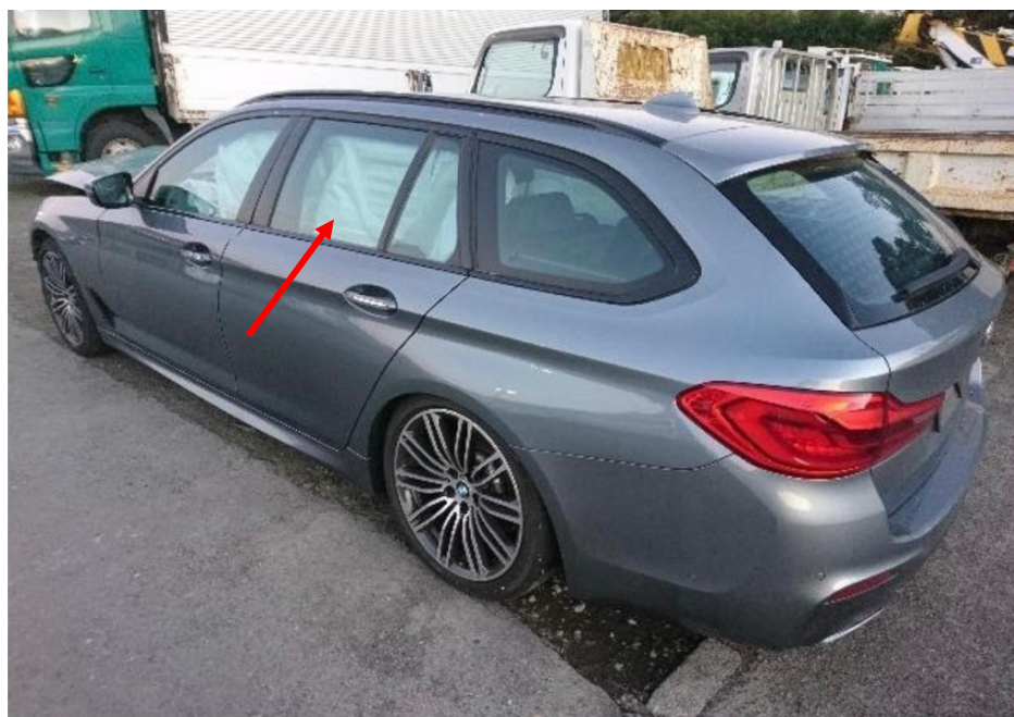
Photo 4 shows the rear left body of the Motor Car (photograph provided to me). The left side curtain airbag (arrowed) was observed to be deployed. Apart for the frontal portion, there was no physical damage seen to other areas of the Motor Car.
