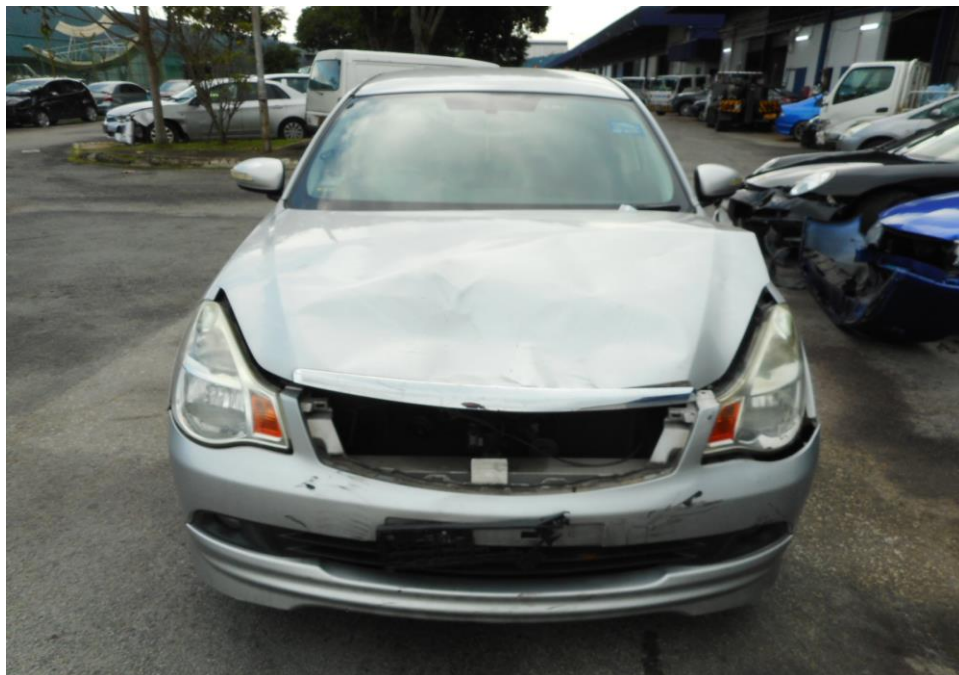
Photo 3 shows a general view of the Motor Car's front body at the time of my inspection. The front portion of the Motor Car was observed to have sustained damage. Its front bonnet, front grille and front bumper was the body parts that were damaged as a result of the accident.
