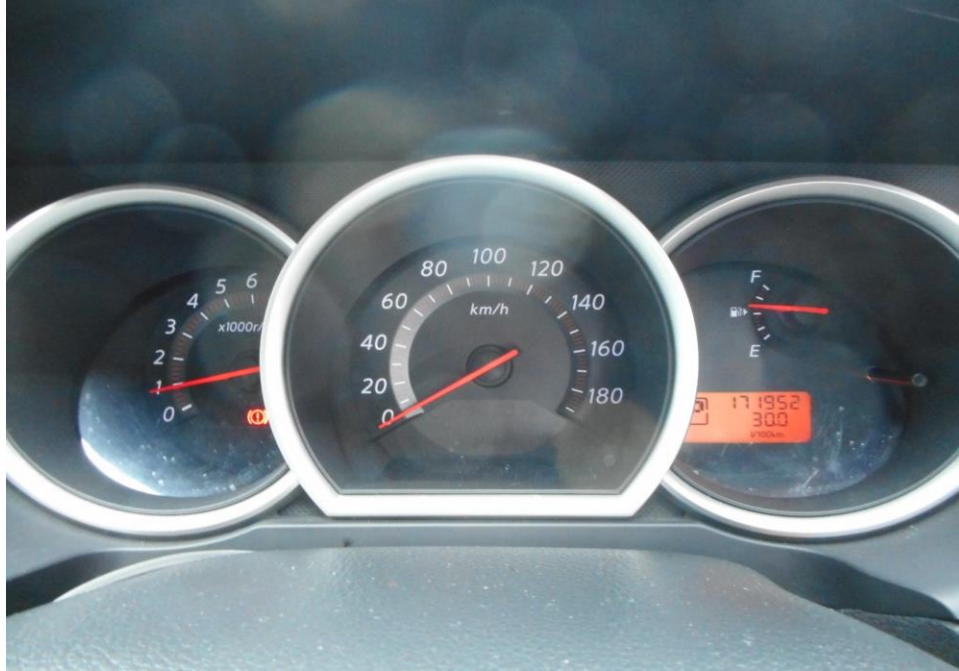
Photo 25 shows no warning lights illuminated on the instrument panel of the Motor Car after the engine was cranked. This would suggest that there was no abnormality to the electronic operating system of the Motor Car, like the ABS, EPS, and SRS etc.
