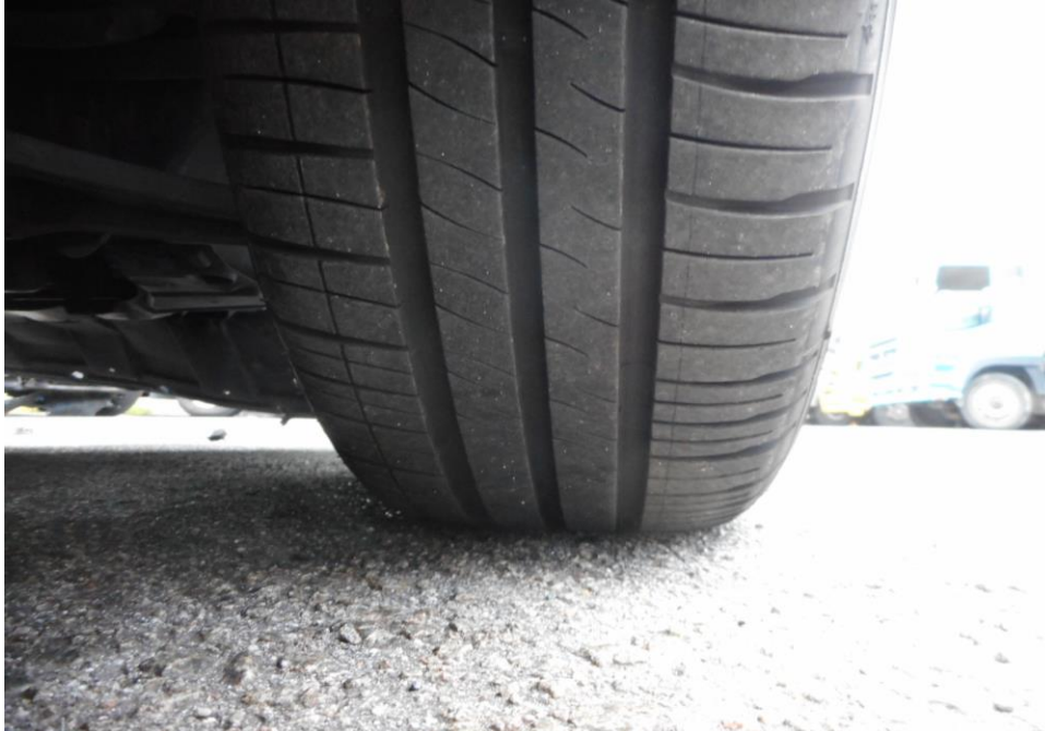
Photo 8 shows the condition of the front right tyre of the Motor Car, which was observed to be in serviceable condition with remaining tread depth of approximately 5.6mm. The tyre was sufficiently inflated for vehicular operation with no tear, cut or burst mark(s) on the outer and the inner sidewalls as well as across the tread. The 4 tyres of the Motor Car were wrapped around standard steel wheel rims without any damage.
