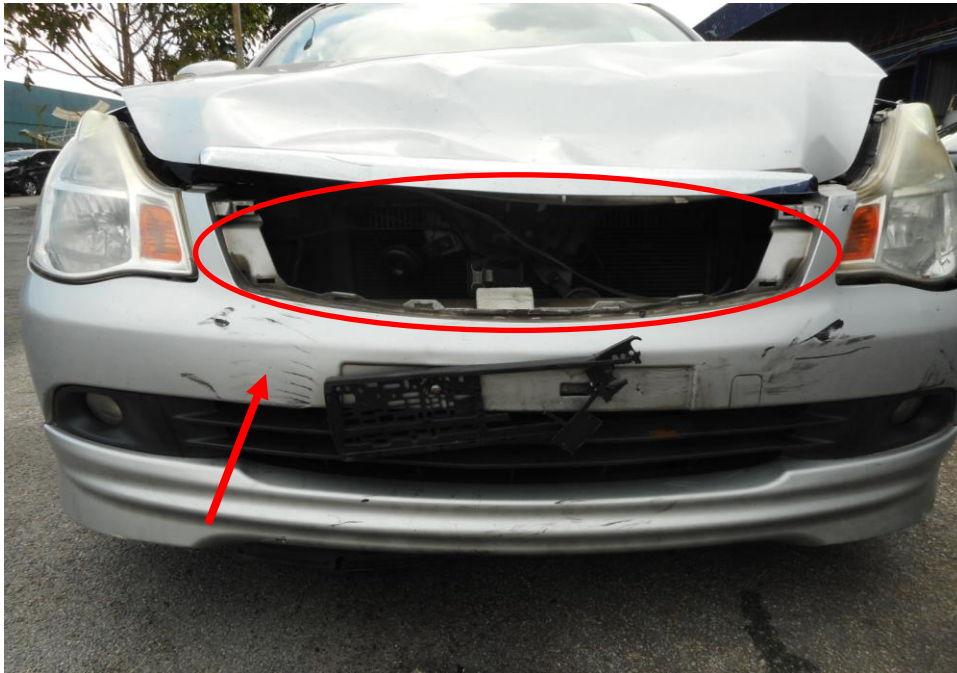
Photo 5 shows the close up view of the Motor Car's front body at the time of my inspection. The Motor Car was observed to have sustained damage at its front grille (circled) and front bumper (arrowed) as a result of the accident.
