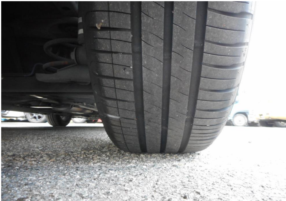
Photo 9 shows the condition of the rear right tyre of the Motor Car, which was observed to be in serviceable condition with remaining tread depth of approximately 4.9mm. The tyre was also observed to be sufficiently inflated for vehicular operation with no tear, cut or burst mark(s).
