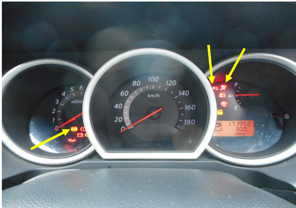
Photo 24 shows the warning light for Anti-Lock Brake System (ABS) and Power Steering System (EPS), and Supplemental Restraint System (SRS)) (arrowed) appearing on the instrument panel of the Motor Car during the self-test of its various electronic operating systems when its engine was cranked.
