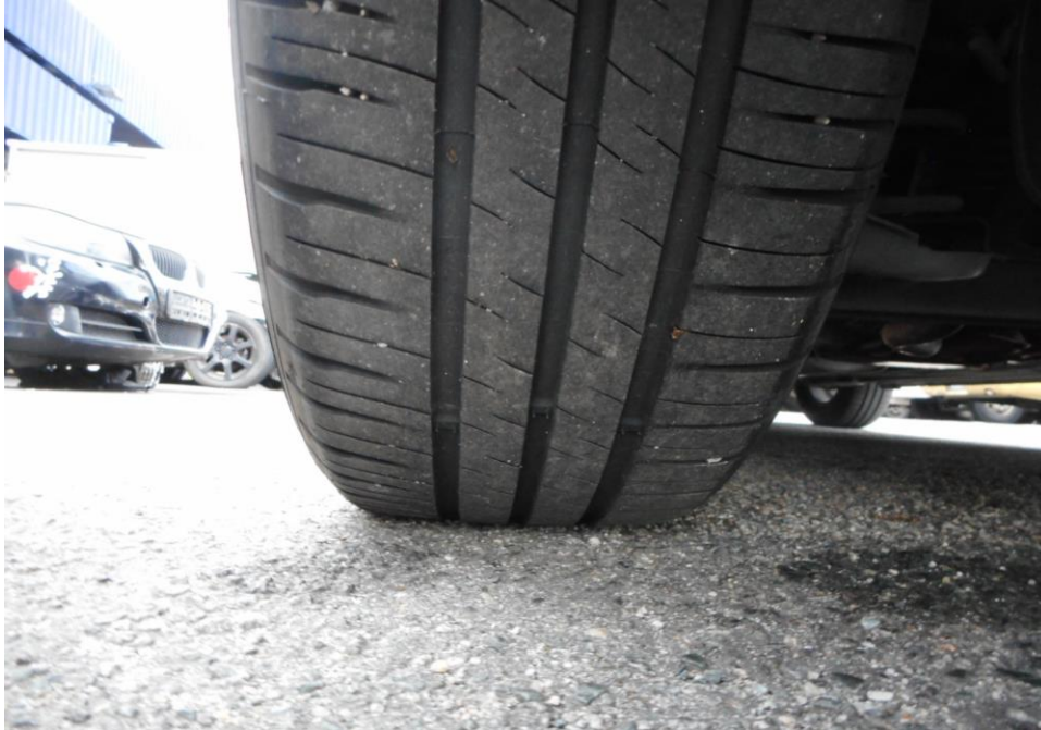
Photo 10 shows the condition of the rear left tyre of the Motor Car, which was observed to be in serviceable condition with remaining tread depth of approximately 4.6mm. The tyre, which was wrapped around steel wheel rim, was also observed to be sufficiently inflated for vehicular operation. The 4 tyres of the Motor Car were wrapped around standard steel wheel rims.
