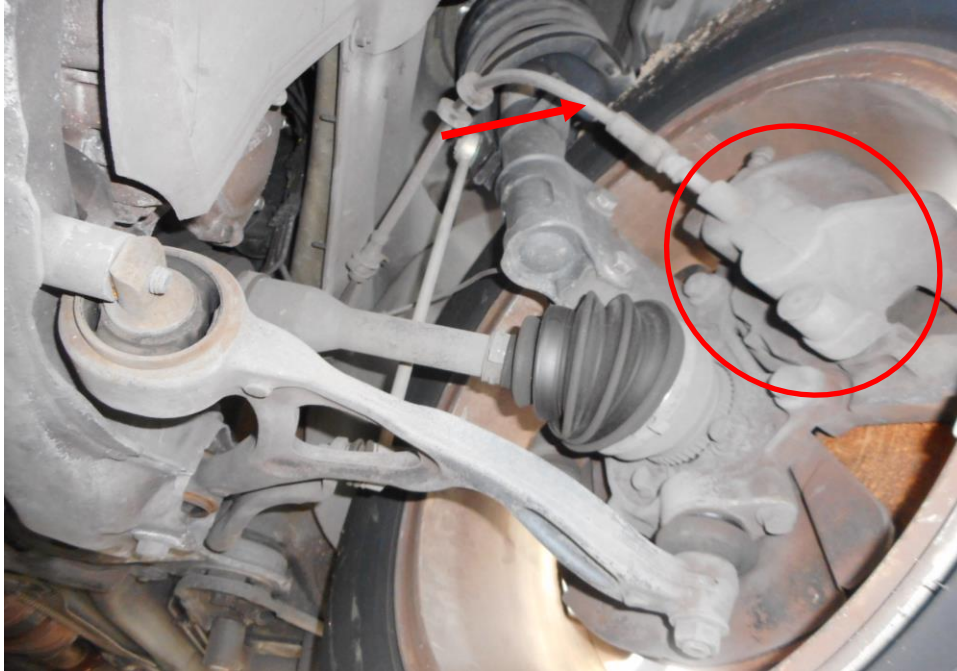
Photo 18 shows the brake hose/pipe (arrowed) at the front left wheel of the Motor Car. No leakage of brake fluid was observed. Visual examination of the various components of the braking system like the brake caliper (circled), brake booster, brake pedal etc had revealed all to be intact and without visible damage.
