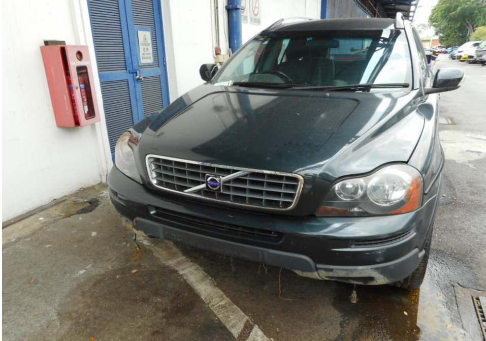
Photo 4 shows a general view of the Motor Car's front body at the time of my inspection. The front portion of the Motor Car was observed to have sustained damage. Its front bumper and number plate was the body parts that were damaged as a result of the accident.
