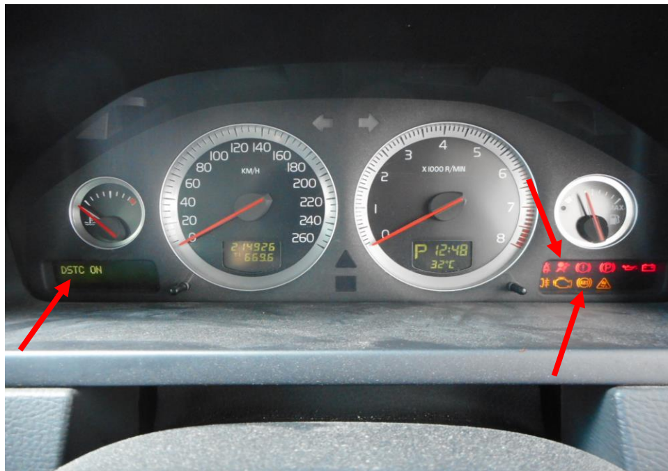
Photo 22 shows the warning light for Anti-Lock Brake System (ABS), Supplemental Restraint System (SRS) and Traction Control (TC) (arrowed) appearing on the instrument panel of the Motor Car during the self-test of its various electronic operating systems when its engine was cranked.
