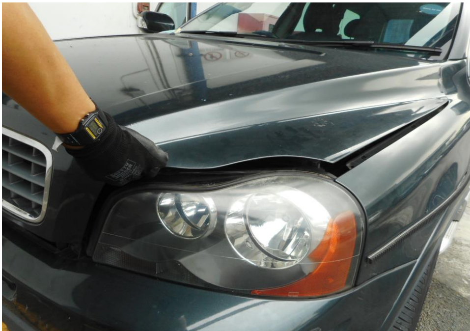
Photo 12 shows a general view of the front bonnet and the attempt to open the front bonnet of the Motor Car. However, the lock and level mechanism of the front bonnet was likely damaged by the accident resulting it unable to open. (Unable to open)
