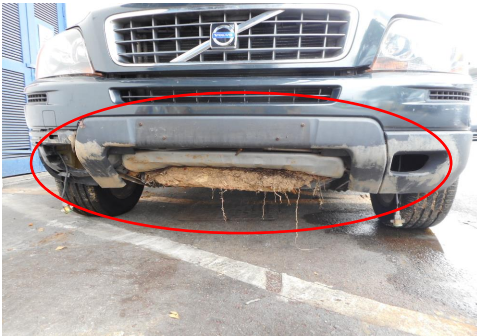
Photo 5 shows the close up view of the Motor Car's front body at the time of my inspection. The front portion of the Motor Car was observed to have sustained damage. Its front bumper and number plate (circled) was the body parts that were damaged as a result of the accident.
