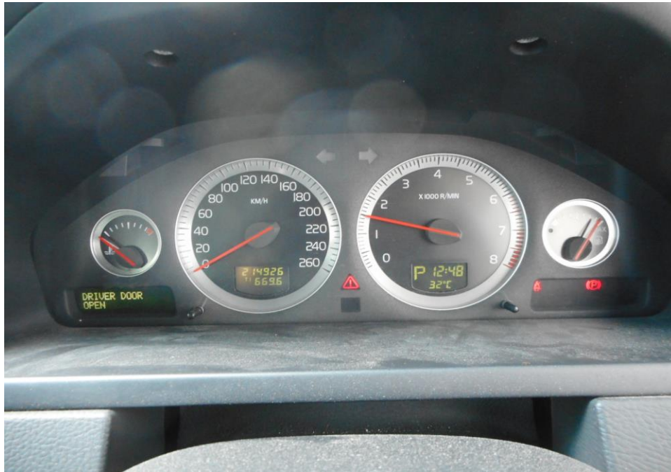
Photo 23 shows no warning lights illuminated on the instrument panel of the Motor Car after the engine was cranked. This would suggest that there was no abnormality to the electronic operating system of the Motor Car, like the ABS, SRS and TC etc.
