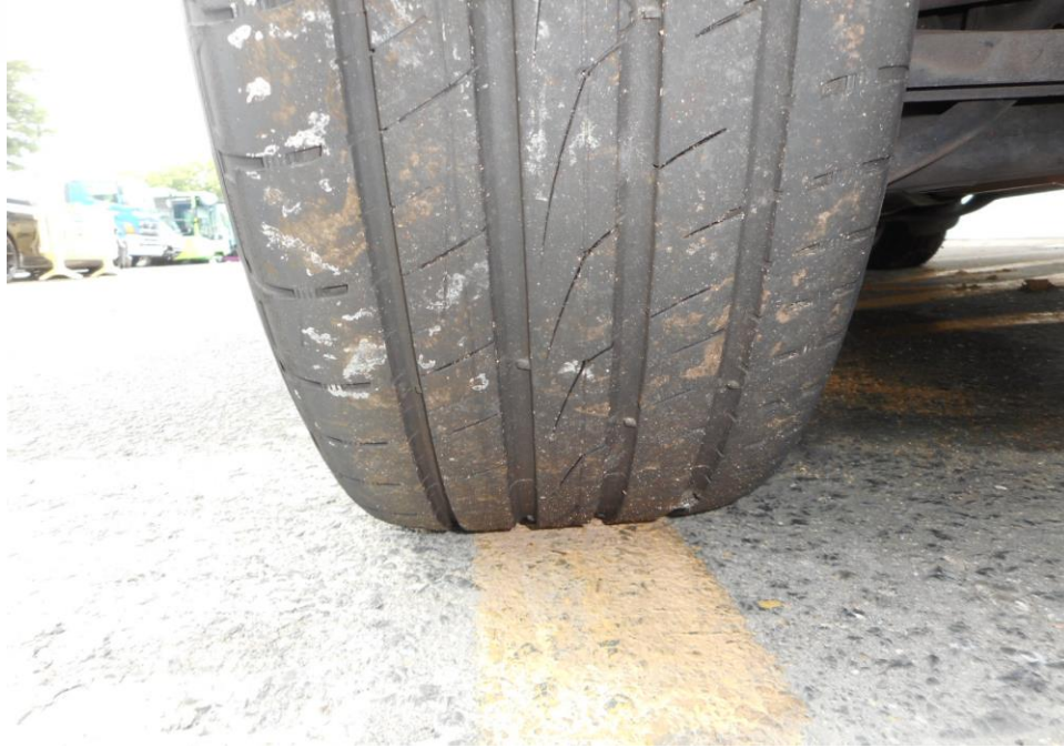
Photo 10 shows the condition of the rear left tyre of the Motor Car, which was observed to be in serviceable condition with remaining tread depth of approximately 5.8mm. The tyre, which was wrapped around steel wheel rim, was also observed to be sufficiently inflated for vehicular operation. The 4 tyres of the Motor Car were wrapped around standard steel wheel rims.
