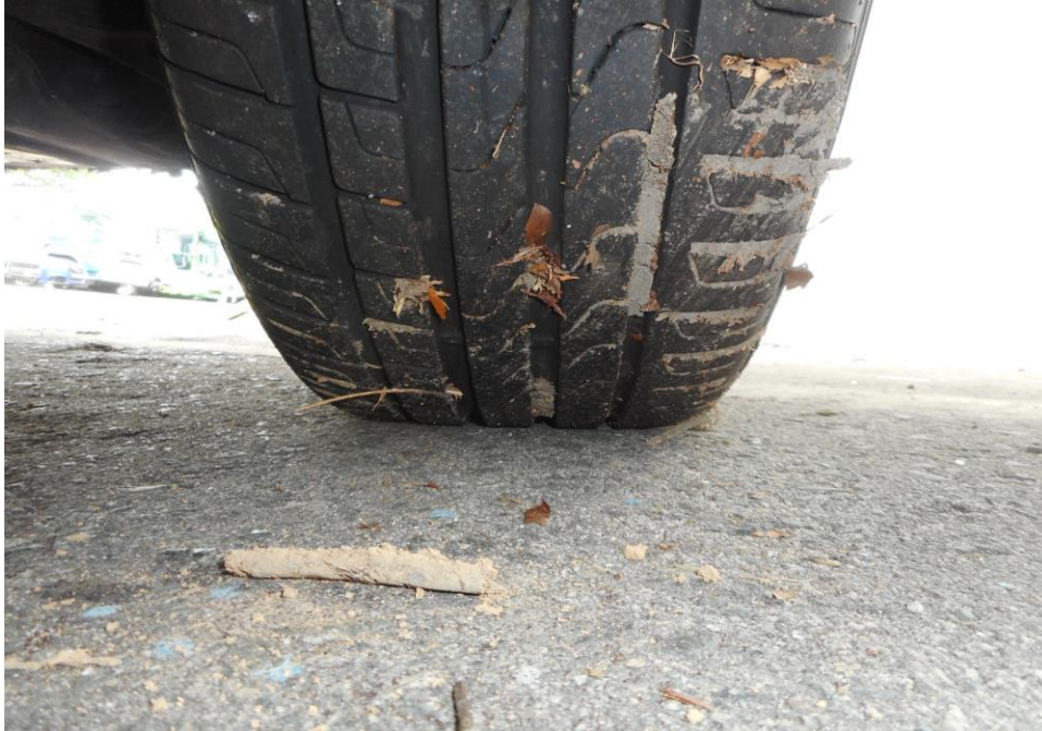
Photo 8 shows the condition of the front right tyre of the Motor Car, which was observed to be in serviceable condition with remaining tread depth of approximately 6.2mm. The tyre was sufficiently inflated for vehicular operation with no tear, cut or burst mark(s) on the outer and the inner sidewalls as well as across the tread. The 4 tyres of the Motor Car were wrapped around standard steel wheel rims without any damage.
