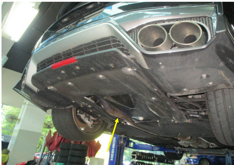
Photo 18 shows a general view of the rear section of the Motor Car's exhaust system. My examination of the Motor Car's exhaust system revealed no sign(s) or indication(s) of any cut or weld marks along its exhaust pipes (arrowed), on its catalytic converters, centre resonator box and its rear mufflers.
