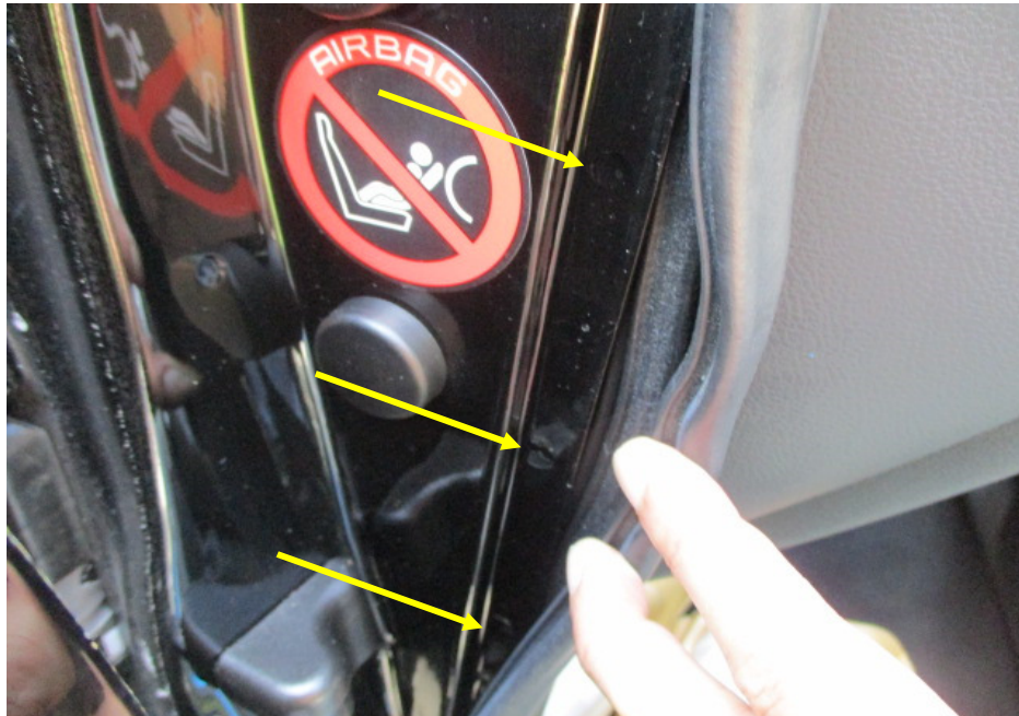
Photo 24 shows the left side "A" pillar of the Motor Car. I did not find any weld marks other than original spot weld marks (arrowed) on the left side "A" pillar of the Motor Car which, indicates that there was no re-welding works carried out. In general, I had found all the non-detachable body panels of the Motor Car to be originally fitted at the time of my inspection.
