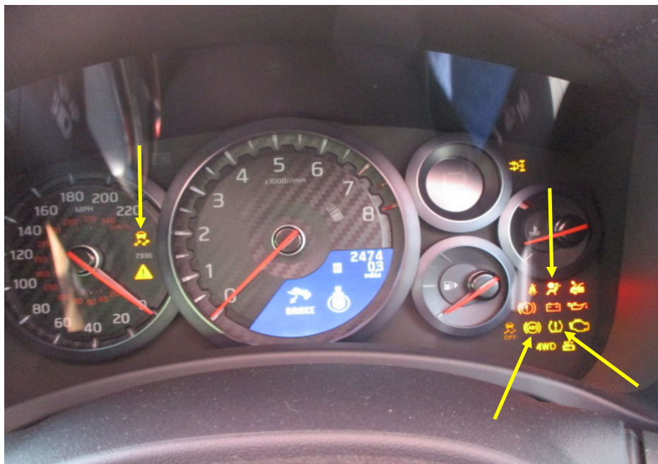
Photo 12 shows the warning lights for the various electronic safety features appearing on the instrument panel of the Motor Car during its self-test when the engine is cranked, in particular the ABS, SRS, TPM and VDC lights (arrowed).
