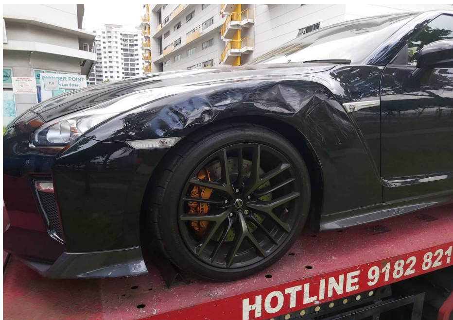
Photo 2 shows a closer view of the damage to the front left fender of the Motor Car (photograph provided to me). There was no physical damage seen to other areas of the Motor Car apart for this damage at the front left fender.
