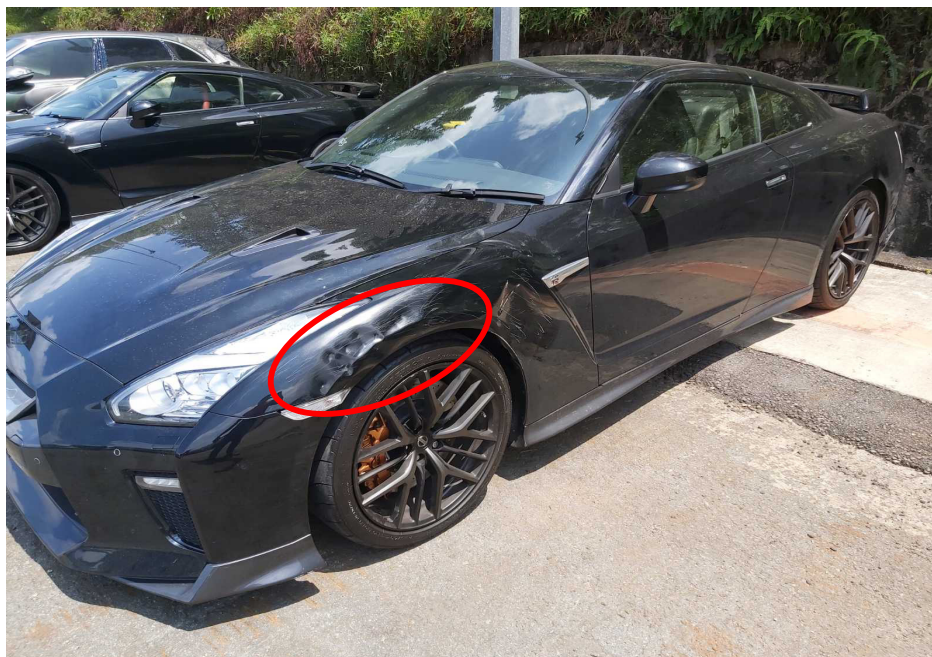
Photo 1 shows the front left body of the Motor Car (photograph provided to me). The Motor Car was observed to have sustained damage at its front left portion (circled). From the photographs provided, I had observed damage to only the front left fender of the Motor Car. The airbags of the Motor Car were not activated.
