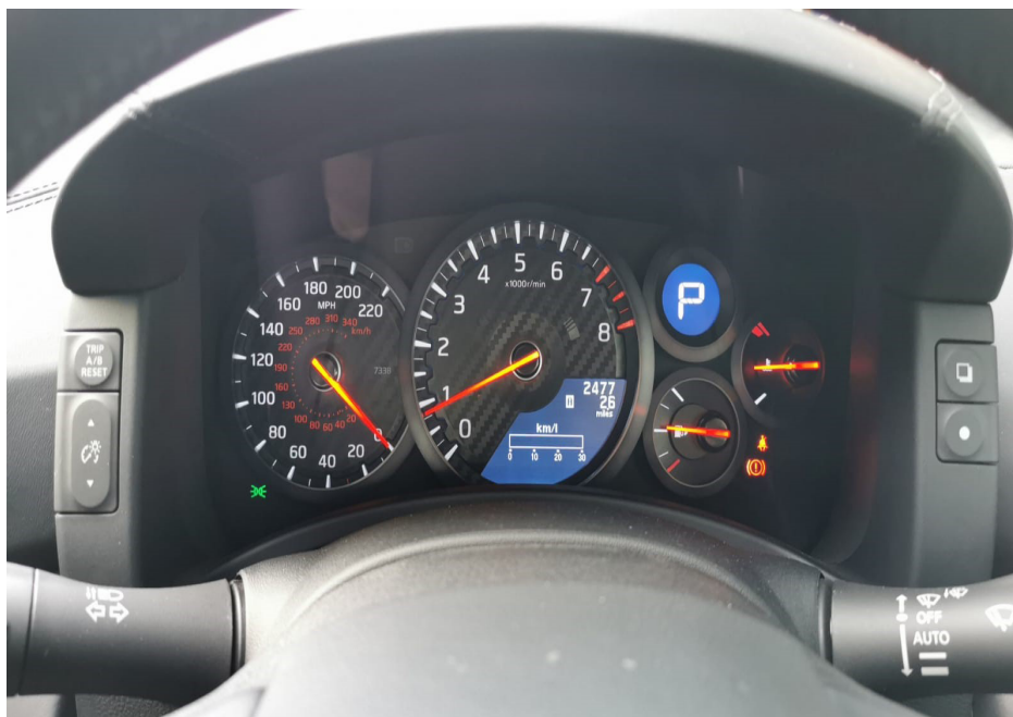
Photo 13 shows the respective warning lights no longer illuminated, indicating that there is no fault detected to the ABS, SRS, TPM and VDC systems of the Motor Car during the self-test. These electronic systems were hence in working condition at the time of my inspection.
