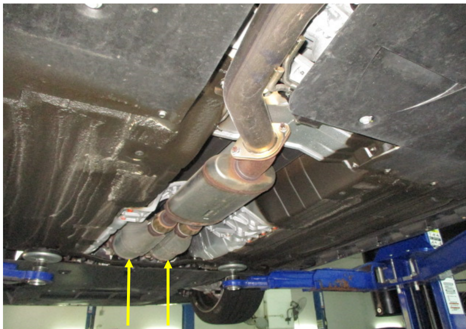
Photo 19 shows the front section of the Motor Car's exhaust system. My examination of the Motor Car's exhaust system revealed no sign(s) or indication(s) of any cut or weld marks along its exhaust pipes, on its catalytic converters (arrowed), centre resonator box and its rear mufflers.
