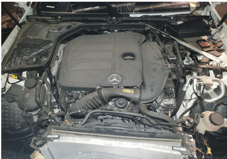
Photo 3 shows the engine compartment of the Motor Car (photograph provided to me). Physical damage was seen to the aircon condenser, radiator, cooling fan and air hose amongst others. The front left and front right headlamp top panels and front top centre panel amongst others were also observed to be missing/dislodged.
