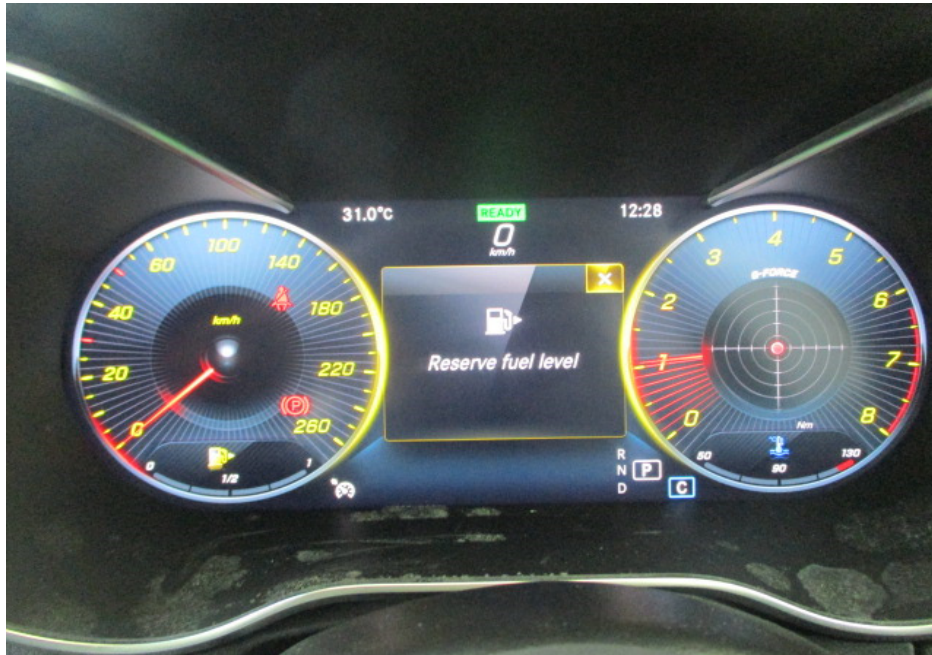
Photo 14 shows the respective warning lights no longer illuminated, indicating that there is no fault detected to the ABS, SRS, EPS and TCS systems of the Motor Car during the self-test. These electronic systems were hence in working condition at the time of my inspection.
