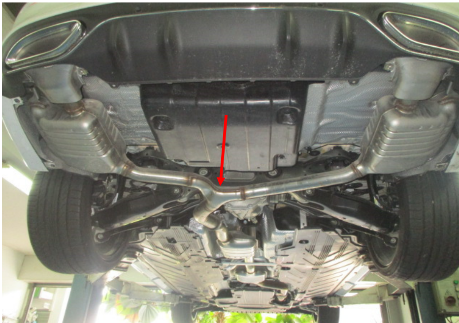
Photo 19 shows a general view of the rear section of the Motor Car's exhaust system. My examination of the Motor Car's exhaust system revealed no sign(s) or indication(s) of any cut or weld marks along its exhaust pipes (arrowed), on its catalytic converter, centre resonator boxes and its rear mufflers.
