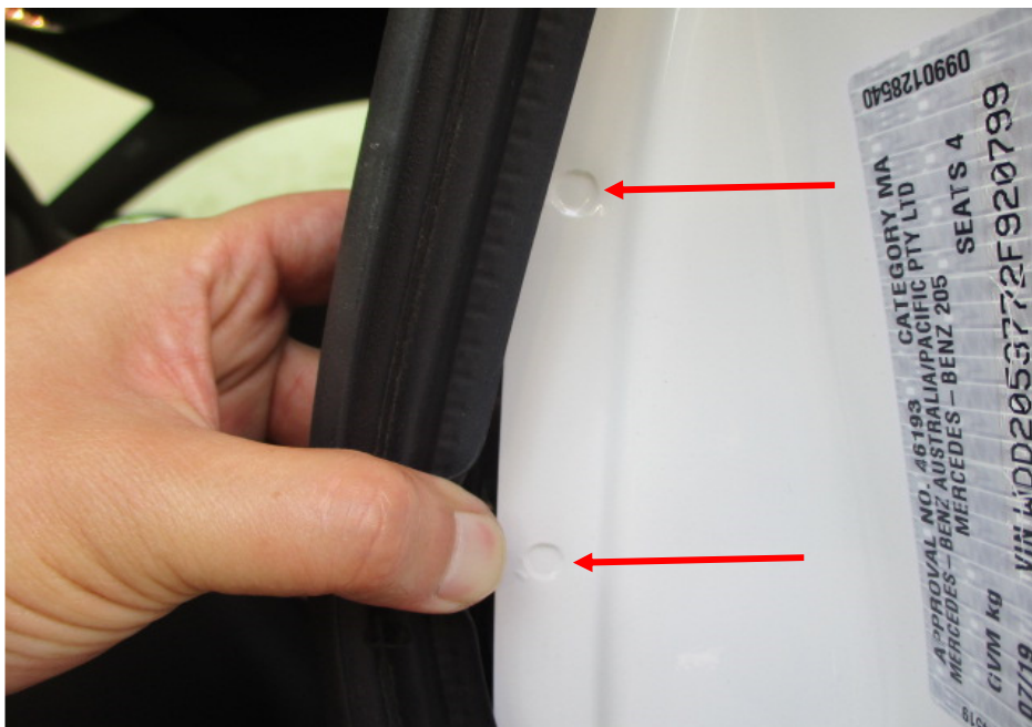
Photo 23 shows the left side rear body panel of the Motor Car. I did not find any weld marks other than original spot weld marks (arrowed) on the left side rear body panel of the Motor Car which, indicates that there was no re-welding works carried out. In general, I had found all the non-detachable body panels of the Motor Car to be originally fitted at the time of my inspection.
