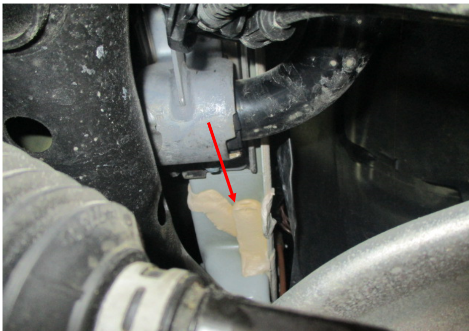
Photo 20 shows the chassis/structural body at the underside front right of the Motor Car. I did not find any weld marks other than original spot weld marks on the chassis/structural body of the Motor Car. The original factory sealant (arrowed) at the joints along the chassis/structural body was untouched, indicating no work was done on the chassis/structural body of the Motor Car and that the chassis/structural body was originally fitted.
