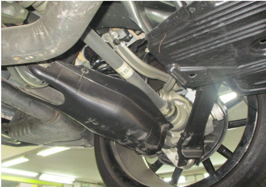
Photo 16 shows a general view of the control arms and linkages at the rear left wheel of the Motor Car. I did not observe any fluid leak and/or fluid stain on the underside of the Motor Car. All of the Motor Car's undercarriage components were observed to be intact and secured in an appropriate manner.
