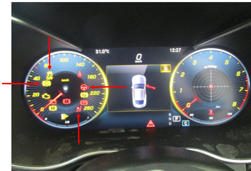
Photo 13 shows the warning lights for the various electronic safety features appearing on the instrument panel of the Motor Car during its self-test when the engine is cranked, in particular the ABS, SRS, EPS and TCS lights (arrowed).
