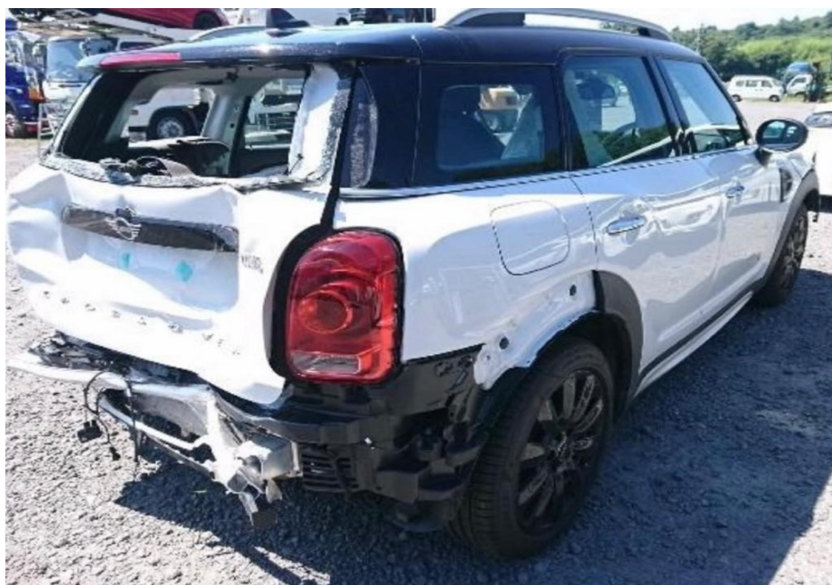
Photo 2 shows the rear right body of the Motor Car (photograph provided to me). The Motor Car was observed to have sustained damage at its rear portion. Physical damage was seen to the rear tailgate, rear tailgate top garnish, rear windscreen and rear right fender wheel arc garnish amongst others.
