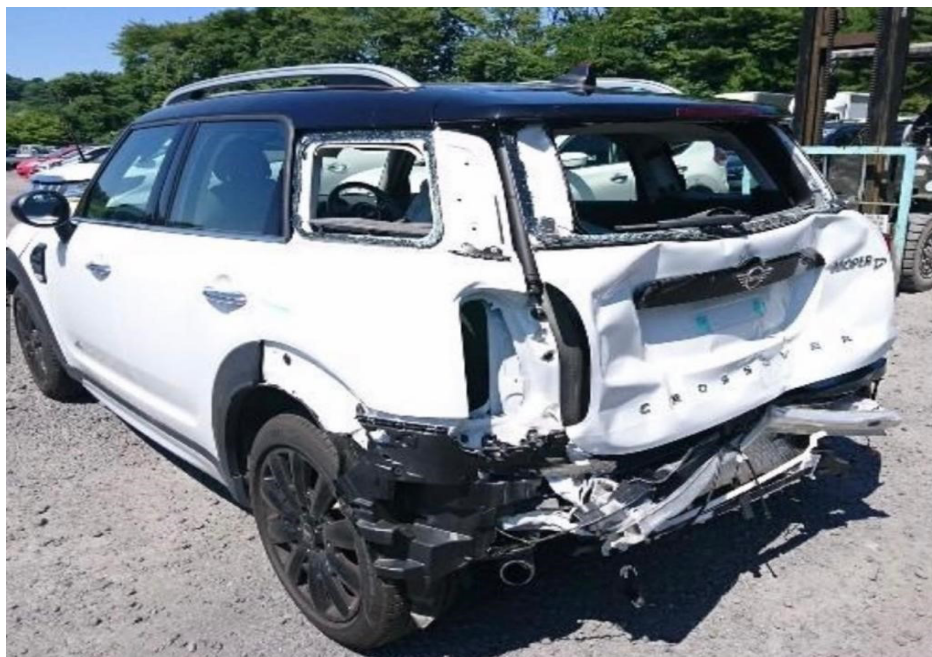
Photo 1 shows the rear left body of the Motor Car (photograph provided to me). The Motor Car was observed to have sustained damage at its rear portion. The front bumper and all its related attachments and rear left taillamp were missing/dislodged. Physical damage was seen to the rear bumper reinforcement, rear exhaust muffler, rear left fender, rear left fender glass, rear left fender wheel arc garnish and rear end panel amongst others.
