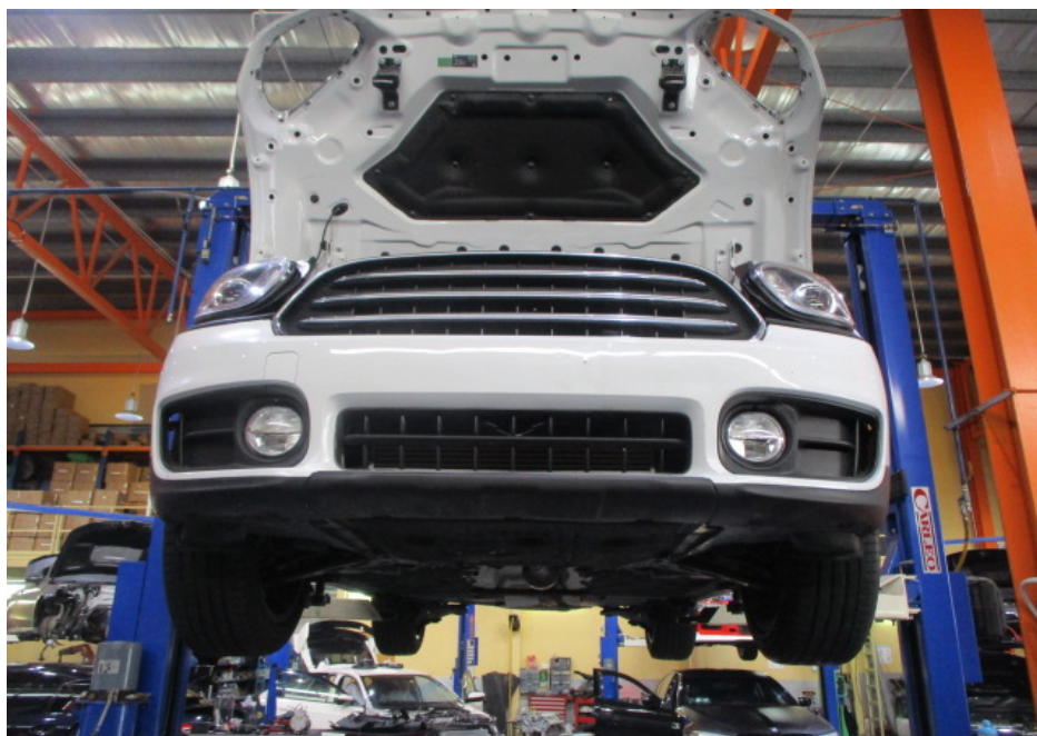
Photo 19 shows the Motor Car hoisted up for checks on its undercarriage. There was no sign(s) or indication(s) of fluid leakage and/or fluid stain(s) on the underside of the Motor Car. The undercarriage components of the Motor Car were also all observed to be intact and secured in an appropriate manner.
