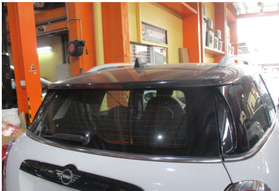
Photo 12 shows a closer view of the rear tailgate, rear tailgate top garnish and rear windscreen of the Motor Car. The body parts at the rear portion of the Motor Car were visually examined and it was observed that the repair/restoration works carried out to the damaged area of the Motor Car (refer to photograph 1 & 2 above) were reasonably adequate and in order.
