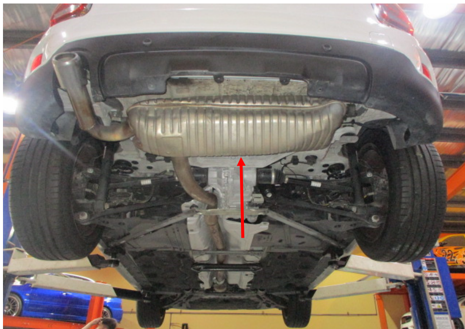
Photo 23 shows a general view of the Motor Car's exhaust system. My examination of the Motor Car's exhaust system revealed no sign(s) or indication(s) of any cut or weld marks along its exhaust pipes, rear muffler (arrowed) and on its catalytic converter.
