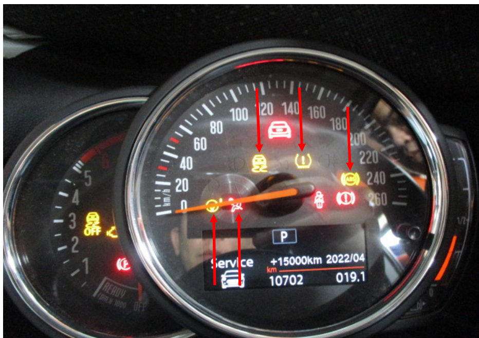
Photo 17 shows the warning lights for the various electronic safety features appearing on the instrument panel of the Motor Car during its self-test when the engine is cranked, in particular the ABS, SRS, PAS, TPM and DSC lights (arrowed).
