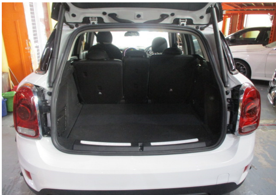
Photo 13 shows the rear boot compartment of the Motor Car at the time of my inspection. All inner trims, hinges and upholstery etc were observed to be properly fitted. The body parts at the rear portion of the Motor Car were visually examined and the repair/restoration works carried out to the damaged area of the Motor Car (refer to photograph 1 & 2 above) were found to be reasonably adequate and in order.
