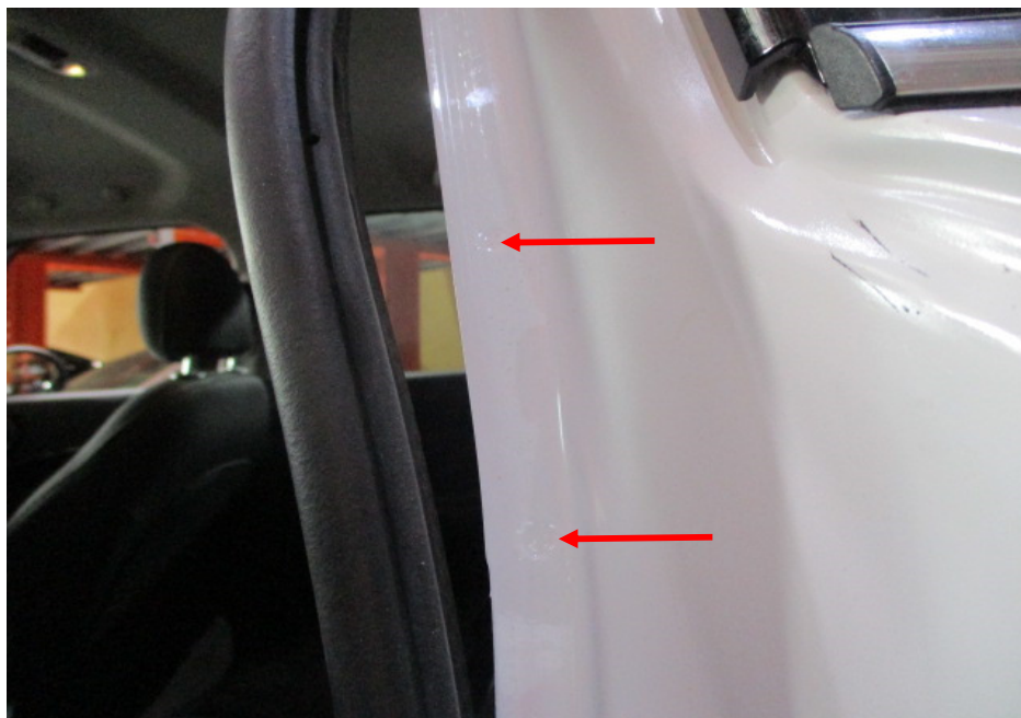
Photo 27 shows the left side "C" pillar of the Motor Car. I did not find any weld marks other than original spot weld marks (arrowed) on the left side "C" pillar of the Motor Car which, indicates that there was no re-welding works carried out. In general, I had found all the non-detachable body panels of the Motor Car to be originally fitted at the time of my inspection.
