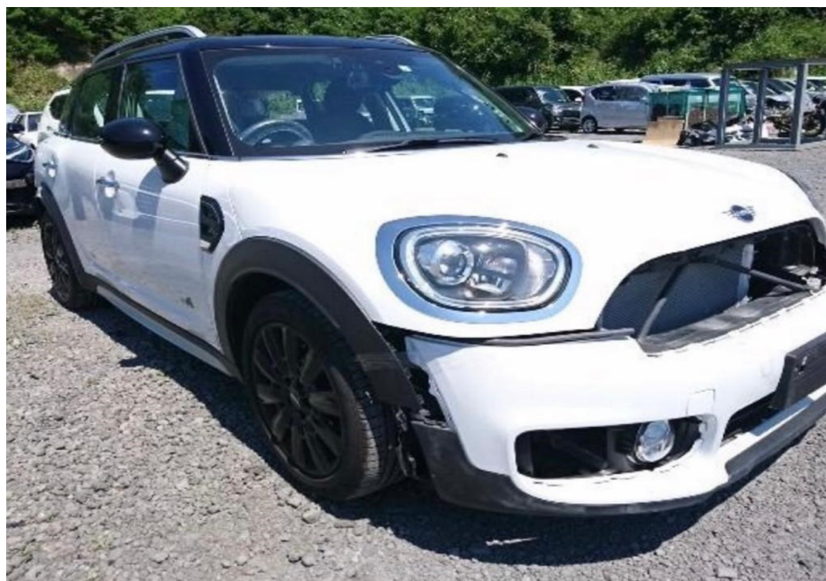
Photo 4 shows the front right body of the Motor Car (photograph provided to me). Apart for the rear portion, the Motor Car had also sustained damage at its frontal portion. The front right fog lamp garnish and front radiator grille were observed to be missing/dislodged. Physical damage was also seen to the front bumper, front right bumper right lower garnish and front right fender wheel arc garnish amongst others.
