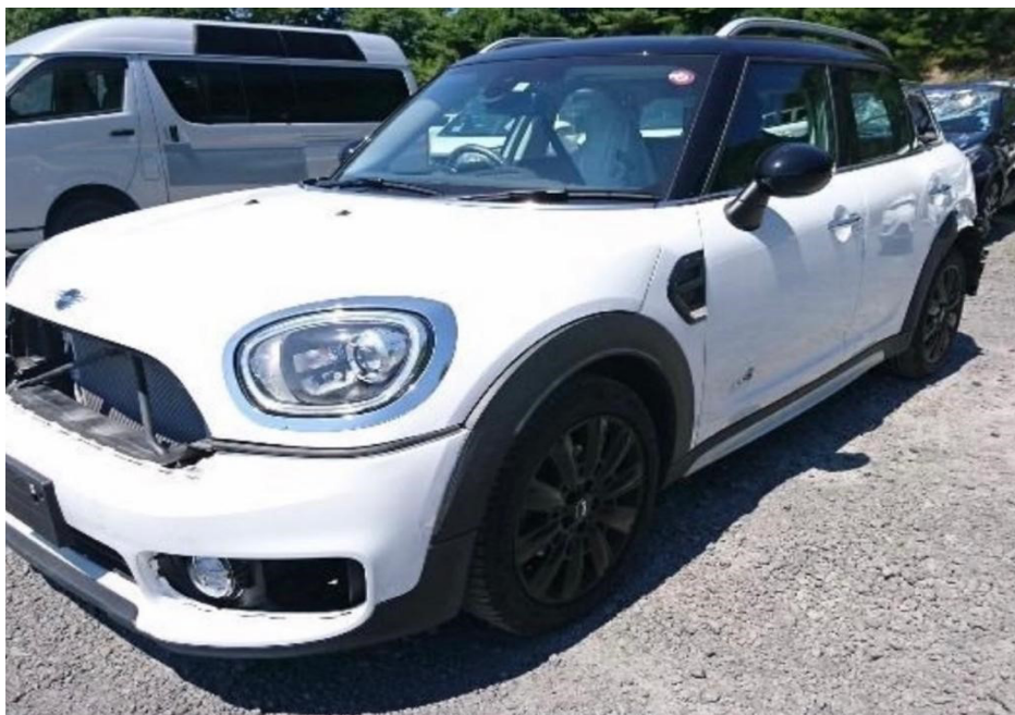
Photo 3 shows the front left body of the Motor Car (photograph provided to me). Apart for the rear portion, the Motor Car had also sustained damage at its frontal portion. The front left fog lamp garnish and front radiator grille were observed to be missing/dislodged.
