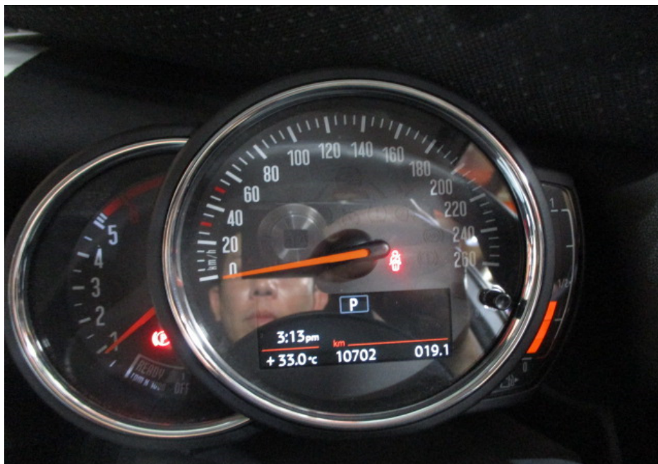
Photo 18 shows the respective warning lights no longer illuminated, indicating that there is no fault detected to the ABS, SRS, PAS, TPM and DSC systems of the Motor Car during the self-test. These electronic systems were hence in working condition at the time of my inspection.
