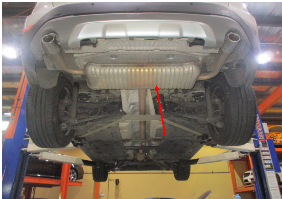
Photo 19 shows a general view of the Motor Car's exhaust system. My examination of the Motor Car's exhaust system revealed no sign(s) or indication(s) of any cut or weld marks along its exhaust pipes, on its rear muffler (arrowed) and on its catalytic converter.
