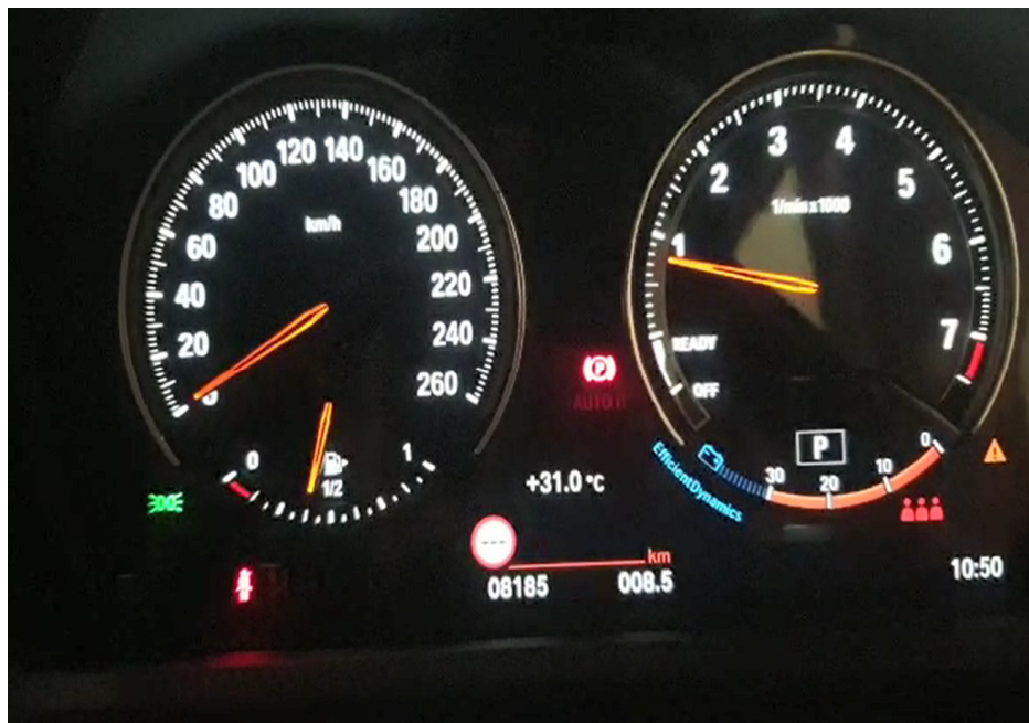
Photo 14 shows the respective warning lights no longer illuminated, indicating that there is no fault detected to the ABS, SRS, IAS, TPM and DSC systems of the Motor Car during the self-test. These electronic systems were hence in working condition at the time of my inspection.
