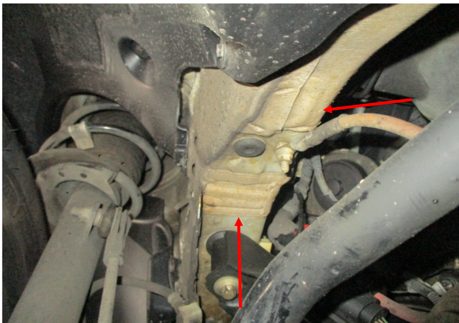
Photo 21 shows the chassis/structural body at the underside front left of the Motor Car. The original factory sealant (arrowed) at the joints along the chassis/structural body was observed to be untouched. In general, I had found no work was carried out on the chassis/structural body of the Motor Car. The chassis/structural body of the Motor Car was originally fitted.
