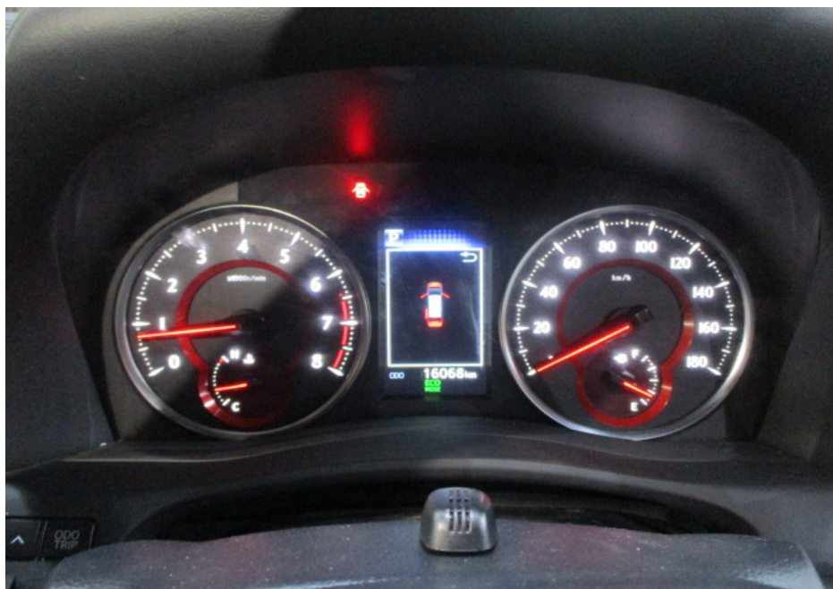
Photo 15 shows the respective warning lights no longer illuminated, indicating that there is no fault detected to the ABS, SRS, EPS and VSC systems of the Motor Car during the self-test. These electronic systems were hence in working condition at the time of my inspection.
