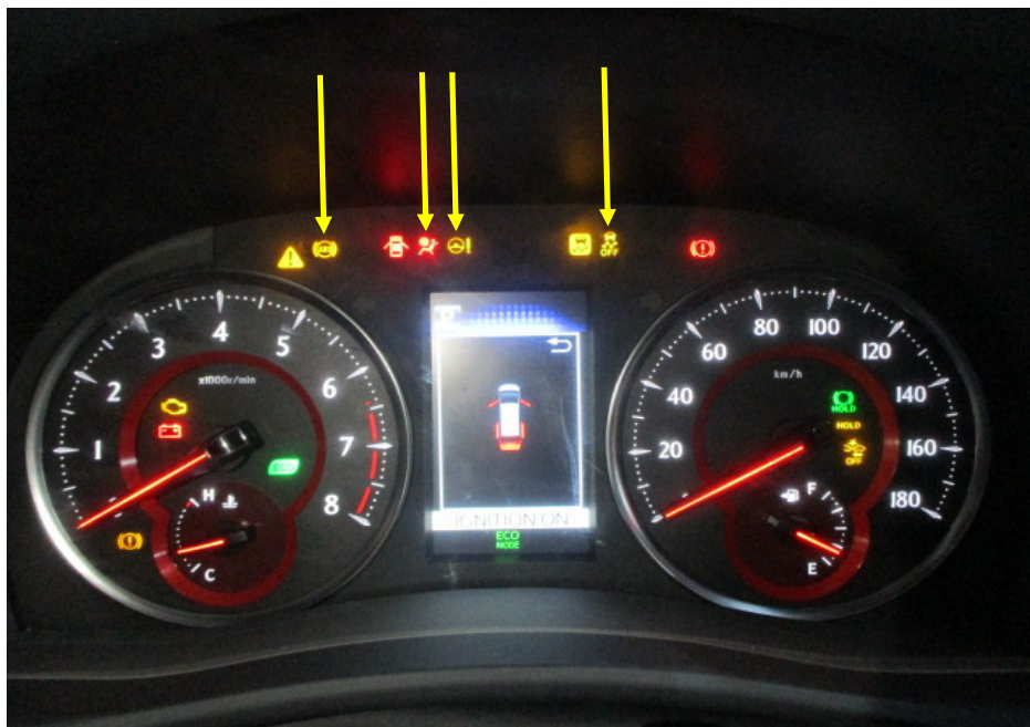
Photo 14 shows the warning lights for the various electronic safety features appearing on the instrument panel of the Motor Car during its self-test when the engine is cranked, in particular the lights for the ABS, SRS, EPS and VSC systems (arrowed).
