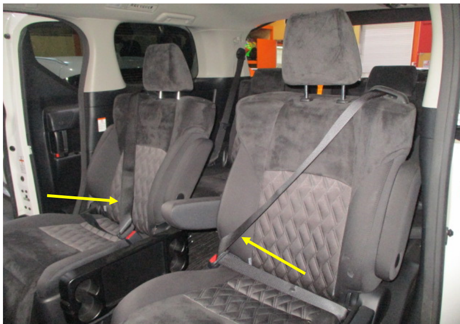
Photo 12 shows the rear seats at the 1 st row of the Motor Car. All the seats of the Motor Car were secured via seat rails to the floorboard. They were also fitted with a retractable seat belt reel and a pre-tensioner. The seat belts (arrowed) were tested and were able to be fastened into the respective pre-tensions that were fitted on the side of each individual seat.
