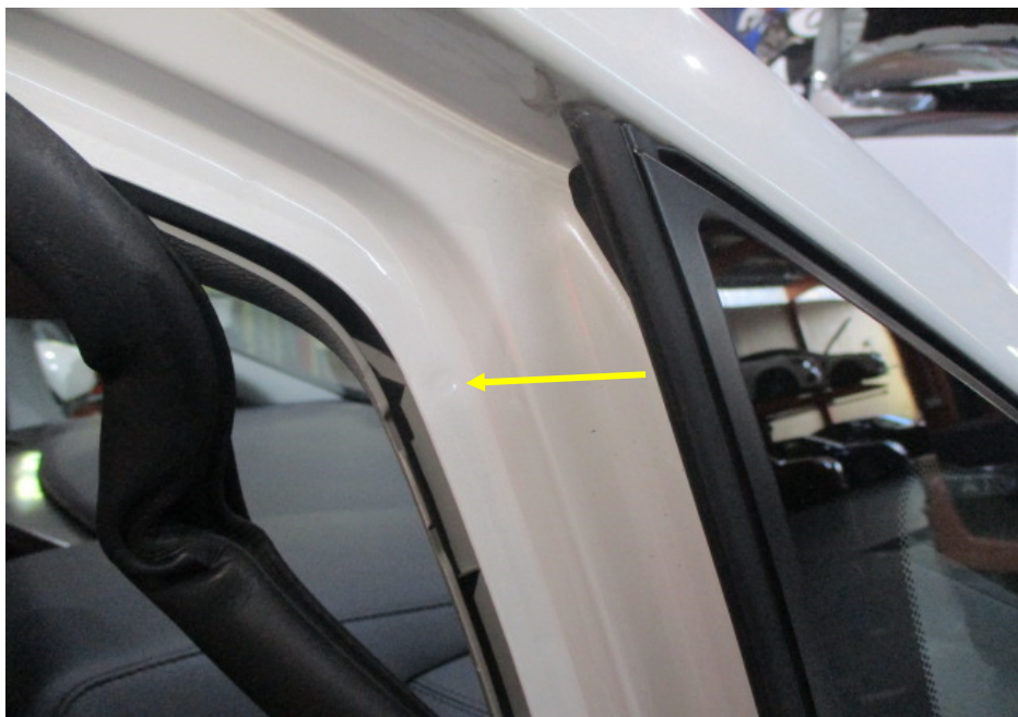
Photo 24 shows the right side “A” pillar of the Motor Car. I did not find any weld marks other than original spot weld marks (arrowed) on the right side “A” pillar of the Motor Car, which indicates that there was no re-welding works carried out. In general, I had found all the non-detachable body panels of the Motor Car to be originally fitted at the time of my inspection.
