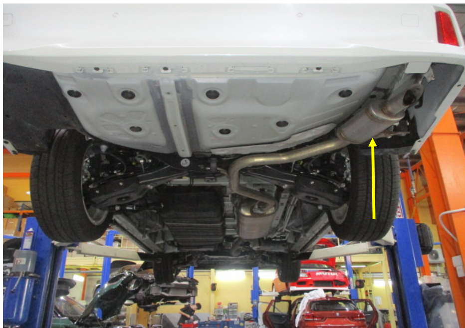
Photo 20 shows a general view of the Motor Car's exhaust system. My examination of the Motor Car's exhaust system revealed no sign(s) or indication(s) of any cut or weld marks along its exhaust pipes, rear muffler (arrowed), centre resonator box and on its catalytic converter.
