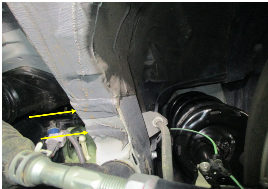
Photo 21 shows the chassis/structural body at the underside front right of the Motor Car. I did not find any weld marks other than original spot weld marks on the chassis/structural body of the Motor Car. The original factory sealant (arrowed) at the joints along the chassis/structural body was untouched, indicating no work was done on the chassis/structural body of the Motor Car and that the chassis/structural body was originally fitted.
