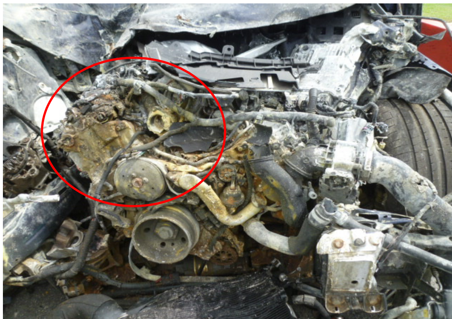
Photo 2 shows the general view of the engine compartment of the Insured Vehicle at the time of our inspection. The Insured Vehicle was observed to have sustained serious fire damage at the engine compartment (circled).
