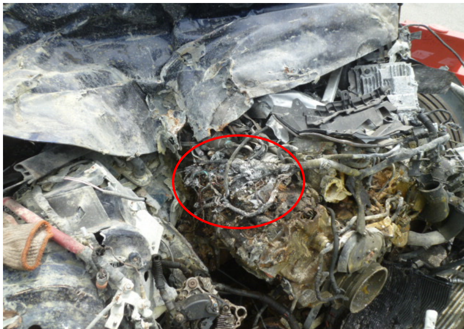
Photo 7 shows the engine compartment of the Insured Vehicle. We found greenish residue on some of the wirings around the rear centre portion of the engine compartment of the Insured Vehicle (circled).
