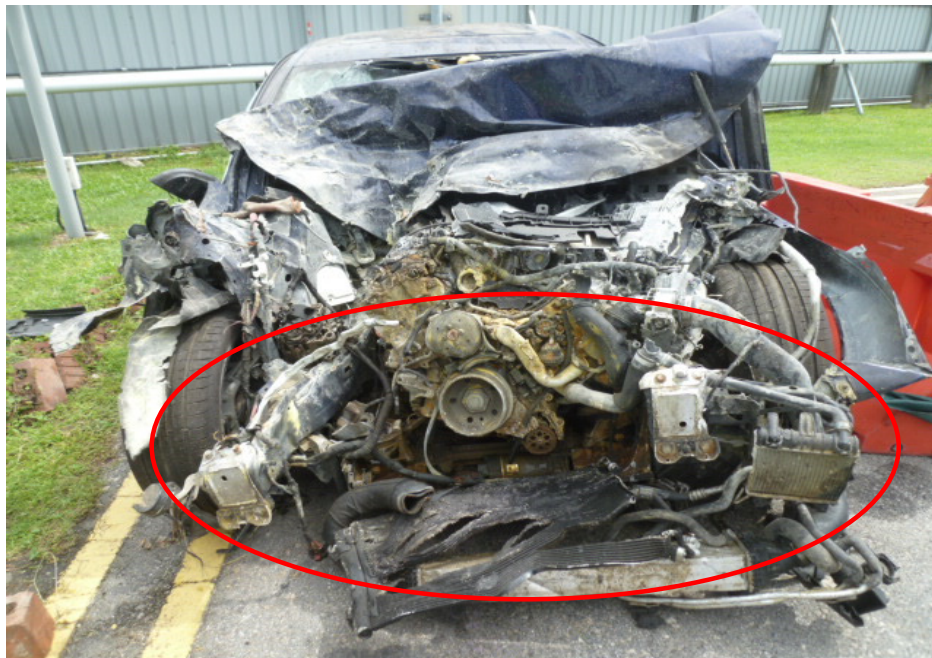
Photo 3 shows the frontal portion of the Insured Vehicle. Impact damage was observed at its front side (circled). Its front wheels, front support panel, front bumper and front bumper reinforcement were amongst the body parts that were bent/ buckled as a result of the impact force.
