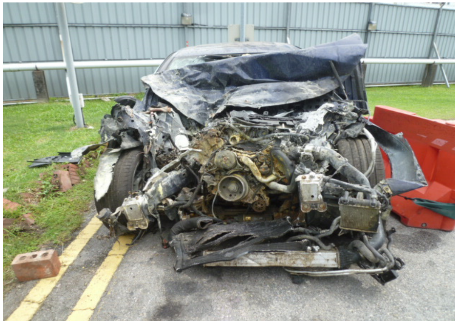
Photo 1 shows the general view of the frontal portion of the Insured Vehicle at the time of our inspection. The Insured Vehicle was observed to have sustained serious fire damage at the engine compartment. The Insured Vehicle had also sustained a direct impact of significant force onto its front side. Its front wheels, front support panel, front bumper and front bumper reinforcement were amongst the body parts that were bent/ buckled as a result of the impact force.
