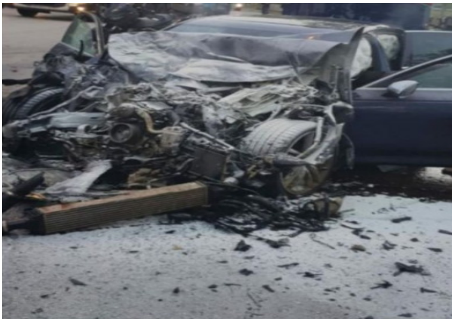
Photo 14 shows the Insured Vehicle after the fire was put out. In general, the information that could be gathered from this photograph had corresponded to the events that were related to us by Mr Raffid, which is the fire started from the front bonnet almost immediately after the collision.
