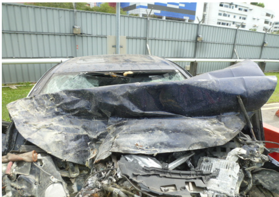
Photo 4 shows the front bonnet of the Insured Vehicle. Its front bonnet was amongst the body parts that was bent/ buckled as a result of the impact force.
