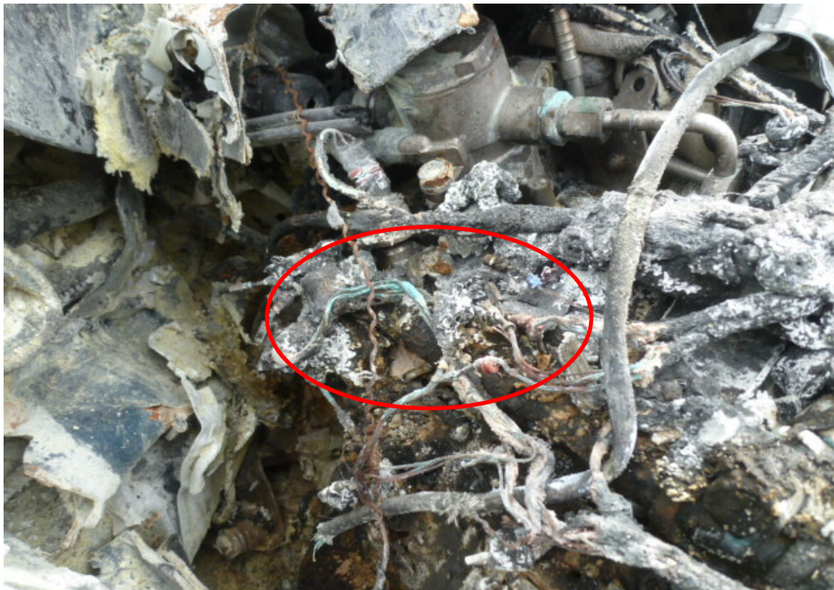
Photo 8 shows a closer view of the wirings with greenish residue found on some of the wirings around the rear centre portion of the engine compartment of the Insured Vehicle (circled). The presence of such greenish residue suggest occurrence of an electrical short circuit.
