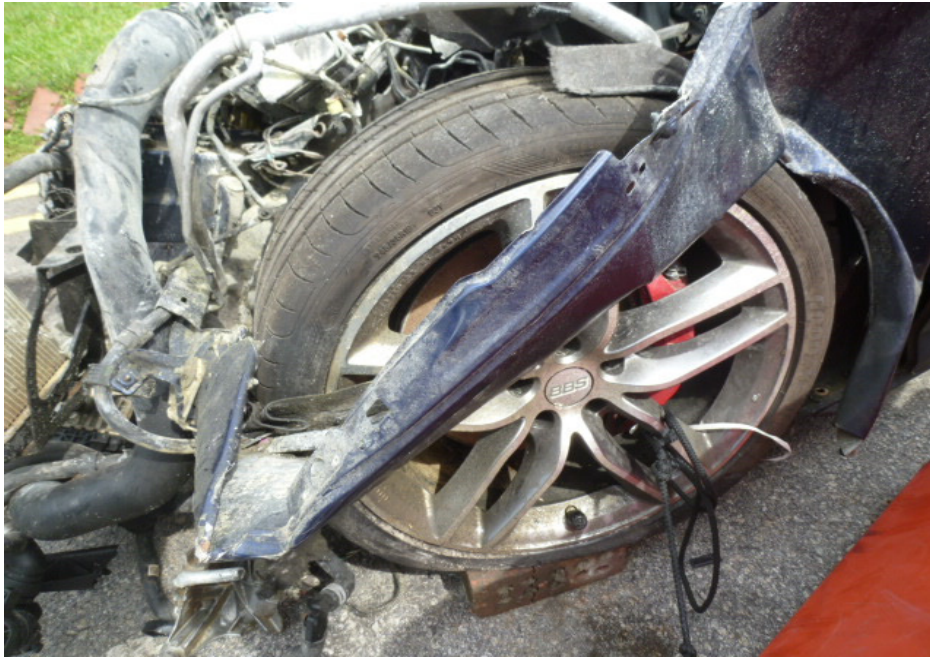
Photo 5 shows the non-standard rim found to be fitted on the Insured Vehicle at the time of our inspection. The 19- inch alloy rims fitted on the Insured Vehicle were not the standard type for the Insured Vehicle.
