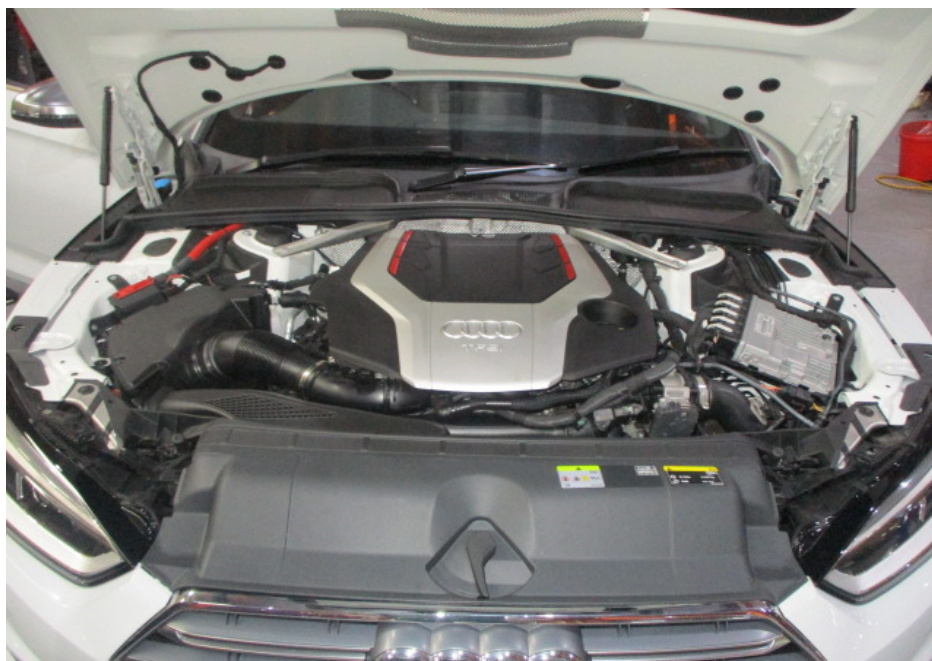
Photo 9 shows a general view of the engine compartment of the Motor Car at the time of my inspection. The various parts and components inside the engine compartment were all observed to be intact and properly fitted. There was also no sign(s) or indication(s) of fluid leak and/or fluid stain found inside the engine compartment.
