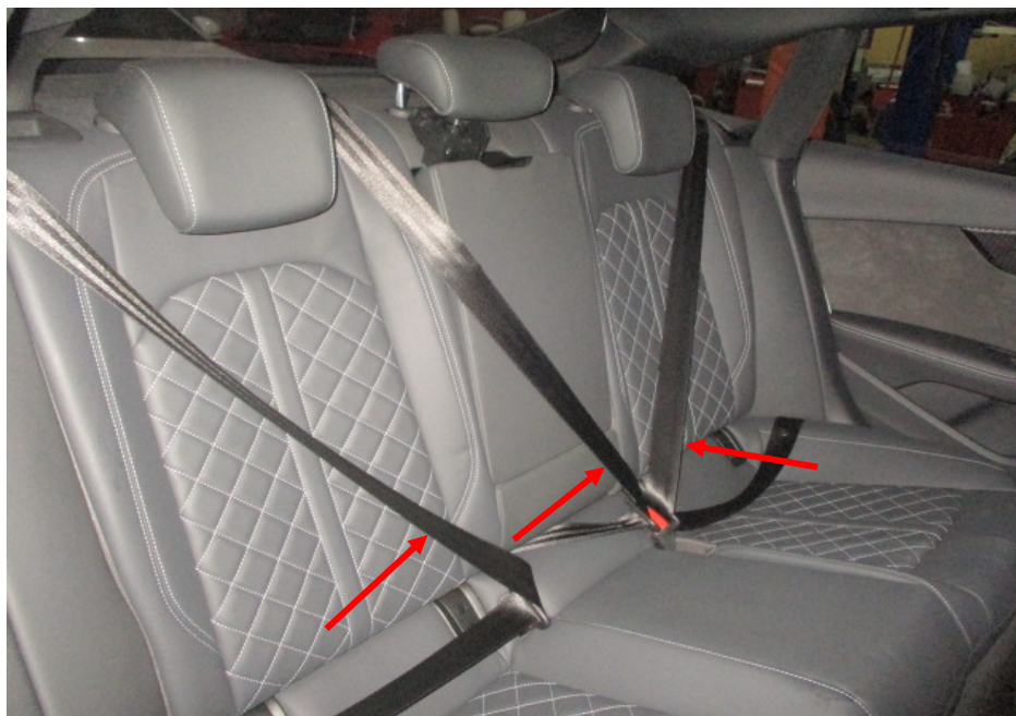
Photo 10 shows the rear seats of the Motor Car. All the seats of the Motor Car were secured via seat rails to the floorboard. They were also fitted with a retractable seat belt reel and a pre-tensioner. The seat belts (arrowed) were tested and were able to be fastened into the respective pre-tensions that were fitted on the side of each individual seat.
