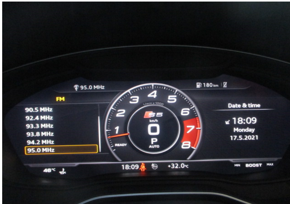
Photo 12 shows the respective warning lights no longer illuminated, indicating that there is no fault detected to the ABS, SRS, EPS, TPM and ESC systems of the Motor Car during the self-test. These electronic systems were hence in working condition at the time of my inspection.
