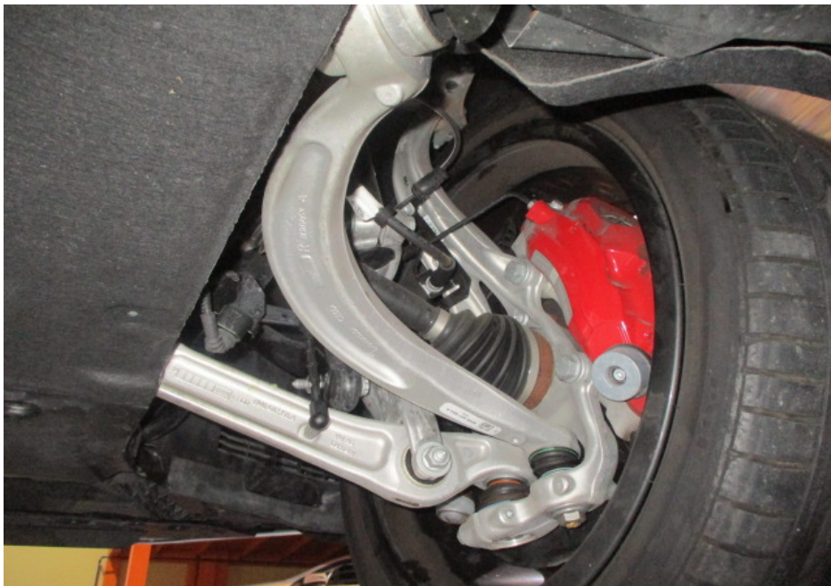
Photo 15 shows the various undercarriage components at the front right wheel of the Motor Car. The mechanical components, control arms and linkages were all found to be intact and secured in an appropriate manner.
