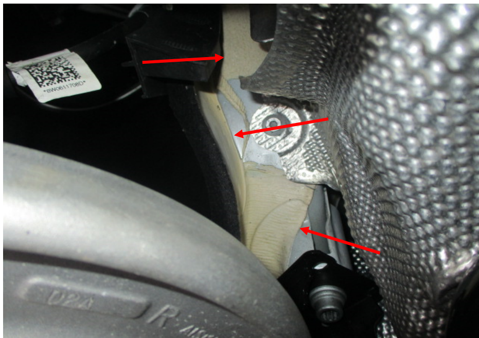
Photo 20 shows the chassis/structural body at the underside front right of the Motor Car. The original factory sealant (arrowed) at the joints along the chassis/structural body was observed to be untouched. In general, I had found no work was carried out on the chassis/structural body of the Motor Car. The chassis/structural body of the Motor Car was originally fitted.
