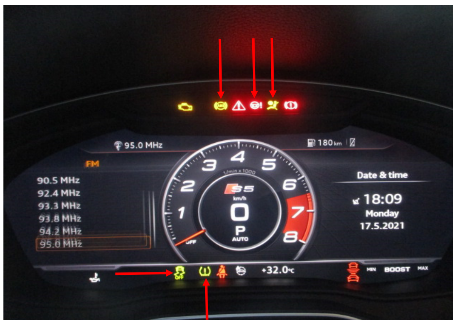
Photo 11 shows the warning lights for the various electronic safety features appearing on the instrument panel of the Motor Car during its self-test when the engine is cranked, in particular the ABS, SRS, EPS, TPM and ESC lights (arrowed).
