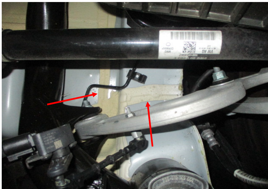
Photo 18 shows the chassis/structural body at the underside rear right of the Motor Car. I did not find any weld marks other than original spot weld marks on the chassis/structural body of the Motor Car. The original factory sealant (arrowed) at the joints along the chassis/structural body was untouched, indicating no work was done on the chassis/structural body of the Motor Car and that the chassis/structural body was originally fitted.
