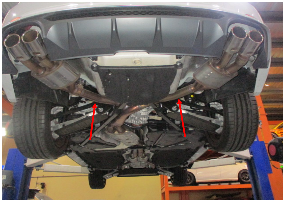
Photo 17 shows a general view of the Motor Car's exhaust system. My examination of the Motor Car's exhaust system revealed no sign(s) or indication(s) of any cut or weld marks along its exhaust pipes (arrowed), catalytic converters and on its rear mufflers.
