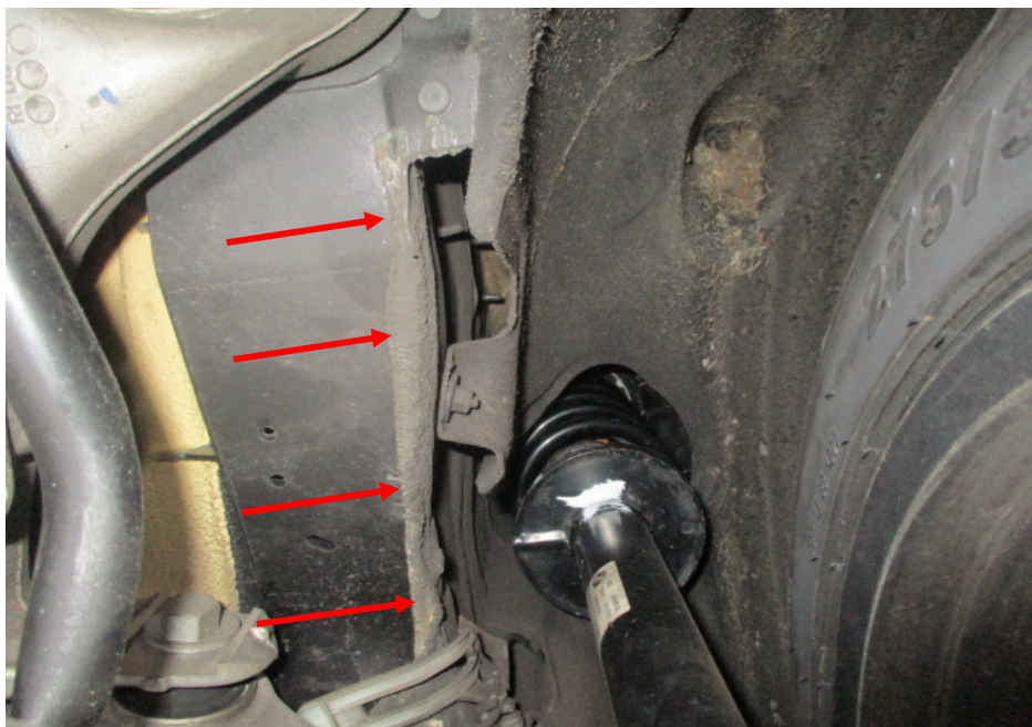
Photo 20 shows the chassis/structural body at the underside rear right of the Motor Car. I did not find any weld marks other than original spot weld marks on the chassis/structural body of the Motor Car. The original factory sealant (arrowed) at the joints along the chassis/structural body was untouched, indicating no work was done on the chassis/structural body of the Motor Car and that the chassis/structural body was originally fitted.
