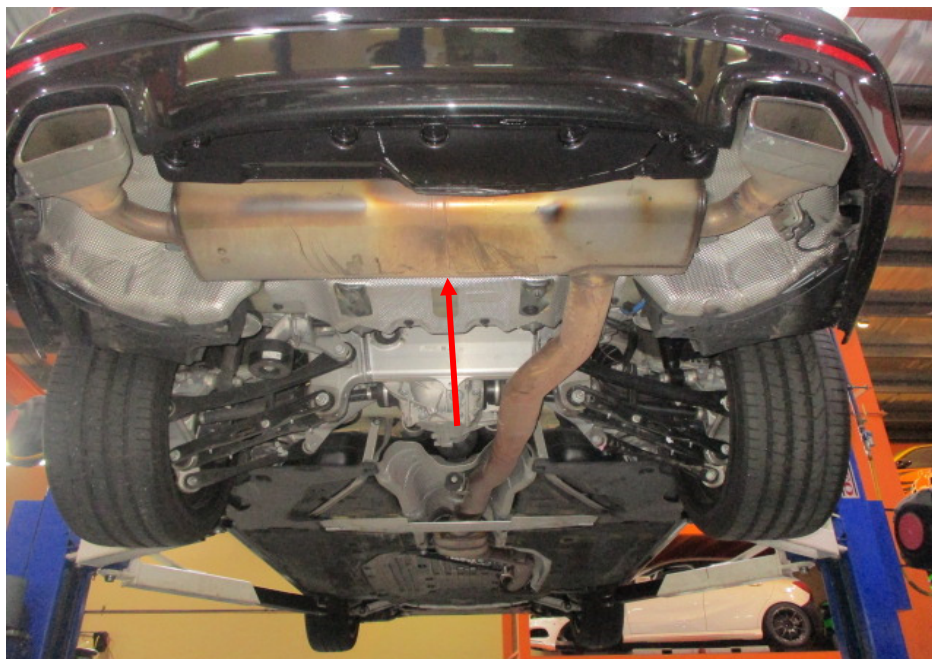
Photo 19 shows a general view of the Motor Car's exhaust system. My examination of the Motor Car's exhaust system revealed no sign(s) or indication(s) of any cut or weld marks along its catalytic converter, exhaust pipes and on its rear muffler (arrowed).
