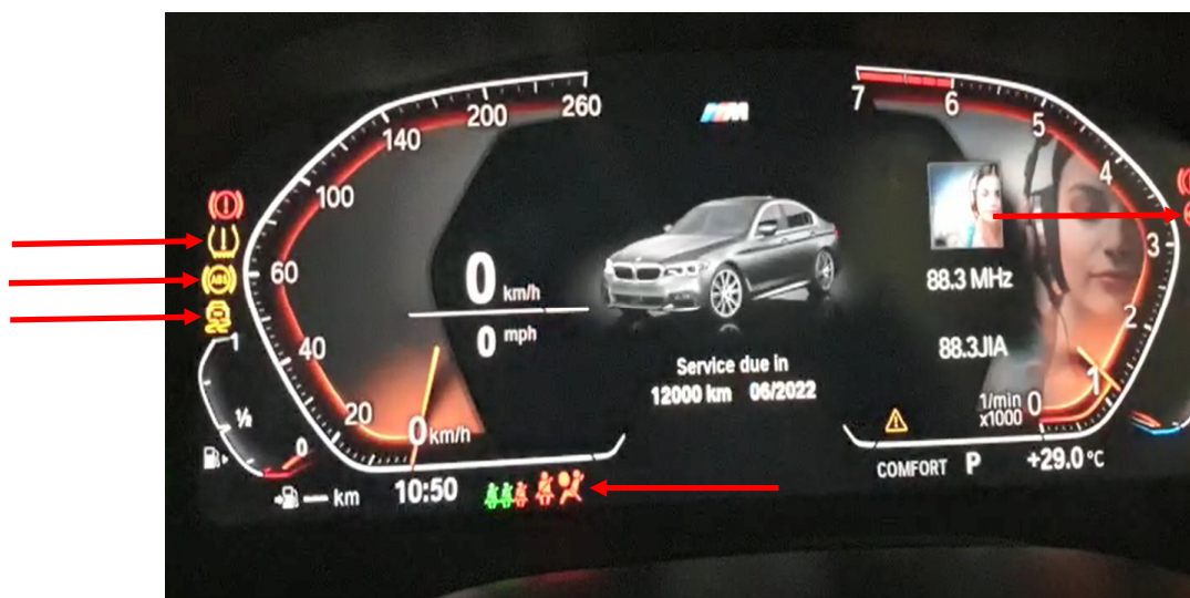
Photo 13 shows the warning lights for the various electronic safety features appearing on the instrument panel of the Motor Car during its self-test when the engine is cranked, in particular the ABS, SRS, IAS, TPM and DSC lights (arrowed).
