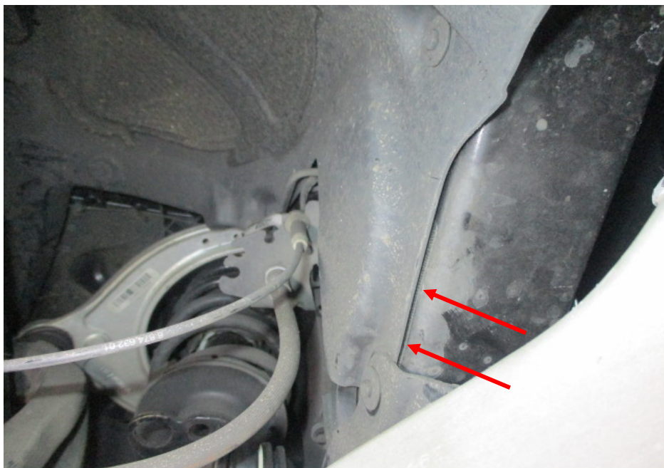
Photo 22 shows the chassis/structural body at the underside front right of the Motor Car. The original factory sealant (arrowed) at the joints along the chassis/structural body was observed to be untouched. In general, I had found no work was carried out on the chassis/structural body of the Motor Car. The chassis/structural body of the Motor Car was originally fitted.
