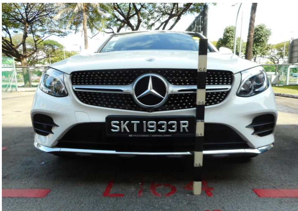
Photo 9 shows a general view of the height measurement being conducted on the front portion of Insured. The crack marks found on the front number plate holder was measured to be between 48cm to 53cm above ground level.
