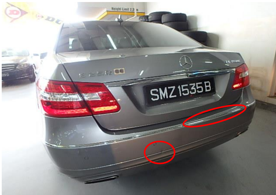
Photo 1 shows the general view of the rear portion of Third Party at the time of inspection. The rear bumper had been damaged. It was also noted that there were paint crack marks and dents (circled) on the rear bumper of Third Party.
