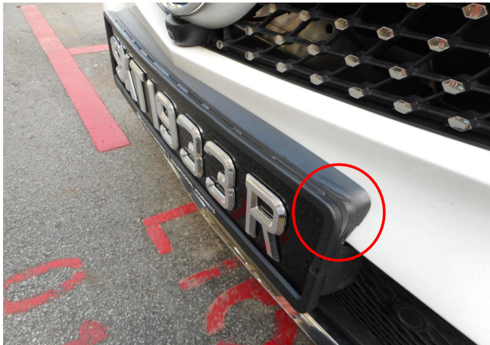
Photo 6 shows a close up view of the Insured front portion. We observed crack marks on the front number plate holder (circled).
