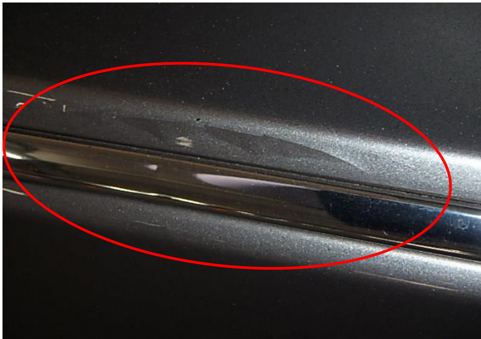
Photo 3 shows a close up view of the rear portion of the Third Party. We noted that there were paint crack marks on the rear bumper (circled).
