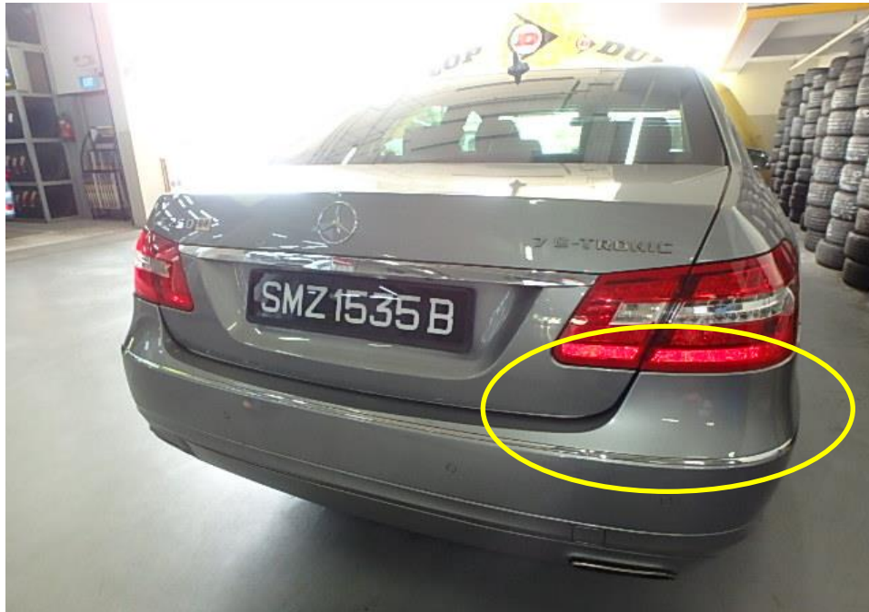
Photo 4 shows a close up view of the rear portion of the Third Party. We note that there was neither dislodgement nor misalignment of the rear bumper at the rear portion (circled) of Third Party.
