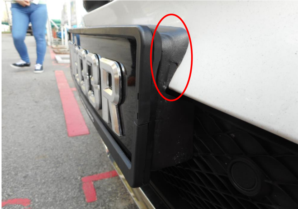
Photo 7 shows a close up view of the Insured front portion. We observed crack marks on the front number plate holder of the front bumper (circled).
