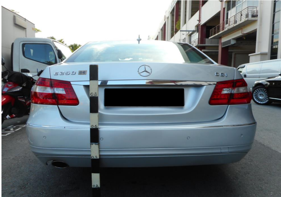
Photo 8 shows the general view of the height measurement being conducted on the rear portion of Third Party. The height above ground level of where the damages were found to the rear bumper of the Third Party was at 58cm and 46cm.
