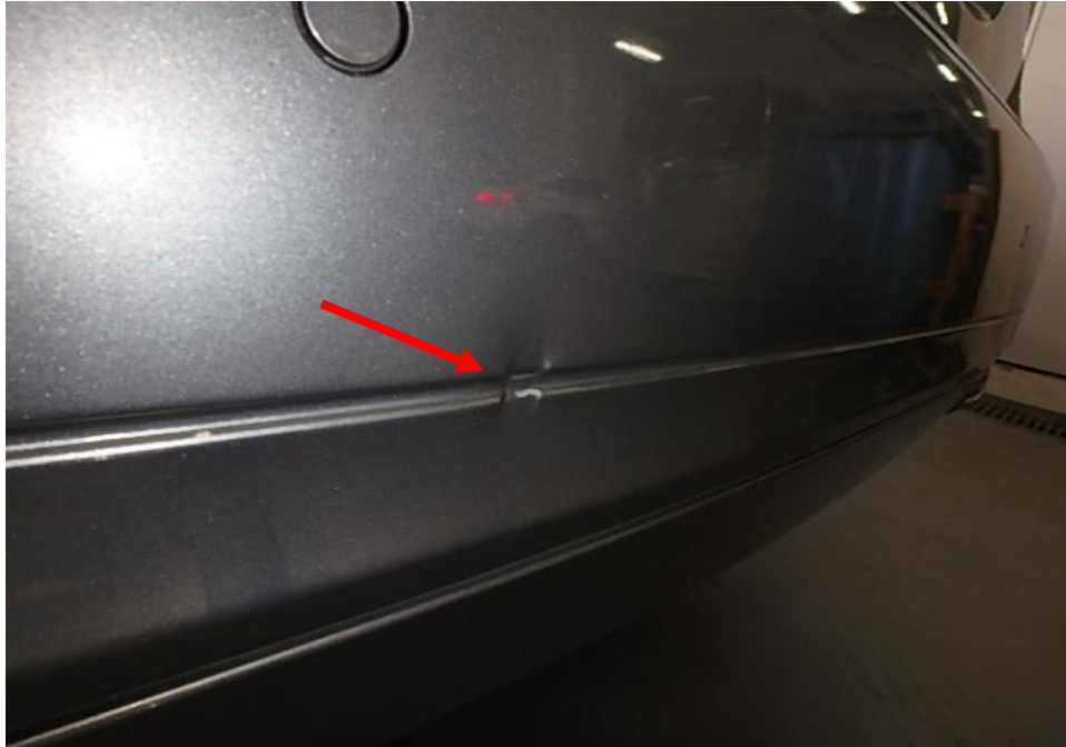
Photo 2 shows a close up view of the rear portion of the Third Party. We noted that there were dent marks on the rear bumper (arrowed).
