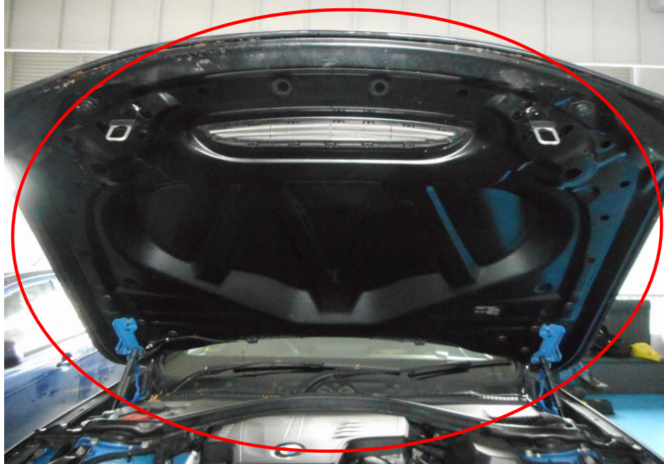
Photo 10 shows an aftermarket bonnet (circled) on the Insured Vehicle, which was observed to be unaffected by the fire.
