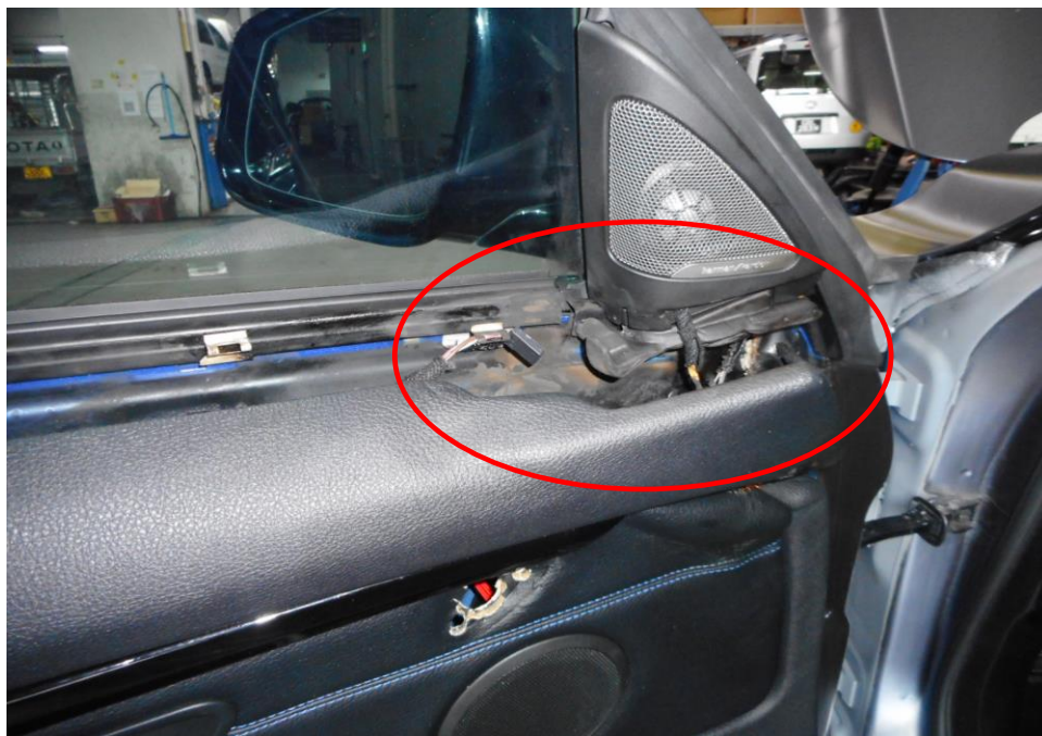
Photo 8 shows the close up view of the front left interior door panel of the Insured Vehicle at the time of our inspection. The door panel had suffered heat and smoke damages (circled) as a result of the fire.
