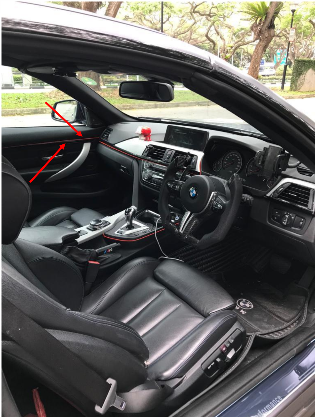
Photo 28 shows additional LED light strips that was already fitted at the front left door panel (arrowed) of the Insured Vehicle at the material time.
