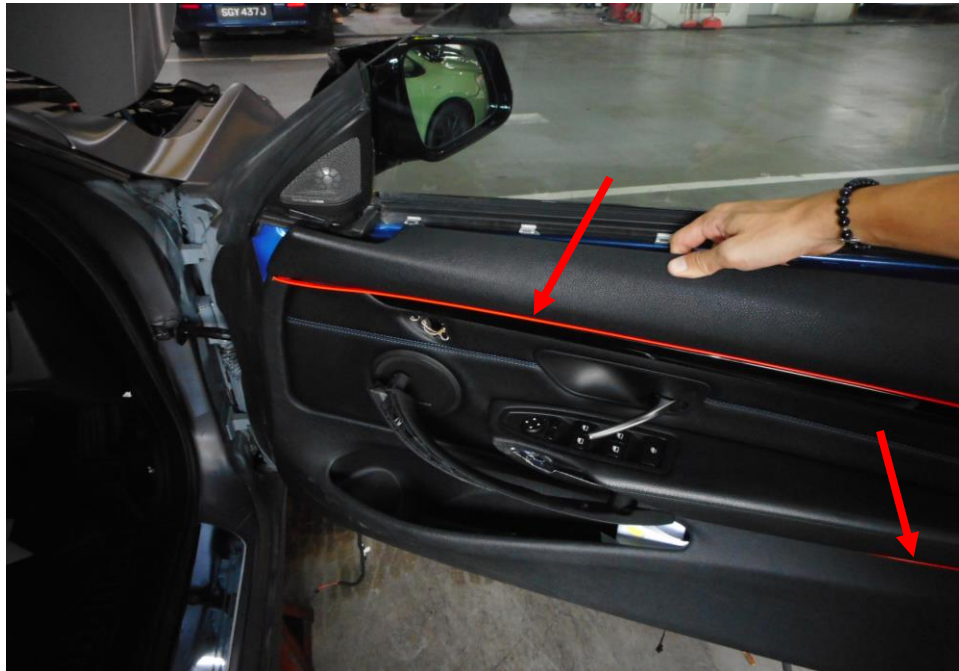
Photo 18 shows the right side door panel general view of the additionally fitted LED light strips wiring harness installed on the door panel (arrowed). These components were not affected by the fire. These wirings and electrical components were not original wirings fitted from manufacturer.
