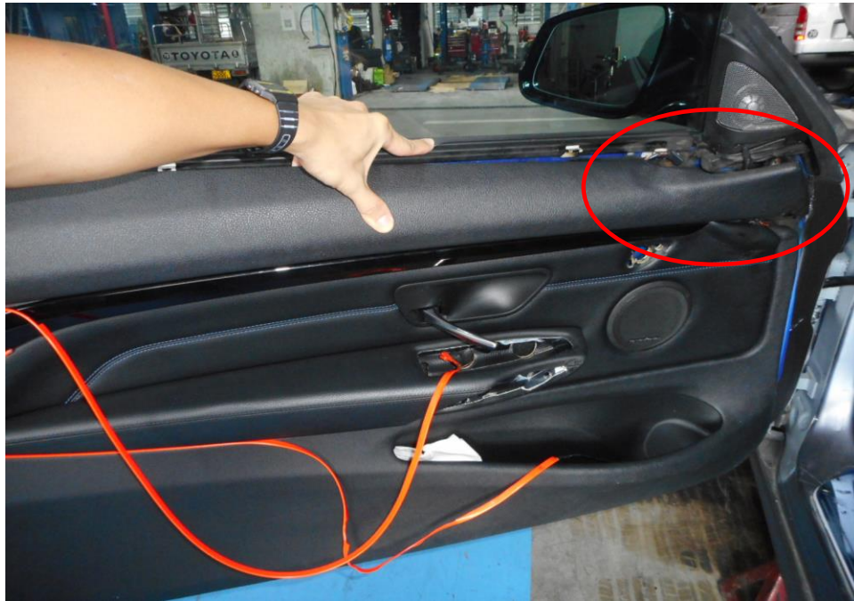
Photo 7 shows the general view of the front left interior door panel of the Insured Vehicle at the time of our inspection. The door panel had suffered heat and smoke damages (circled) as a result of the fire.
