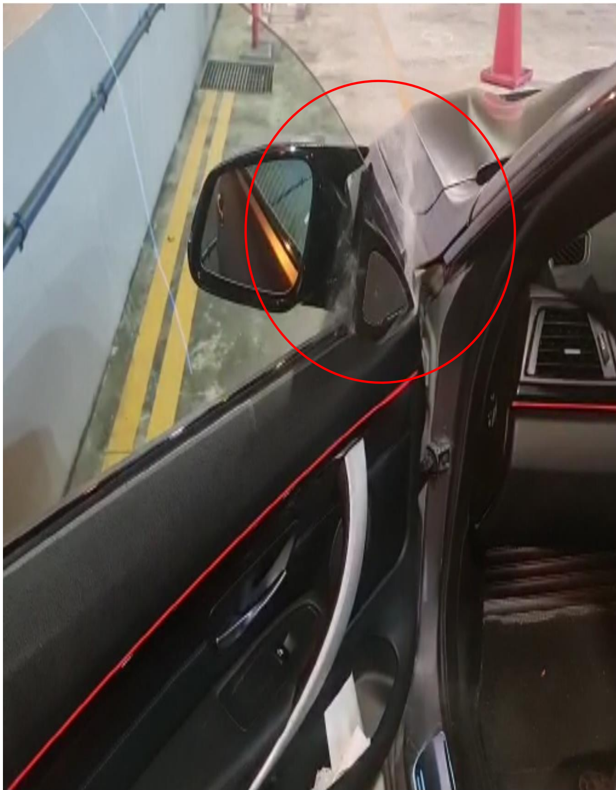
Photo 36 shows the front left door panel, where the fire had started on Insured Vehicle. Observed is smoke emitting out of the front left door panel (circled). In general, the information that could be gathered from this photograph had corresponded to the events that were related to us by Mr Harrison, location when the fire broke out.
