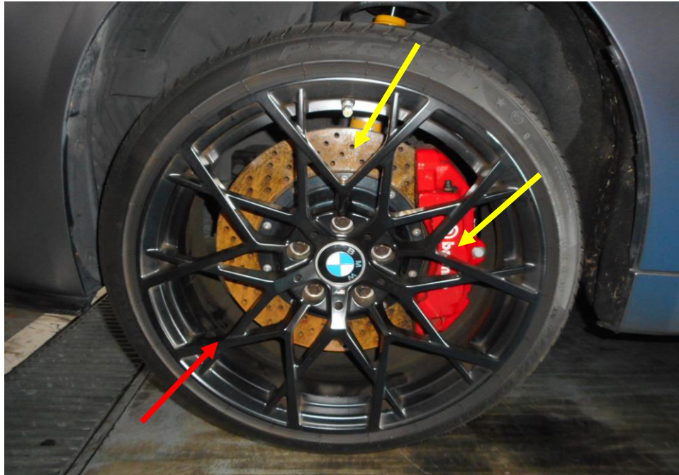
Photo 12 shows an aftermarket rim (red arrow) and upgraded brake caplier and disc brake (yellow arrow) on the Insured Vehicle, which was observed to be unaffected by the fire.
