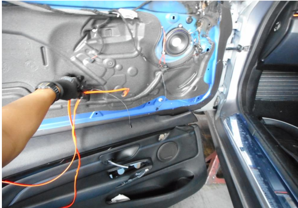
Photo 15 shows the general inside view of the front left door panel of the Insured Vehicle at the time of our inspection. Observed that the electrical components around then surrounding had sustain heat & smoke damage.
