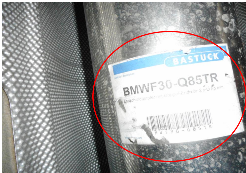
Photo 14 shows a set of aftermarket exhaust system (circled) on the Insured Vehicle, which was observed to be unaffected by the fire.
