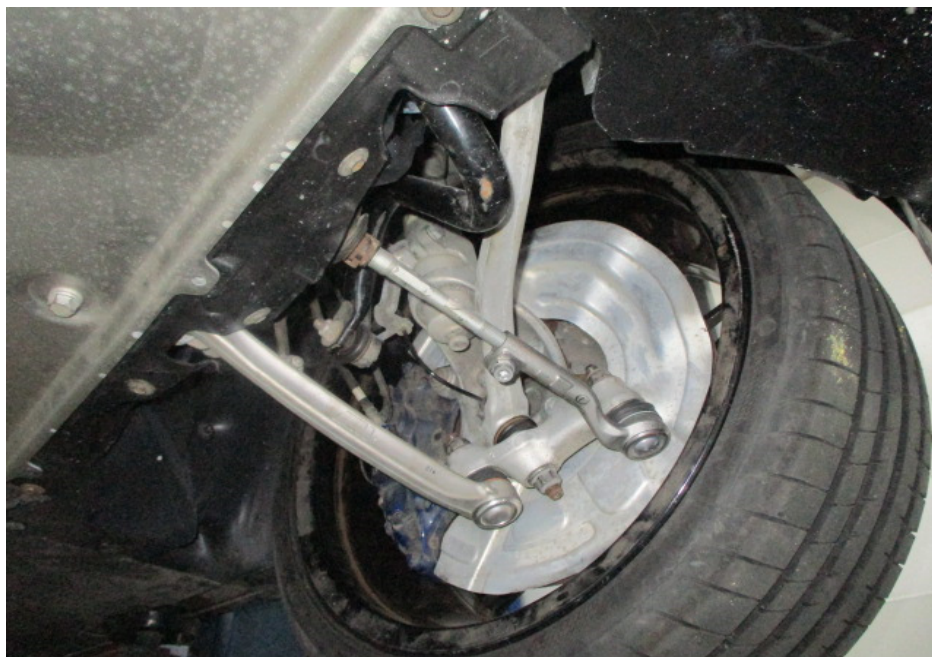
Photo 16 shows the various undercarriage components at the front left wheel of the Motor Car. The mechanical components, control arms and linkages were all found to be intact and secured in an appropriate manner.
