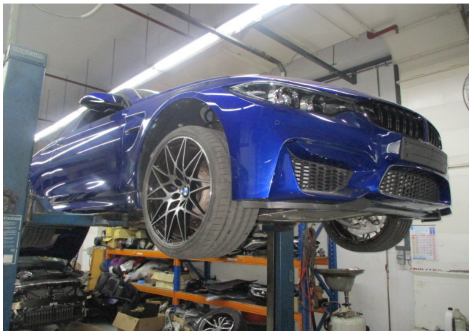
Photo 14 shows the Motor Car hoisted up for checks on its undercarriage. There was no sign(s) or indication(s) of fluid leakage and/or fluid stain(s) on the underside of the Motor Car. The undercarriage components of the Motor Car were also all observed to be intact and secured in an appropriate manner.
