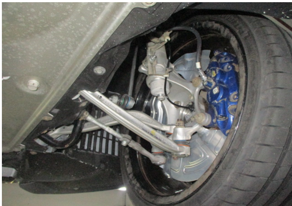
Photo 15 shows the various undercarriage components at the front right wheel of the Motor Car. The mechanical components, control arms and linkages were all found to be intact and secured in an appropriate manner. I also did not observe any fluid leak and/or fluid stain on the underside of the Motor Car.
