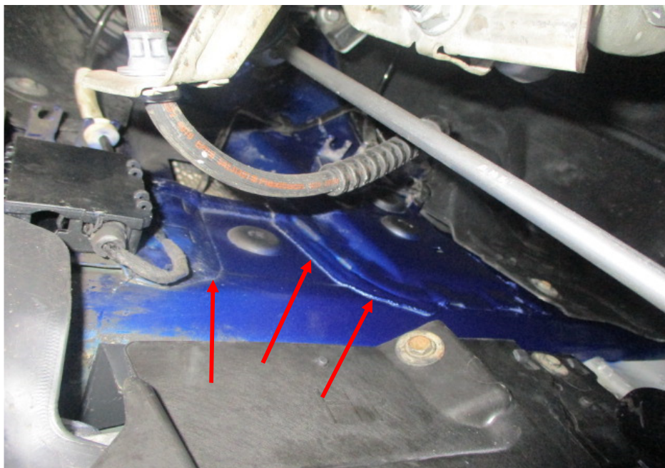
Photo 21 shows the chassis/structural body at the underside front right of the Motor Car. The original factory sealant (arrowed) at the joints along the chassis/structural body was observed to be untouched. In general, I had found no work was carried out on the chassis/structural body of the Motor Car. The chassis/structural body of the Motor Ca was originally fitted.
