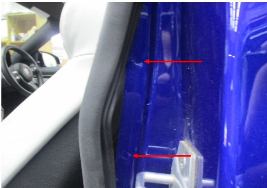
Photo 24 shows the left side rear body panel of the Motor Car. I did not find any weld marks other than original spot weld marks (arrowed) on the left side rear body panel of the Motor Car which, indicates that there was no re-welding works carried out. In general, I had found all the non-detachable body panels of the Motor Car to be originally fitted at the time of my inspection.
