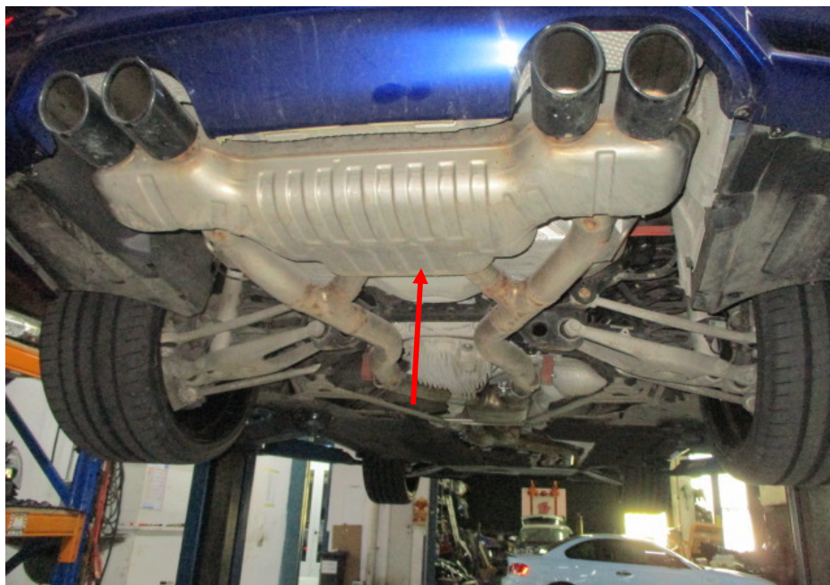
Photo 18 shows the Motor Car's rear muffler (arrowed). My examination of the Motor Car's exhaust system revealed no sign(s) or indication(s) of any cut or weld marks along its exhaust pipes and on its catalytic converters.
