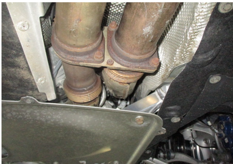
Photo 19 shows the Motor Car's catalytic converters. My examination of the Motor Car's exhaust system revealed no sign(s) or indication(s) of any cut or weld marks along its exhaust pipes and on its rear muffler.
