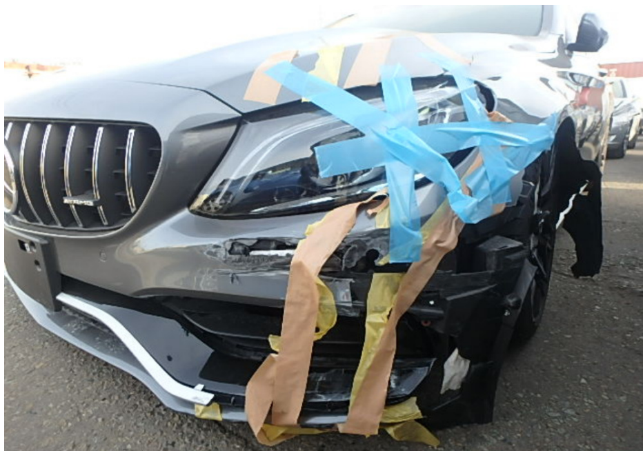
Photo 2 shows a closer view of the damage at the front left portion of the Motor Car (photograph provided to me). The front bumper, front bumper left lower grille, front bumper left lower grille garnish, front bumper lower lip, front left headlamp, front left fender and front left fender inner shield were amongst the parts that were observed to have been damaged.
