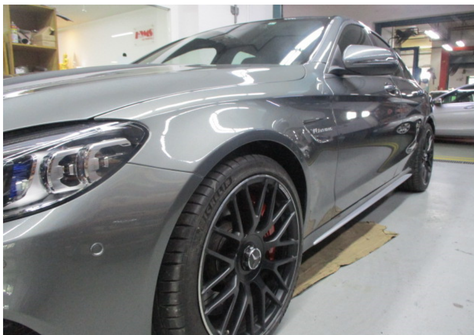
Photo 9 shows a closer view of the front bumper, front bonnet, front left fender and front left wheel rim of the Motor Car at the time of my inspection. The body parts at the front left portion of the Motor Car were visually examined and it was observed that the repair/restoration works carried out to the damaged area of the Motor Car (refer to photograph 1 & 2 above) were reasonably adequate and in order.
