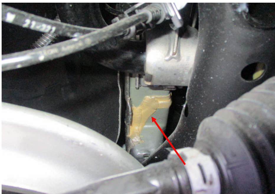
Photo 23 shows the chassis/structural body at the underside front right of the Motor Car. The original factory sealant (arrowed) at the joints along the chassis/structural body was observed to be untouched. In general, I had found no work was carried out on the chassis/structural body of the Motor Car. The chassis/structural body of the Motor Ca was originally fitted.
