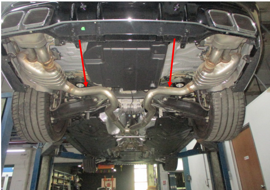
Photo 21 shows the Motor Car's exhaust system. My examination of the Motor Car's exhaust system revealed no sign(s) or indication(s) of any cut or weld marks along its exhaust pipes (arrowed), rear mufflers and on its catalytic converters.
