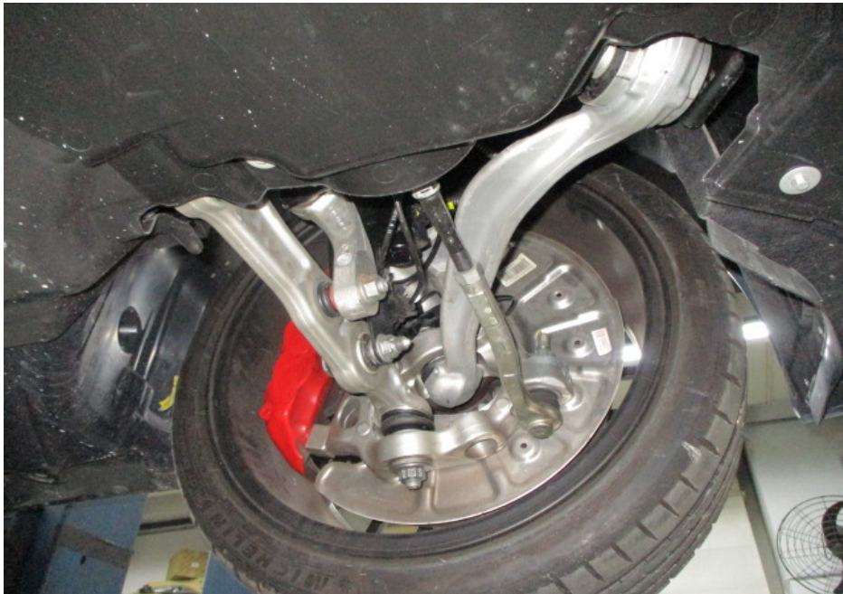
Photo 20 shows the various undercarriage components at the front left wheel of the Motor Car. The mechanical components, control arms and linkages were all found to be intact and secured in an appropriate manner. I also did not observe any fluid leak and/or fluid stain on the underside of the Motor Car.
