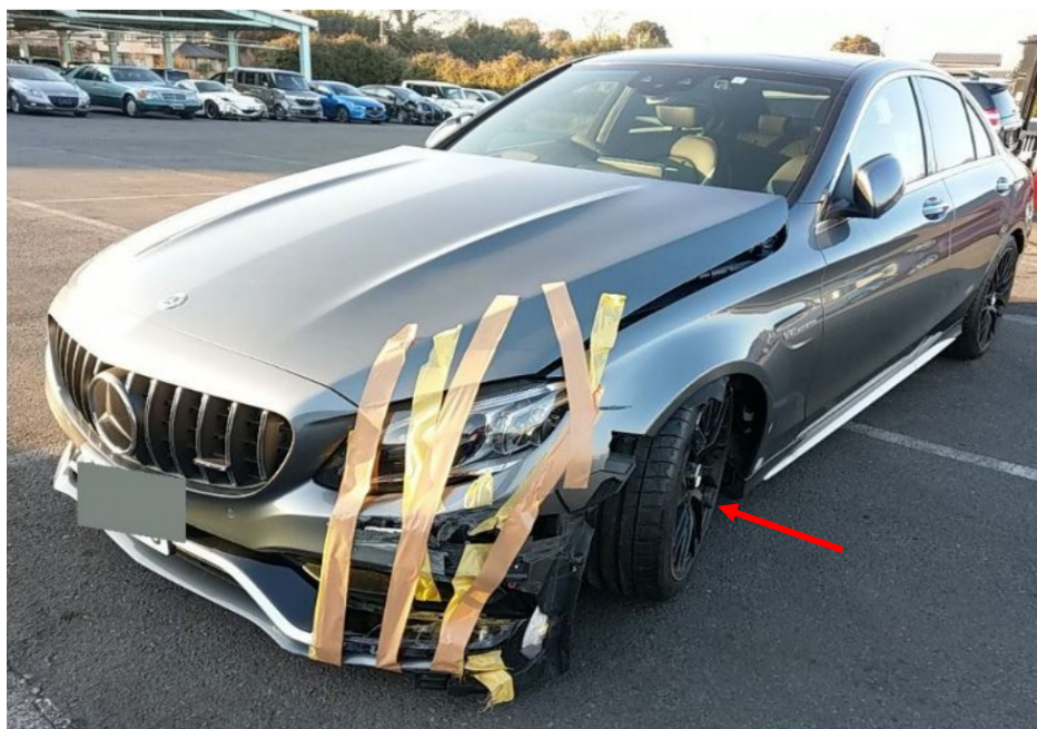
Photo 1 shows the front left body of the Motor Car (photograph provided to me). The Motor Car was observed to have sustained damage at its front left portion. The front bumper, front left headlamp and front bonnet were amongst the parts that were observed to have been damaged. The orientation of the front right wheel (refer to photograph 3 below) and front left wheel (arrowed) indicates to me that there was damage to the front left undercarriage parts of the Motor Car.
