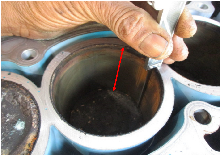
Photo 17 shows measurement being carried out to the stroke (arrowed) of cylinder 3 of the Toyota engine. The bore and stroke measurements of the Toyota engine were carried out using a digital Vernier Caliper that was calibrated before the start of measurements.
