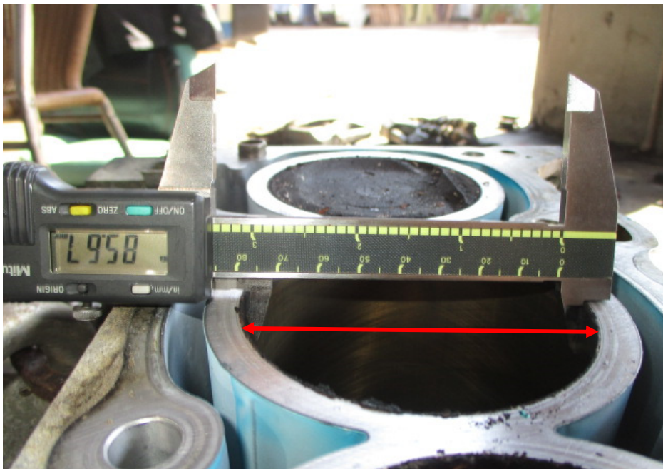
Photo 12 shows measurement being carried out to the bore (arrowed) of cylinder 2 of the Toyota engine. The bore measurement of cylinder 2 was recorded to be 85.67mm.
