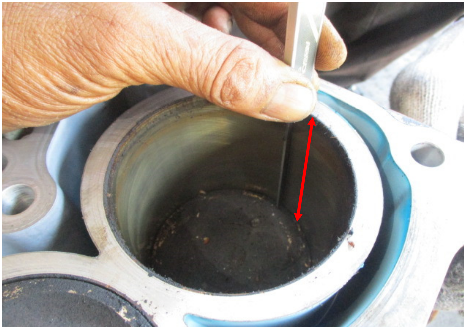
Photo 10 shows measurement being carried out to the stroke (arrowed) of cylinder 1 of the Toyota engine. The bore and stroke measurements of the Toyota engine were carried out using a digital Vernier Caliper that was calibrated before the start of the measurements,
