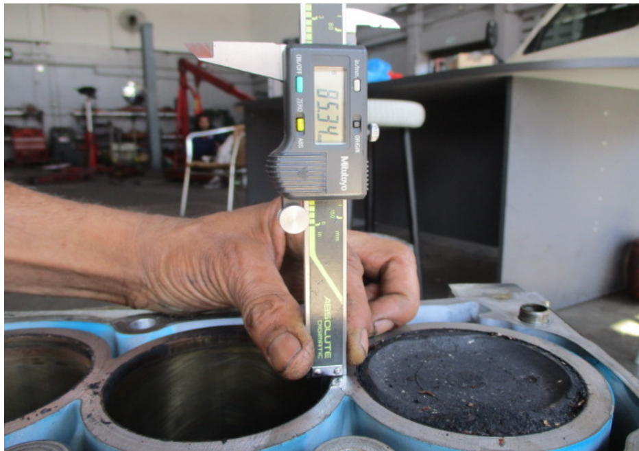
Photo 15 shows the stroke measurement of cylinder 2, which was recorded to be 85.34mm.
