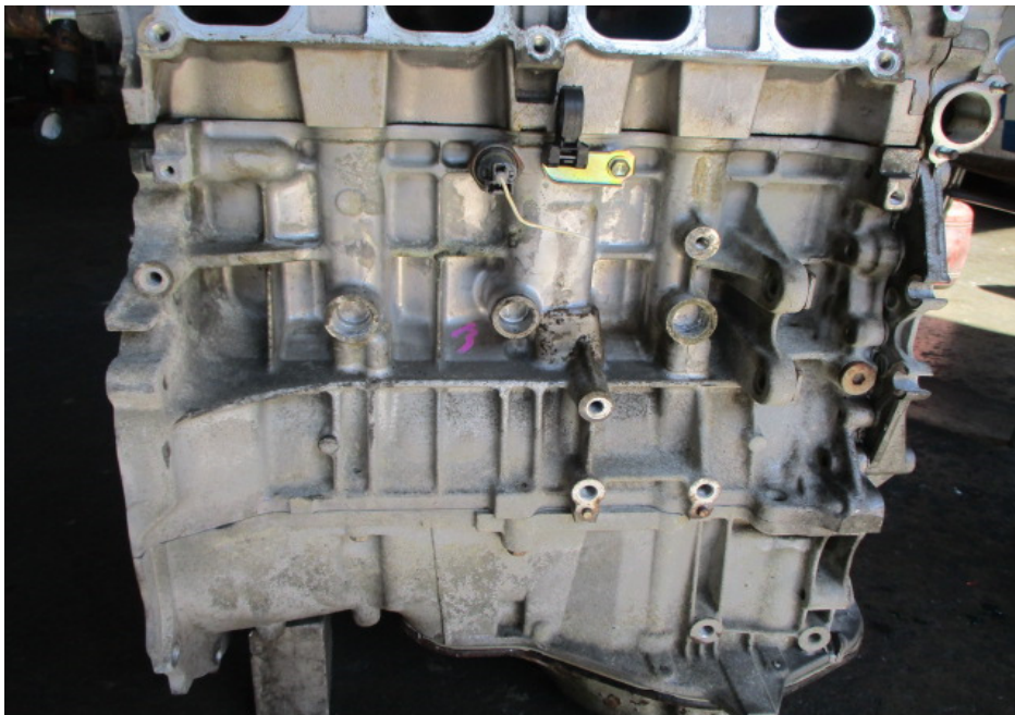
Photo 2 shows a closer view of the Toyota engine that I had inspected. My visual examination of the engine housing revealed the housing to be of serviceable/satisfactory condition. There was no crack and/or hole observed on the engine housing.
