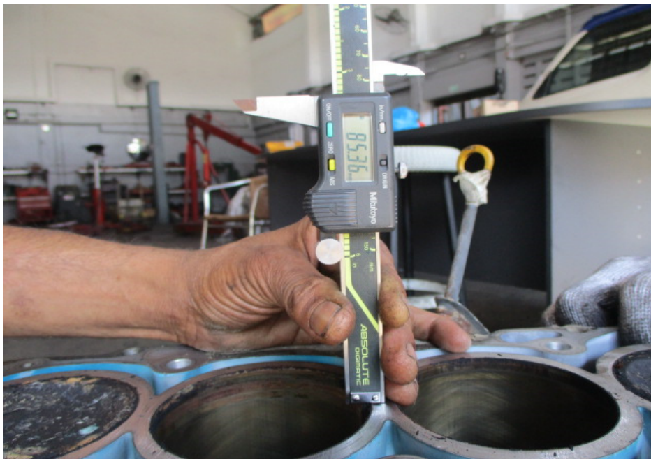
Photo 18 shows the stroke measurement of cylinder 3, which was recorded to be 85.36mm.
