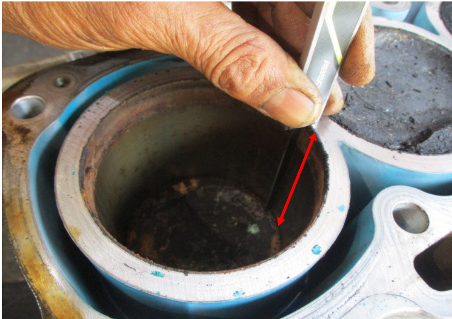
Photo 21 shows measurement being carried out to the stroke (arrowed) of cylinder 4 of the Toyota engine. The bore and stroke measurements of the Toyota engine were carried out using a digital Vernier Caliper that was calibrated prior to the start of measurements.
