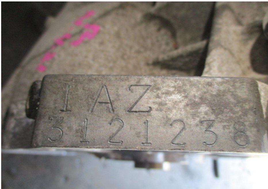
Photo 4 shows the engine number engraved on the housing of the Toyota engine that I had inspected. The engine number was 1AZ3121238.
