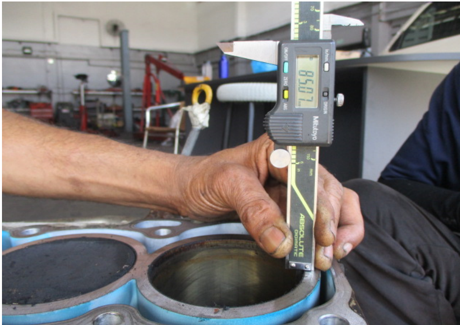
Photo 11 shows the stroke measurement of cylinder 1, which was recorded to be 85.07mm.
