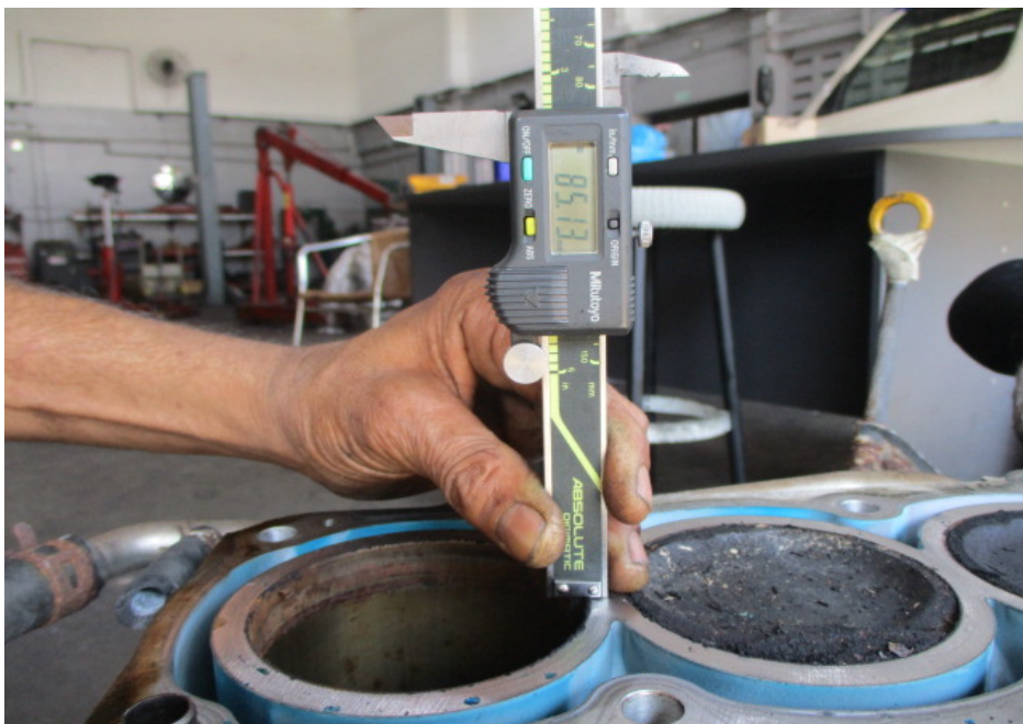
Photo 22 shows the stroke measurement of cylinder 4, which was recorded to be 85.13mm.
