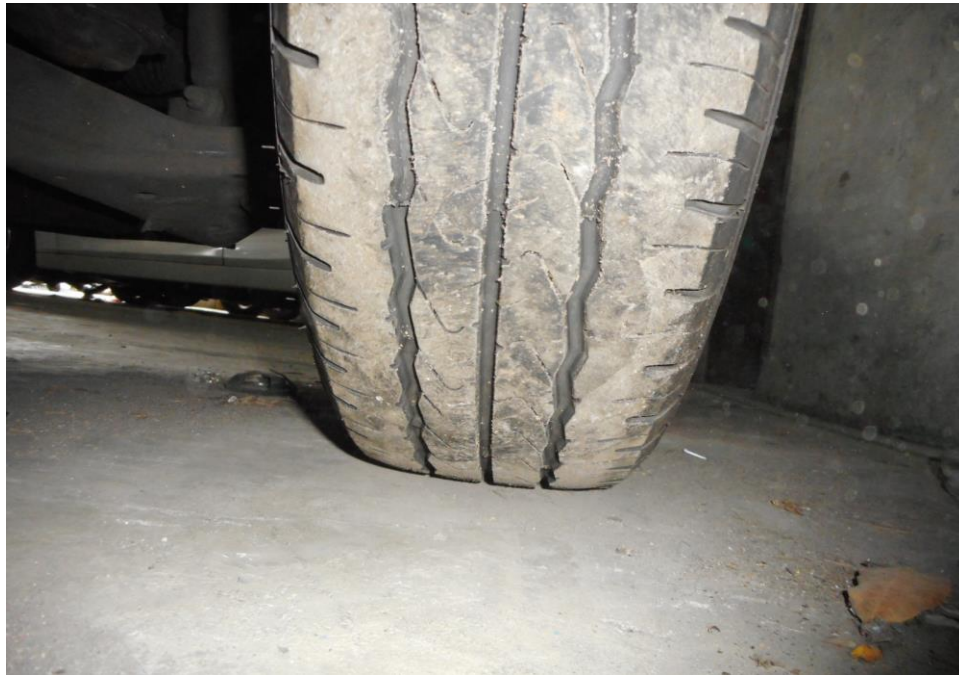
Photo 7 shows the condition of the front right tyre of the Tow-Truck, which was observed to be in serviceable condition with remaining tread depth of approximately 7.2mm. The tyre, which was wrapped around standard steel wheel rim, was also observed to be sufficiently inflated for vehicular operation. There was no tear, cut or burst mark(s) on the outer and the inner sidewalls as well as across the tread of the 4 tyres that were fitted on the Tow-Truck.
