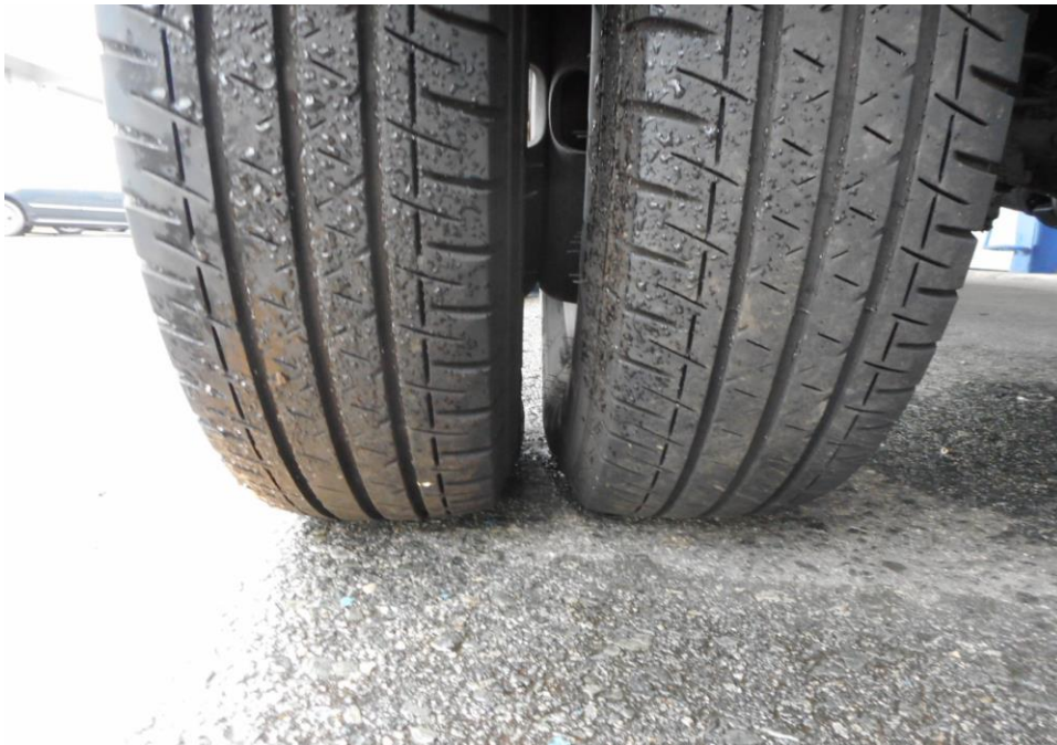
Photo 9 shows the condition of the rear left tyres of the Tow-Truck, which was observed to be in serviceable condition with remaining tread depth of approximately 5.5mm. The tyres, which were wrapped around standard steel wheel rim, were also observed to be sufficiently inflated for vehicular operation. There was also no damage found on all 4 steel wheel rims of the Tow-Truck.
