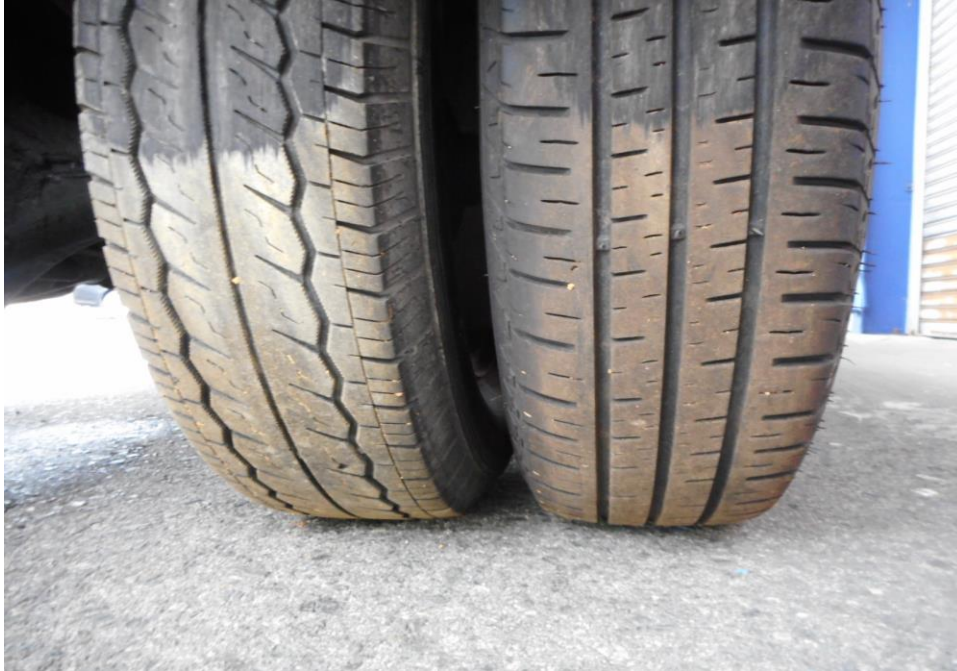
Photo 8 shows the condition of the rear right tyre of the Tow-Truck, which was observed to be in serviceable condition with remaining tread depth of approximately 4.5mm. The tyre, which was wrapped around standard steel wheel rim, it was observed to be sufficiently inflated for vehicular operation.
