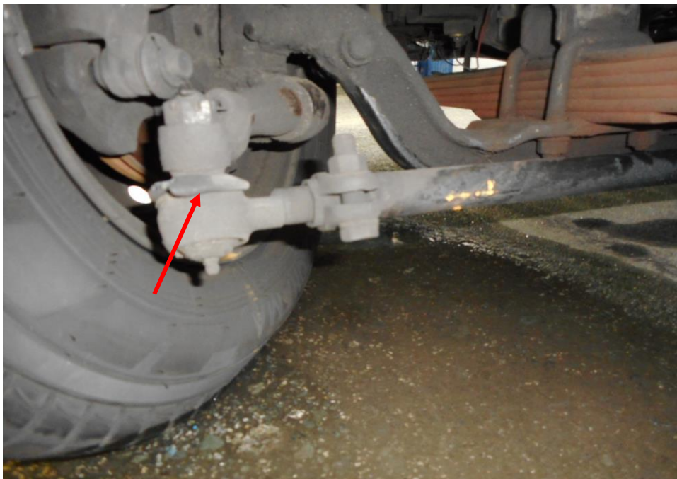
Photo 17 shows the various undercarriage components at the front left wheel of the Tow-Truck, in particular the steering tie rod end (arrowed). The various undercarriage components of the Tow-Truck were all found to be intact without any visible damage. There was also no sign of fluid stain(s) observed on the various undercarriage components.
