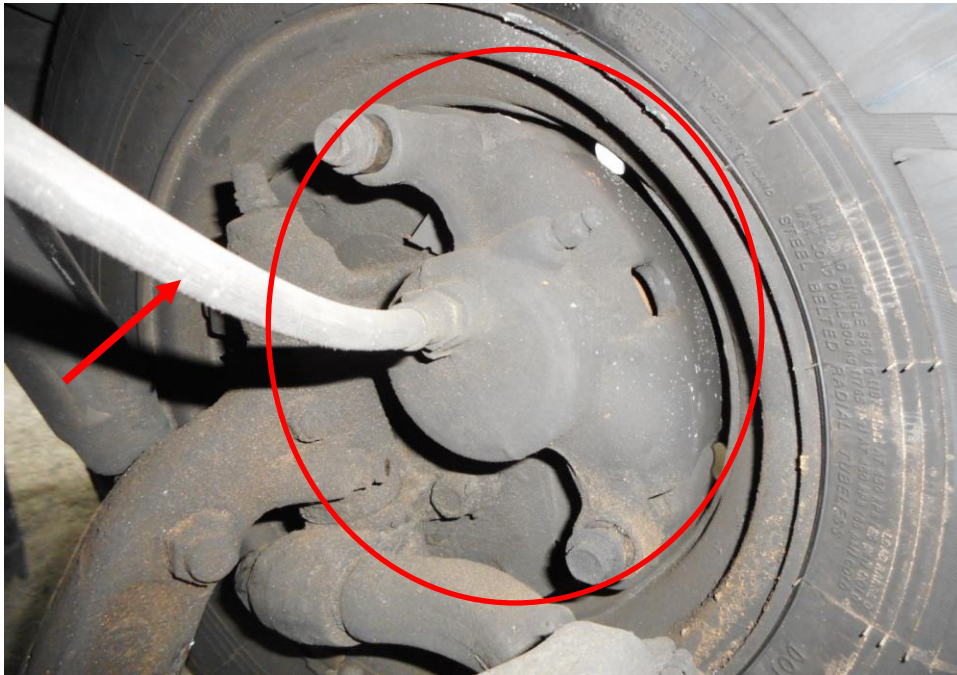
Photo 20 shows the brake hose/pipe (arrowed) at the front right wheel of the Tow-Truck. No leakage of brake fluid was observed. Visual examination of the various components of the braking system like the brake caliper (circled), brake booster, brake pedal etc had revealed all to be intact and without visible damage at the time of accident. There was also no sign of fluid stain(s) observed on the various undercarriage components.
