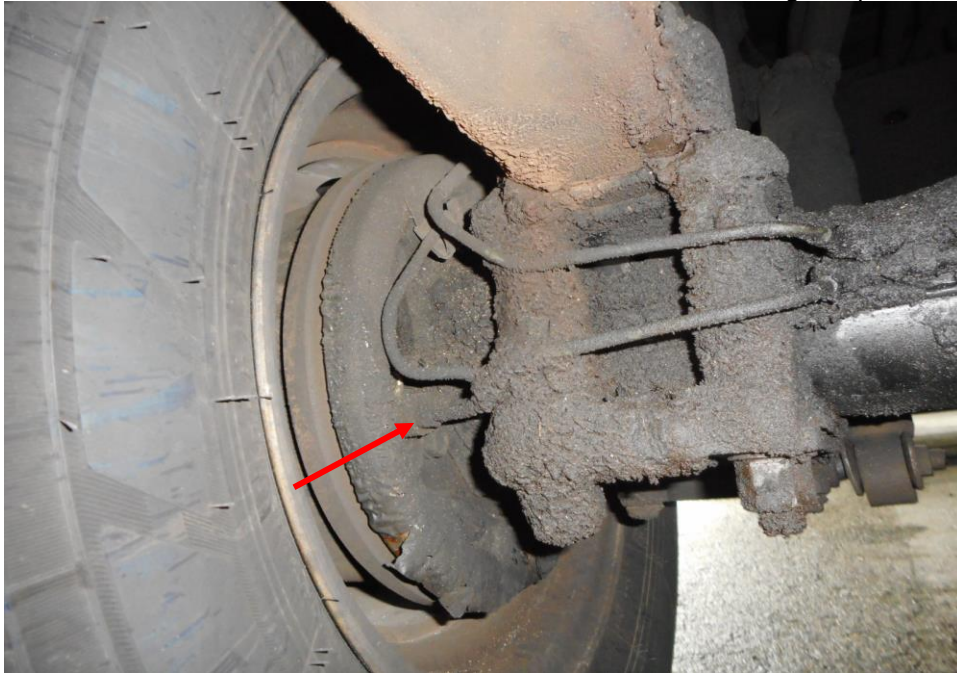
Photo 19 shows the brake pipe (arrowed) at the rear left wheel of the Tow-Truck. I did not observe any leakage of brake fluid at the time of my inspection of the Tow-Truck. However, we observed old fluid stain on the braking components.
