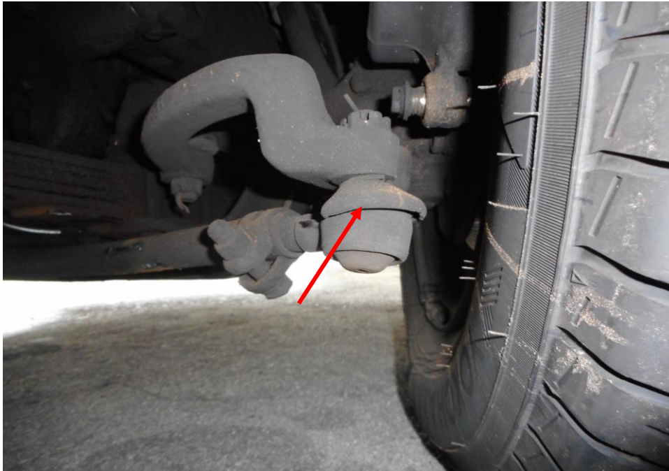
Photo 16 shows the various undercarriage components at the front right wheel of the Tow-Truck, in particular the steering tie rod end (arrowed). The various steering components were all found to be intact, suggesting that the steering system of the Tow-Truck was likely to be in serviceable condition at the material time of accident. There was also no sign of fluid stain(s) observed on the various undercarriage components.
