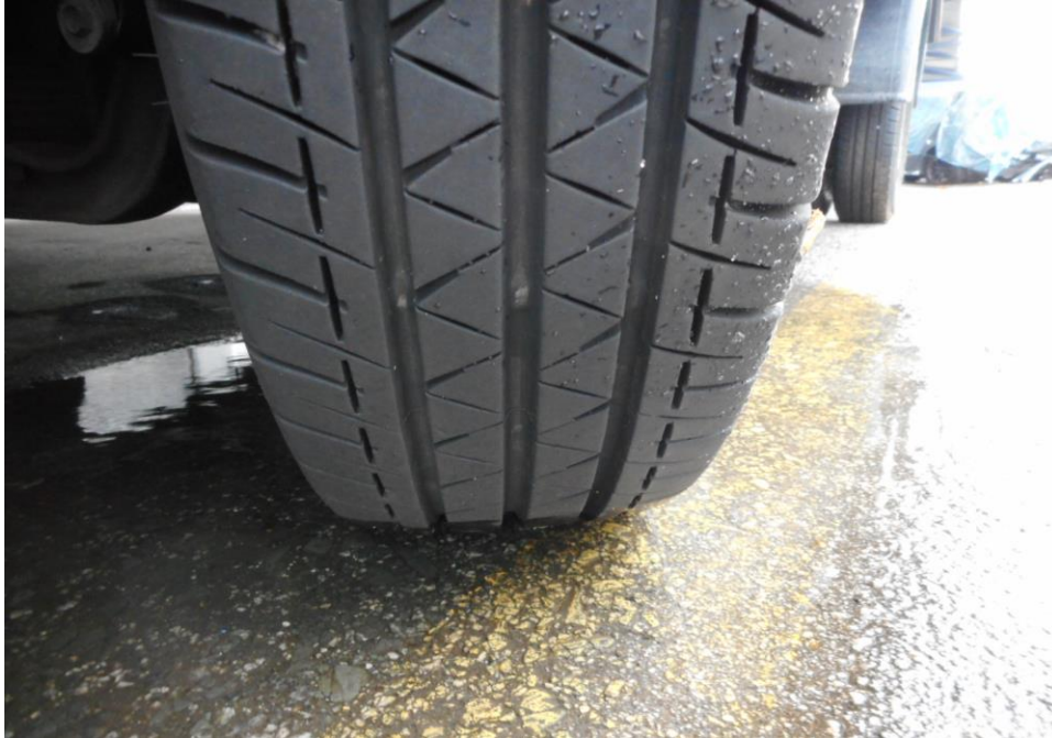
Photo 10 shows the condition of the rear right tyres of the Tow-Truck, which were observed to be in serviceable condition with remaining, tread depth of approximately 7.7mm. There was also no tear, cut or burst mark(s) on the outer and the inner sidewalls as well as across the tread of the 4 tyres that were fitted on the Tow-Truck.
