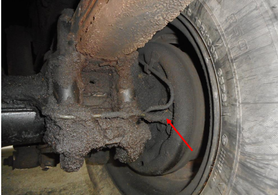
Photo 18 shows the brake pipe (arrowed) at the rear right wheel of the Tow-Truck. I did not observe any leakage of brake fluid at the time of my inspection of the Tow-Truck. However, we observed old fluid stain on the braking components.
