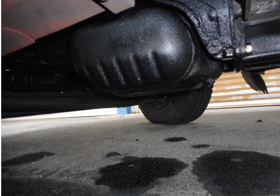
Photo 15 shows the undercarriage of the Tow-Truck, at the area where the engine housing and transmission housing are located. I observed sign(s) of fluid leakage on the ground and old fluid stain(s) on the underside of the Tow-Truck.
