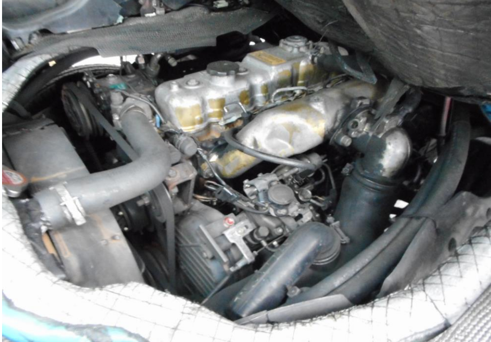
Photo 11 shows a general view of the Tow-Truck's engine compartment, which was accessed by lifting the front cabin of the Tow-Truck. The various parts and components inside the engine compartment were unaffected by the accident. There was also no sign(s) or indication(s) of fresh fluid leakage and/or fluid stain within the engine compartment
