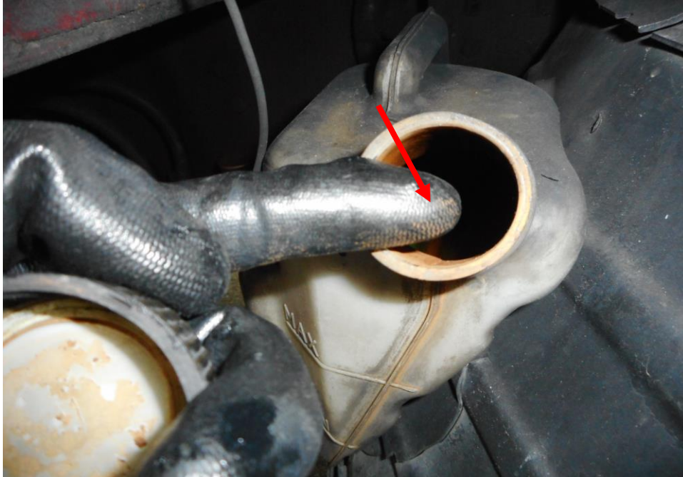
Photo 13 shows the engine coolant reservoir of the Tow-Truck at the time of my inspection. The engine coolant was observed to be of insufficient level (arrowed).
