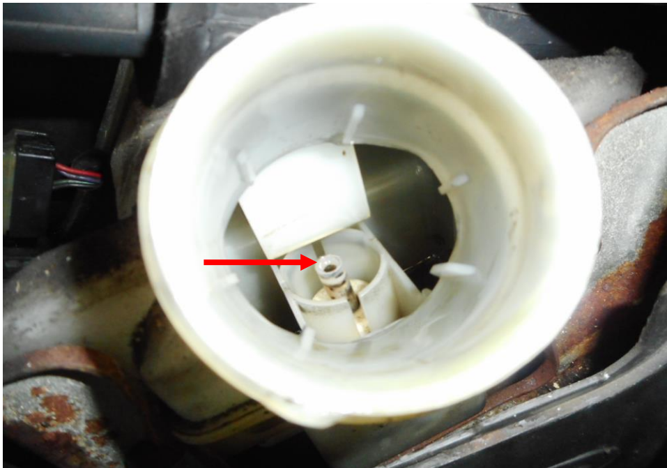
Photo 12 shows the brake fluid reservoir of the Tow-Truck at the time of my inspection. The brake fluid was observed to be of insufficient level (arrowed).
