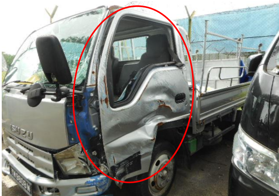
Photo 5 shows a close up view of the Motor Lorry's front portion at the time of my inspection. Its front left door (circled) was damage at the time of my inspection as a result of the accident.
