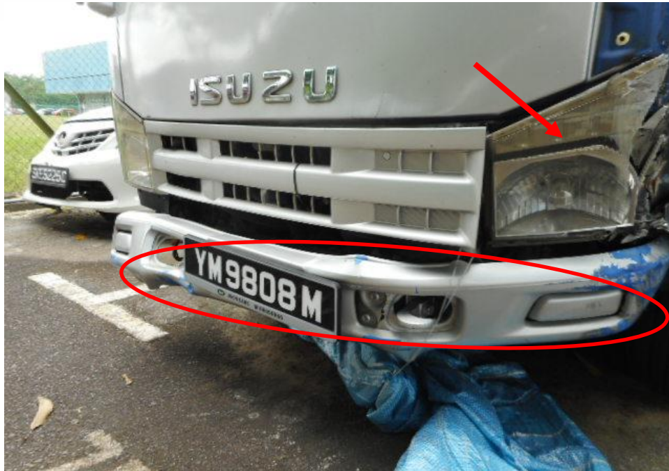
Photo 4 shows a close up view of the Motor Lorry's front portion at the time of my inspection. Its front bumper (circled) and front left headlamp (arrowed) was damage at the time of my inspection as a result of the accident.
