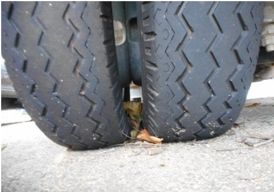
Photo 11 shows the condition of the rear left tyres of the Motor Lorry, which was observed to be in serviceable condition with remaining tread depth of approximately 1.9mm. The tyres, which were wrapped around standard steel wheel rim, were also observed to be sufficiently inflated for vehicular operation.
