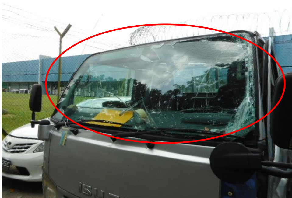
Photo 3 shows a close up view of the Motor Lorry's front portion at the time of my inspection. Its front windscreen (circled) was damage at the time of my inspection as a result of the accident.
