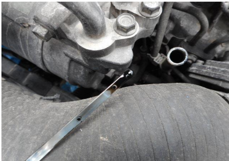
Photo 16 shows the engine oil dip stick of the Motor Lorry at the time of my inspection. The engine oil was observed to be of sufficient level and without any visible contamination.
