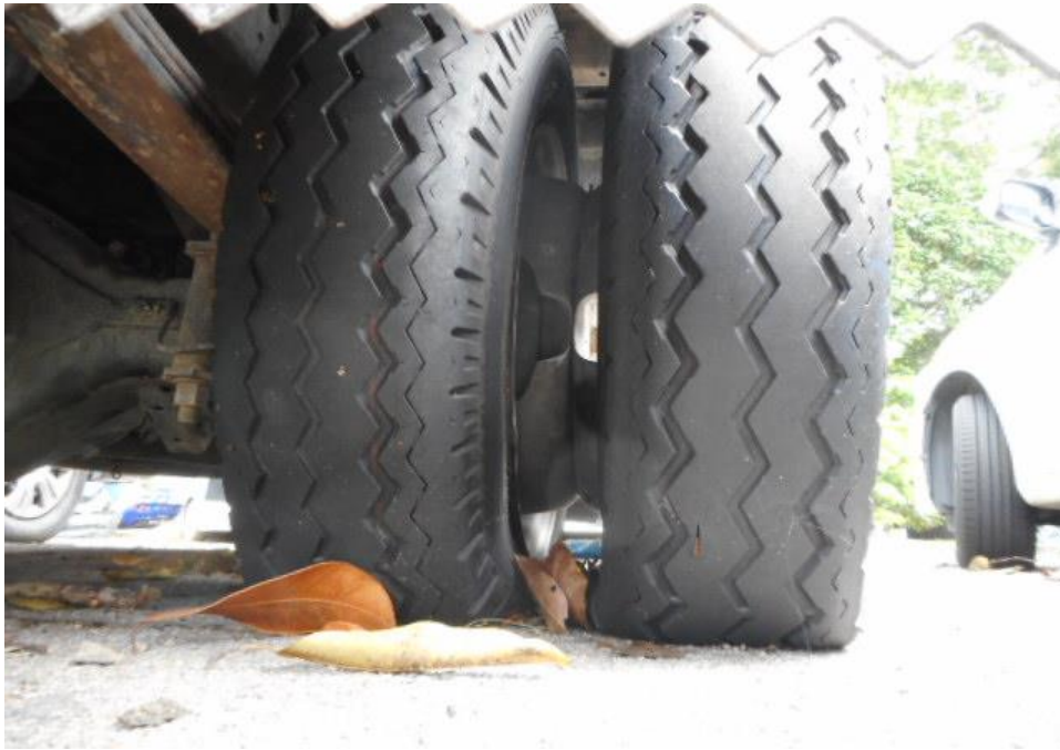
Photo 10 shows the condition of the rear right tyre of the Motor Lorry, which was observed to be in serviceable condition with remaining tread depth of approximately 1.8mm. The tyre, which was wrapped around standard steel wheel rim, it was observed to be sufficiently inflated for vehicular operation.
