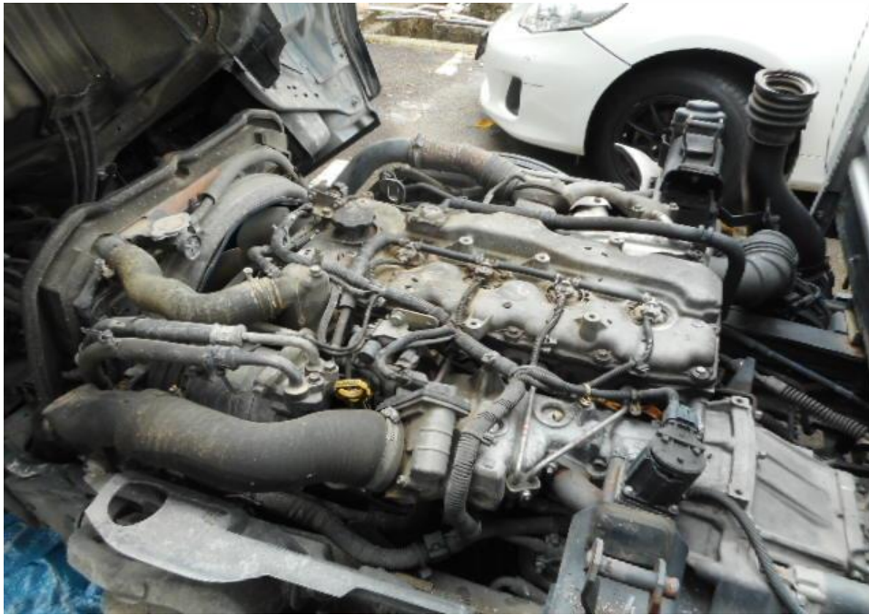
Photo 13 shows a general view of the Motor Lorry's engine compartment, which was accessed by lifting the front cabin of the Motor Lorry. The various parts and components inside the engine compartment were unaffected by the accident. There was also no sign(s) or indication(s) of fresh fluid leakage and/or fluid stain within the engine compartment
