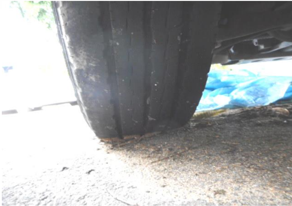
Photo 12 shows the condition of the rear right tyres of the Motor Lorry, which were observed to be in serviceable condition with remaining, tread depth of approximately 7.4mm. There was also no tear, cut or burst mark(s) on the outer and the inner sidewalls as well as across the tread of the 6 tyres that were fitted on the Motor Lorry.
