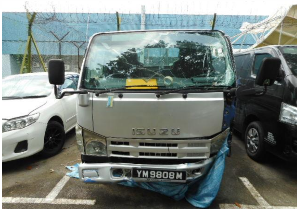
Photo 2 shows a general view of the Motor Lorry's frontal portion at the time of my inspection. It appeared to have sustained damage at its front portion. Its front windscreen, front bumper, front left headlamp and front left door were damage at the time of my inspection as a result of the accident.
