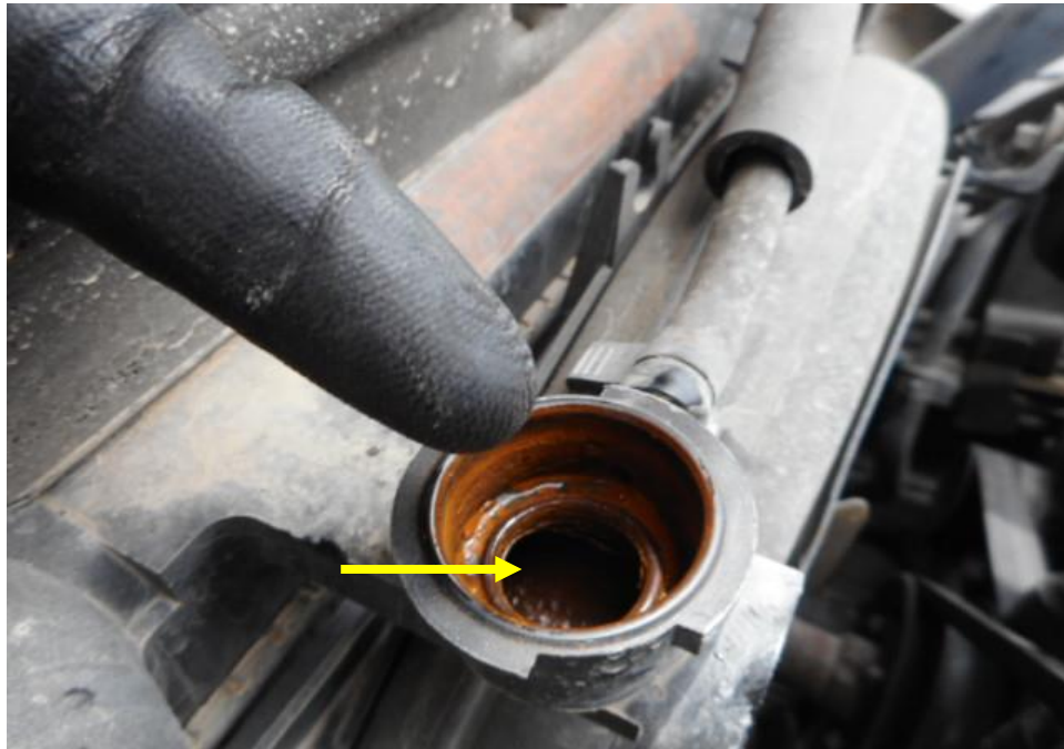
Photo 15 shows the engine coolant reservoir of the Motor Lorry at the time of my inspection. The engine coolant was observed to be of insufficient level (arrowed) which was likely caused by a leakage as a result of the accident.
