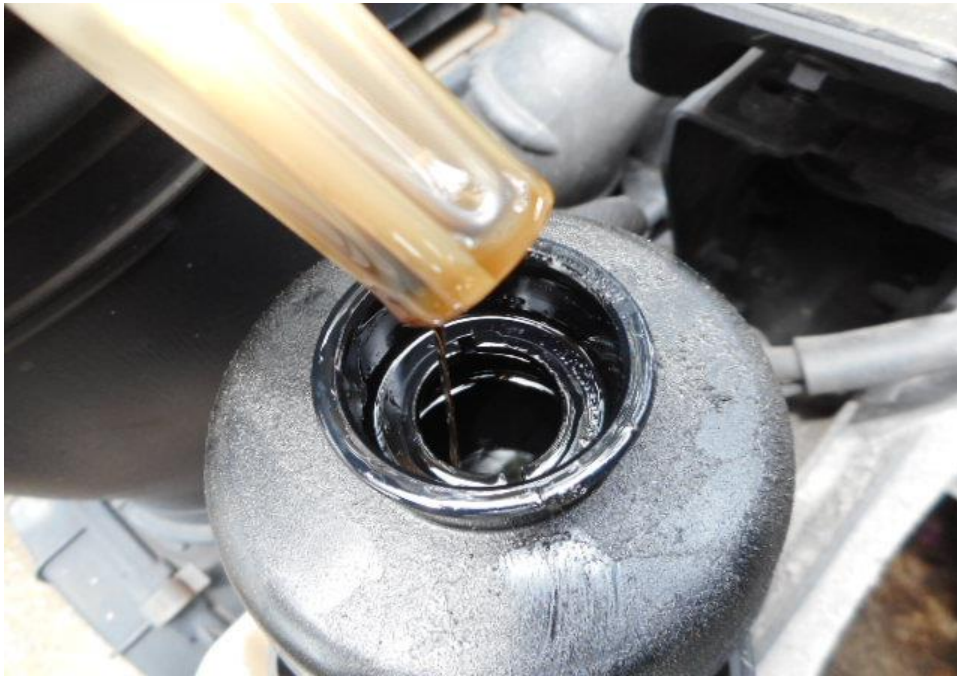
Photo 17 shows the power steering fluid reservoir of the Motor Lorry at the time of my inspection. The power steering fluid was observed to be of sufficient level and without any visible contamination.
