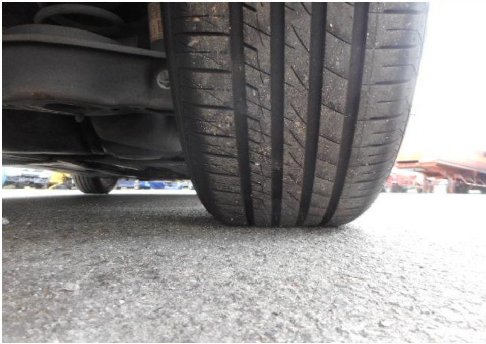
Photo 10 shows the condition of the rear right tyre of the Motor Car, which was observed to be in serviceable condition with remaining tread depth of approximately 6.4mm. The tyre was also observed to be sufficiently inflated for vehicular operation with no tear, cut or burst mark(s).
