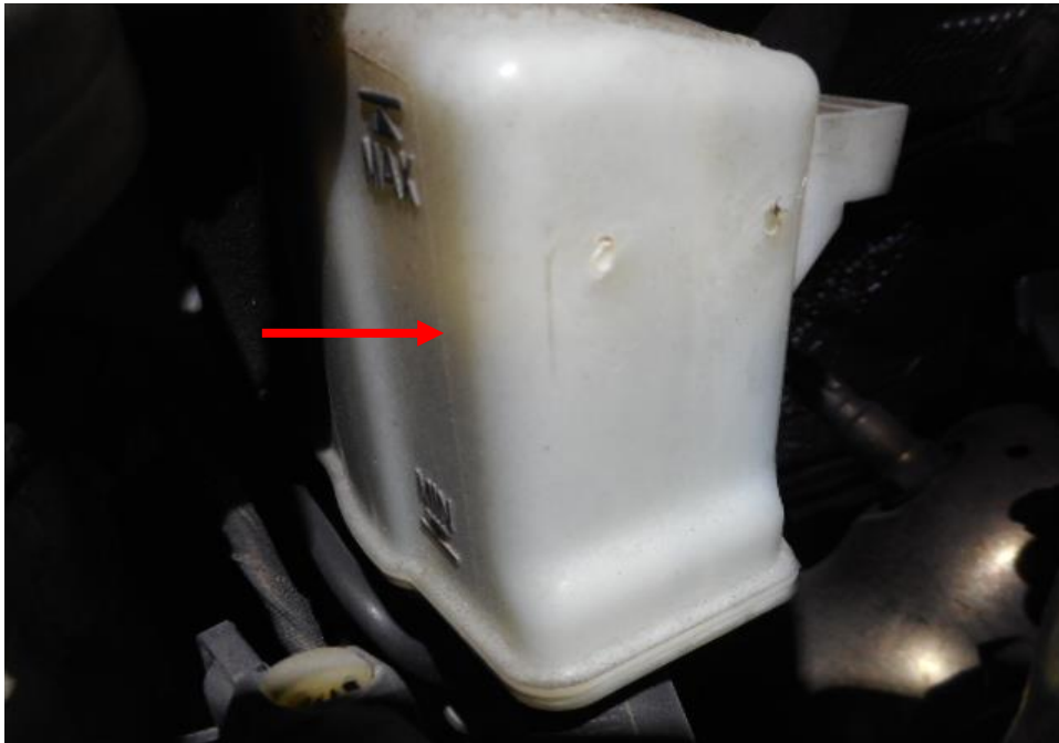
Photo 14 shows the brake fluid reservoir of the Motor Car at the time of my inspection. The brake fluid was observed to be of sufficient level (arrowed) and without any visible contamination.
