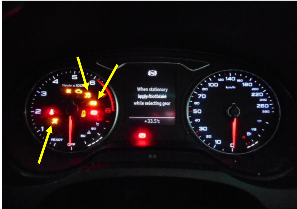
Photo 25 shows the warning light for Anti-Lock Brake System (ABS), Traction Control System (TCS) and Supplemental Restraint System (SRS) (arrowed) appearing on the instrument panel of the Motor Car during the self-test of its various electronic operating systems when its engine was cranked.
