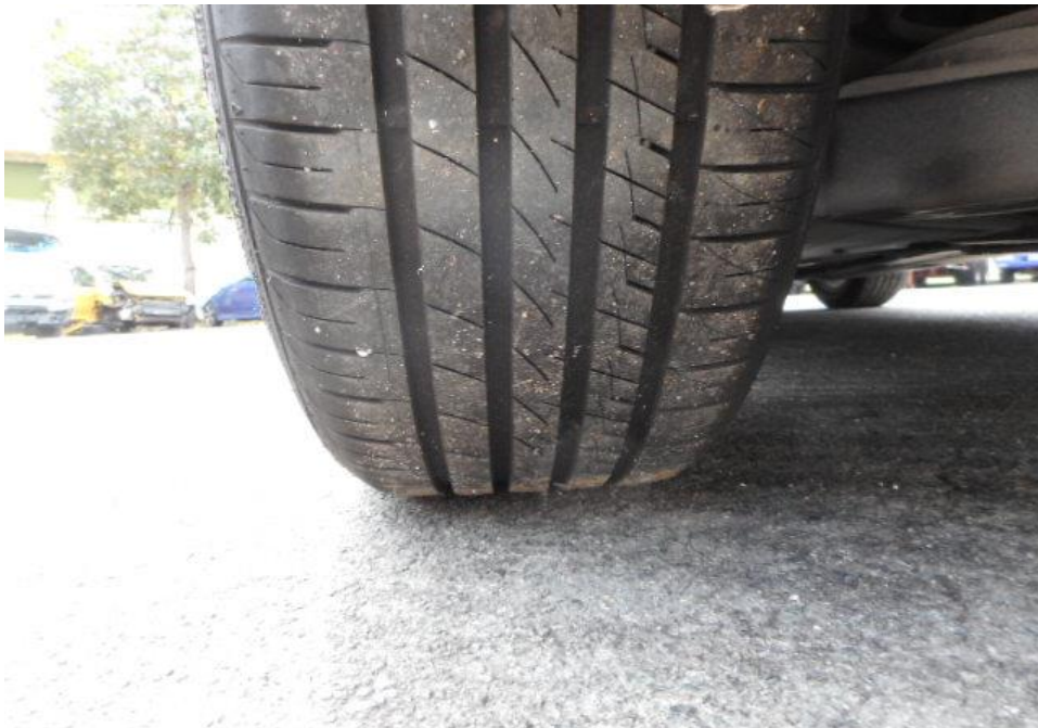
Photo 11 shows the condition of the rear left tyre of the Motor Car, which was observed to be in serviceable condition with remaining tread depth of approximately 6.1mm. The tyre, which was wrapped around steel wheel rim, was also observed to be sufficiently inflated for vehicular operation. The 4 tyres of the Motor Car were wrapped around standard steel wheel rims.
