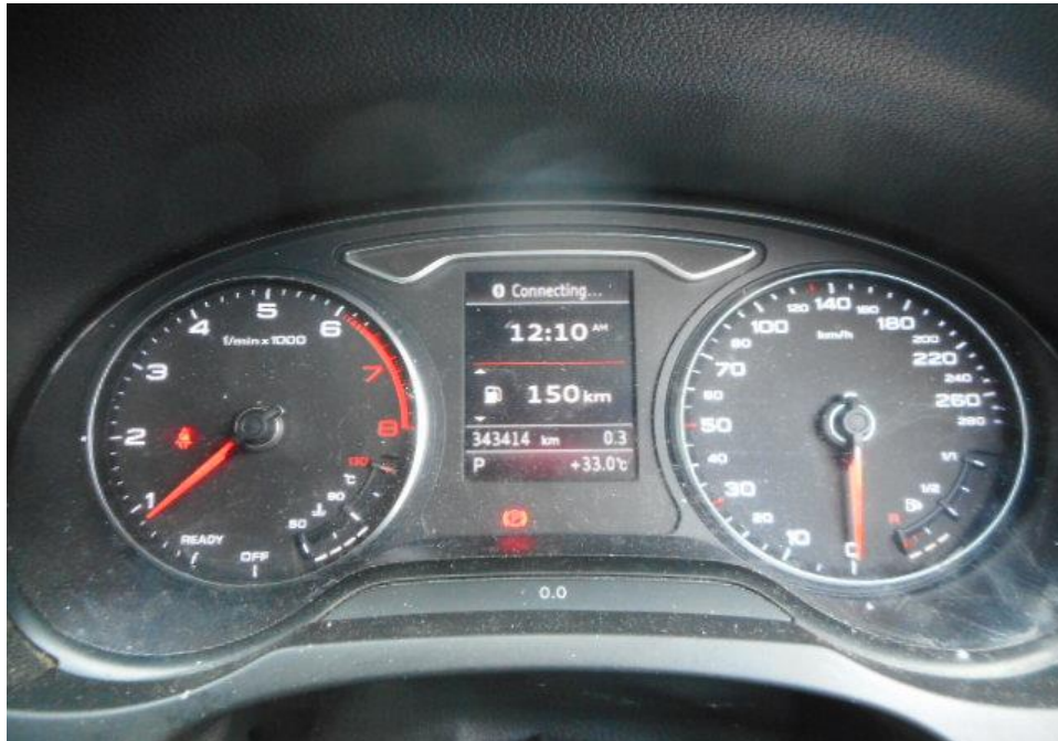
Photo 26 shows no warning lights illuminated on the instrument panel of the Motor Car after the engine was cranked. This would suggest that there was no abnormality to the electronic operating system of the Motor Car, like the ABS, TCS and SRS etc.
