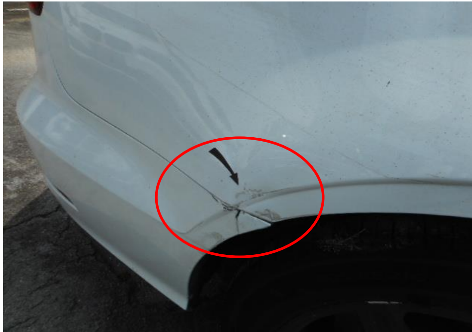
Photo 6 shows a close up view of the Motor Car's front body at the time of my inspection. The right portion of the Motor Car was observed to have sustained damage. Its rear right fender (circled) was the body part that were damaged as a result of the accident.
