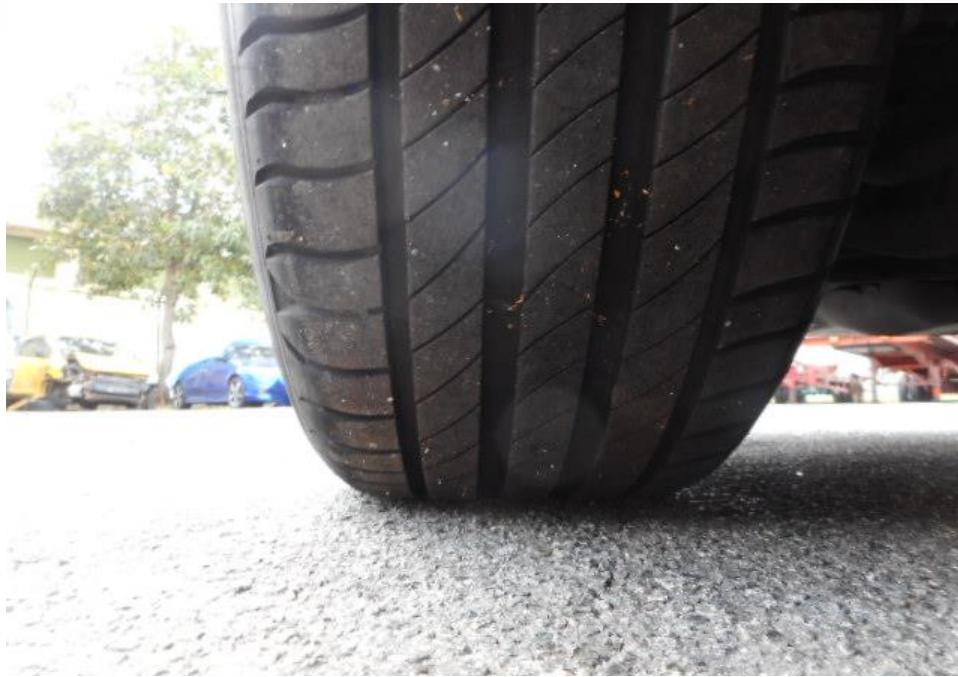
Photo 12 shows the condition of the front left tyre of the Motor Car, which was observed to be in serviceable condition with remaining tread depth of approximately 6.1mm. There was also no tear, cut or burst mark(s) on the outer and the inner sidewalls as well as across the tread of the Motor Car's 4 tyres.
