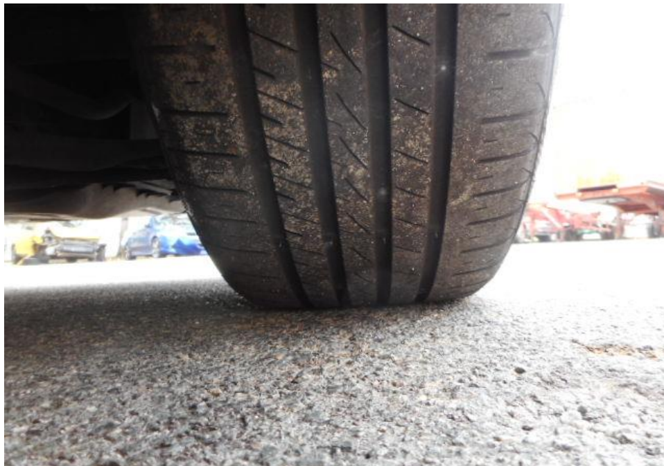
Photo 9 shows the condition of the front right tyre of the Motor Car, which was observed to be in serviceable condition with remaining tread depth of approximately 4.1mm. The tyre was sufficiently inflated for vehicular operation with no tear, cut or burst mark(s) on the outer and the inner sidewalls as well as across the tread. The 4 tyres of the Motor Car were wrapped around standard steel wheel rims without any damage.
