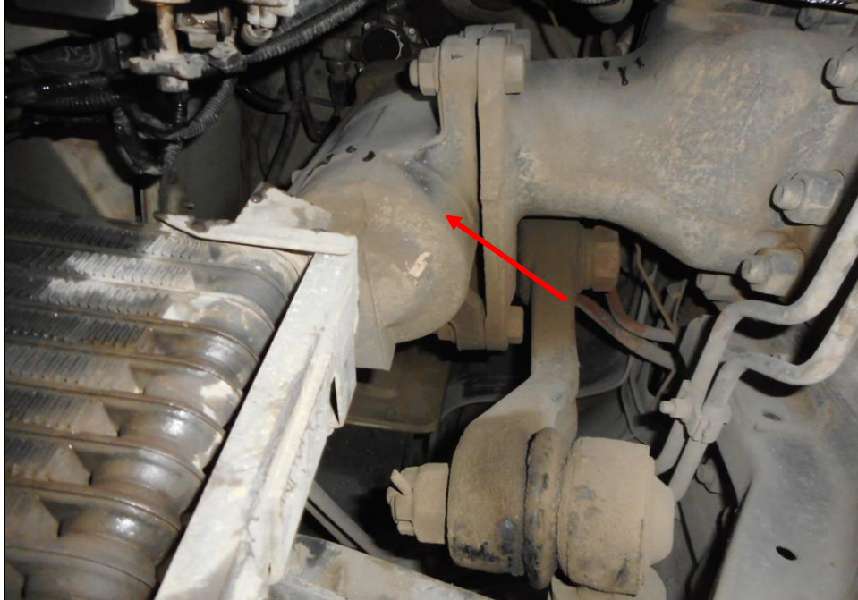
Photo 22 shows the steering box component (arrowed) at the undercarriage of the Motor Trailer was found to be intact without any visible damage. There was also no sign of fluid stain(s) observed on the various undercarriage components.
