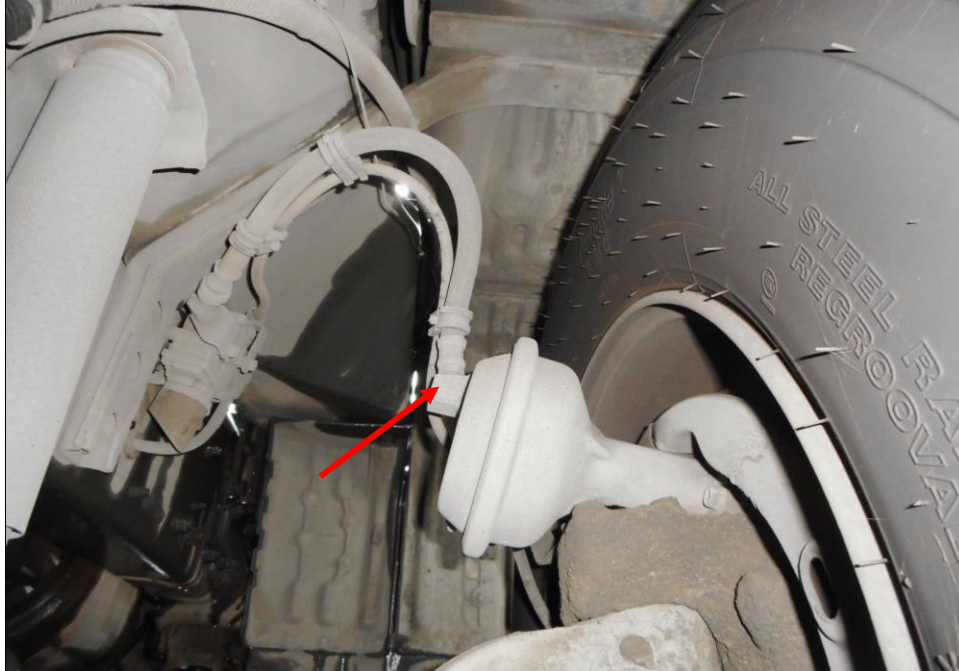
Photo 18 shows the brake pipe (arrowed) at the front left wheel of the Motor Trailer. I did not observe any leakage of brake fluid at the time of my inspection of the Motor Trailer. My visual examination of the various mechanical components in the braking system had indicated that there was no internal leakage of pressure/vacuum and there components were generally in good condition.
