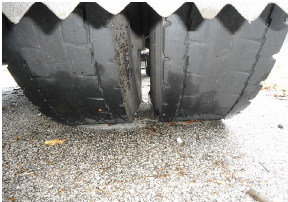
Photo 10 shows the condition of the rear right tyre of the Motor Trailer, which was observed to be in serviceable condition with remaining tread depth of approximately 3mm. The tyre, which was wrapped around standard steel wheel rim, was also observed to be sufficiently inflated for vehicular operation.
