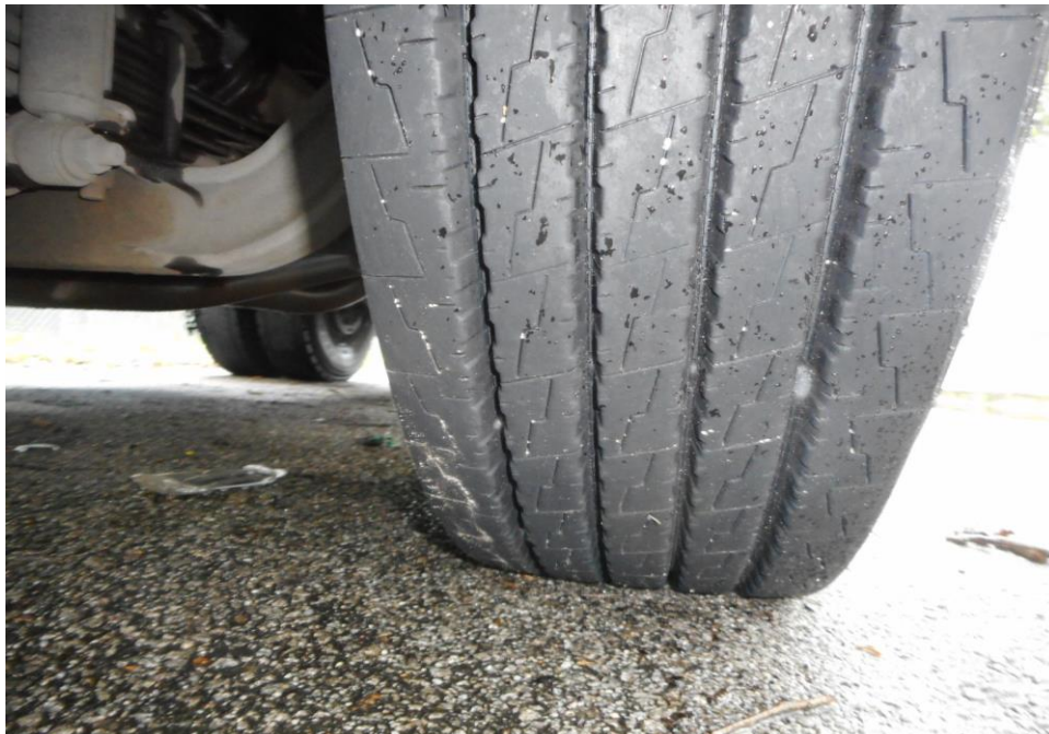
Photo 12 shows the condition of the front left tyres of the Motor Trailer, which were observed to be in serviceable condition with remaining tread depth of approximately 12mm. There was also no tear, cut or burst mark(s) on the outer and the inner sidewalls as well as across the tread of the 6 tyres that were fitted on the Trailer.
