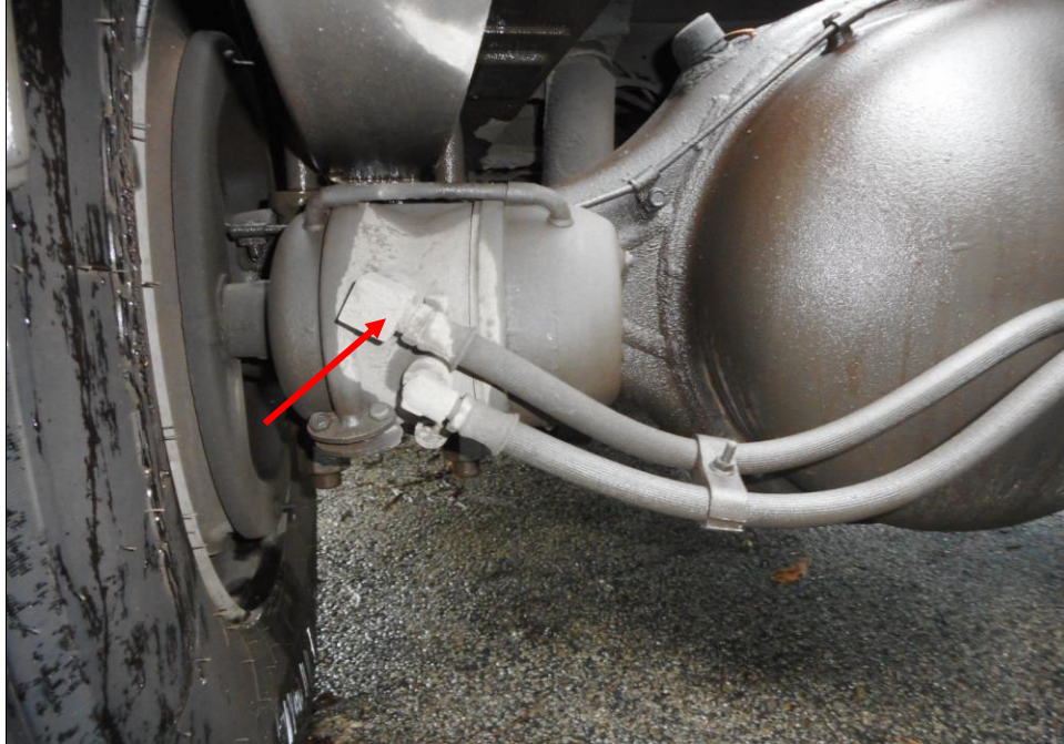
Photo 16 shows the brake pipe (arrowed) at the rear left wheel of the Motor Trailer. I did not observe any leakage of brake fluid at the time of my inspection of the Motor Trailer. My static tests of the Motor Trailer's braking system, along with my visual examination of the various mechanical components in the braking system, had indicated that there was no internal leakage of pressure/vacuum and there components were generally in good condition.
