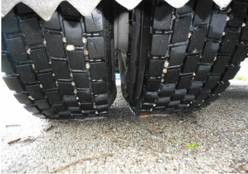
Photo 11 shows the condition of the rear left tyres of the Motor Trailer, which was observed to be in serviceable condition with remaining tread depth of approximately 10.2mm. The tyres, which were wrapped around standard steel wheel rim, were also observed to be sufficiently inflated for vehicular operation. There was also no damage found on all 6 steel wheel rims of the Trailer.
