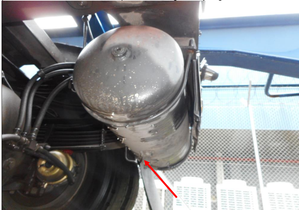
Photo 19 shows the air brake cylinders (arrowed) at the undercarriage of the Motor Trailer. I did not observe any leakage of air brake fluid at the time of my inspection of the Motor Trailer. My visual examination of the various mechanical components in the braking system had indicated that there was no internal leakage of pressure/vacuum and there components were generally in good condition.
