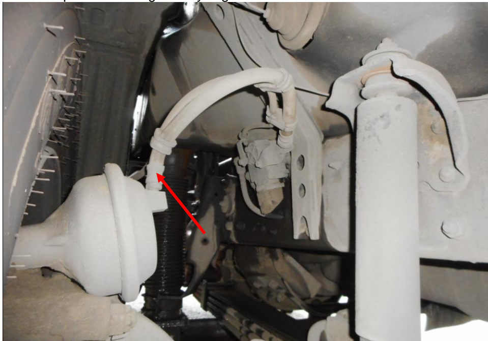
Photo 17 shows the brake pipe (arrowed) at the front right wheel of the Motor Trailer. I did not observe any leakage of brake fluid at the time of my inspection of the Motor Trailer. My static tests of the Motor Trailer's braking system, along with my visual examination of the various mechanical components in the braking system, had indicated that there was no internal leakage of pressure/vacuum and there components were generally in good condition.
