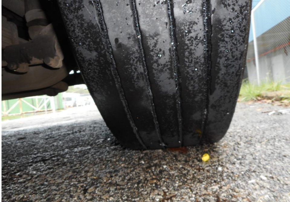
Photo 9 shows the condition of the front right tyre of the Motor Trailer, which was observed to be in serviceable condition with remaining tread depth of approximately 6.6 mm. The tyre, which was wrapped around standard steel wheel rim, was also observed to be sufficiently inflated for vehicular operation. There was no tear, cut or burst mark(s) on the outer and the inner sidewalls as well as across the tread of the 6 tyres that were fitted on the Motor Trailer.
