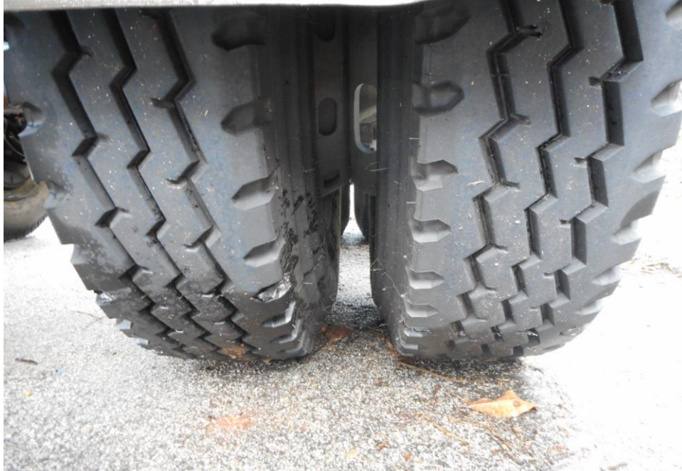
Photo 13 shows the condition of the right tyres of the Trailer, which was observed to be in serviceable condition with remaining, tread depth of approximately 11.9mm. The tyre, which was wrapped around standard steel wheel rim, was also observed to be sufficiently inflated for vehicular operation.
