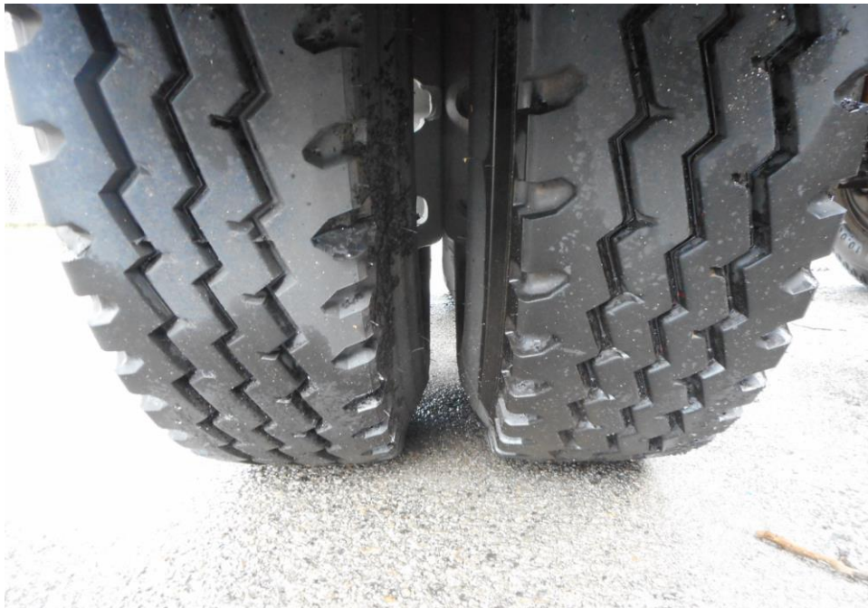
Photo 14 shows the condition of the left tyres of the Trailer, which was observed to be in serviceable condition with remaining tread depth of approximately 9.2mm. The tyres, which were wrapped around standard steel wheel rim, were also observed to be sufficiently inflated for vehicular operation. There was also no damage found on all 12 steel wheel rims of the Trailer.
