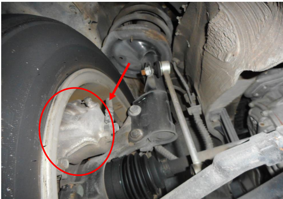
Photo 21 shows the brake hose/pipe (arrowed) at the front left wheel of the Police Car. No leakage of brake fluid was observed. Visual examination of the various components of the braking system like the brake caliper (circled), brake booster, brake pedal etc had revealed all to be intact and without visible damage.
