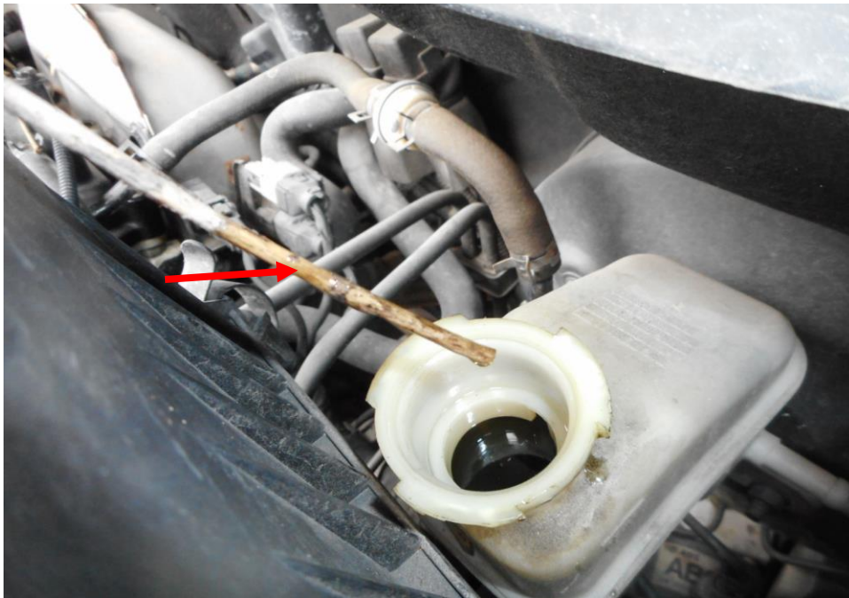
Photo 14 shows the brake fluid reservoir of the Police Car at the time of my inspection. The brake fluid was observed to be of sufficient level (arrowed) and without any visible contamination.
