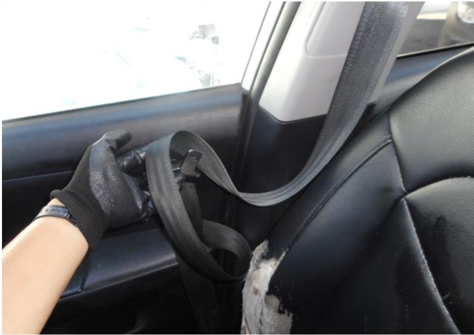
Photo 28 shows that the seat belt on the right seat was worn at the material time of accident as the safety pre-tensioners was activated at the moment of impact and caused the seat belts to be locked into the last position of the user.
