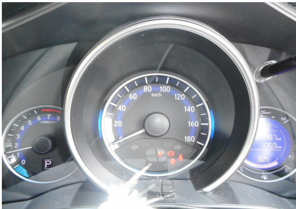
Photo 26 shows only the Supplemental Restraint System (SRS) warning light remained illuminated on the instrument panel of the Police Car after the engine was cranked. This was due to the deployment of the airbag.
