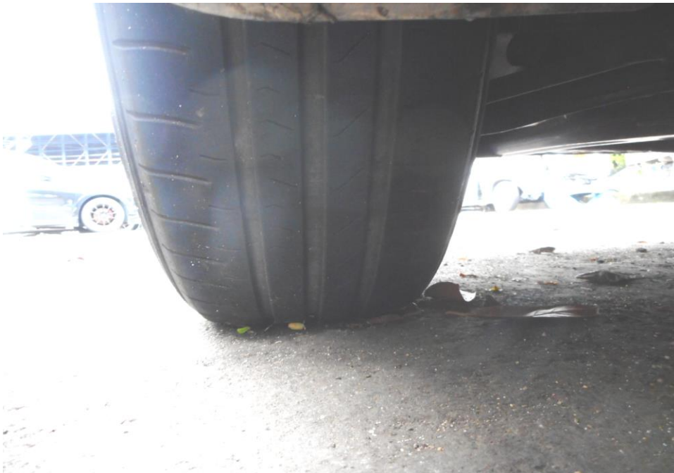
Photo 11 shows the condition of the front left tyre of the Police Car, which was observed to be in serviceable condition with remaining tread depth of approximately 4.7mm. The tyre, which was wrapped around steel wheel rim, was also observed to be sufficiently inflated for vehicular operation. The 4 tyres of the Police Car were wrapped around standard steel wheel rims.
