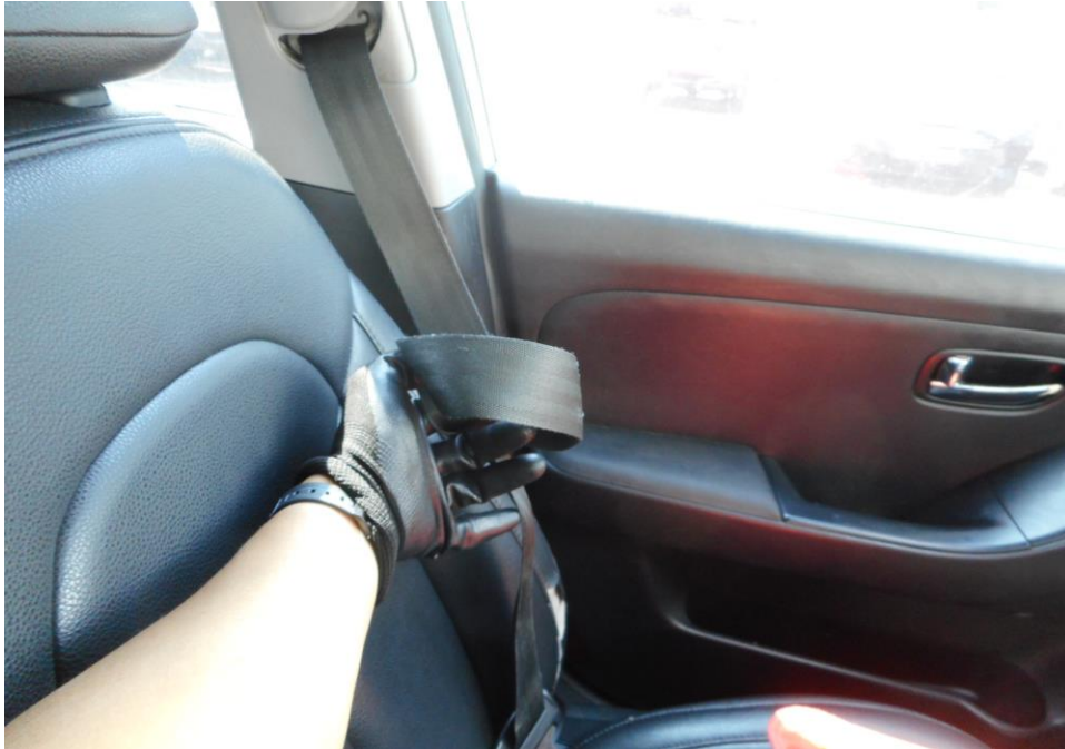
Photo 27 shows that the seat belt on the left seat was worn at the material time of accident as the safety pre-tensioners was activated at the moment of impact and caused the seat belts to be locked into the last position of the user.
