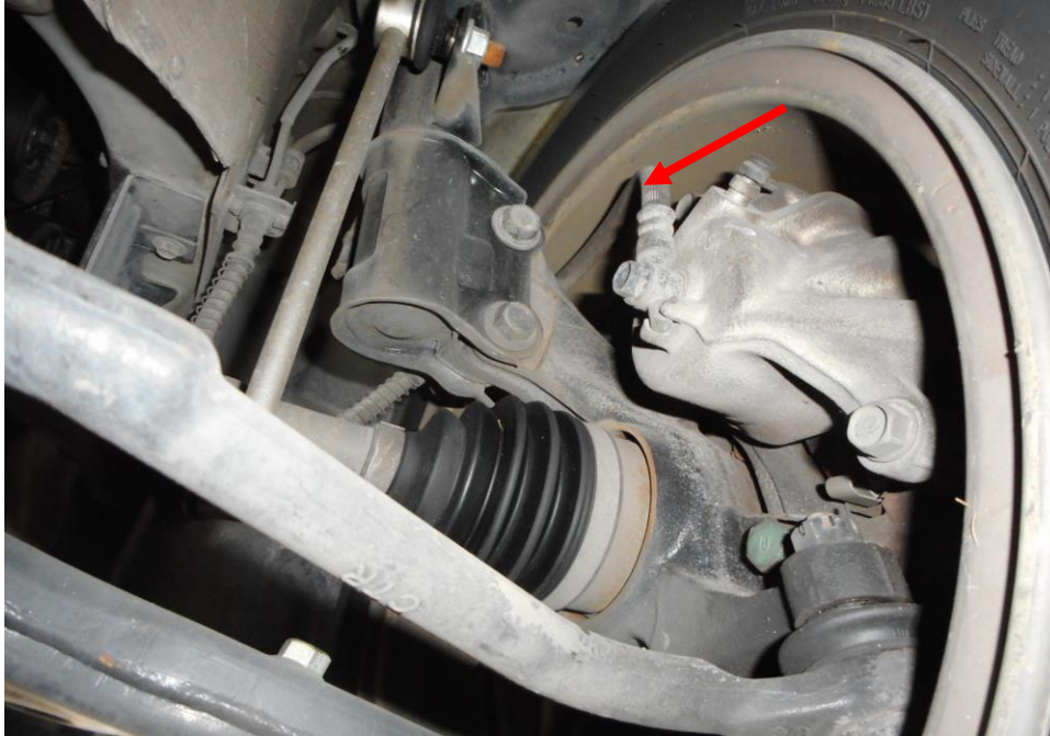
Photo 20 shows the brake hose/pipe (arrowed) at the front right wheel of the Police Car. I did not observe any leakage of brake fluid at the time of my inspection of the Police Car. Static tests of the Police Car's braking system had indicated that there was no internal leakage of pressure/vacuum. The undercarriage components of the Police Car were also all found to be intact and without any visible damage.
