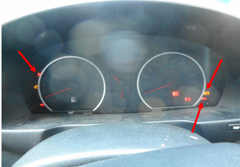
Photo 25 shows the warning light for Anti-Lock Brake System (ABS) and Power Steering System (EPS), and Supplemental Restraint System (SRS) (arrowed) appearing on the instrument panel of the Police Car during the self-test of its various electronic operating systems when its engine was cranked.
