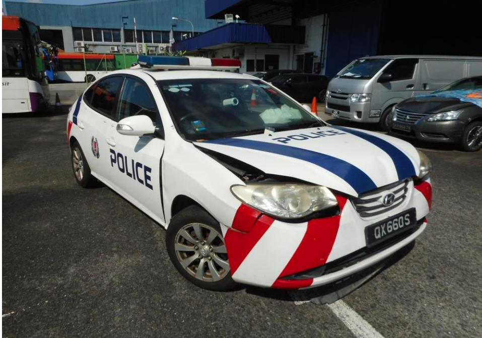
Photo 22 shows the front right wheel of the Police Car turned to its full left. During my steering system test, I did not experience any abnormal free play and/or resistance when I had turned the steering wheel towards the left and right. This would suggest that the steering system of the Police Car was likely to be in serviceable condition at the material time of accident.
