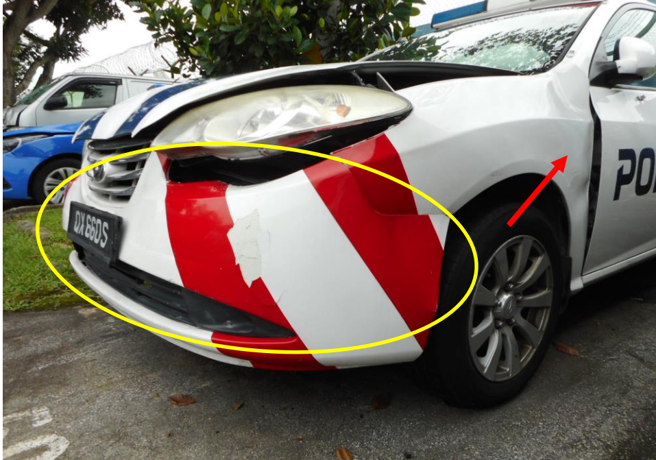
Photo 4 shows the close up view of the Police Car's front body at the time of my inspection. The Police Car was observed to have sustained damage at its front bumper (circled) & front left fender (arrowed), as a result of the accident.
