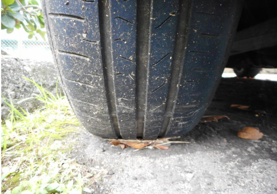
Photo 8 shows the condition of the front right tyre of the Police Car, which was observed to be in serviceable condition with remaining tread depth of approximately 4.5mm. The tyre was sufficiently inflated for vehicular operation with no tear, cut or burst mark(s) on the outer and the inner sidewalls as well as across the tread. The 4 tyres of the Police Car were wrapped around standard steel wheel rims without any damage.
