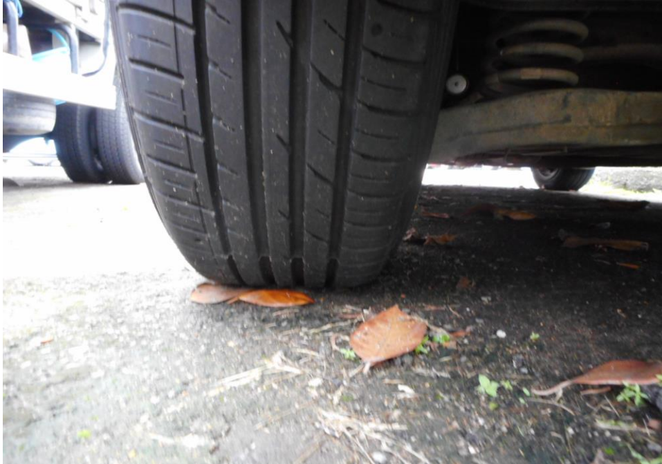
Photo 10 shows the condition of the rear left tyre of the Police Car, which was observed to be in serviceable condition with remaining tread depth of approximately 6.7mm. The tyre, which was wrapped around steel wheel rim, was also observed to be sufficiently inflated for vehicular operation. The 4 tyres of the Police Car were wrapped around standard steel wheel rims.
