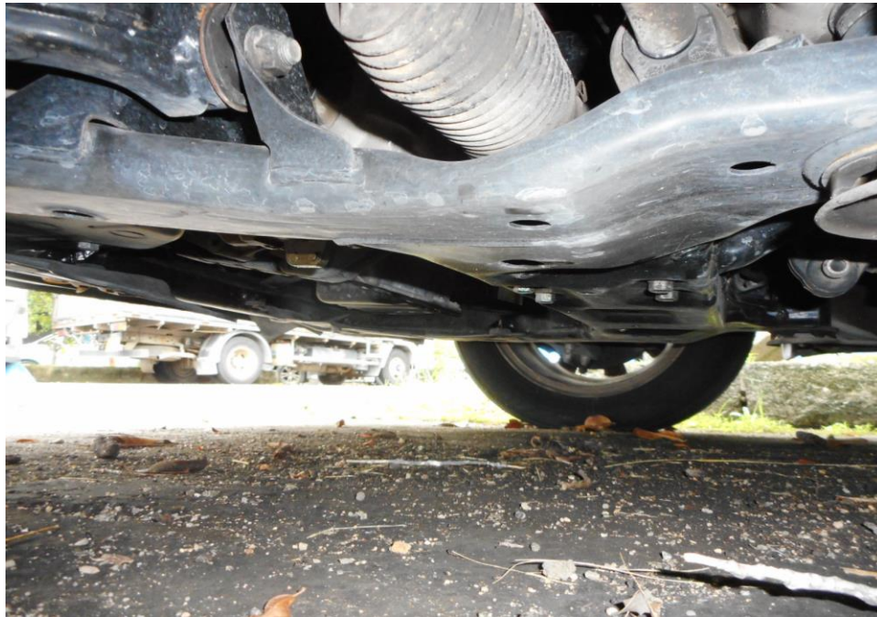
Photo 17 shows the undercarriage of the Police Car, at the area where the engine housing and transmission housing are located. I did not find any sign(s) or indication(s) of fluid leak and/or fluid stain(s) on the underside of the Police Car.
