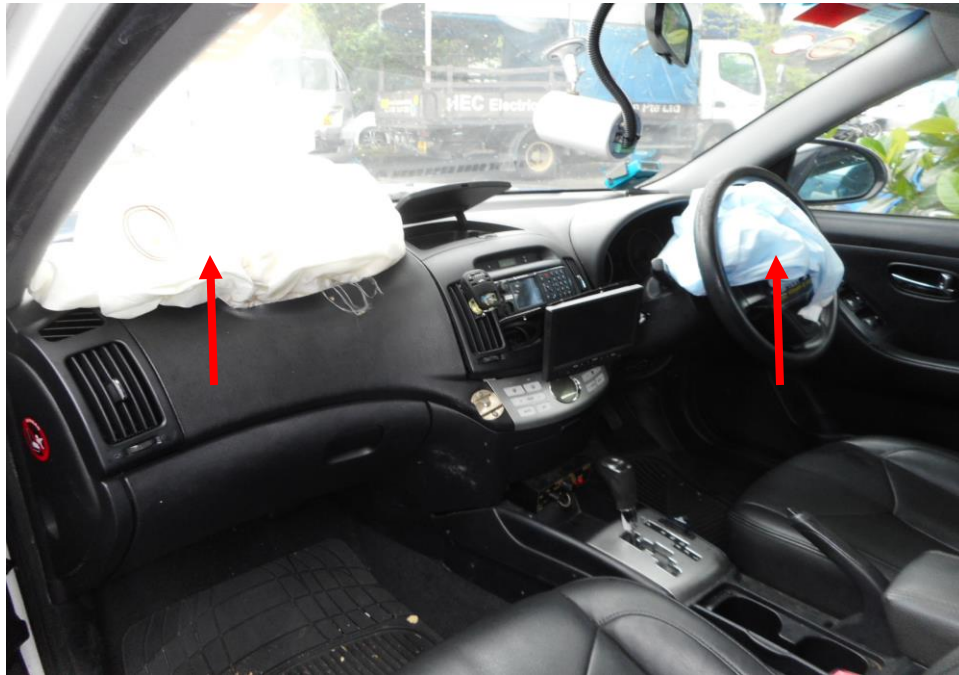
Photo 12 shows the deployment of the Supplemental Restraint System (SRS) airbag (arrowed) in the Police Car as a result of the accident.
