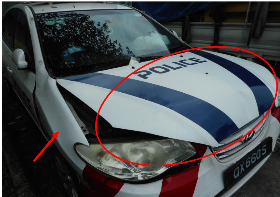
Photo 3 shows the close up view of the Police Car's front body at the time of my inspection. The Police Car was observed to have sustained damage at its front bonnet (circled) & front right fender (arrowed), as a result of the accident.
