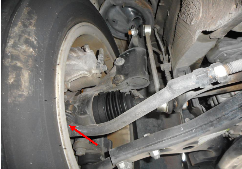
Photo 24 shows the various undercarriage components at the front left wheel of the Police Car, which had included the steering tie rod (red arrow). The various undercarriage components of the Police Car were all found to be intact without any visible damage.
