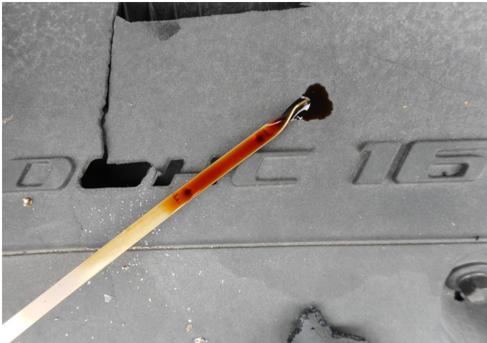
Photo 16 shows the engine oil dip stick of the Police Car at the time of my inspection. The engine oil was observed to be of sufficient level and without any visible contamination.
