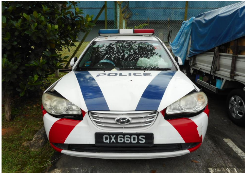
Photo 2 shows a general view of the Police Car's front body at the time of my inspection. The front portion of the Police Car was observed to have sustained damage. Its front bumper, front bumper, both front left and right fender was the body parts that were damaged as a result of the accident. The Supplemental Restraint System (SRS) was activated as a result of the accident.
