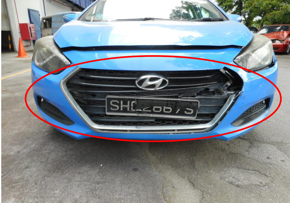
Photo 4 shows the close up view of the Motor Taxi's front body at the time of my inspection. The Motor Taxi was observed to have sustained damage at its front bumper, number plate and front grille (circled) as a result of the accident.
