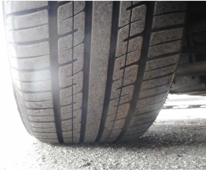
Photo 10 shows the condition of the front left tyre of the Motor Taxi, which was observed to be in serviceable condition with remaining tread depth of approximately 5.9mm. There was also no tear, cut or burst mark(s) on the outer and the inner sidewalls as well as across the tread of the Motor Taxi's 4 tyres.
