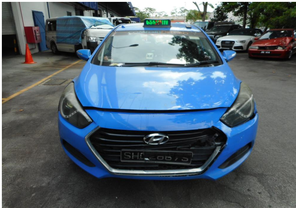
Photo 3 shows a general view of the Motor Taxi's front body at the time of my inspection. The front portion of the Motor Taxi was observed to have sustained damage. Its front bumper, number plate and front right headlamp was the body parts that were damaged as a result of the accident.
