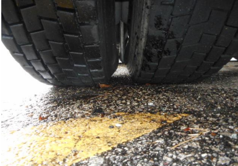
Photo 11 shows the condition of the rear left tyres of the Motor Trailer, which was observed to be in serviceable condition with remaining tread depth of approximately 6.3mm. The tyres, which were wrapped around standard steel wheel rim, were also observed to be sufficiently inflated for vehicular operation. There was also no damage found on all 10 steel wheel rims of the Trailer.
