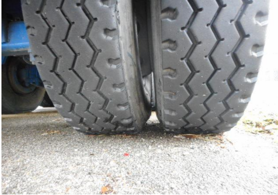
Photo 13 shows the condition of the right tyres of the Trailer, which was observed to be in serviceable condition with remaining tread depth of approximately 10.6mm. The tyre, which was wrapped around standard steel wheel rim, was also observed to be sufficiently inflated for vehicular operation.
