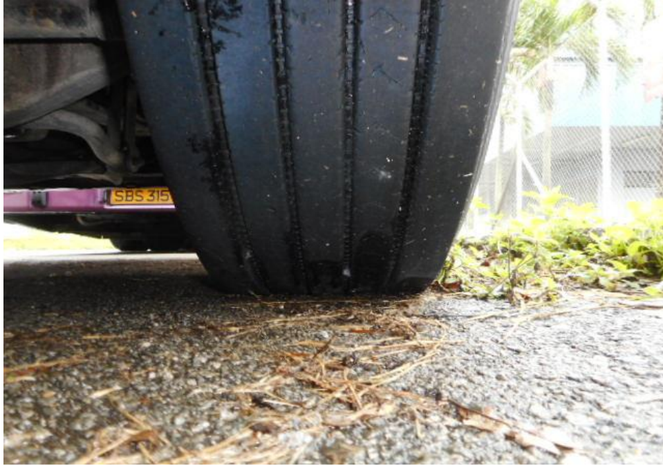
Photo 9 shows the condition of the front right tyre of the Motor Trailer, which was observed to be in serviceable condition with remaining tread depth of approximately .8.9 mm. The tyre, which was wrapped around standard steel wheel rim, was also observed to be sufficiently inflated for vehicular operation. There was no tear, cut or burst mark(s) on the outer and the inner sidewalls as well as across the tread of the 10 tyres that were fitted on the Motor Trailer.
