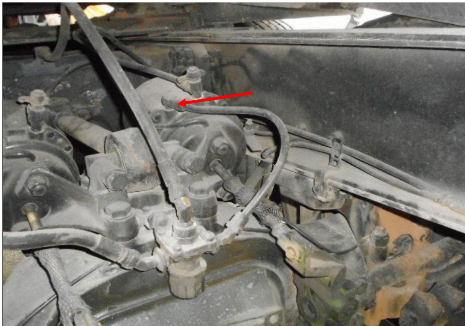
Photo 15 shows the brake pipe (arrowed) at the rear right wheel of the Motor Trailer. I did not observe any leakage of brake fluid at the time of my inspection of the Motor Trailer. My visual examination of the various mechanical components in the braking system, had indicated that there was no internal leakage of pressure/vacuum and there components were generally in good condition.
