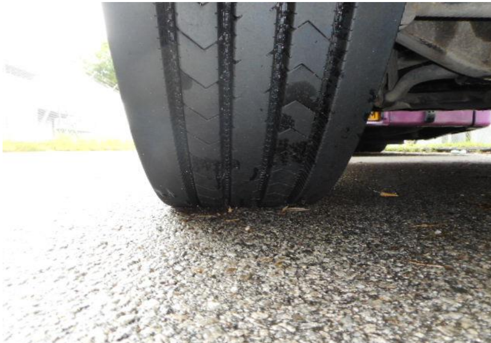
Photo 12 shows the condition of the front left tyres of the Motor Trailer, which were observed to be in serviceable condition with remaining tread depth of approximately 13.1mm. There was also no tear, cut or burst mark(s) on the outer and the inner sidewalls as well as across the tread of the 10 tyres that were fitted on the Trailer.
