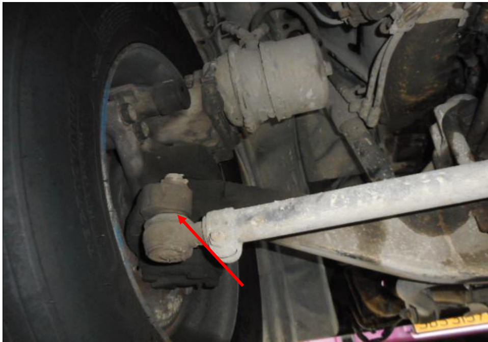
Photo 21 shows the various undercarriage components at the front left wheel of the Motor Trailer, in particular the steering tie rod end (arrowed). The various undercarriage components of the Motor Trailer were all found to be intact without any visible damage. There was also no sign of fluid stain(s) observed on the various undercarriage components.
