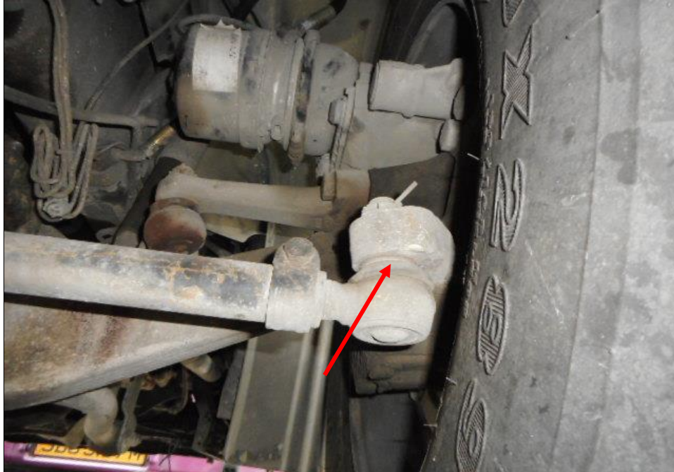
Photo 20 shows the various undercarriage components at the front right wheel of the Motor Trailer, in particular the steering tie rod end (arrowed). The various steering components were all found to be intact, suggesting that the steering system of the Motor Trailer was likely to be in serviceable condition at the material time of accident. There was also no sign of fluid stain(s) observed on the various undercarriage components.
