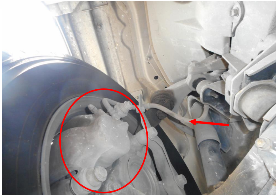
Photo 22 shows the brake hose/pipe (arrowed) at the front left wheel of the Motor Lorry. No leakage of brake fluid was observed. Visual examination of the various components of the braking system like the brake caliper (circled), brake booster, brake pedal etc had revealed all to be intact and without visible damage at the time of accident. There was also no sign of fluid stain(s) observed on the various undercarriage components.
