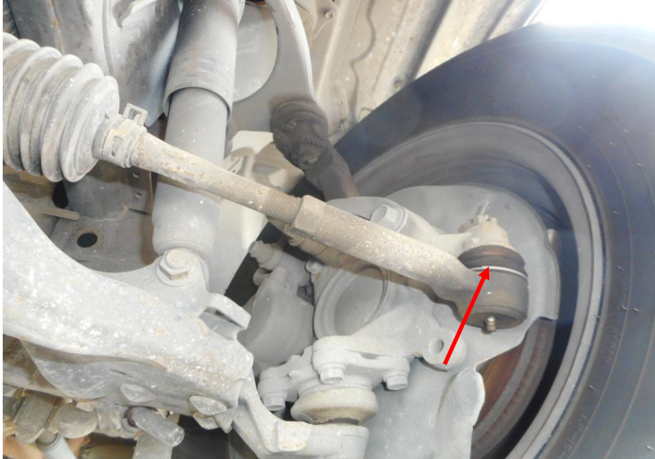
Photo 18 shows the various undercarriage components at the front left wheel of the Motor Lorry, in particular the steering tie rod end (arrowed). The various undercarriage components of the Motor Lorry were all found to be intact without any visible damage. There was also no sign of fluid stain(s) observed on the various undercarriage components.
