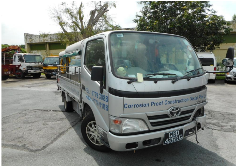
Photo 23 shows the front right wheel of the Motor Lorry turned to its full left. During my steering system test, I did not experience any abnormal free play and/or resistance when I had turned the steering wheel towards full left and full right. This would suggest that the steering system of the Motor Lorry was likely to be in serviceable condition at the material time of accident.
