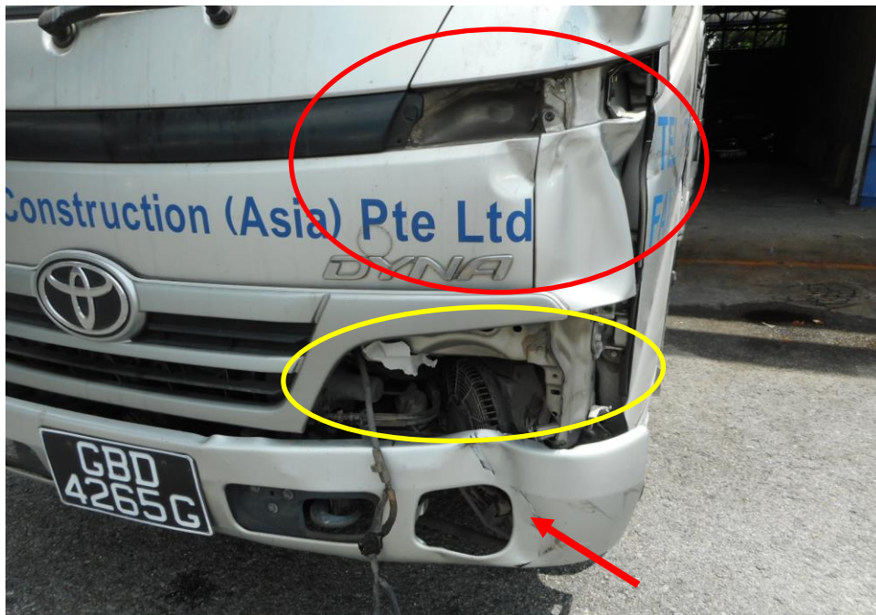
Photo 3 shows a close up view of the Motor Lorry's front portion at the time of my inspection. Its front left headlamp (yellow circle) and front body panel (red circle) and front bumper (arrowed) was damage at the time of my inspection as a result of the accident.
