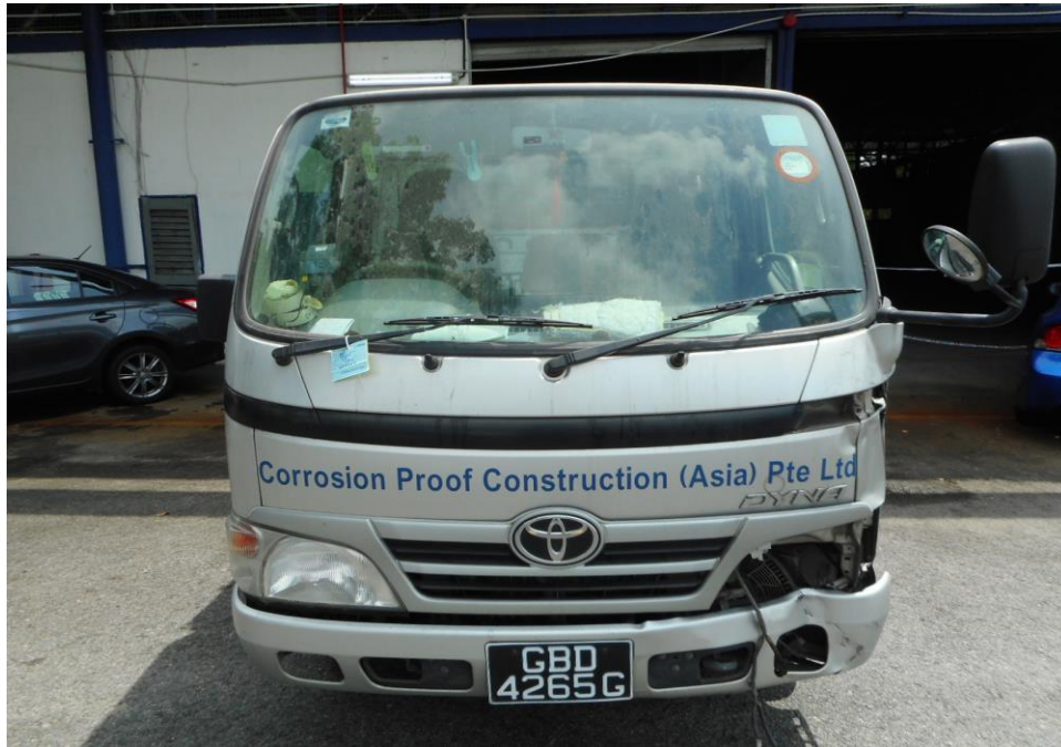
Photo 2 shows a general view of the Motor Lorry's frontal portion at the time of my inspection. It appeared to have sustained damage at its front portion. Its front left headlamp, front body panel and front bumper were damage at the time of my inspection as a result of the accident.
