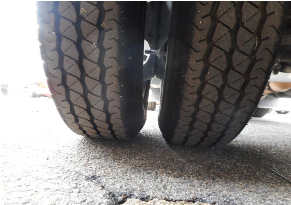
Photo 9 shows the condition of the rear left tyres of the Motor Lorry, which was observed to be in serviceable condition with remaining tread depth of approximately 5.8mm. The tyres, which were wrapped around standard steel wheel rim, were also observed to be sufficiently inflated for vehicular operation. There was also no damage found on all 6 steel wheel rims of the Motor Lorry.
