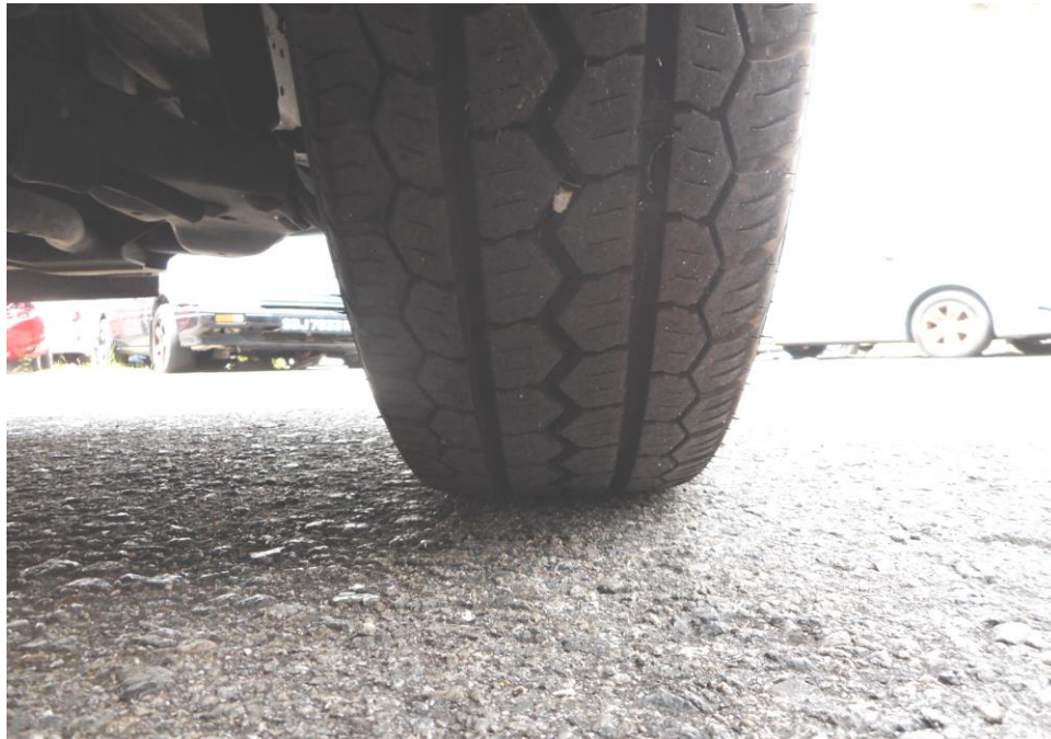
Photo 7 shows the condition of the front right tyre of the Motor Lorry, which was observed to be in serviceable condition with remaining tread depth of approximately 8mm. The tyre, which was wrapped around standard steel wheel rim, was also observed to be sufficiently inflated for vehicular operation. There was no tear, cut or burst mark(s) on the outer and the inner sidewalls as well as across the tread of the 6 tyres that were fitted on the Motor Lorry.
