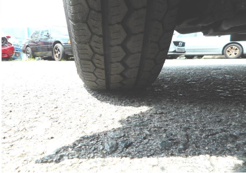
Photo 10 shows the condition of the rear right tyres of the Motor Lorry, which were observed to be in serviceable condition with remaining, tread depth of approximately 7.7mm. There was also no tear, cut or burst mark(s) on the outer and the inner sidewalls as well as across the tread of the 6 tyres that were fitted on the Motor Lorry.
