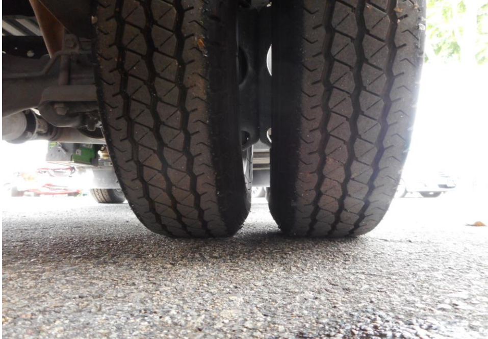
Photo 8 shows the condition of the rear right tyre of the Motor Lorry, which was observed to be in serviceable condition with remaining tread depth of approximately 5.5mm. The tyre, which was wrapped around standard steel wheel rim, it was observed to be sufficiently inflated for vehicular operation.
