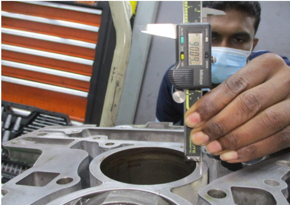
Photo 11 shows the stroke measurement of cylinder 1, which was recorded to be 90.09mm.
