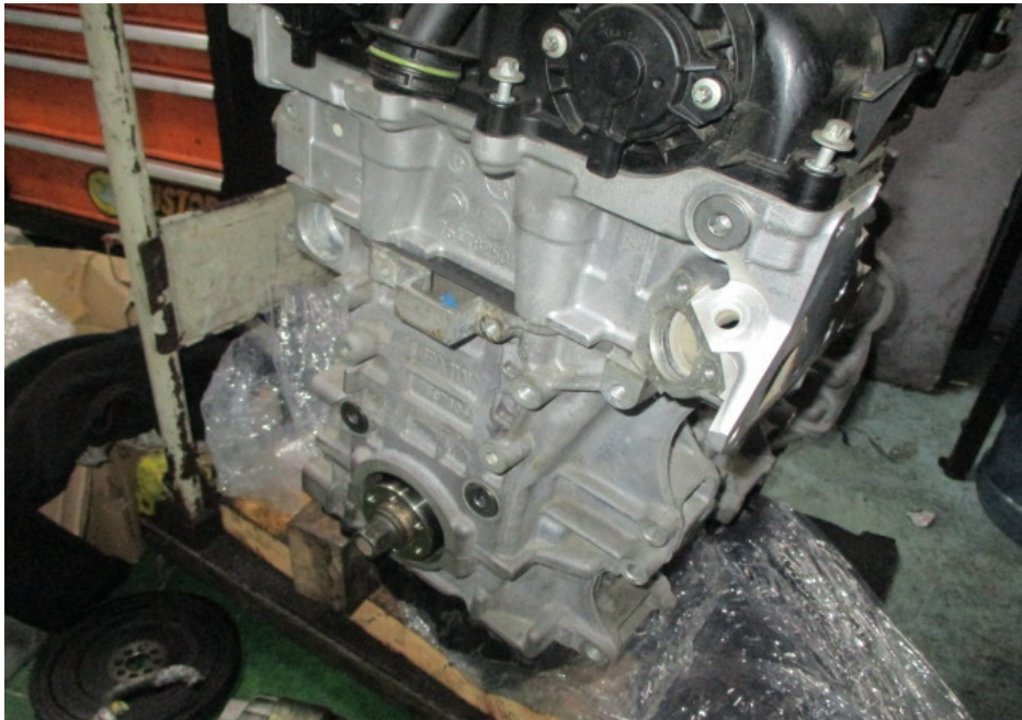
Photo 3 shows a general view of the BMW engine that I had inspected. My visual examination of the engine housing revealed the housing to be of serviceable/satisfactory condition. There was no crack and/or hole observed on the engine housing.
