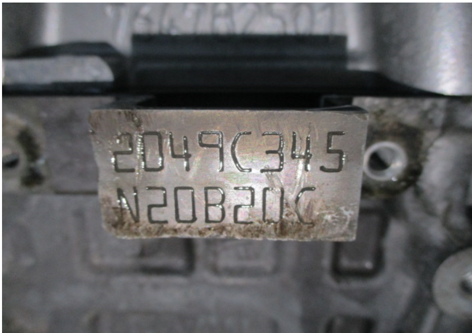
Photo 4 shows the engine number engraved on the housing of the BMW engine that I had inspected. The engine number was 2049C345N20B20C.
