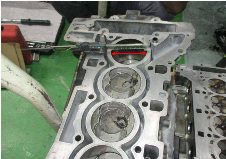
Photo 7 shows measurement being carried out to the bore (arrowed) of cylinder 1 of the BMW engine. The measurements were carried out using a digital Vernier Caliper that was calibrated before the start of the measurements.
