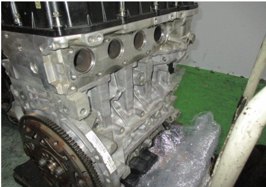
Photo 2 shows a general view of the BMW engine that I had inspected. My visual examination of the engine housing revealed the housing to be of serviceable/satisfactory condition. There was no crack and/or hole observed on the engine housing.
