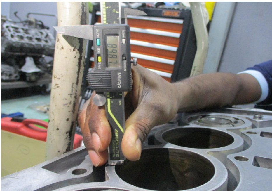
Photo 18 shows the stroke measurement of cylinder 3, which was recorded to be 89.87mm.
