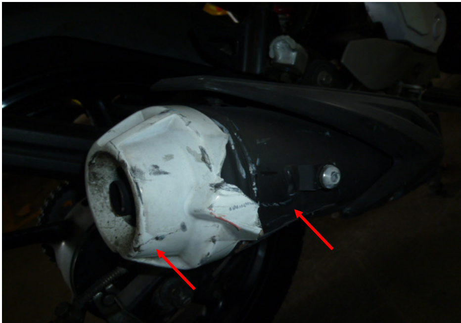
Photo 15 shows a closer view of the exhaust muffler and exhaust muffler heat shield which were amongst the body parts of the Motorcycle that had sustained damages of grazing nature as a result of the accident (arrowed).
