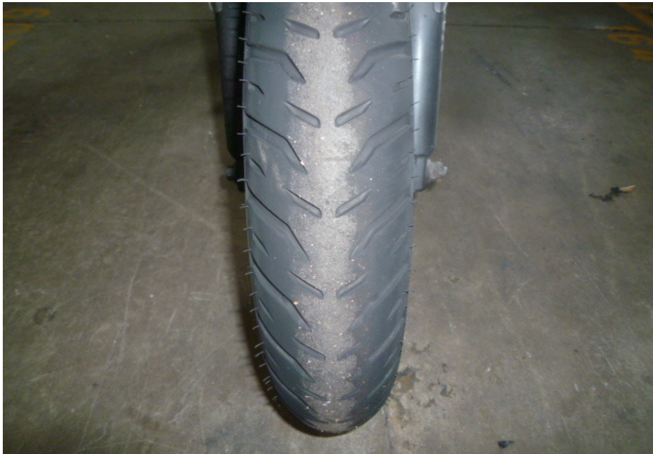
Photo 16 shows the front tyre of the Motorcycle at the time of our inspection. The front tyre was observed to be in serviceable condition with remaining tread depth of approximately 4mm. The pattern of the tread was also clearly visible. There was no tear, burst mark(s) and/or punctured hole(s) on the sidewalls as well as across the tread of the front tyre.
