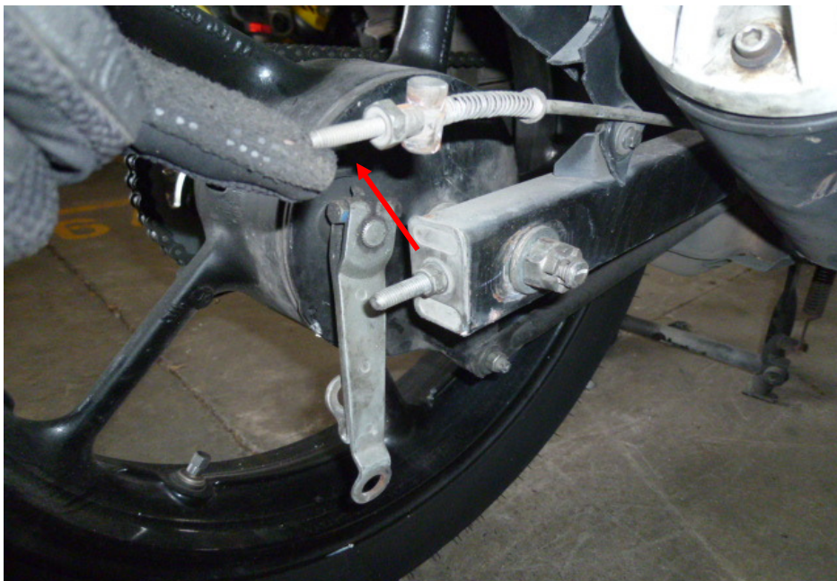
Photo 28 shows the rear wheel of the Motorcycle. The type of brake system for the rear wheel was of a mechanical type, controlled by the brake foot pedal of the Motorcycle. Our checks of the spring and drum which are all part of the components in the rear brake system of the Motorcycle reveal all to be intact and without damage. However the rear brake cable was observed to be dislodged as a result of the accident (arrowed).
