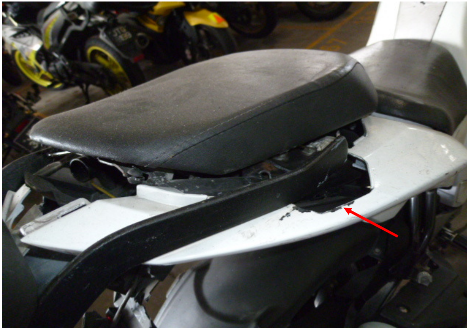
Photo 10 shows a closer view of the cracked right rear side cover (arrowed) of the Motorcycle as a result of the accident.
