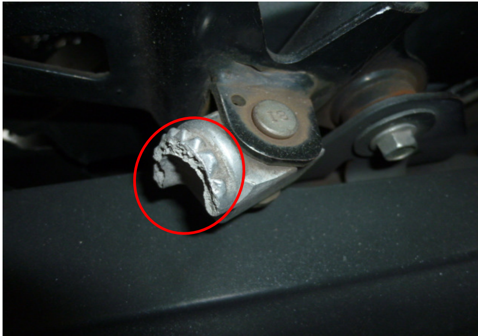
Photo 12 shows a closer view of the broken right pillion footpeg of the Motorcycle as a result of the accident (circled).
