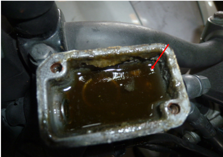
Photo 26 shows the brake fluid reservoir for the front brake of the Motorcycle. The brake fluid was found to be of sufficient level for operating purposes. However the brake fluid was found to be contaminated (arrowed).
