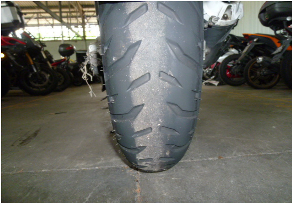
Photo 17 shows the condition of the Motorcycle's rear tyre. The rear tyre was observed to be in serviceable condition with remaining tread depth of approximately 4mm. The tyre was also observed to be sufficiently inflated for vehicular operation. We did not observe any tear, burst mark(s) and/or punctured hole(s) on the sidewalls as well as across the tread of the rear tyre.
