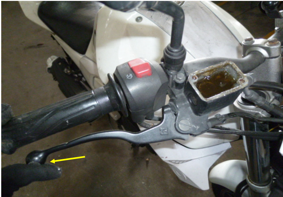
Photo 27 shows the front brake lever being depressed. There was some resistance felt (spongy like feel) upon pressing the front brake lever (arrowed). This would indicate that there is no leakage of pressure/vacuum in the front brake system.
