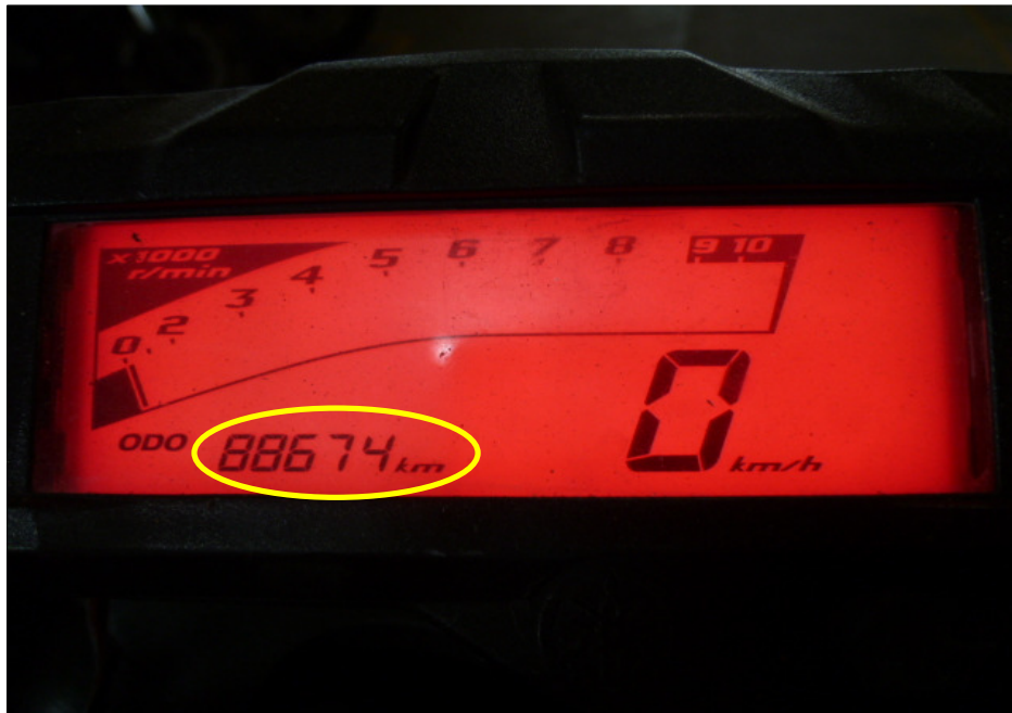
Photo 1 shows the speedometer gauge of the Motorcycle. The mileage of the Motorcycle at the time of our inspection was 88, 674km (circled).
