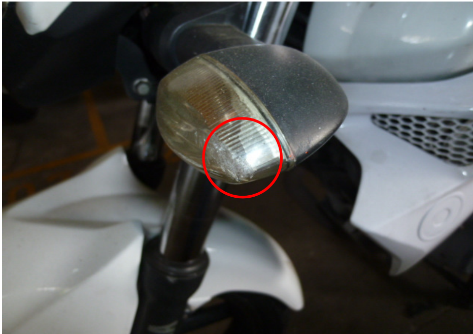
Photo 6 shows a closer view of the left front signal lamp which was amongst the body parts of the Motorcycle that had sustained damage as a result of the accident (circled).
