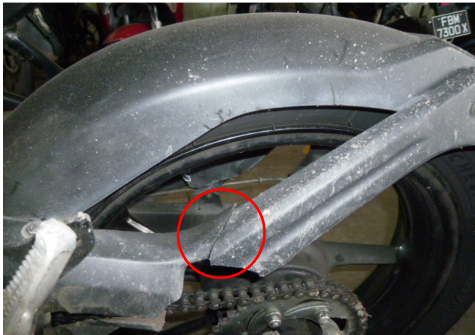
Photo 13 shows the cracked rear mudguard (circled) of the Motorcycle as a result of the accident.
