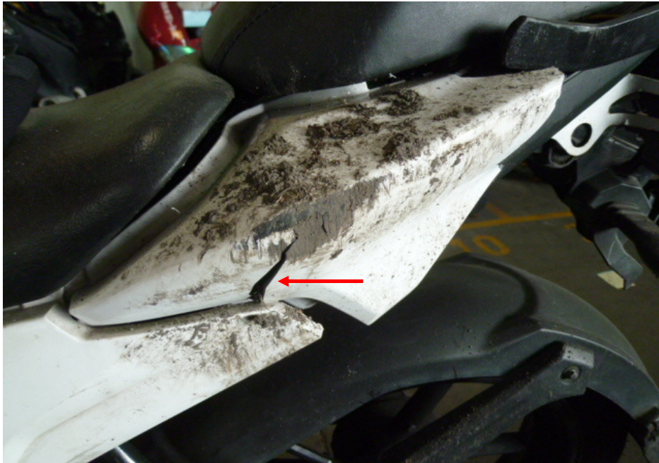
Photo 9 shows a closer view of the cracked left rear side cover (arrowed) of the Motorcycle as a result of the accident.
