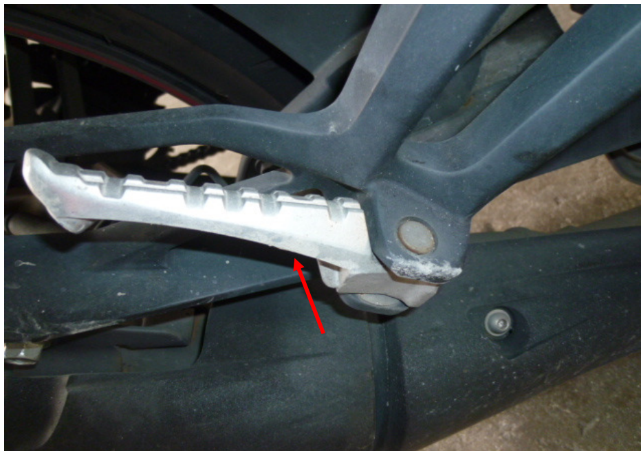
Photo 9 shows a closer view of the right pillion footpeg which was amongst the body parts of the Motorcycle that had sustained damage as a result of the accident (arrowed).
