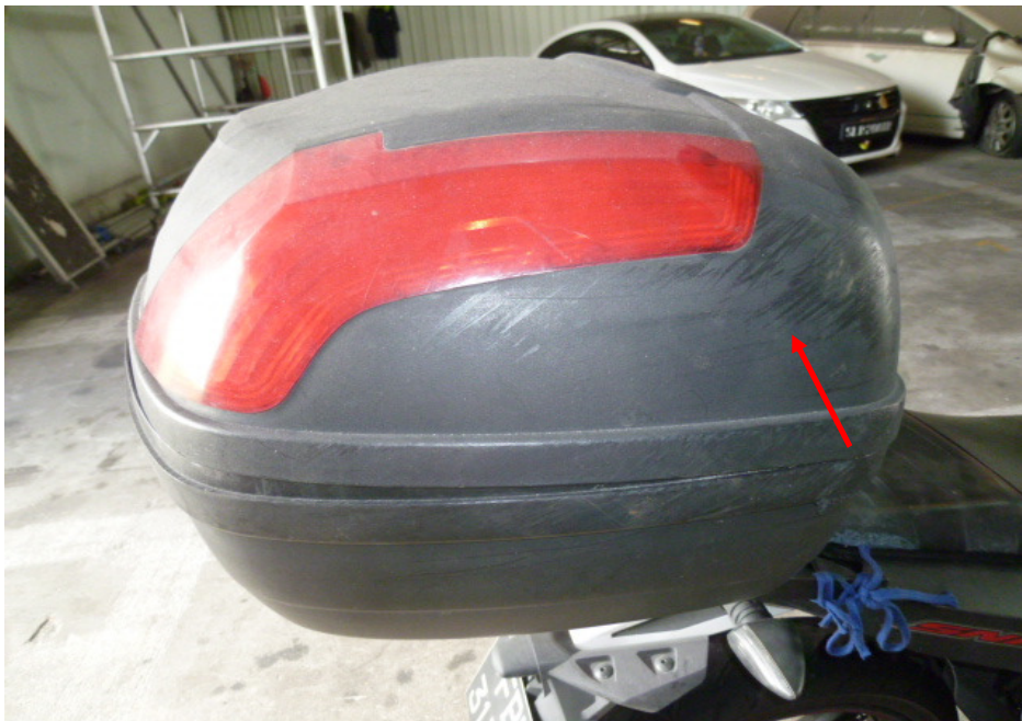
Photo 11 shows a closer view of top box which was amongst the body parts of the Motorcycle that had sustained damages of grazing nature as a result of the accident (circled).
