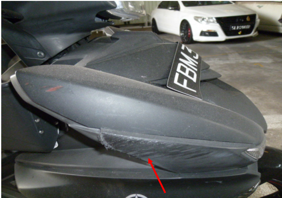
Photo 6 shows the front cowling (arrowed), which were amongst the body parts of the Motorcycle that had sustained damage as a result of the accident.
