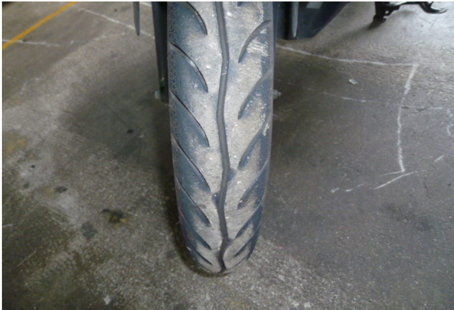
Photo 14 shows the front tyre of the Motorcycle at the time of our inspection. The front tyre was observed to be in serviceable condition with remaining tread depth of approximately 3mm. The pattern of the tread was also clearly visible. There was no tear, burst mark(s) and/or punctured hole(s) on the sidewalls as well as across the tread of the front tyre.
