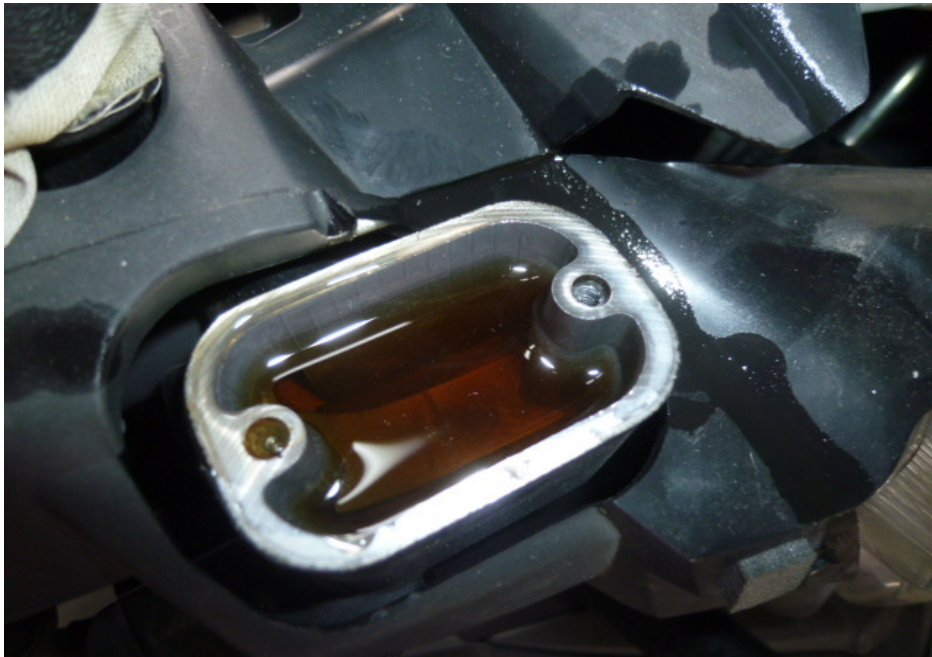
Photo 24 shows the brake fluid reservoir for the front brake of the Motorcycle. The brake fluid was found to be without contamination and of sufficient level for operating purposes.
