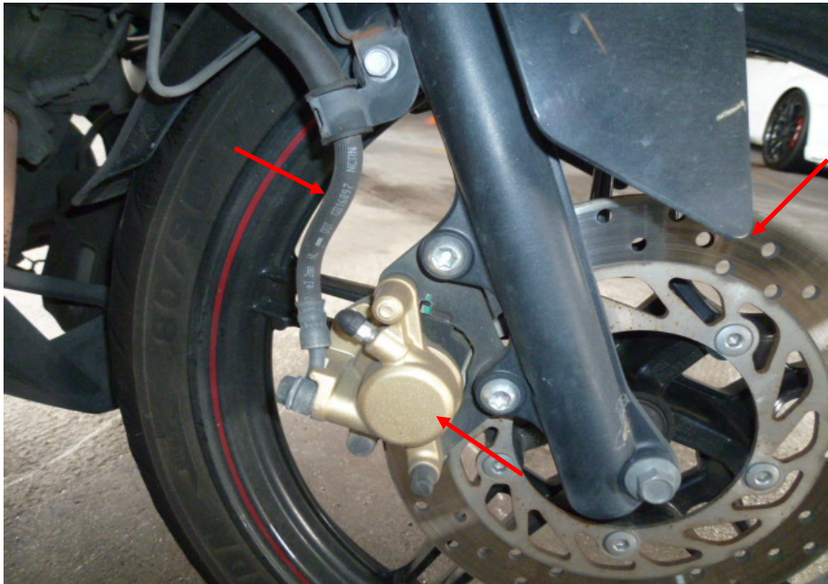
Photo 23 shows a close up view of the front brake caliper, front brake disc and front brake hose (arrowed) of the Motorcycle, which are all part of the components in the hydraulic front brake system of the Motorcycle. Our visual checks of these various components had revealed all to be intact with no visible damage. No leakage of brake fluid was also observed.
