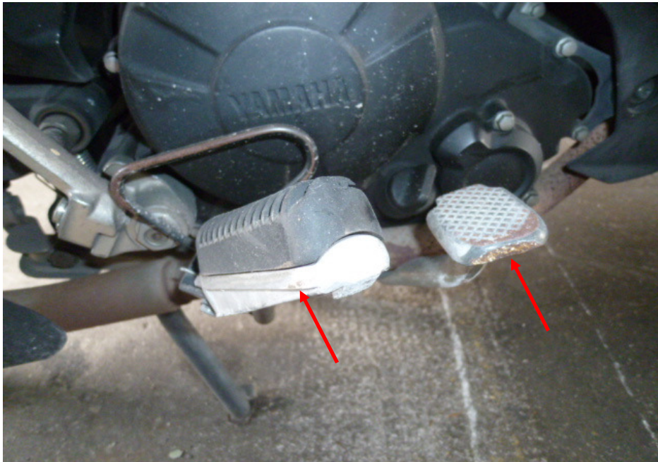
Photo 12 shows the rear brake pedal and right front footrest of the Motorcycle that had sustained damage as a result of the accident (arrowed).
