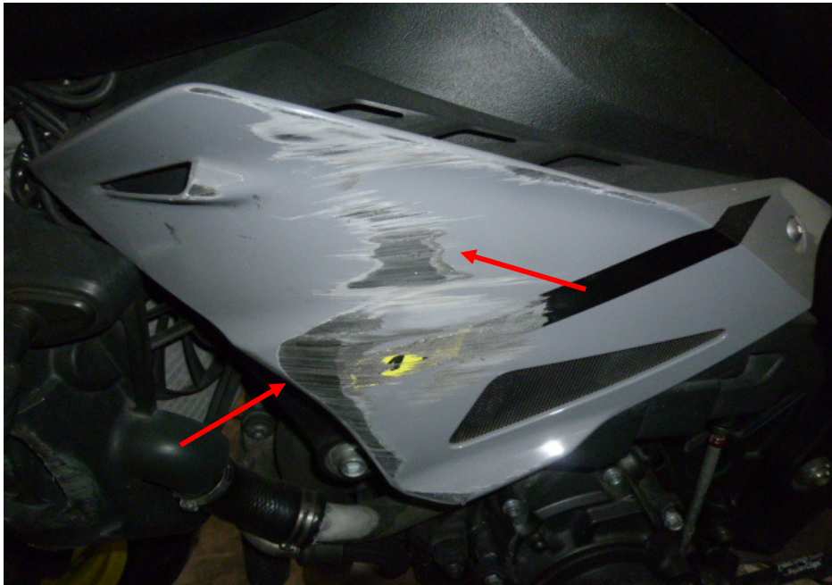
Photo 10 shows a closer view of the left cowling which was amongst the body parts of the Motorcycle that had sustained damages of grazing nature as a result of the accident (arrowed).
