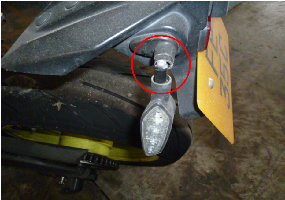
Photo 12 shows a closer view of the dislodged left rear signal lamp of the Motorcycle as a result of the accident (circled).
