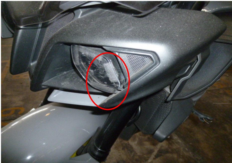
Photo 5 shows a close up view of the head cowling was amongst the body parts of the Motorcycle that had sustained damage as a result of the accident (circled).
