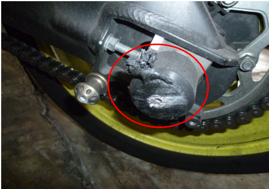
Photo 11 shows a closer view of the left rear axle slider (circled) which was amongst the body parts of the Motorcycle that had sustained damages of grazing nature as a result of the accident.
