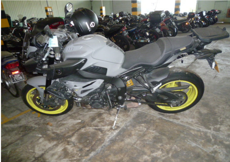
Photo 4 shows a general view of the left body of the Motorcycle at the time of our inspection. The Motorcycle was observed to have sustained damages at its frontal portion and left body. The body parts that were found to have been damaged include its head cowling, front mudguard, left cowling, left radiator cover, left signal lamps, clutch lever, left side mirror and left front footrest, amongst others.
