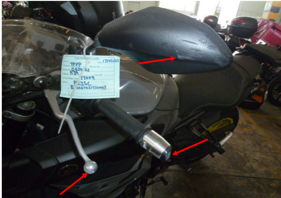
Photo 8 shows a closer view of the left handlebar end, clutch lever and left side mirror (arrowed) which were amongst the body parts of the Motorcycle that had sustained damage as a result of the accident.
