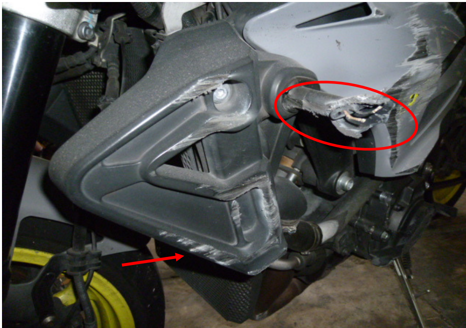
Photo 7 shows a closer view of the broken left front signal lamp (circled) and left radiator cover (arrowed) of the Motorcycle that had sustained damages of grazing nature as a result of the accident.
