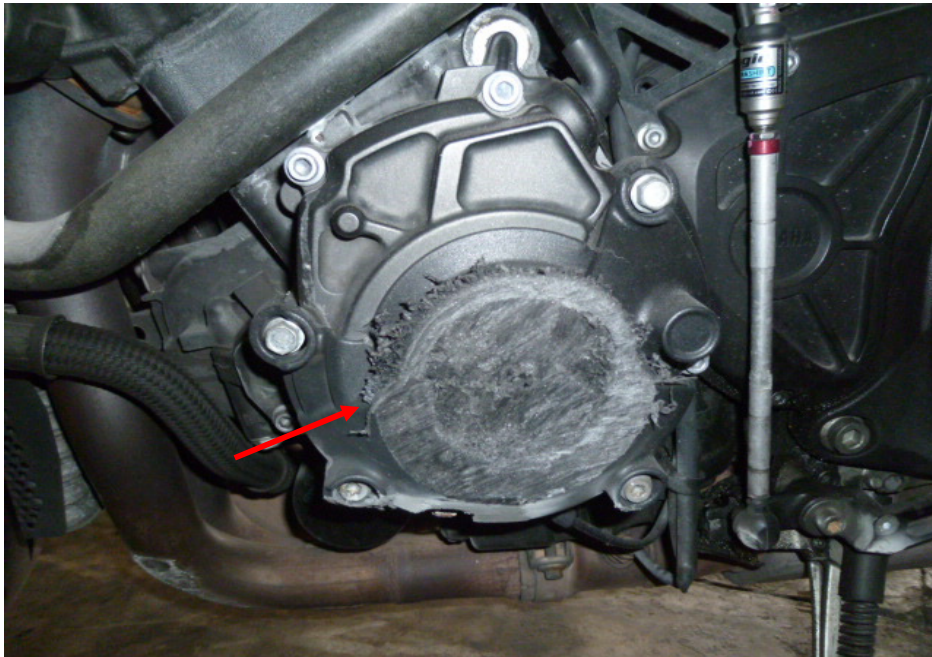
Photo 15 shows the left side of the engine of the Motorcycle at the time of our inspection. The various left engine components had sustained damage of grazing nature as a result of the accident (arrowed) however the engine components were still intact. There was also no fluid leak and/or fluid stain found around the left engine area of the Motorcycle.
