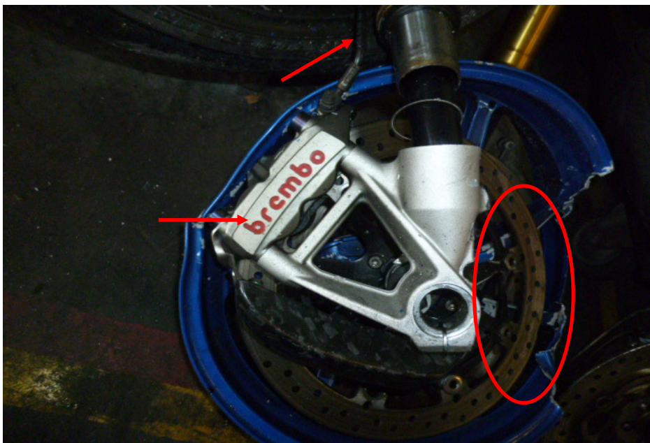
Photo 19 shows a close up view of the front brake caliper, front brake disc and front brake hose (arrowed) at the right side of the Motorcycle's front wheel, which are all part of the components in the hydraulic front brake system of the Motorcycle. Our visual checks of these various components had revealed all to be intact with no visible damage except for the front brake disc which was observed to be bent as a result of the accident (circled). No leakage of brake fluid was also observed.
