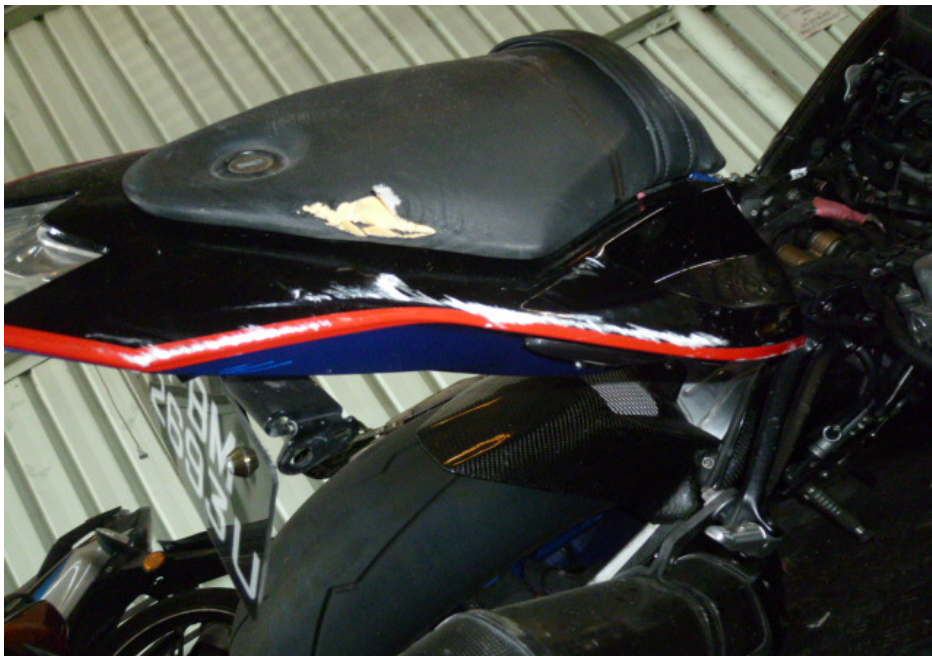
Photo 6 shows a closer view of the grazed right rear side cover of the Motorcycle as a result of the accident.
