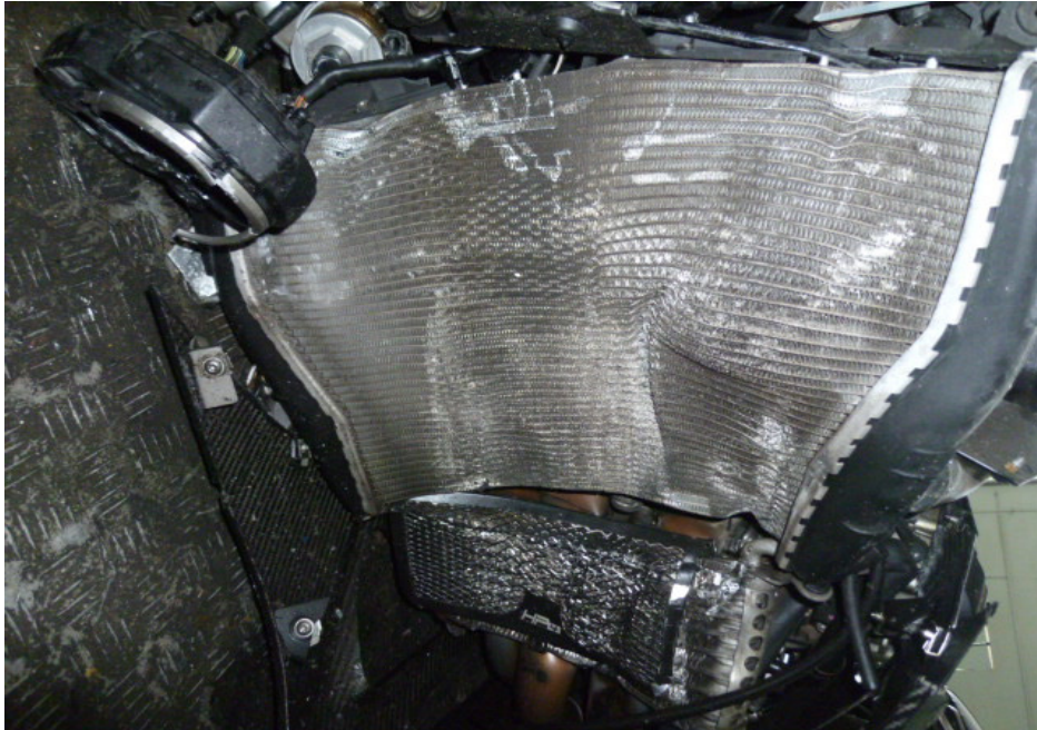
Photo 3 shows a closer view of the radiator which was amongst the body parts at the front body of the Motorcycle that had sustained damage as a result of the accident.
