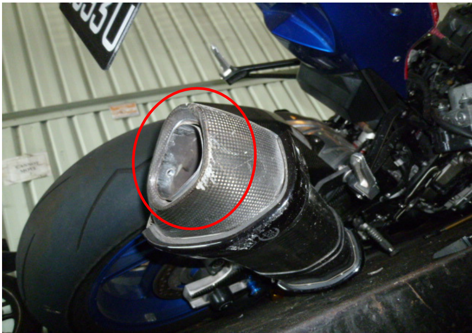
Photo 8 shows a closer view of the damaged exhaust muffler of the Motorcycle as a result of the accident (circled).
