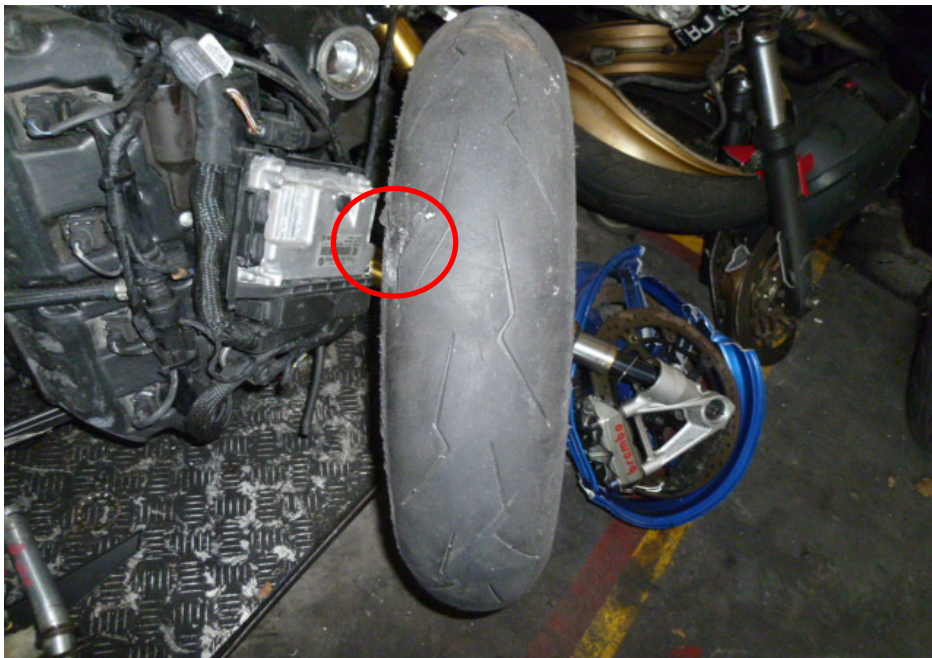
Photo 10 shows the condition of the Motorcycle's front tyre. The front tyre was observed to be in serviceable condition with remaining tread depth of approximately 3mm. The tyre was observed to be deflated. We also observed a tear on the right sidewall of the front tyre as a result of the accident (circled).
