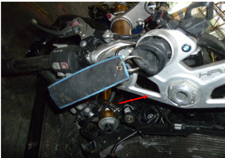
Photo 4 shows a closer view of the damaged top clamp the Motorcycle as a result of the accident (arrowed).
