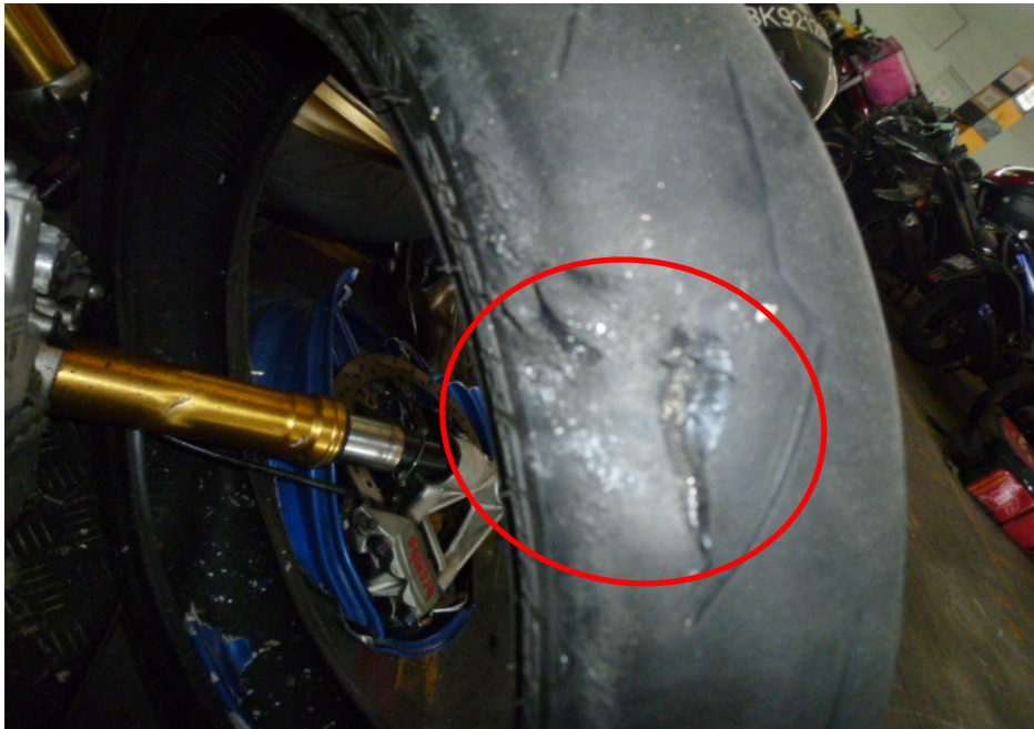
Photo 11 shows a closer view of the tear on the right sidewall of the front tyre as a result of the accident (circled).
