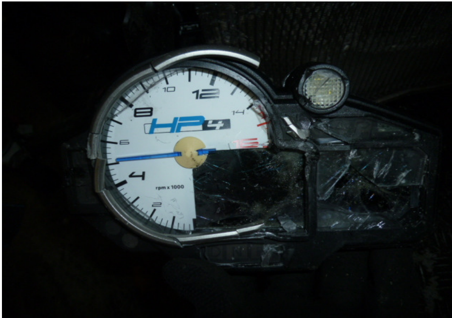
Photo 5 shows a closer view of the speedometer gauge of the Motorcycle. The mileage of the Motorcycle at the time of our inspection was not recorded due to the damage sustained to the speedometer gauge as a result of the accident.
