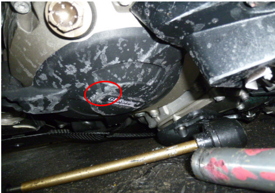
Photo 15 shows the right side of the engine of the Motorcycle at the time of our inspection. The various right engine components had sustained damage of grazing nature as a result of the accident (circled) however the engine components were still intact. There was also no fluid leak and/or fluid stain found around the right engine area of the Motorcycle.
