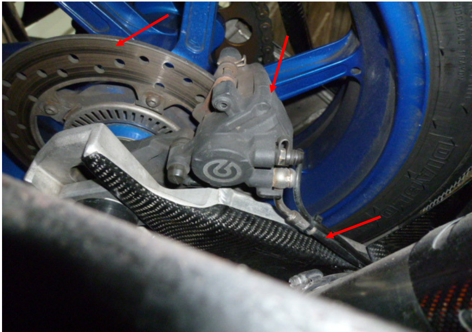
Photo 22 shows a close up view of the rear brake caliper, rear brake disc and rear brake hose (arrowed) of the Motorcycle, which are all part of the components in the hydraulic rear brake system of the Motorcycle. Our visual checks of these various components had revealed all to be intact with no visible damage. No leakage of brake fluid was also observed.
