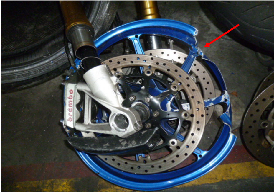
Photo 13 shows the broken front wheel rim of the Motorcycle as a result of the accident (arrowed) at the time of our inspection.
