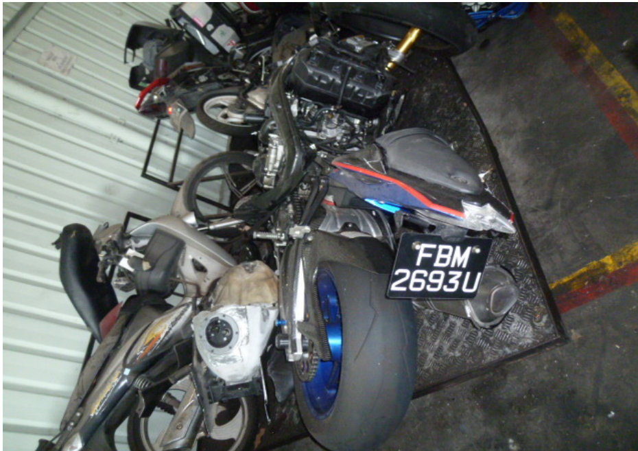
Photo 1 shows a general view of the rear portion of the Motorcycle at the time of our inspection. The Motorcycle had sustained damages all around. Body parts that were found to have been damaged include its top clamp, front fork assembly, radiator, speedometer gauge, left cowling, fuel tank, left front footrest, right rear side cover and exhaust muffler, amongst others.
