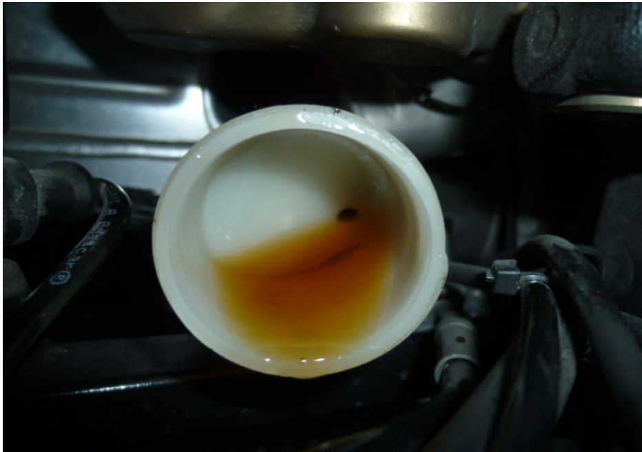
Photo 23 shows the brake fluid reservoir for the rear brake of the Motorcycle. The brake fluid was observed to be of sufficient level for operational purposes and without contamination.
