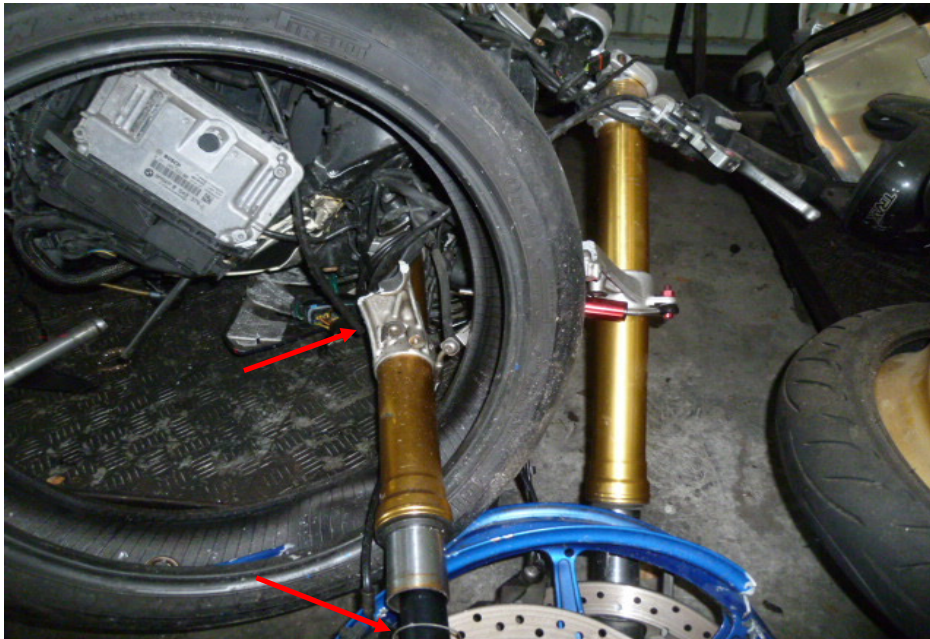
Photo 18 shows the front forks of the Motorcycle. The front forks were found to be broken as a result of the accident (arrowed) which had rendered the Motorcycle immobile. Hence we were not able to conduct any test(s) on the steering system of the Motorcycle.
