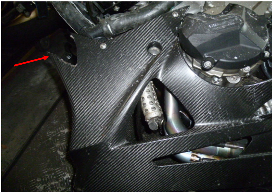
Photo 2 shows a closer view of the cracked left cowling which was amongst the body parts of the Motorcycle that had sustained damage as a result of the accident (arrowed).
