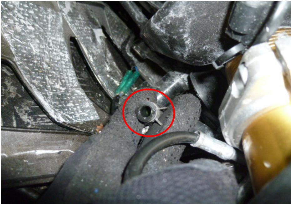
Photo 21 shows the missing front brake fluid reservoir of the Motorcycle at the time of our inspection (circled). Hence static brake tests conducted on the Motorcycle had appear to indicate that the front braking system of the Motorcycle was not in serviceable condition.
