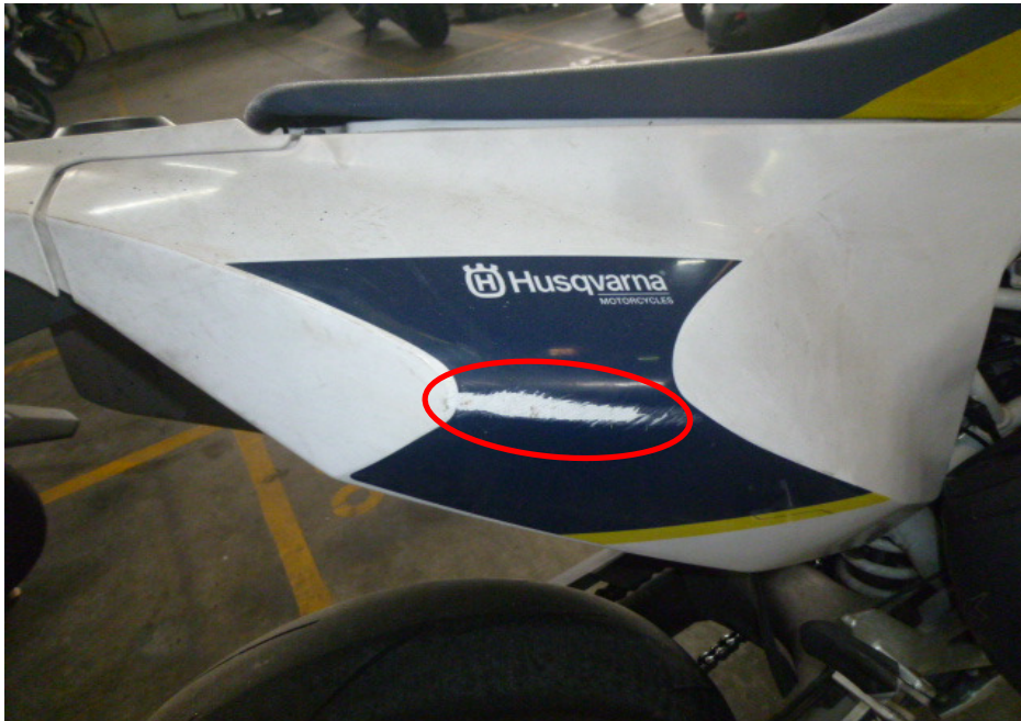
Photo 18 shows a closer view of right rear side cover which was amongst the body parts of the Motorcycle that had sustained damages of grazing nature as a result of the accident (circled).
