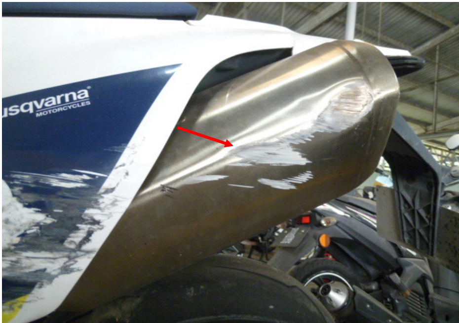
Photo 19 shows the exhaust muffler which was amongst the body parts of the Motorcycle that had sustained damage as a result of the accident.
