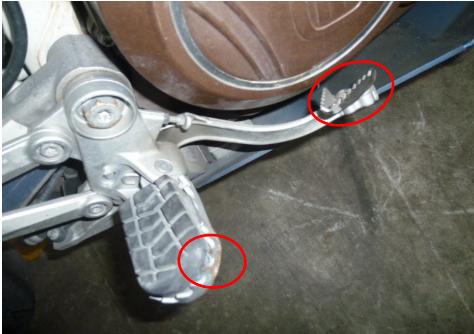
Photo 14 shows a closer view of the rear brake pedal and right front footrest (circled) which were amongst the body parts of the Motorcycle that had sustained damage as a result of the accident.
