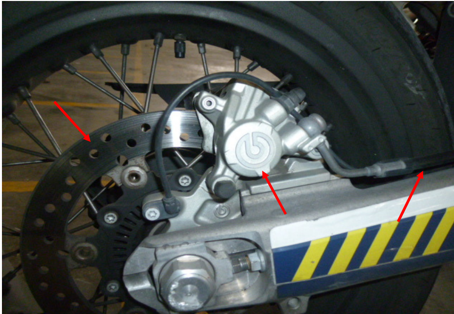
Photo 31 shows a close up view of the rear brake caliper, rear brake disc and rear brake hose (arrowed) of the Motorcycle, which are all part of the components in the hydraulic rear brake system of the Motorcycle. Our visual checks of these various components had revealed all to be intact with no visible damage. No leakage of brake fluid was also observed.
