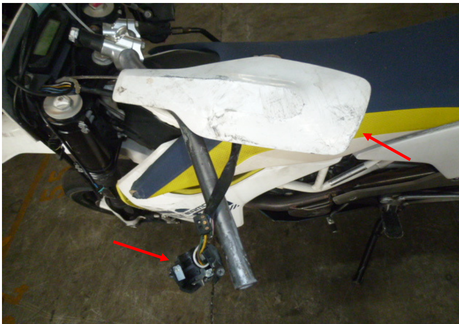
Photo 11 shows the missing clutch lever, left handlebar switch and clutch lever guard (arrowed), which were amongst the body parts of the Motorcycle that had sustained damage as a result of the accident.
