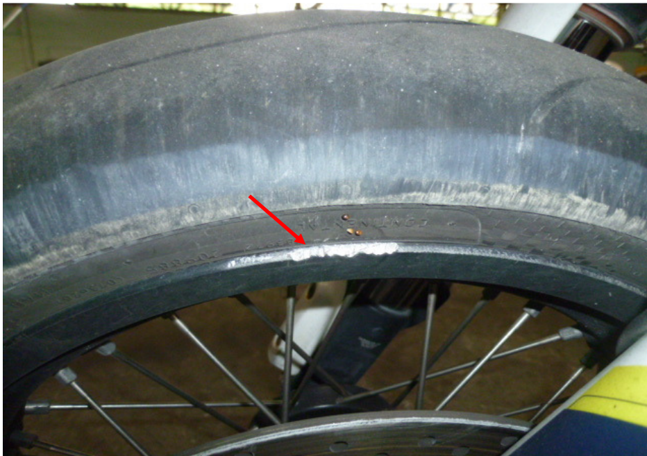
Photo 21 shows the front wheel rim of the Motorcycle which had sustained damages of grazing nature as a result of the accident (arrowed).
