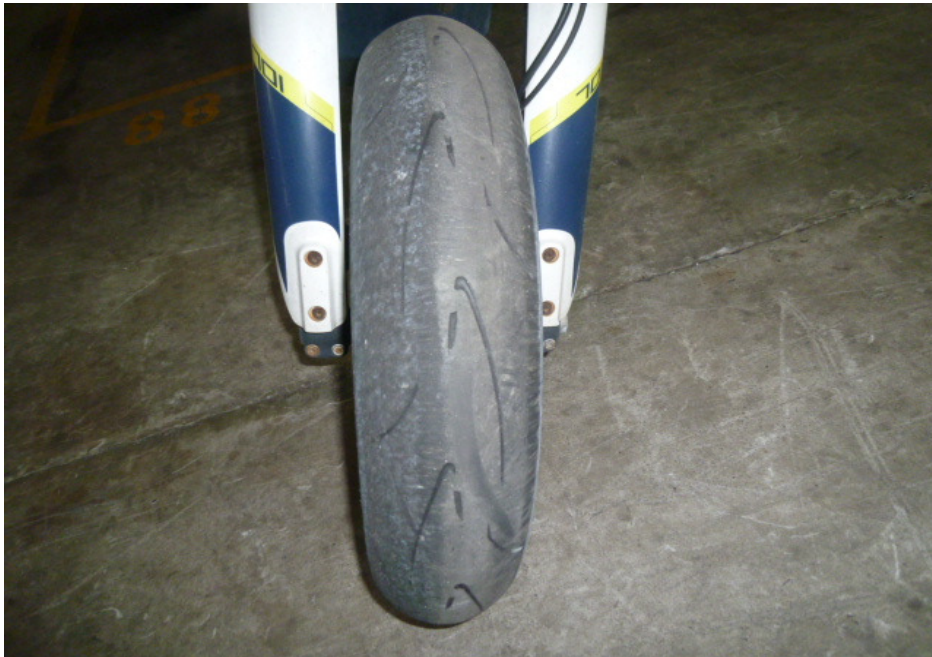
Photo 20 shows the front tyre of the Motorcycle at the time of our inspection. The front tyre was observed to be in serviceable condition with remaining tread depth of approximately 3mm. The pattern of the tread was also clearly visible. There was no tear, burst mark(s) and/or punctured hole(s) on the sidewalls as well as across the tread of the front tyre.
