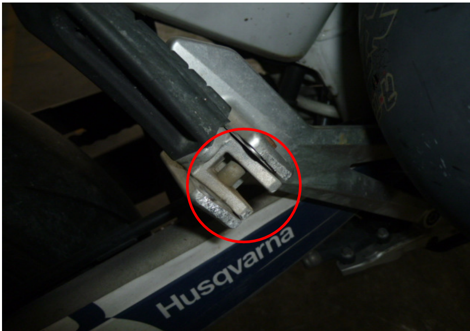
Photo 15 shows a closer view of the right pillion foot peg bracket (circled) which was amongst the body parts of the Motorcycle that had sustained damage as a result of the accident.
