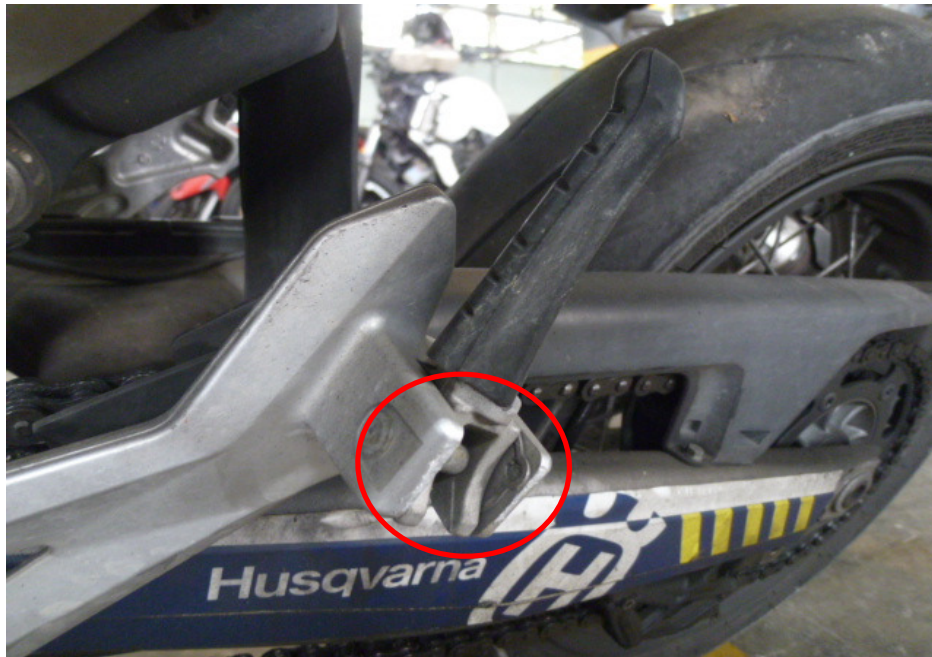
Photo 16 shows a closer view of the left pillion foot peg bracket (circled) which was amongst the body parts of the Motorcycle that had sustained damage as a result of the accident.
