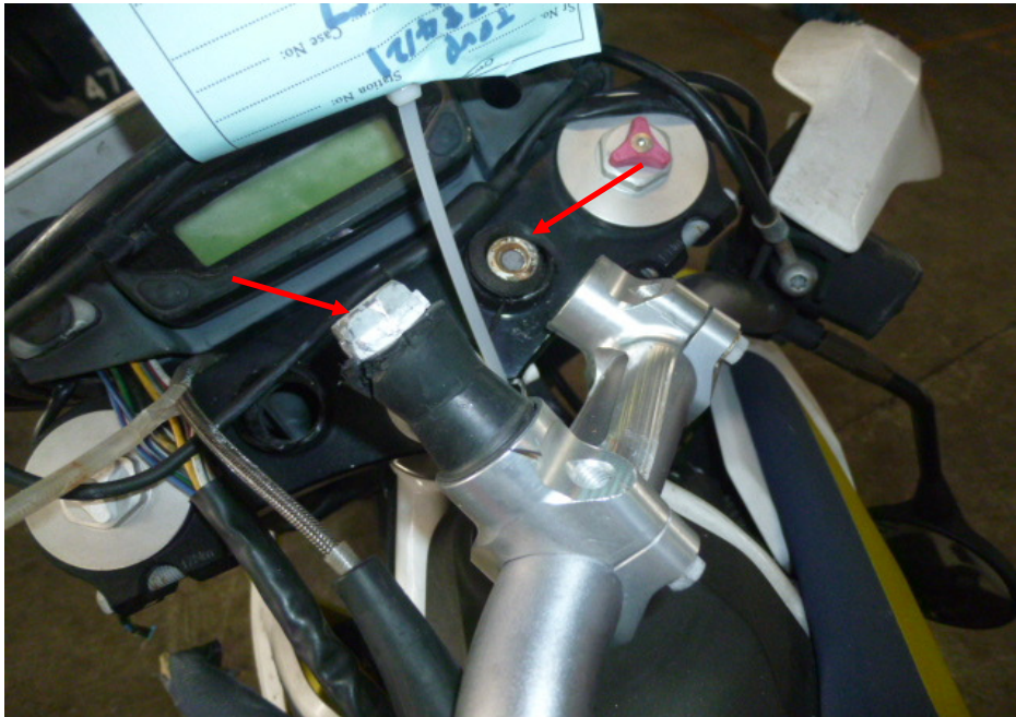
Photo 27 shows the handlebar clamp of the Motorcycle which was broken as a result of the accident (arrowed). We were hence not able to turn the handlebar of the Motorcycle towards the left or right.
