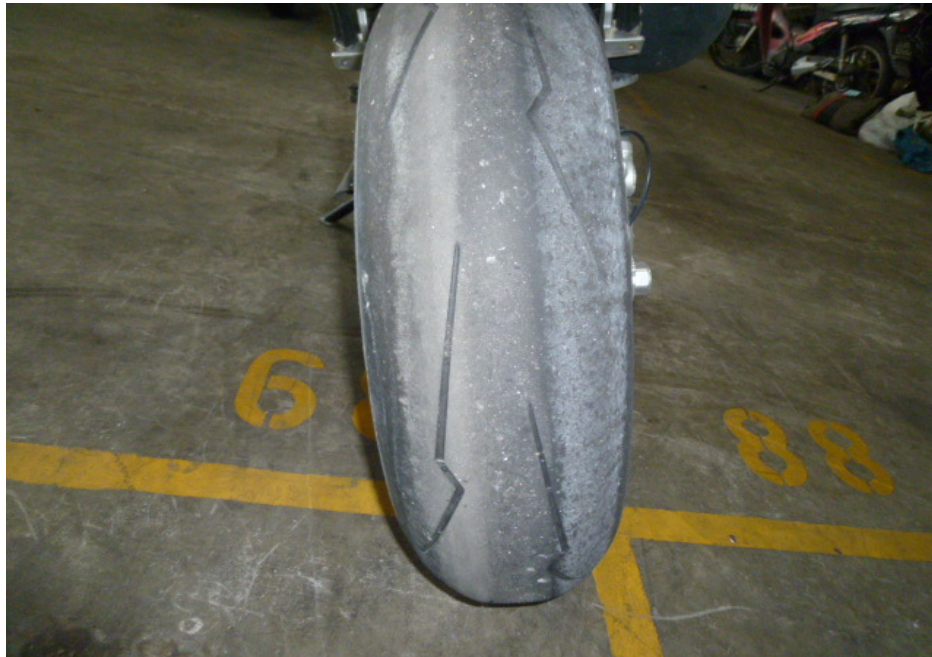
Photo 22 shows the condition of the Motorcycle's rear tyre. The rear tyre was observed to be in serviceable condition with remaining tread depth of approximately 3mm. The tyre was also observed to be sufficiently inflated for vehicular operation. We did not observe any tear, burst mark(s) and/or punctured hole(s) on the sidewalls as well as across the tread of the rear tyre.
