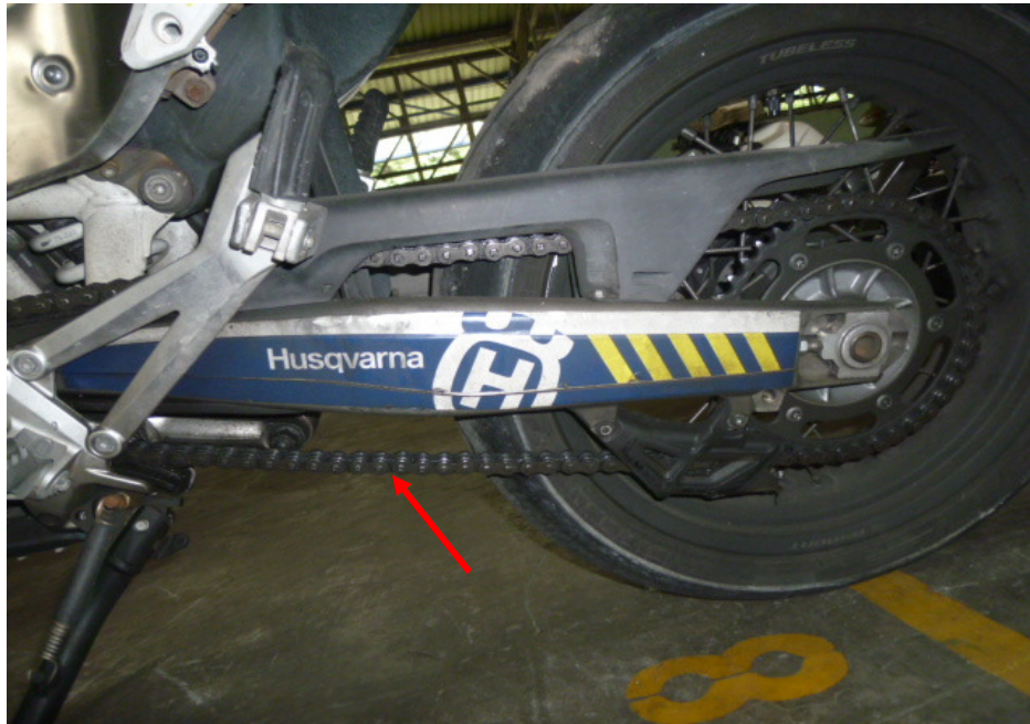
Photo 25 shows the general view of the gear train (arrowed) of the Motorcycle, which was observed to be intact with no misalignment. It was also adequately lubricated for operating purposes.
