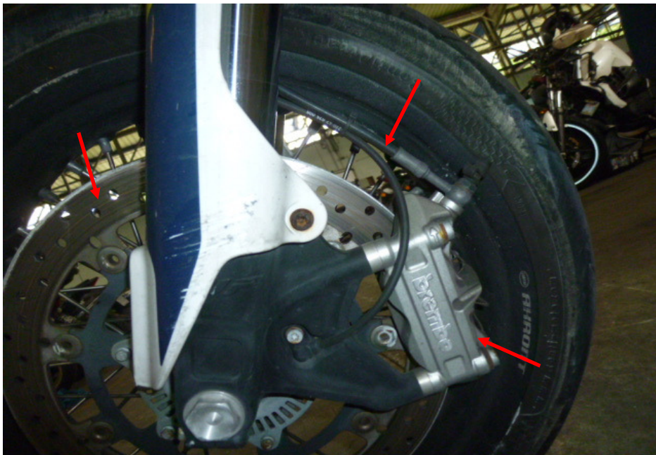
Photo 30 shows a close up view of the front brake caliper, front brake disc and front brake hose (arrowed) of the Motorcycle, which are all part of the components in the hydraulic front brake system of the Motorcycle. Our visual checks of these various components had revealed all to be intact with no visible damage.
