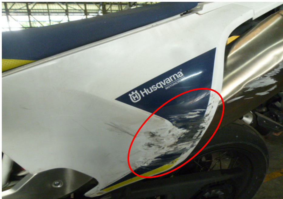
Photo 17 shows a closer view of left rear side cover which was amongst the body parts of the Motorcycle that had sustained damages of grazing nature as a result of the accident (circled).
