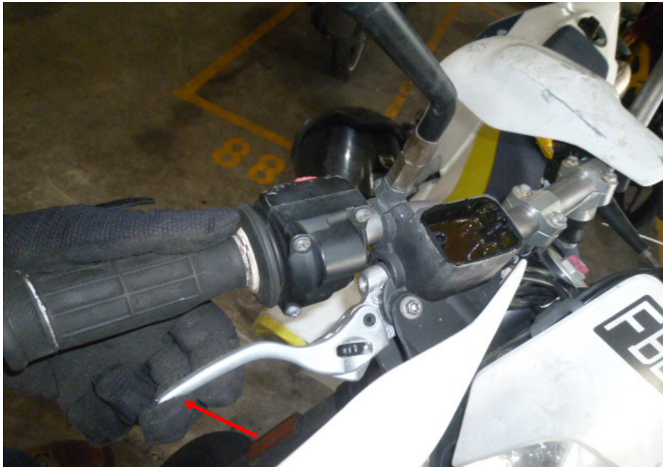
Photo 29 shows the front brake lever being depressed. There was some resistance felt (spongy like feel) upon pressing the front brake lever (arrowed). This would indicate that there is no leakage of pressure/vacuum in the front brake system.
