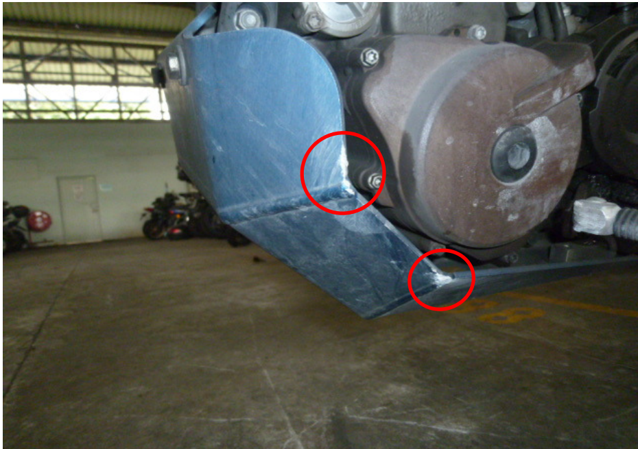
Photo 10 shows a closer view of the belly pan (circled) which was amongst the body parts of the Motorcycle that had sustained damage as a result of the accident.
