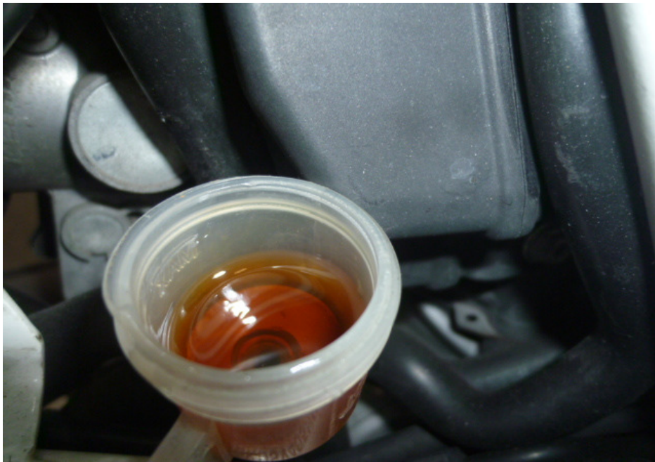
Photo 32 shows the brake fluid reservoir for the rear brake of the Motorcycle. The brake fluid was observed to be of sufficient level for operational purposes and without contamination.
