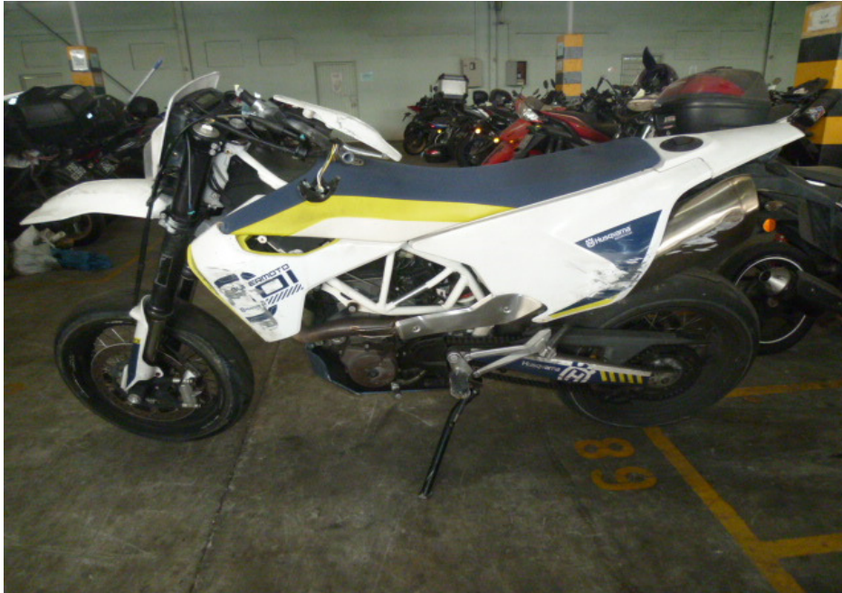
Photo 4 shows a general view of the left body of the Motorcycle at the time of our inspection. The Motorcycle was observed to have sustained damages all around. Amongst the body parts that were found to have been damaged include its head cowling, left cowling, front mudguard, front brake lever, belly pan rear brake pedal, right front footrest, rear side covers and exhaust muffler, amongst others.
