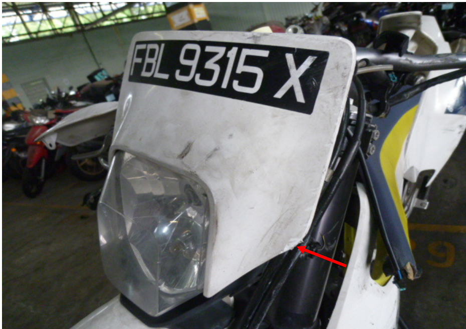
Photo 5 shows a close up view of the head cowling which was amongst the body parts of the Motorcycle that had sustained damage as a result of the accident (arrowed).
