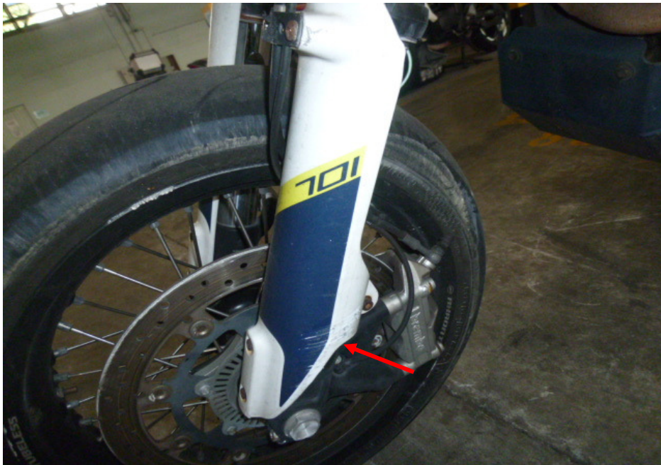
Photo 7 shows a closer view of the left lower front fork guard (arrowed) which was amongst the body parts at the front body of the Motorcycle that had sustained damage as a result of the accident.
