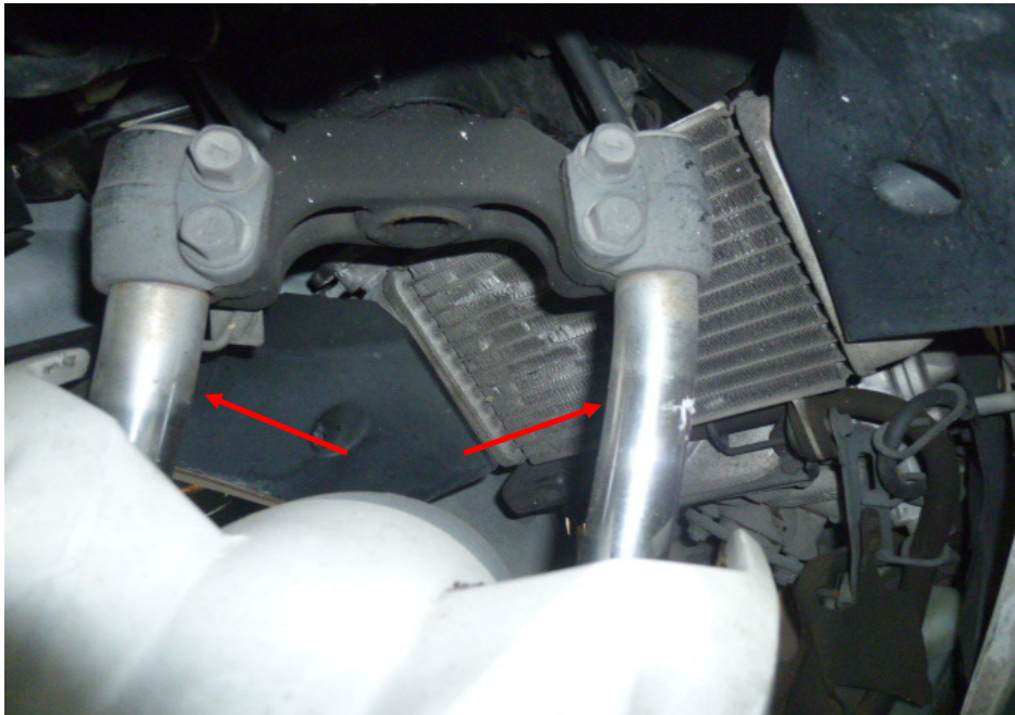
Photo 23 shows the front forks of the Motorcycle. The front forks (arrowed) were observed to be bent as a result of the accident. We were hence not able to conduct any tests on the steering system of the Motorcycle.
