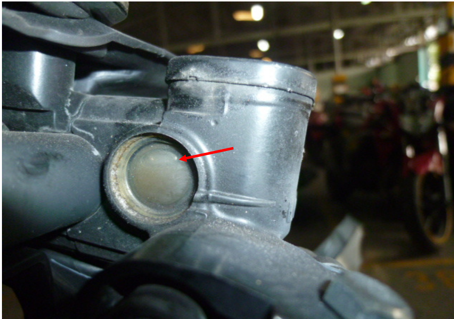
Photo 25 shows the brake fluid reservoir for the front brake of the Motorcycle. The brake fluid was observed to be of sufficient level (arrowed) and without contamination for operational purposes.
