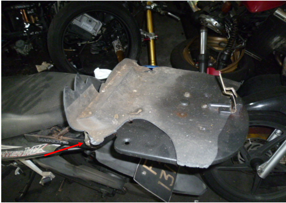
Photo 14 shows the broken top box rack of the Motorcycle at the time of our inspection (arrowed).
