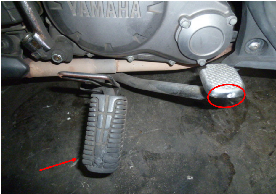
Photo 13 shows a closer view of the rear brake pedal (circled) and right front footrest (arrowed) which were amongst the body parts of the Motorcycle that had sustained damage as a result of the accident.
