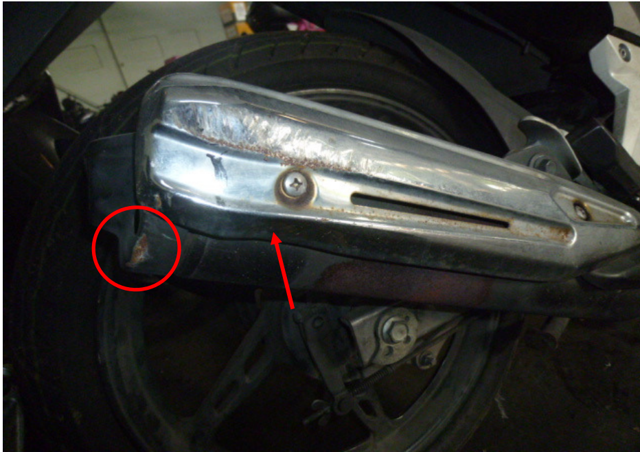
Photo 12 shows a closer view of the grazed exhaust muffler (circled) and dented exhaust muffler heat shield (arrowed) which were amongst the body parts of the Motorcycle that had sustained damage as a result of the accident.
