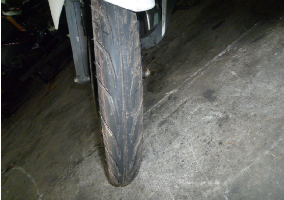
Photo 16 shows the condition of the Motorcycle's front tyre. The front tyre was observed to be in serviceable condition with remaining tread depth of approximately 3mm. We did not observe any tear, burst mark(s) and/or punctured hole(s) on the sidewalls as well as across the tread of the front tyre. However the front tyre was observed to be deflated as a result of the accident.
