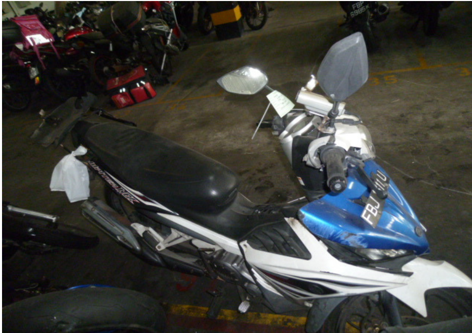
Photo 4 shows a general view of the right body of the Motorcycle at the time of our inspection. The Motorcycle had sustained damages all around. Body parts that were found to have been damaged include its headlight assembly, head cowl, front fork assembly, front mudguard, side cowlings, left side mirror, right rear side cover, rear brake pedal, right front footrest, rear number plate, top box rack, exhaust muffler and exhaust muffler heat shield, amongst others.
