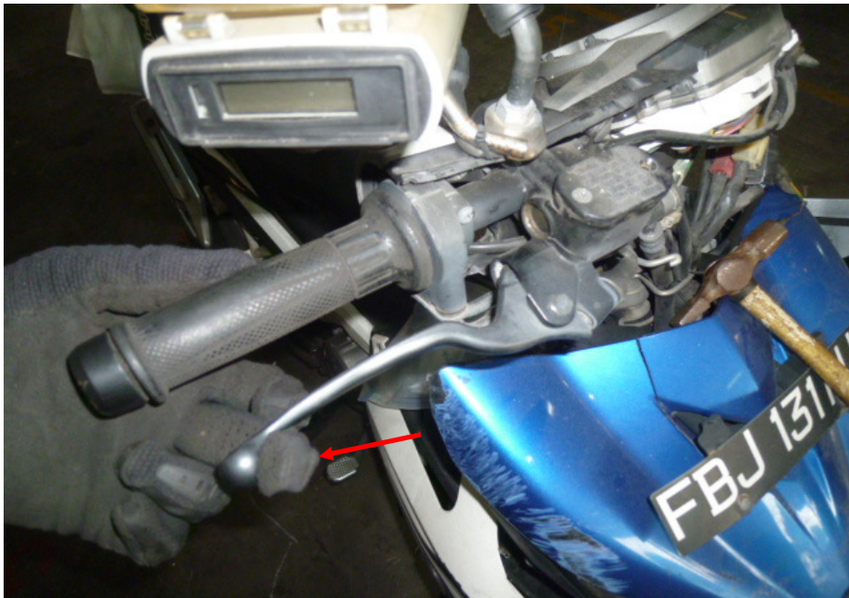
Photo 26 shows the front brake lever being depressed. There was some resistance felt (spongy like feel) upon pressing the front brake lever (arrowed). This would indicate that there is no leakage of pressure/vacuum in the brake system.
