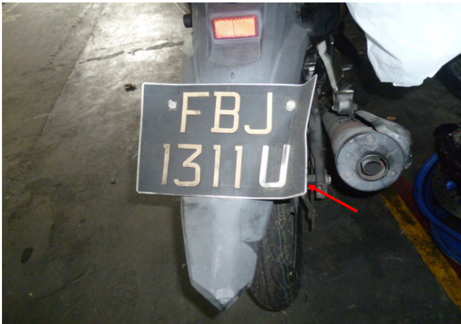
Photo 15 shows the dented rear number plate of the Motorcycle as a result of the accident (arrowed).
