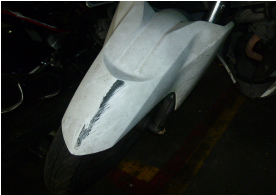
Photo 7 shows a closer view of the front mudguard, which was amongst the body parts of the Motorcycle that had sustained damage as a result of the accident.
