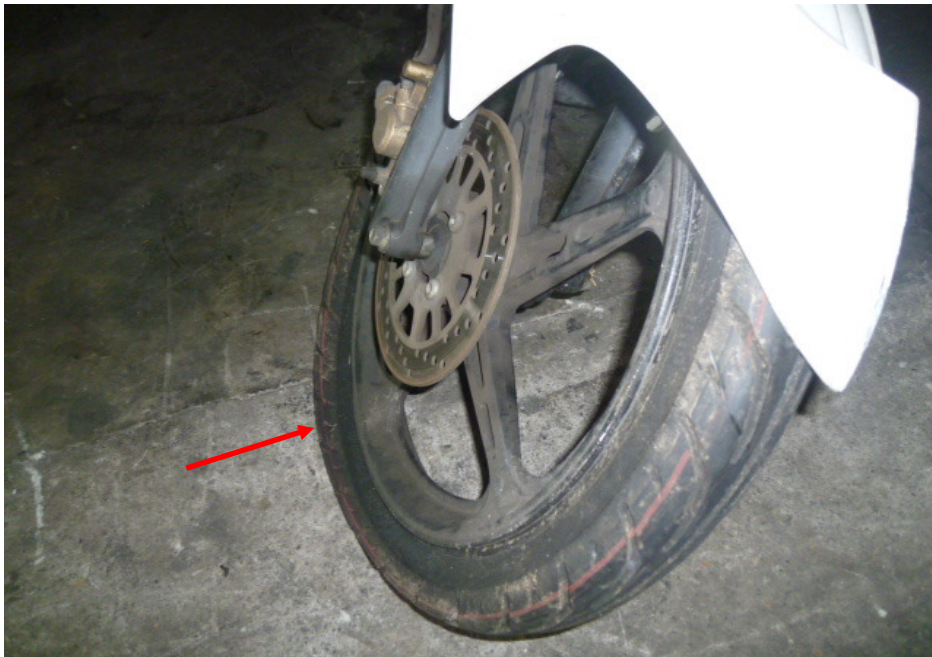
Photo 17 shows a closer view of the deflated front tyre of the Motorcycle as a result of the accident (arrowed).
