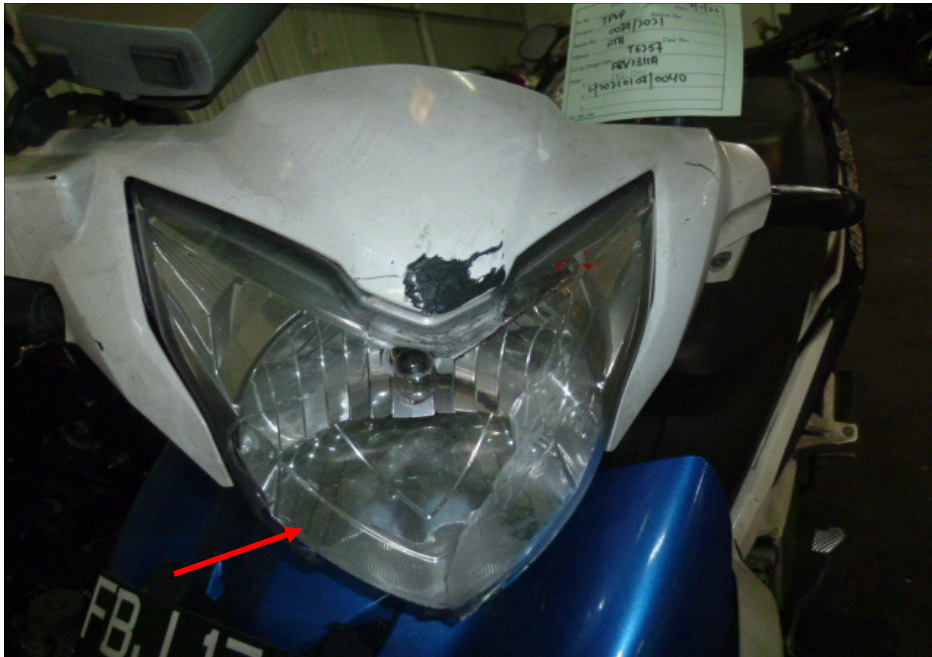
Photo 5 shows a closer view of the cracked headlight assembly of the Motorcycle as a result of the accident (arrowed).
