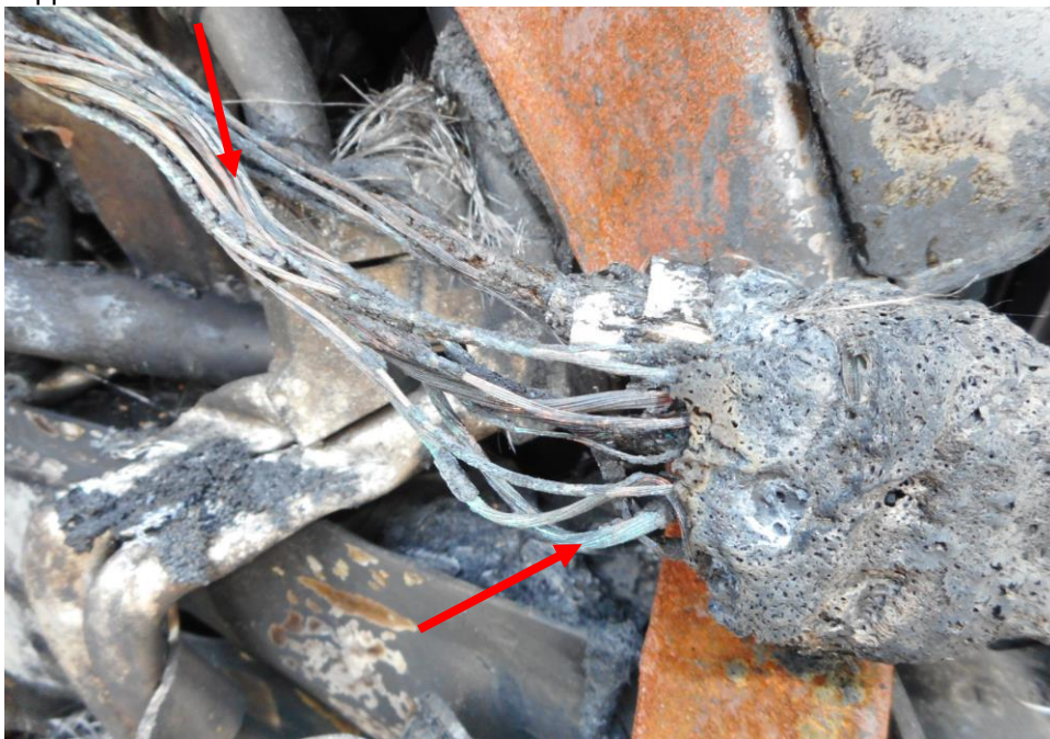
Photo 27 shows the close-up view of the headlamp assembly. Observed was greenish residue on the wiring harness leading (arrowed) from the fuse box to the headlamp assembly (arrowed). Observed was greenish residue on the wiring harness. The presence of greenish residue indicates internal heating of copper wires, a sign of an electrical short circuit occurring. The greenish residue is normally left behind from oxidation as a result of chemical reaction involving the copper wires.
