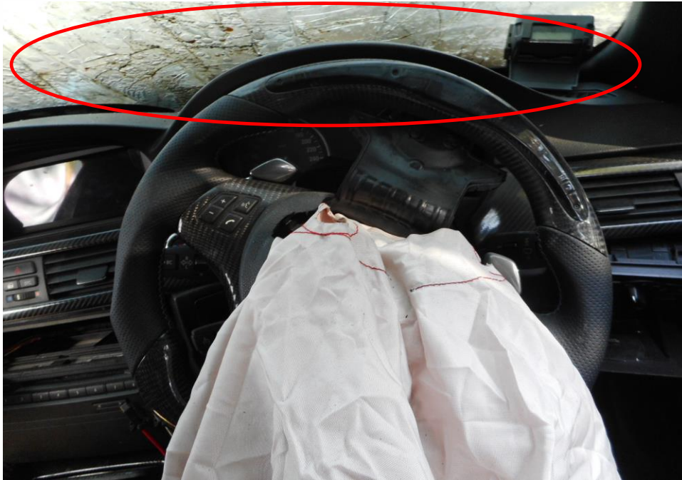
Photo 2 shows the close-up interior view of the front portion of the Insured Vehicle at the time of our inspection. The fire damage to the Insured Vehicle was confined to its front portion. As observed its front windscreen (circled) had suffered heat and smoke damage as a result of the fire.
