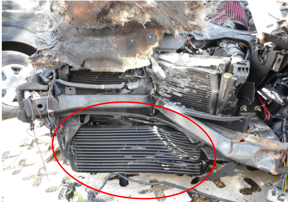
Photo 15 shows an aftermarket intercooler (circled) of the Insured Vehicle, which was observed to be damaged by the accident.
