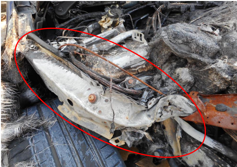
Photo 6 shows the close-up view of the front engine compartment portion of the Insured Vehicle at the time of our inspection. As observed whitish burn marks (circled) on the surface are a result of exposure to prolonged heat intensity as a result of the fire.
