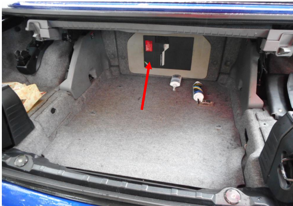
Photo 18 shows a general view of an additionally fitted audio amplifier system fitted at the boot of the Insured Vehicle, which was observed to be unaffected by the fire at the time of inspection.
