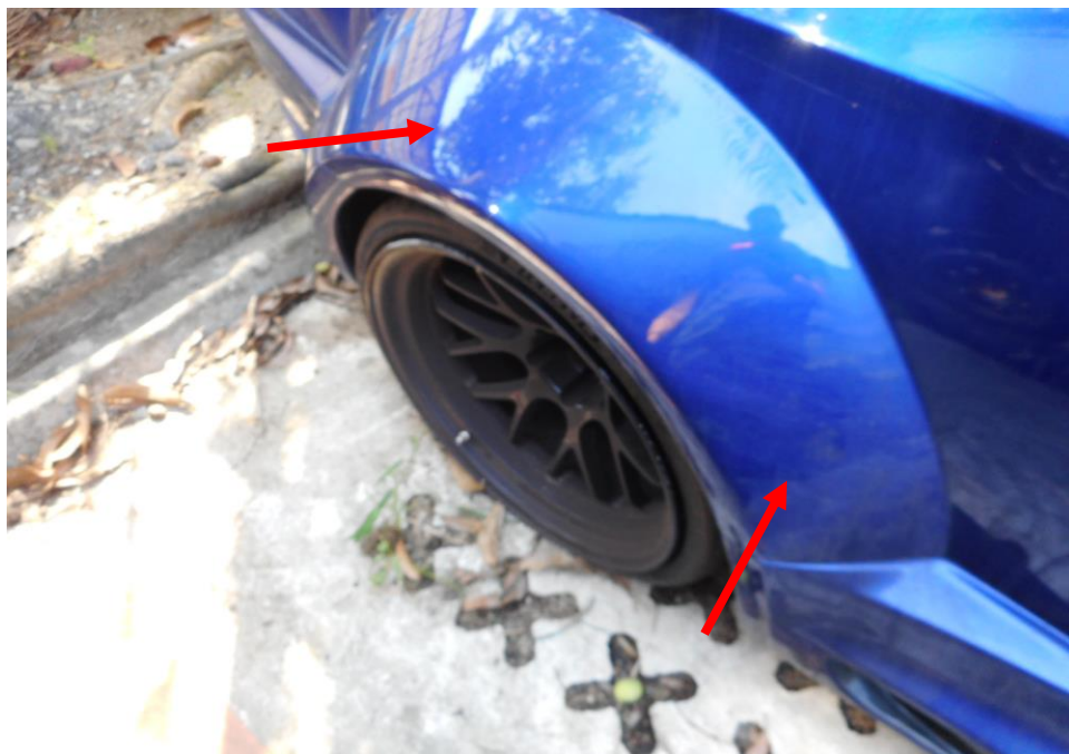
Photo 21 shows the close up view of the aftermarket wide body kit additional attachments (arrowed) fitted on the Insured Vehicle, which was observed to be protruding laterally out of the body of the Insured Vehicle.
