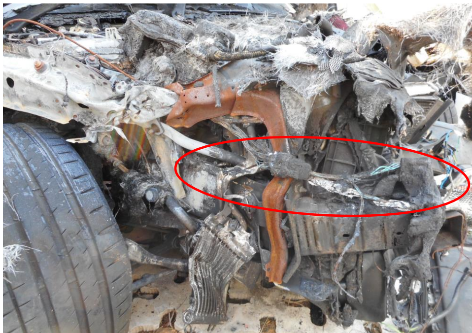
Photo 25 shows general view of the wirings leading from the fuse box to the headlamp assembly (circled). Both the fuse box to the headlamp assembly were factory fitted. The presence of greenish residue indicates internal heating of copper wires, a sign of an electrical short circuit occurring. The greenish residue is normally left behind from oxidation as a result of chemical reaction involving the copper wires.
