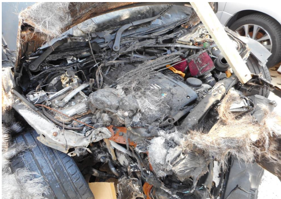
Photo 4 shows the general view of the engine compartment of the Insured Vehicle at the time of our inspection. The fire damage to the Insured Vehicle was confined to its front portion. This had included its right headlamp, bonnet, bumper and several parts inside the engine compartment were also observed to sustain heat damage. This includes the coolant fluid reservoir, brake fluid reservoir, ABS pump and its factory wiring harness are amongst the body parts that were found to have been affected as a result of the fire.
