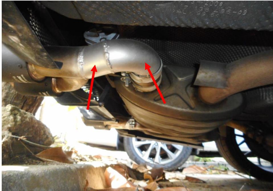
Photo 17 shows a modified exhaust system fitted on the Insured Vehicle, which was observed to be unaffected by the fire at the time of inspection.
