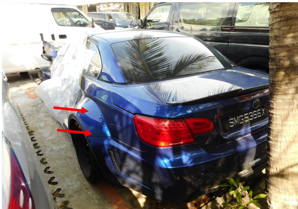
Photo 20 shows the general view of the aftermarket wide body kit additional attachments (arrowed) fitted on the Insured Vehicle, which was observed to be protruding laterally out of the body of the Insured Vehicle.
