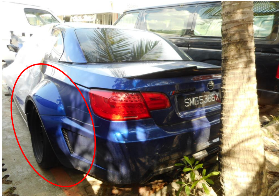
Photo 11 shows the aftermarket wide body kit (circled) of the Insured Vehicle, which was observed to be unaffected by the fire.
