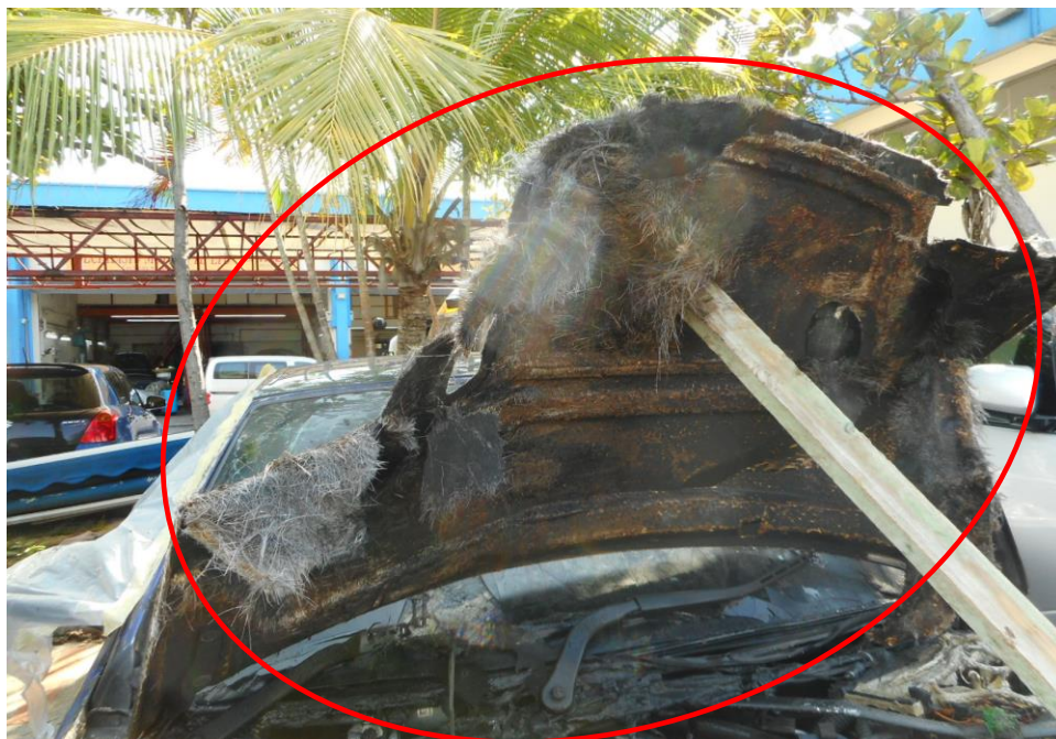
Photo 12 shows the aftermarket carbon fibre bonnet (circled) of the Insured Vehicle, which was observed to be damaged by the fire.
