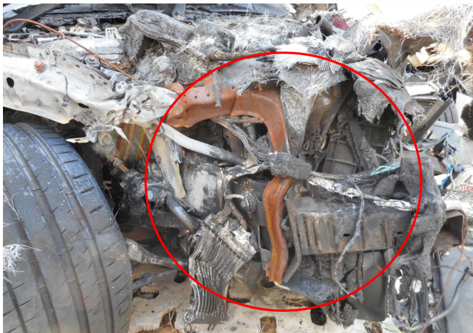
Photo 7 shows the close-up view of the front right head lamp portion of the Insured Vehicle at the time of our inspection. The whole of the head lamp including its housing and its factory wiring harness (circled) were damaged and melted down as a result of the fire.
