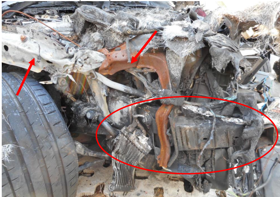
Photo 24 shows a close up view of the front right headlamp assembly (circled) and the various surrounding components. The headlamp assembly and various components were observed to be melted from the high heat intensity. Rust and high intensity burn marks (whitish burn marks) development was also observed on the metal brackets (arrowed) of the Insured Vehicle.
