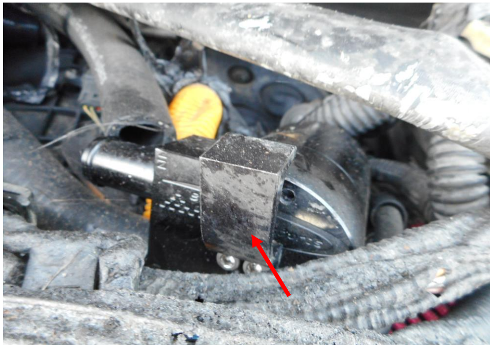
Photo 14 shows the additional fitted engine oil catch tank (arrowed) of the Insured Vehicle, which was observed to be damaged by the accident.
