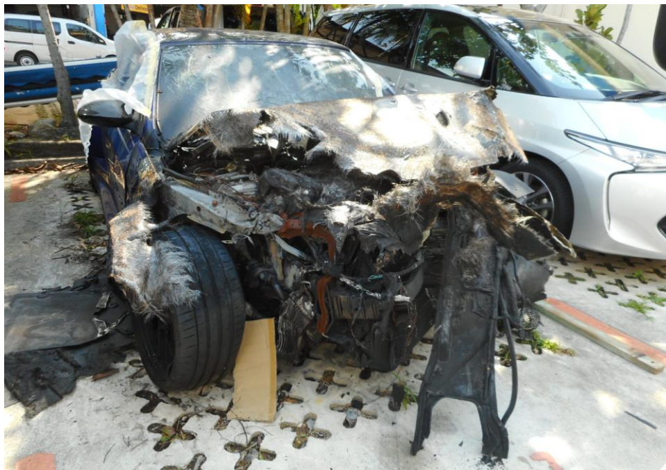
Photo 1 shows the general view of the front portion of the Insured Vehicle at the time of our inspection. The fire damage to the Insured Vehicle was confined to its front portion. This had included its front windscreen, right headlamp, bonnet, bumper and several parts inside the engine compartment were also observed to sustain heat damage. This includes the coolant fluid reservoir, brake fluid reservoir, ABS pump and its factory wiring harness are amongst the body parts that were found to have been affected as a result of the fire.
