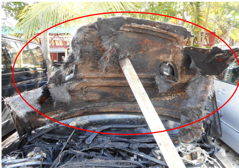
Photo 3 shows the close-up view of the front portion of the Insured Vehicle at the time of our inspection. The fire damage to the Insured Vehicle was confined to its front portion. As observed whitish burn marks (circled) on the surface are a result of exposure to prolonged heat intensity as a result of the fire.
