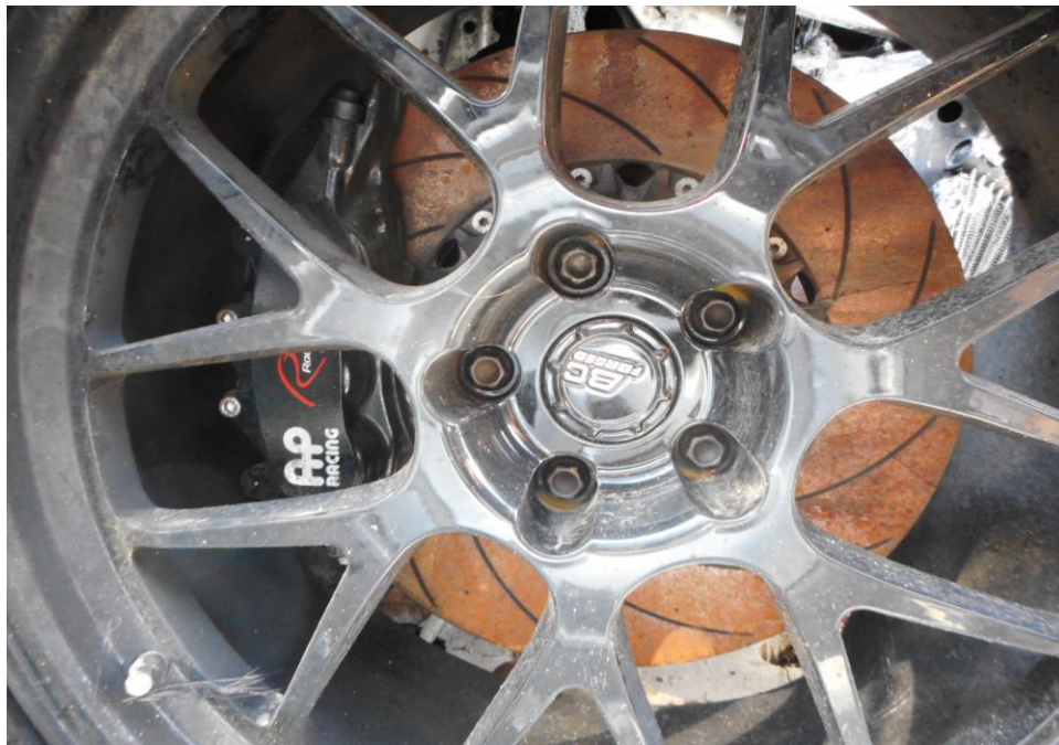
Photo 16 shows an aftermarket brake kit on of the Insured Vehicle, which was observed to be unaffected by the fire.
