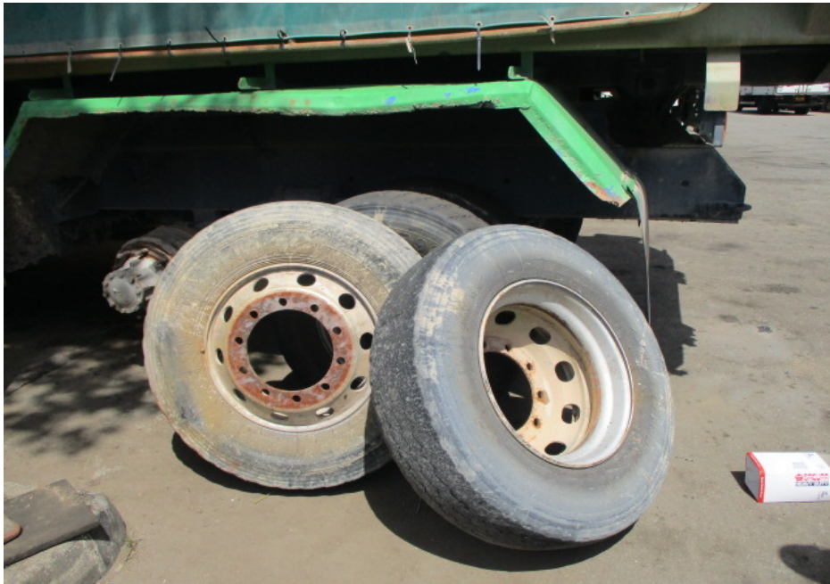
Photo 4 shows a general view of the left inner and outer tyres at the 2 nd axle of the Insured Vehicle that were retrieved from the container bin of the Insured Vehicle.
