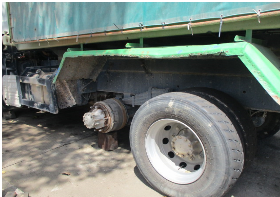
Photo 2 shows a closer view of the 2 nd axle and 3 rd axle at the left side of the Insured Vehicle. At the time of my inspection, the left inner and outer tyres at the 2 nd axle were not fitted on the Insured Vehicle.
