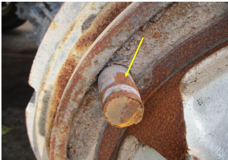
Photo 7 shows a closer view of the broken wheel bolt. Rust was seen on the tread area (arrowed) and broken surface area of the broken wheel bolt.
