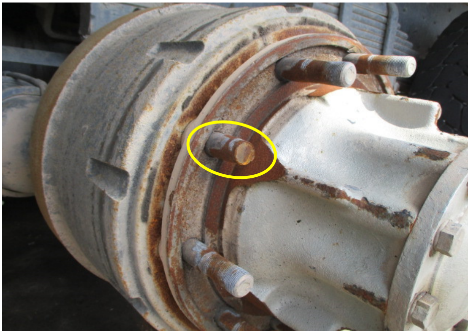
Photo 6 shows a general view of the broken wheel bolt (circled). Rust was seen on the tread area of the broken wheel bolt and similarly seen on the tread area of the remaining 9 unbroken wheel bolts. The broken surface area of the broken wheel bolt was also rusted.
