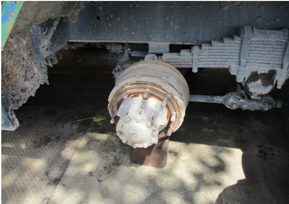
Photo 5 shows a general view of the wheel drum at the left side of the 2 nd axle of the Insured Vehicle at the time of my inspection. 10 bolts are used to fit the tyres to the wheel drum. Out of the 10 bolts, one bolt was broken. All 10 bolts were also observed to be not loosely fitted into their respective bolt holes.
