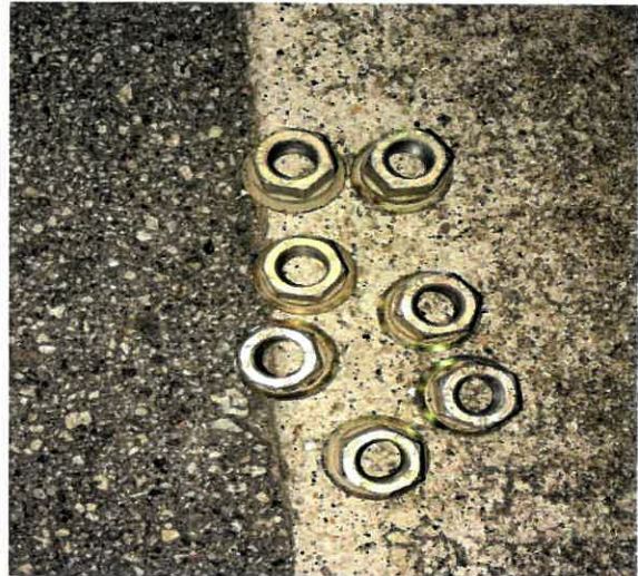
7 nuts retrieved after the accident with remaining scattered off
