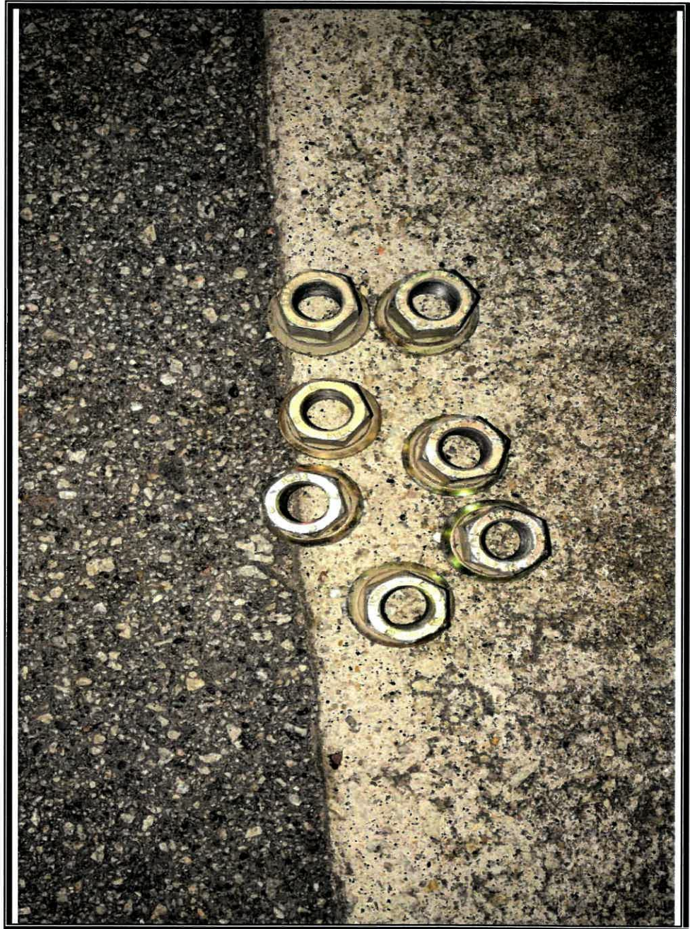
7 nuts retrieved after the accident with remaining scattered off
