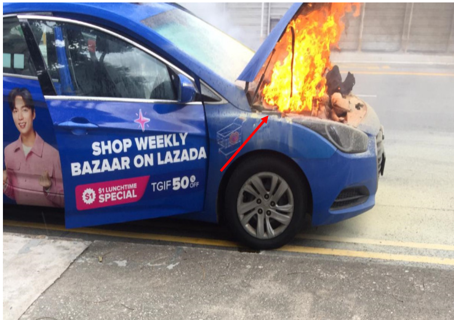
Photo 14 shows the Insured Vehicle on fire before the arrival of the SCDF. In general, the information that could be gathered from this photograph had corresponded to the events that were related to us by Mr Lim, which is the fire had started from the right portion of the engine compartment of the Insured Vehicle (arrowed).
