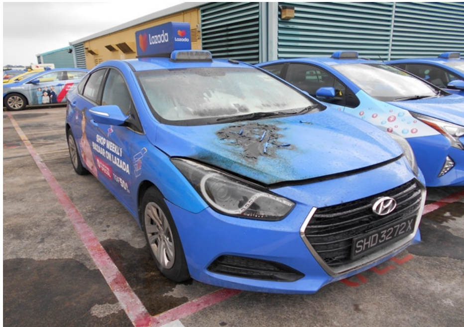
Photo 3 shows the closer view of the right front body of the Insured Vehicle at the time of our inspection. The fire damage to the Insured Vehicle was confined to its frontal portion. Its front bumper, front bonnet, front grille, front headlamps, front windscreen and front windscreen wipers were amongst the body parts that were found to have been affected by the fire.
