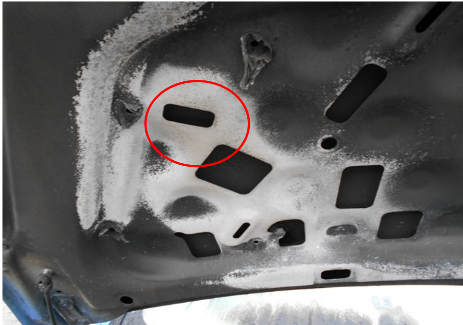
Photo 9 shows the rust that had developed on the underside of the front bonnet, around the right portion (circled). The development of rust is an indication that this area was subjected to prolonged exposure to high heat intensity, which had caused the steel/metal material of the front bonnet to be exposed to natural environmental condition. Hence the fire to the Insured Vehicle can be determined to have originated towards the right portion of the engine compartment.
