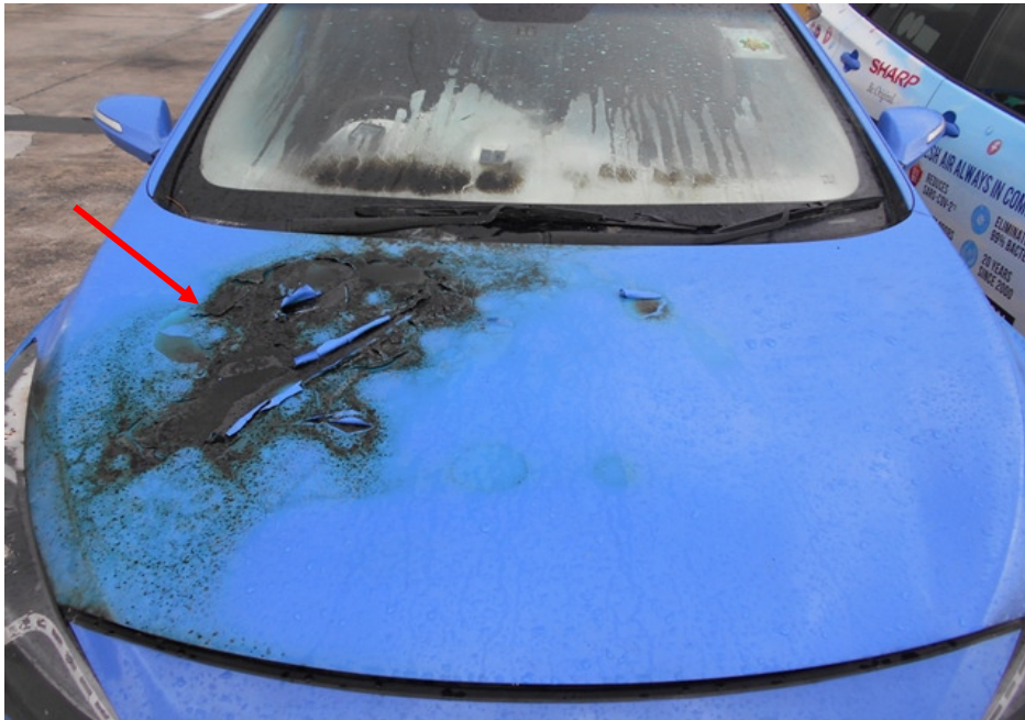
Photo 7 shows the burn pattern that was found on the right portion of the front bonnet of the Insured Vehicle (arrowed). Such whitish burn marks are a result of exposure to prolonged heat intensity, which may indicate where the fire had started. Rust would also begin to develop on these areas soon after the fire.
