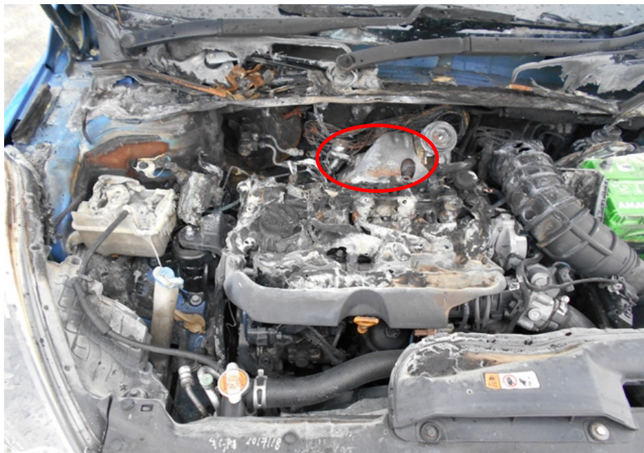
Photo 17 shows during our physical inspection of the Insured Vehicle, we observed that the turbocharger was fitted at the rear right portion of the engine compartment (circled) and this is in the immediate vicinity to where the fire had likely started.
