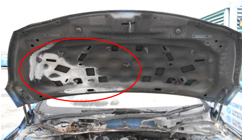
Photo 8 shows the whitish marks that were found on the underside of the front bonnet of the Insured Vehicle, at the right portion (circled). Such whitish burn marks are a result of exposure to prolonged heat intensity, which may indicate where the fire had started. Rust would also begin to develop on these areas soon after the fire.
