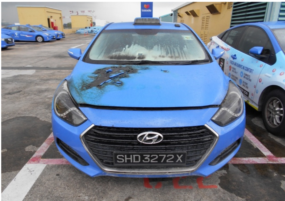
Photo 2 shows the general view of the frontal portion of the Insured Vehicle at the time of our inspection. The fire damage to the Insured Vehicle was confined to its frontal portion. The entire engine compartment of the Insured Vehicle was observed to be severely burnt while the interior compartment was observed to be severely affected by the fire.
