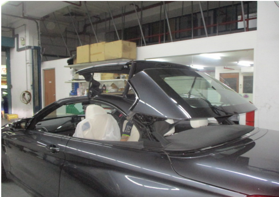
Photo 11 shows the Motor Car's hard top roof (convertible) being tested. It was observed that as a safety feature, the hard top roof could only open and close when the Motor Car was in a stationary position. When opened, the hard top roof is completely folded into the rear boot compartment with no parts protruding out of the Motor Car's body. It was also observed that during the folding and unfolding process, the hard top roof did not extend laterally beyond the Motor Car's body.
