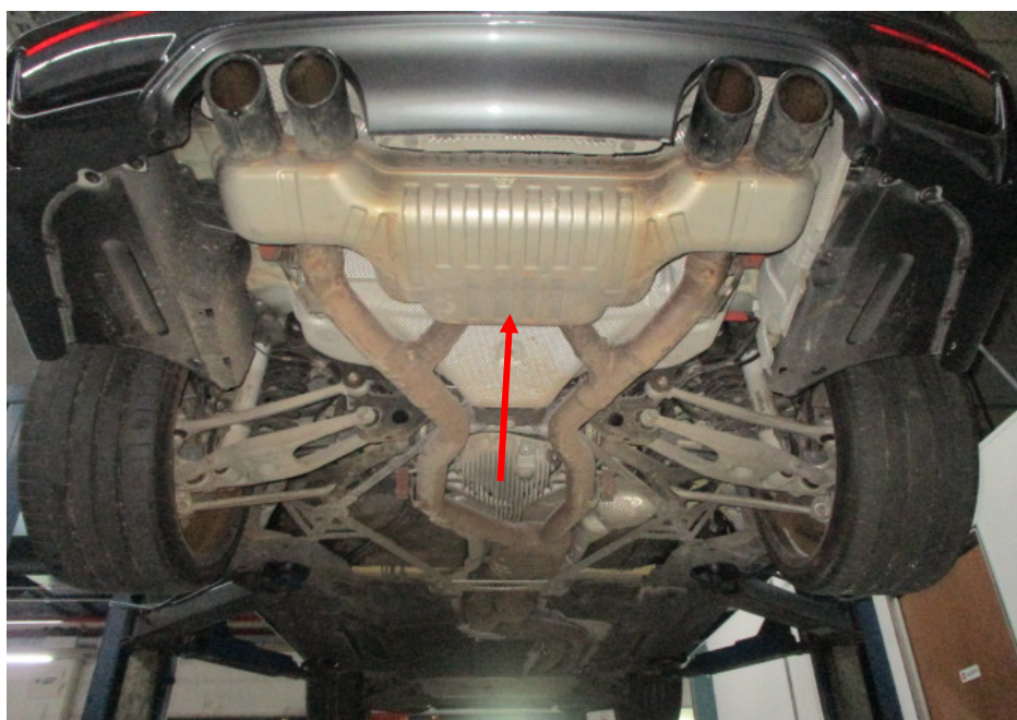
Photo 22 shows the Motor Car's rear muffler (arrowed). My examination of the Motor Car's exhaust system revealed no sign(s) or indication(s) of any cut or weld marks along its exhaust pipes and on its catalytic converters.
