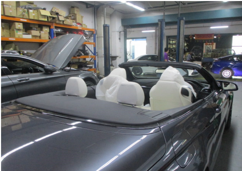
Photo 12 shows the Motor Car with its hard top roof completely folded. When opened, the hard top roof is completely folded into the rear boot compartment with no parts protruding out of the Motor Car's body. The hard top roof was also found adequately secured to the "A" pillar after closing.
