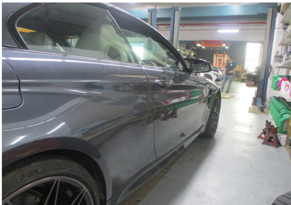
Photo 8 shows a closer view of the rear right body panel, front right door and right side rocker panel garnish of the Motor Car. The body parts at the right centre portion of the Motor Car were visually examined and it was observed that the repair/restoration works carried out to the damaged area of the Motor Car (refer to photograph 1 & 2 above) were reasonably adequate and in order.
