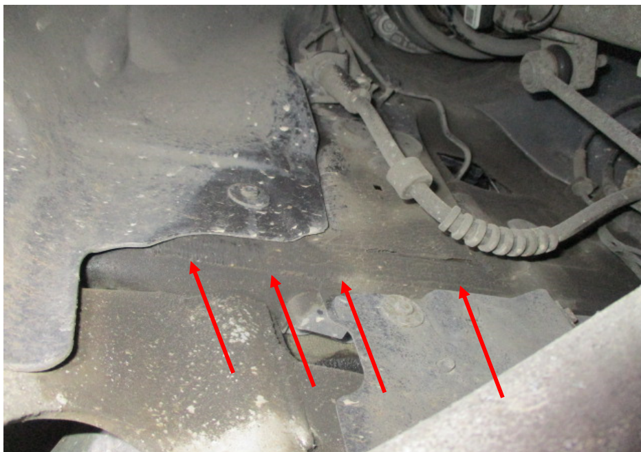
Photo 25 shows the chassis/structural body at the underside front left of the Motor Car. I did not find any weld marks other than original spot weld marks on the chassis/structural body of the Motor Car. The original factory sealant (arrowed) at the joints along the chassis/structural body was also untouched, indicating no work was done on the chassis/structural body of the Motor Car and that the chassis/structural body was originally fitted.
