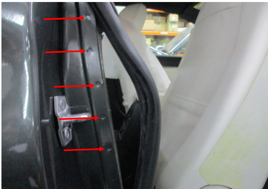
Photo 27 shows the right side rear body panel of the Motor Car. I did not find any weld marks other than original spot weld marks (arrowed) on the right side rear body panel of the Motor Car which, indicates that there was no re-welding works carried out. In general, I had found all the non-detachable body panels of the Motor Car to be originally fitted at the time of my inspection.
