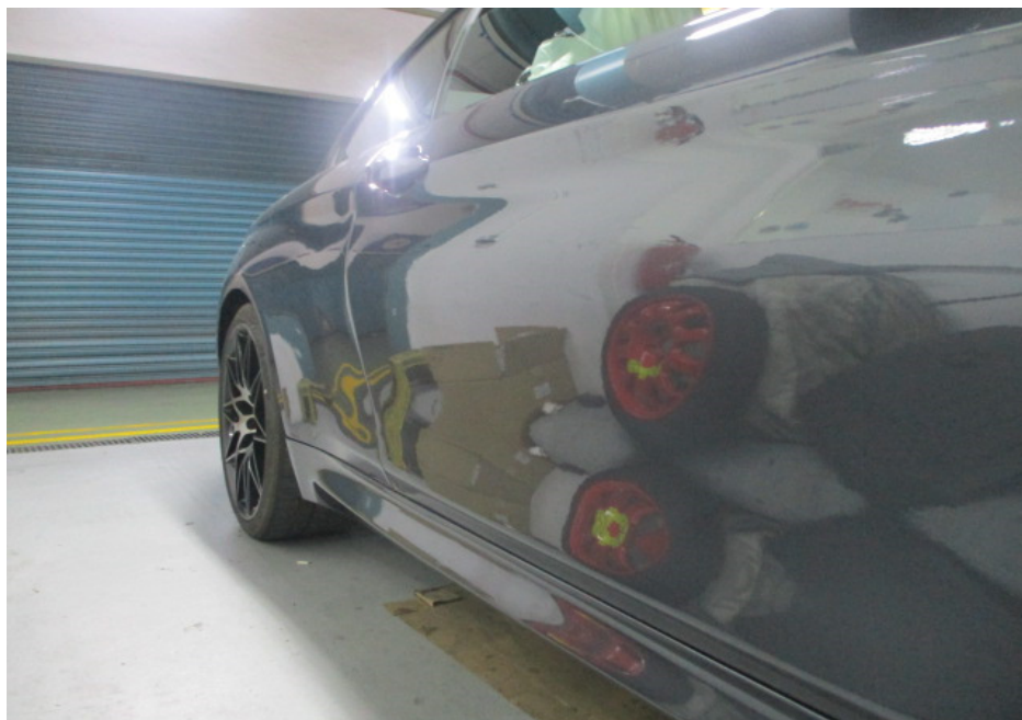
Photo 7 shows a closer view of the front right door and right side rocker panel garnish of the Motor Car. The body parts at the right centre portion of the Motor Car were visually examined and it was observed that the repair/restoration works carried out to the damaged area of the Motor Car (refer to photograph 1 & 2 above) were reasonably adequate and in order.
