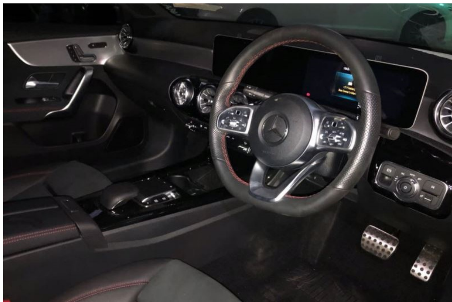
Photo 5 shows the front dashboard of the Motor Car (photograph provided to me). The interior compartment of the Motor Car was observed to be intact and unaffected. The airbags of the Motor Car were also not deployed.
