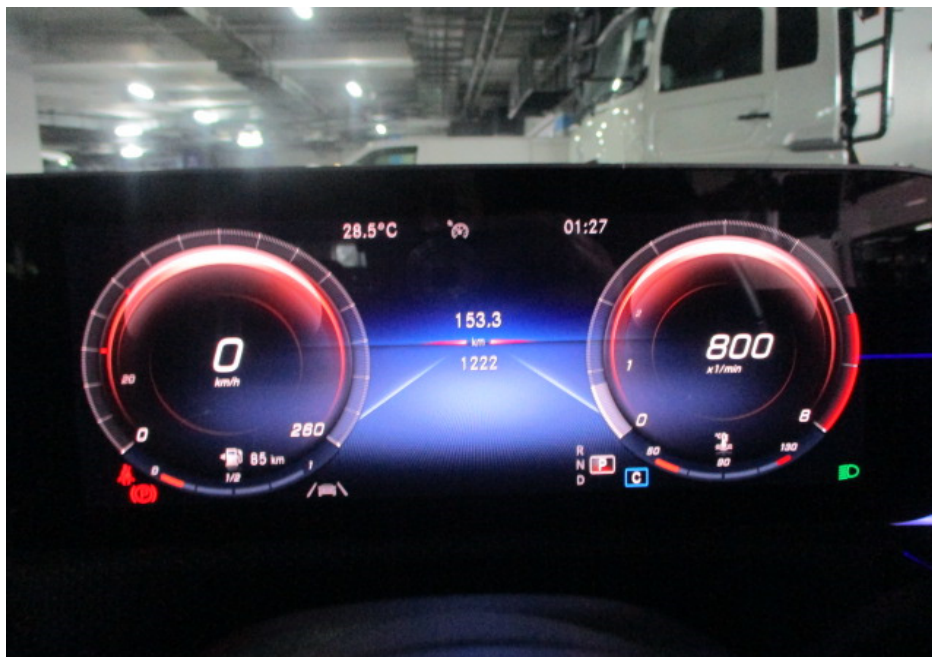
Photo 16 shows the respective warning lights no longer illuminated, indicating that there is no fault detected to the ABS, SRS, EPS and TCS systems of the Motor Car during the self-test. These electronic systems were hence in working condition at the time of my inspection.
