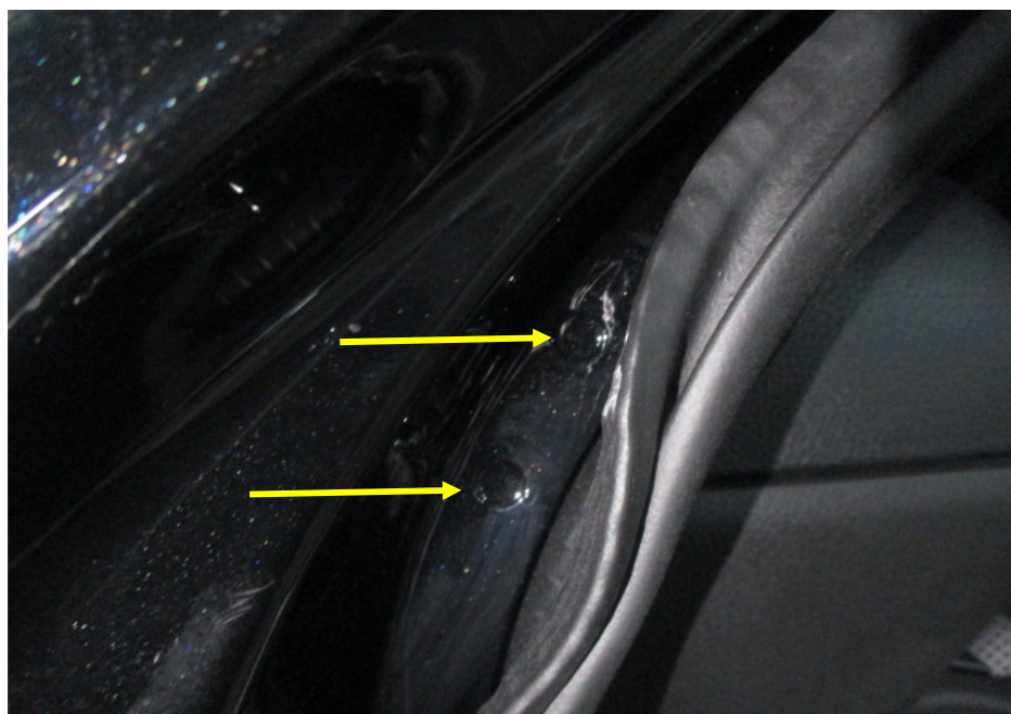
Photo 25 shows the left side "A" pillar of the Motor Car. I did not find any weld marks other than original spot weld marks (arrowed) on the left side "A" pillar of the Motor Car which, indicates that there was no re-welding works carried out. In general, I had found all the non-detachable body panels of the Motor Car to be originally fitted at the time of my inspection.
