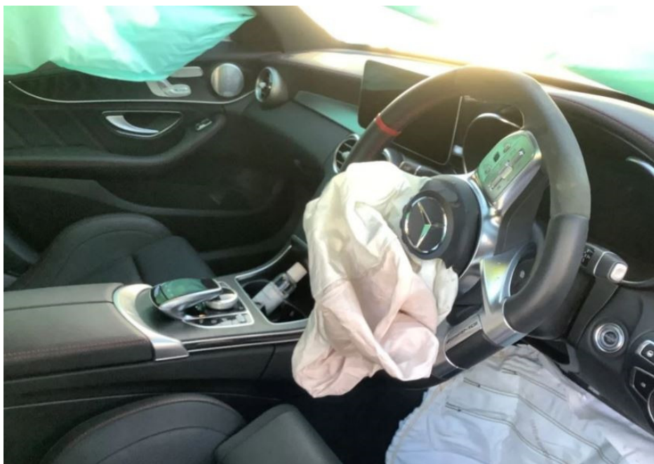
Photo 4 shows the interior compartment of the Motor Car prior to any repairs being carried out (photograph provided to me). The driver's airbag, driver's knee airbag, right side curtain airbag and left side curtain airbags were deployed as seen from the photographs that were provided to me.
