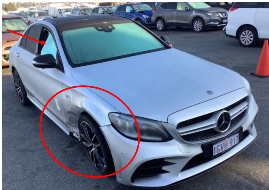
Photo 1 shows the front right body of the Motor Car prior to any repairs being carried out (photograph provided to me). The Motor Car was observed to have sustained damages at its right front portion (circled). The front bumper, front right fender, front right wheel, front right door and right side rocker panel garnish were amongst the body parts that were observed to have been damaged. The right side curtain airbag (arrowed) was observed to have been deployed.
