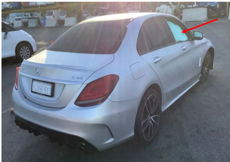
Photo 3 shows the rear right body of the Motor Car (photograph provided to me). Apart for the right front portion, there was no physical damage seen to other areas of the Motor Car. However, the right side curtain airbag (arrowed) was observed to have been deployed.
