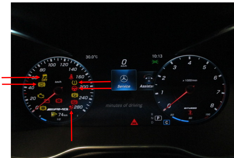
Photo 14 shows the warning lights for the various electronic safety features appearing on the instrument panel of the Motor Car during its self-test when the engine is cranked, in particular the ABS, SRS, EPS, TPM and TCS lights (arrowed).
